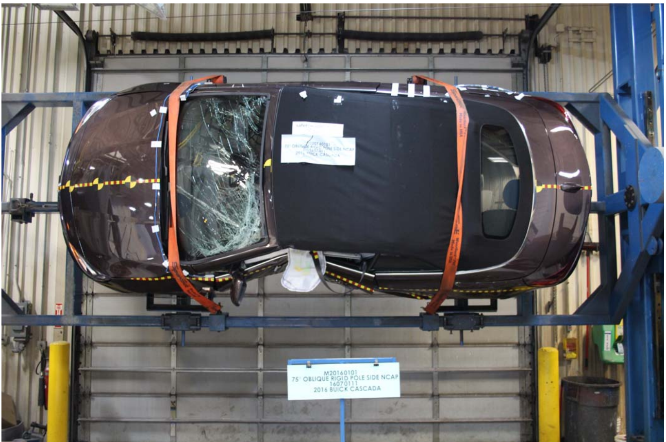
Photo No. 066 - FMVSS No. 301 Static Rollover 270 Degrees
