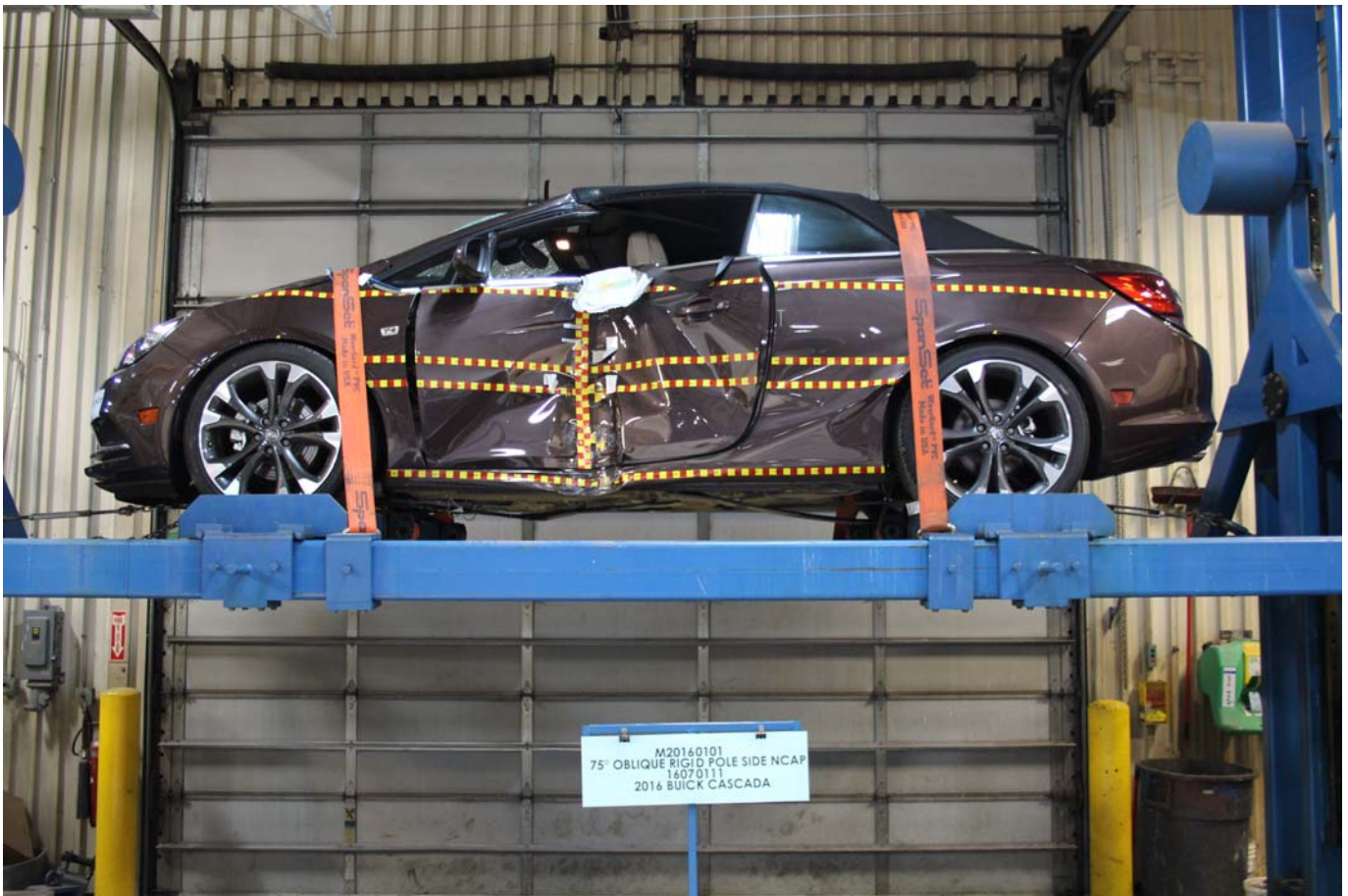
Photo No. 067 - FMVSS No. 301 Static Rollover 360 Degrees
