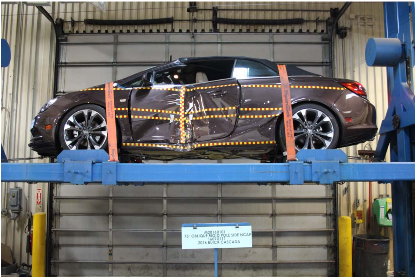
Photo No. 063 - FMVSS No. 301 Static Rollover 0 Degrees
