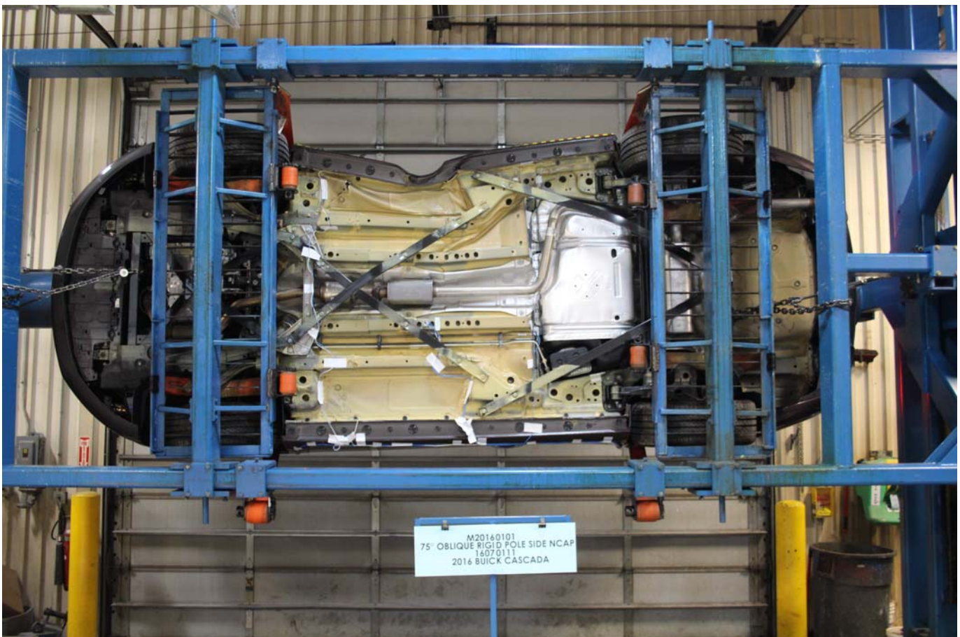
Photo No. 064 - FMVSS No. 301 Static Rollover 90 Degrees
