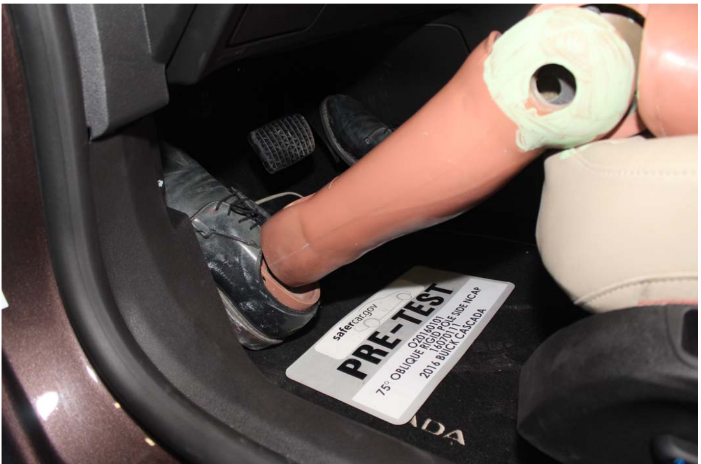
Photo No. 032 - Pre-Test Placement of Dummy's Feet
