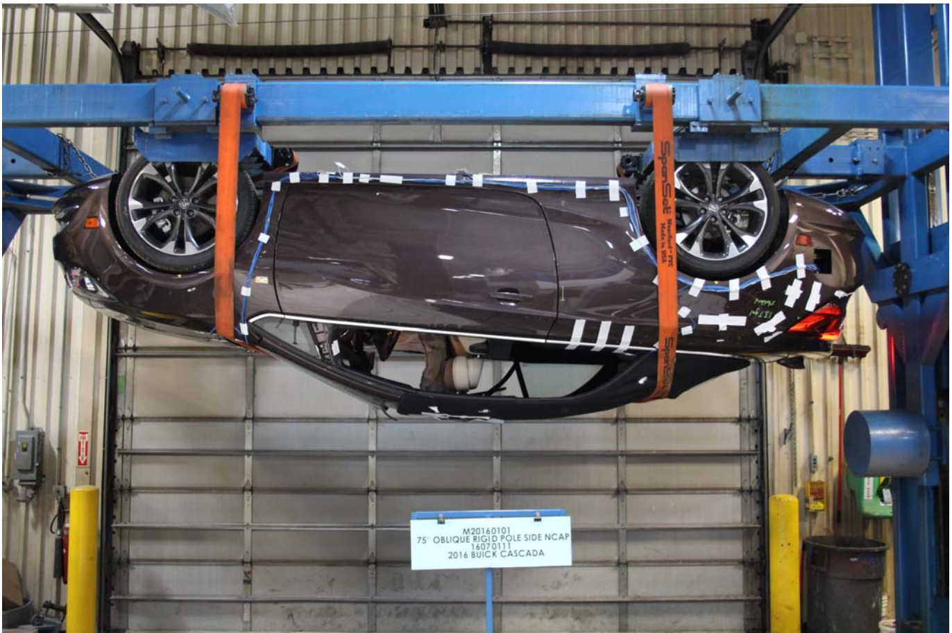
Photo No. 065 - FMVSS No. 301 Static Rollover 180 Degrees
