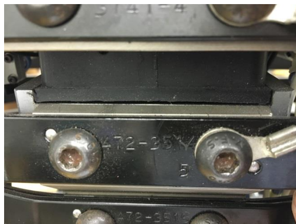
De-bonding of Thoracic Spine & Metal
