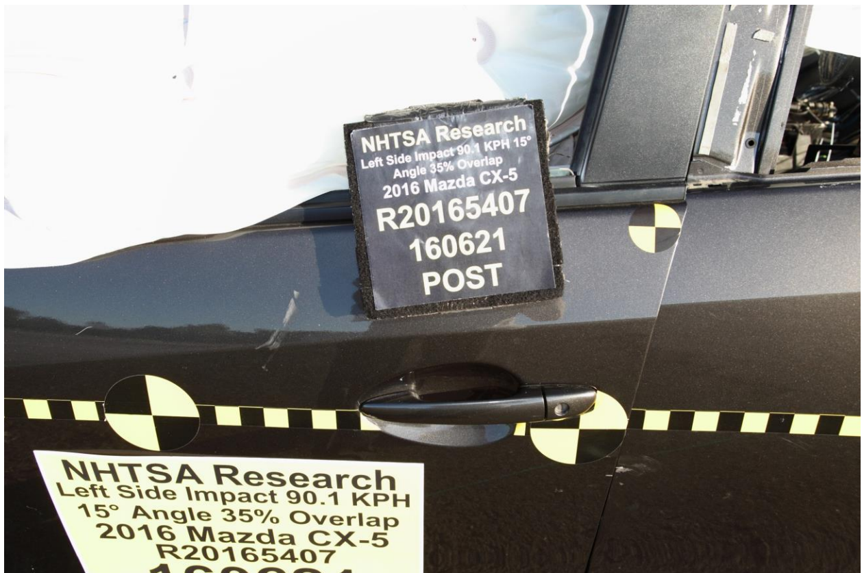
No. 55 Post-Test Close-Up View of Driver's Door Latch
