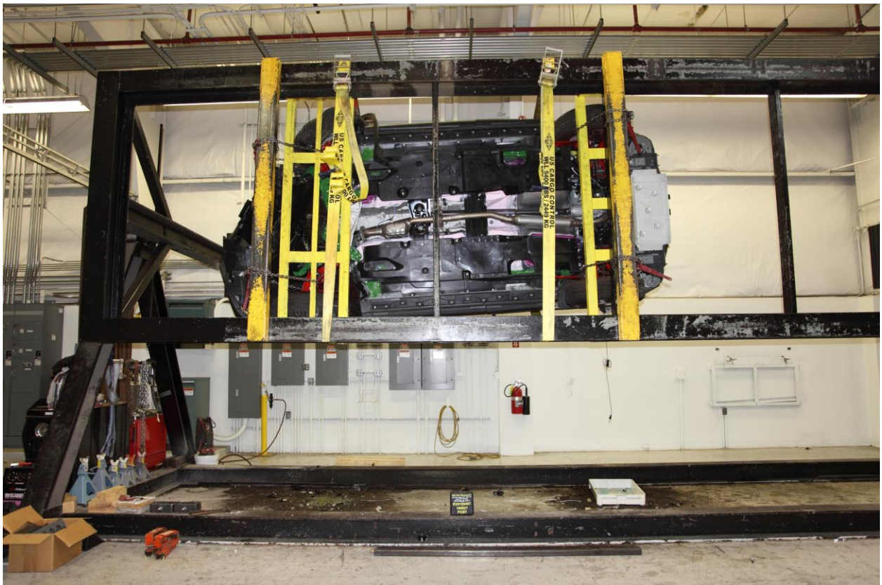
No. 211 Static Rollover 270 Degrees
