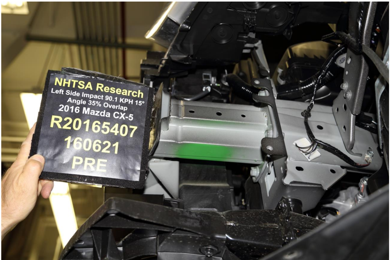
No. 168 Pre-Test Left Side Energy Absorber with Parts Removed
