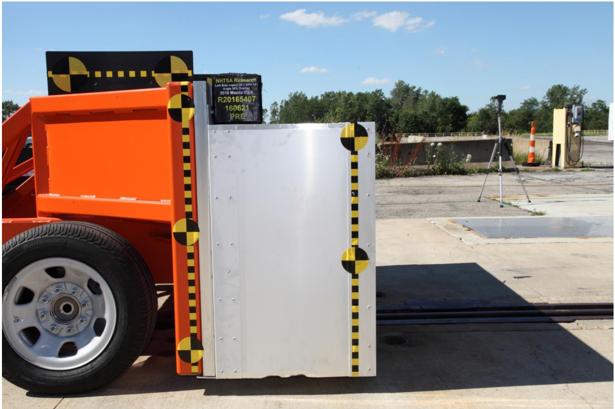
No. 204 Pre-Test Right Side Honeycomb
