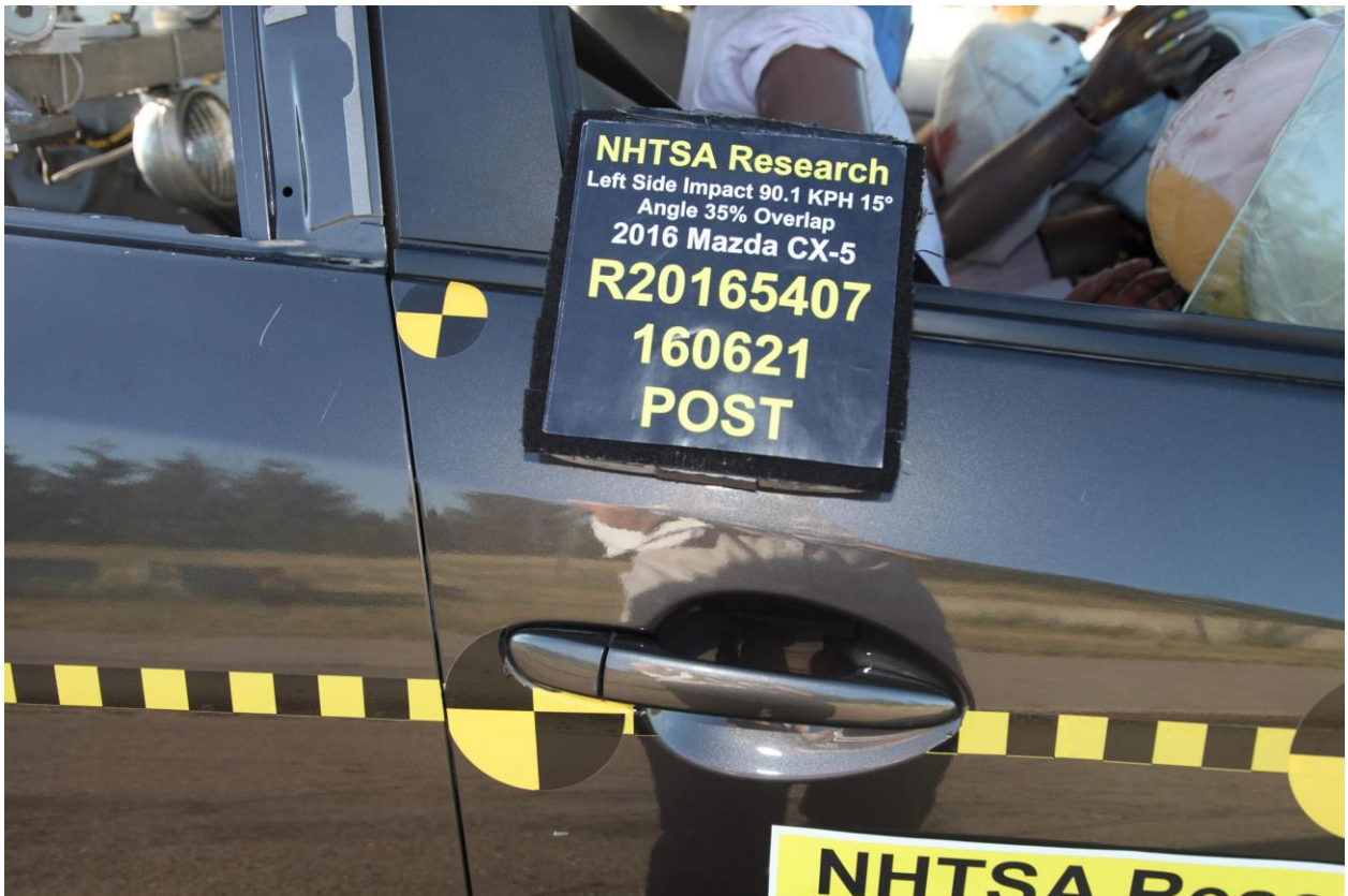
No. 109 Post-Test Close-Up View of Passenger's Door Latch
