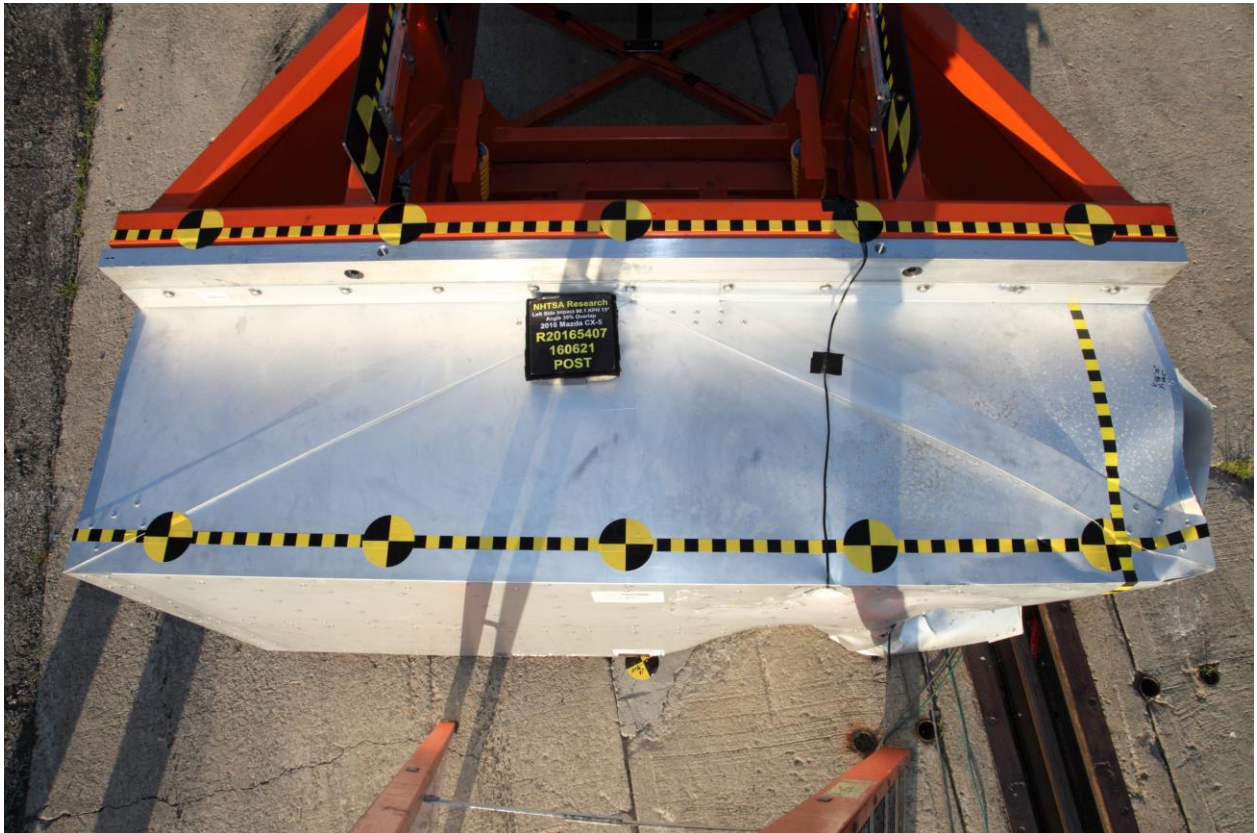
No. 207 Post-Test Overhead View of the Honeycomb
