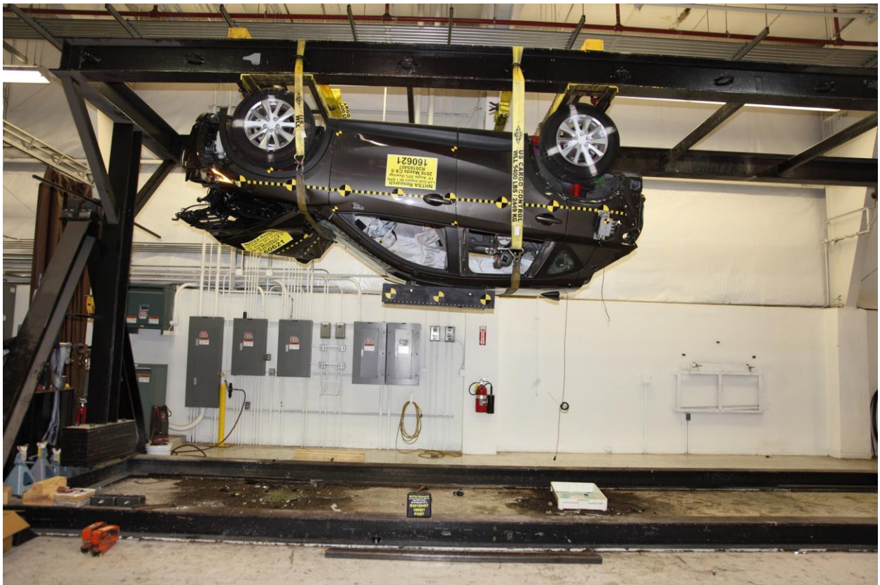
No. 210 Static Rollover 180 Degrees
