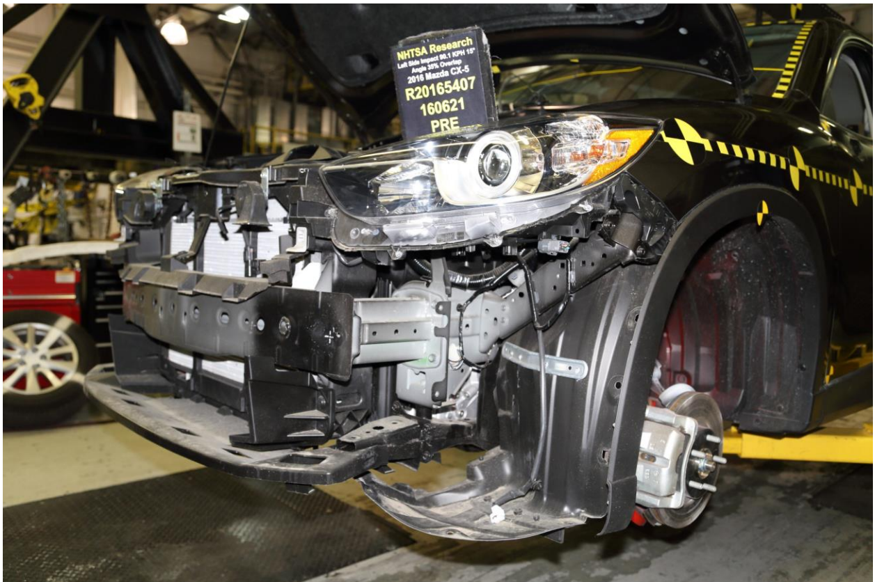
No. 172 Pre-Test Oblique View of Left Front of the Vehicle with Parts Removed
