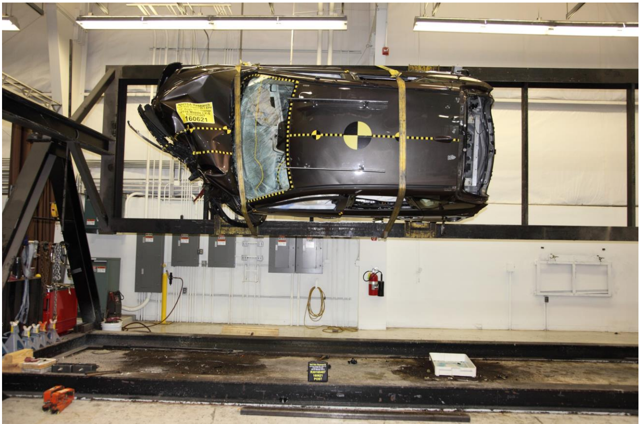
No. 209 Static Rollover 90 Degrees
