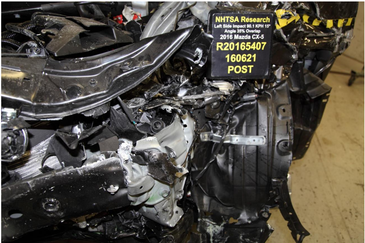
No. 182 Post-Test Left Shotgun View 1 with Parts Removed
