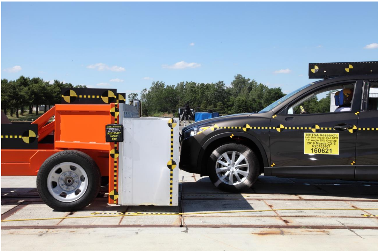
No. 29 Pre-test Right Side of O MDB against Target Vehicle at Ideal Impact Point
