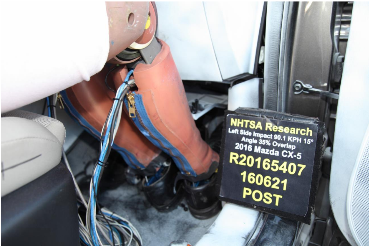
No. 143 Post-Test View of The Passenger's Feet
