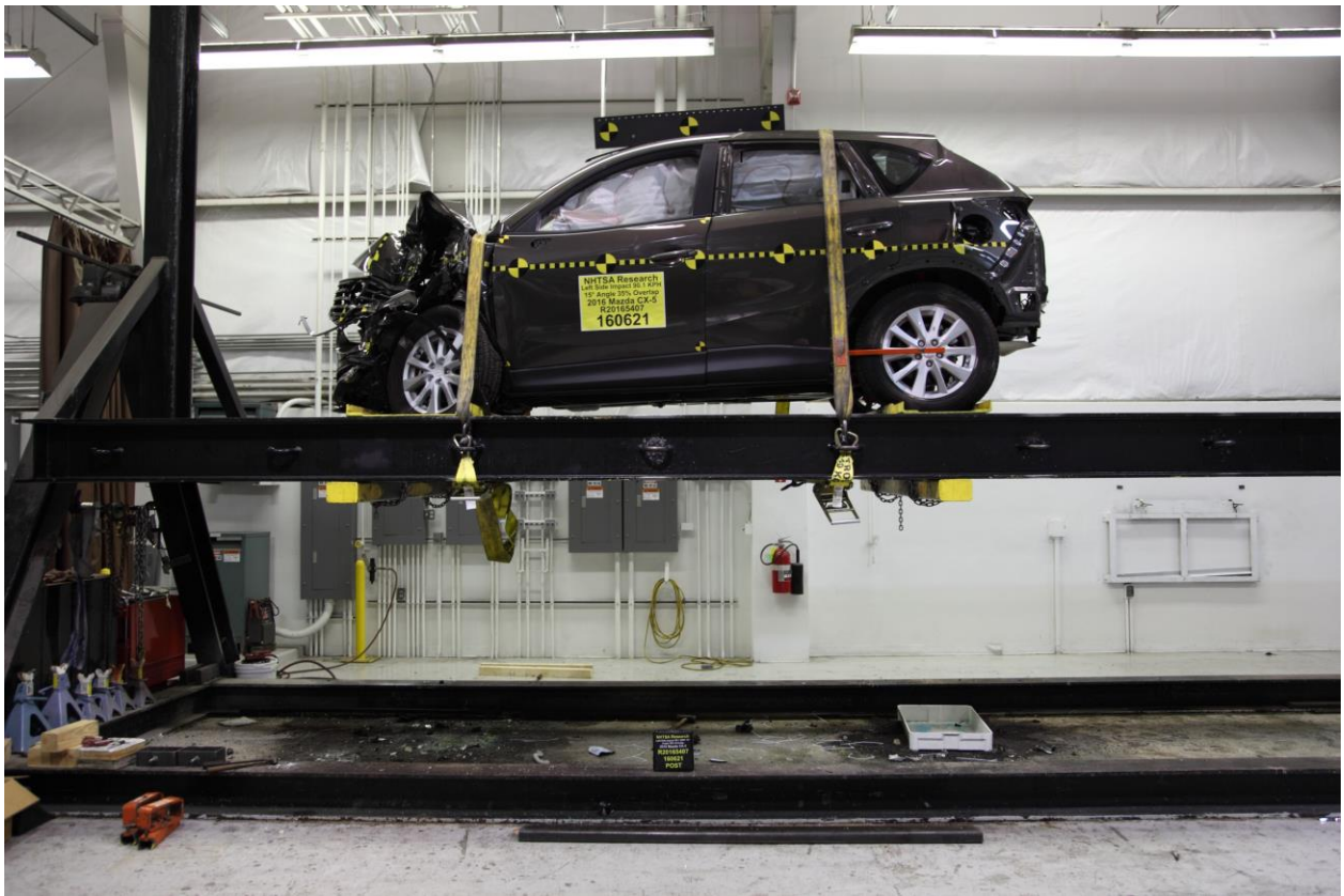
No. 212 Static Rollover 360 Degrees
