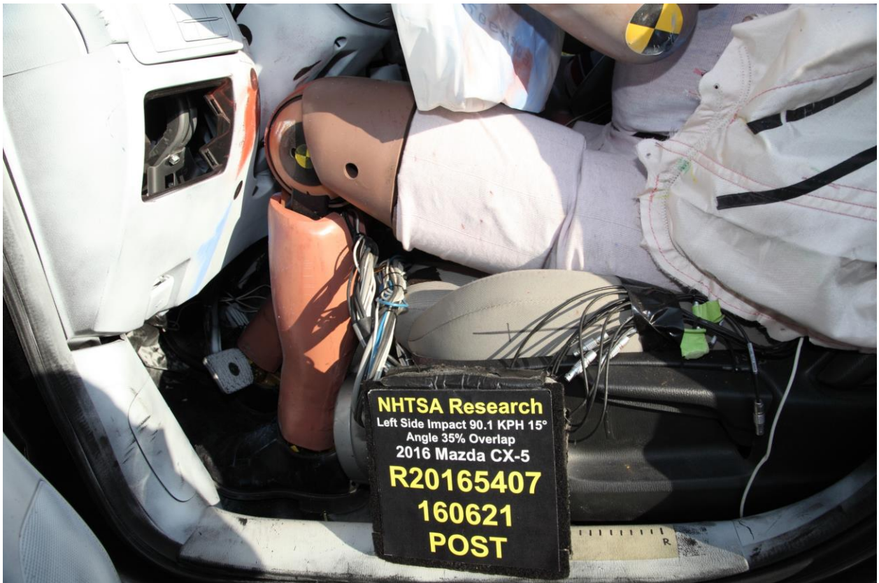
No. 91 Post-Test View of the Driver Left Leg
