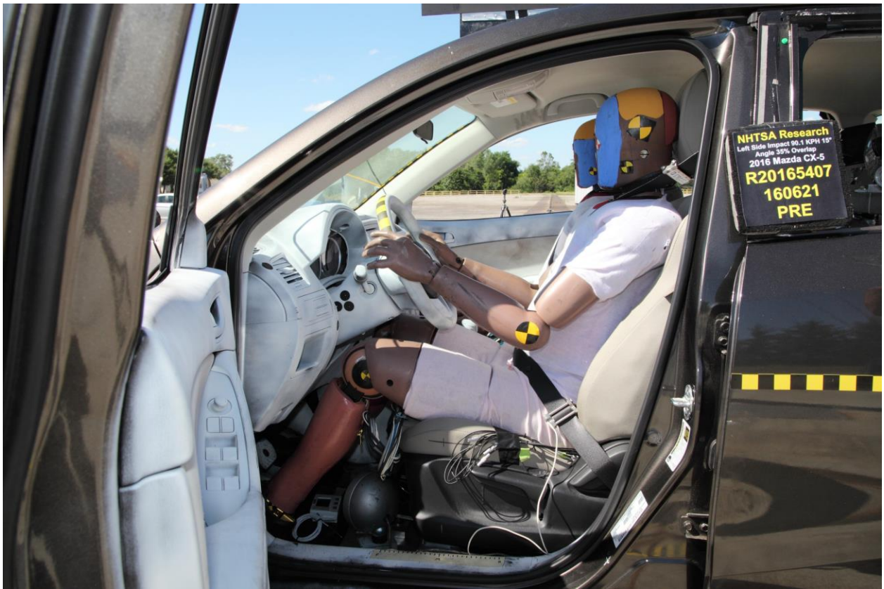
No. 64 Pre-Test Left Side View of Driver and Interior (Perpendicular View)
