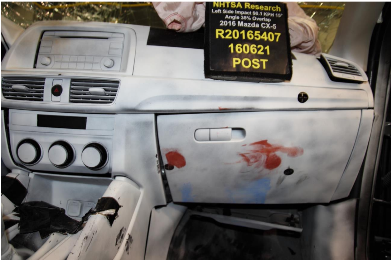
No. 127 Post-Test Overall View of Passenger Knee Bolsters
