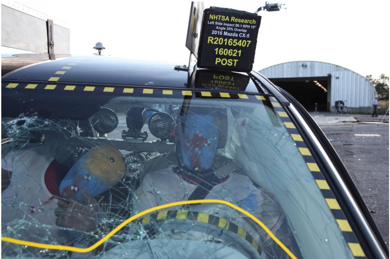
No. 49 Post-Test Driver Front Windshield View
