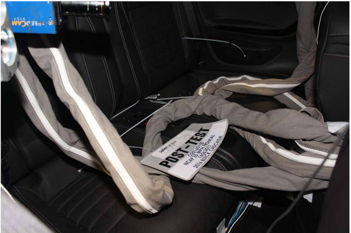
Photo No. 029 - Post-Test Dummy Cable Routing
