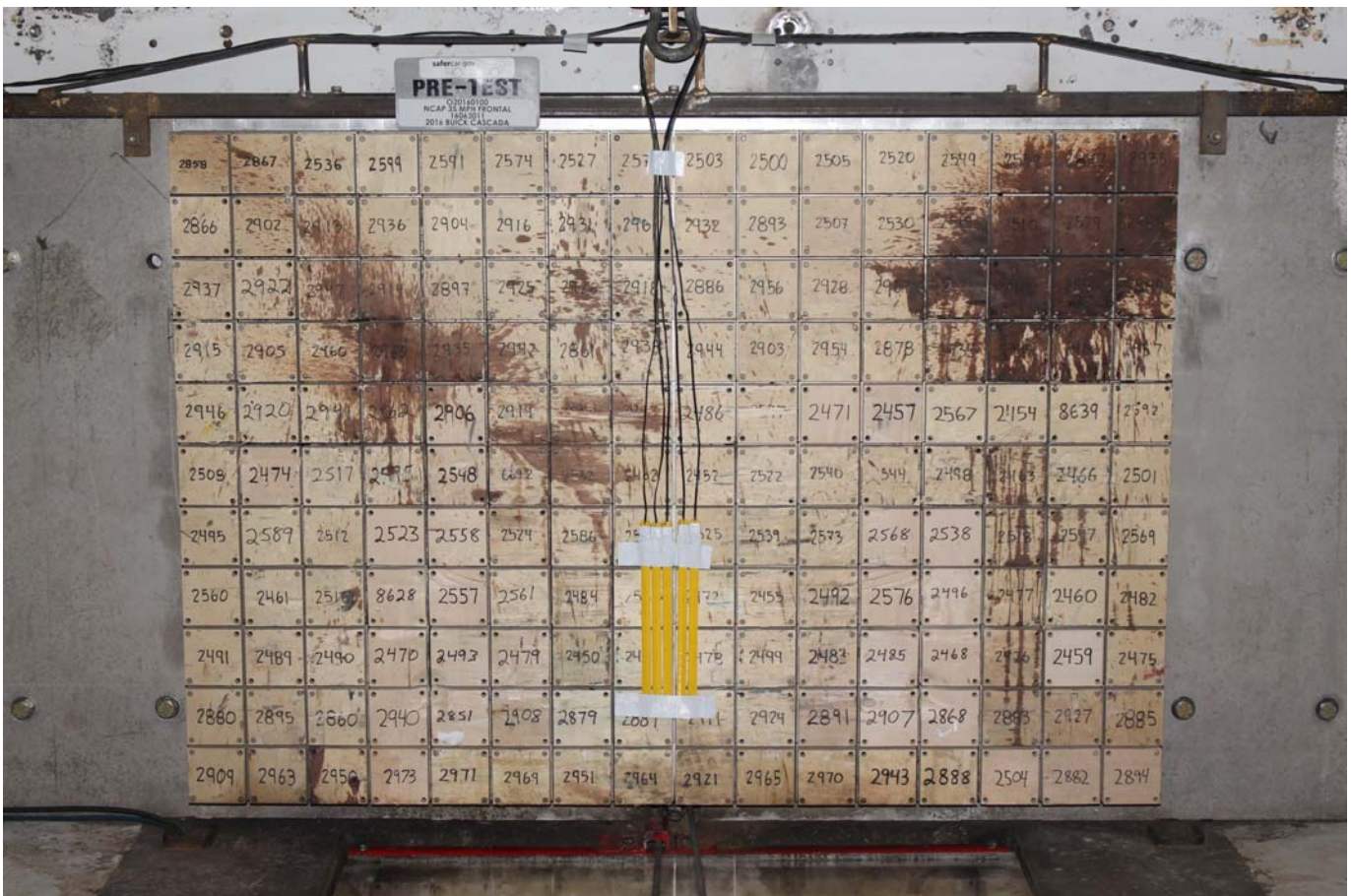
Photo No. 002 - Pre-Test Load Cell Wall
