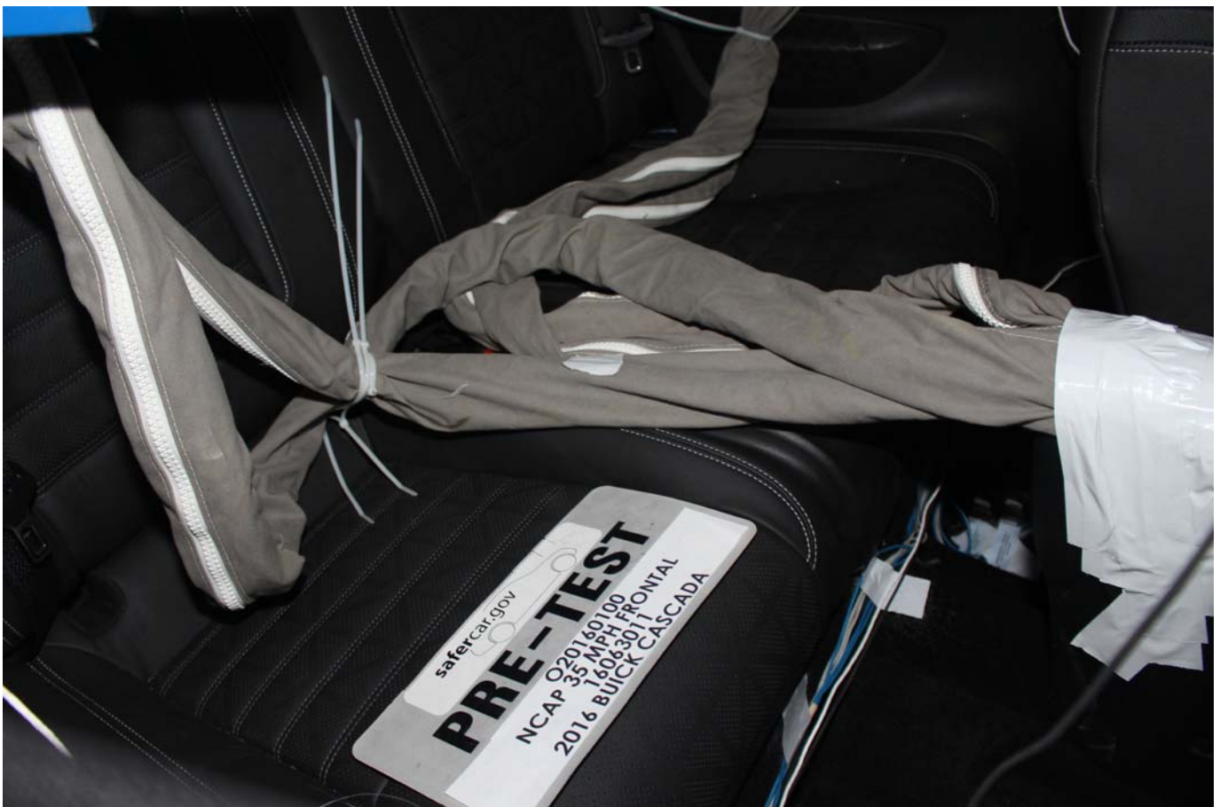
Photo No. 028 - Pre-Test Dummy Cable Routing
