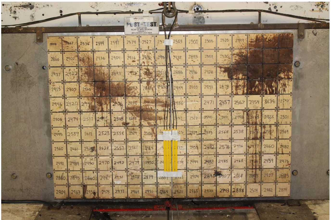
Photo No. 003 - Post-Test Load Cell Wall
