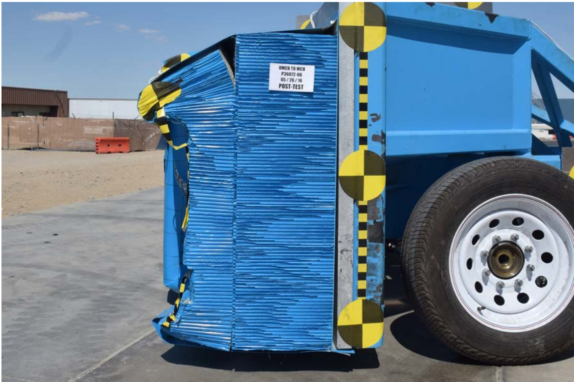
FIGURE 18. Post-Test Left View of OMDB Impactor Face
