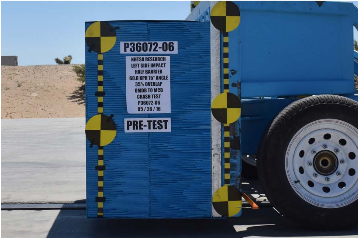
FIGURE 17. Pre-Test Left View of OMDB Impactor Face
