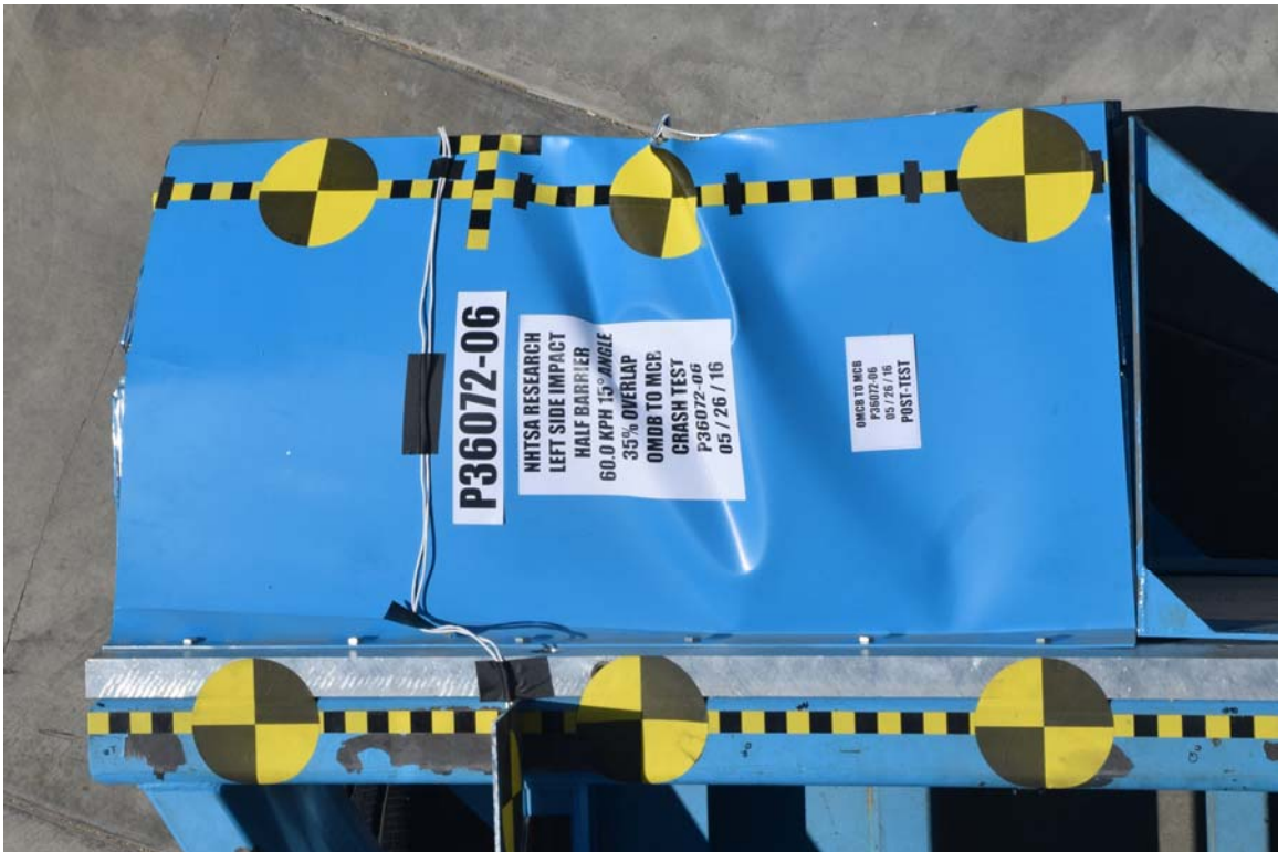
FIGURE 22. Post-Test Top View of OMDB Impactor Face
