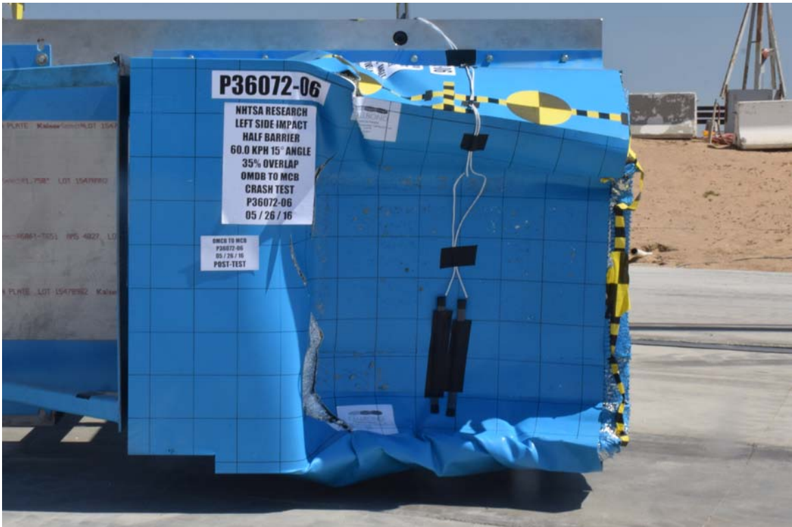
FIGURE 24. Post-Test Front View of OMDB Impactor Face
