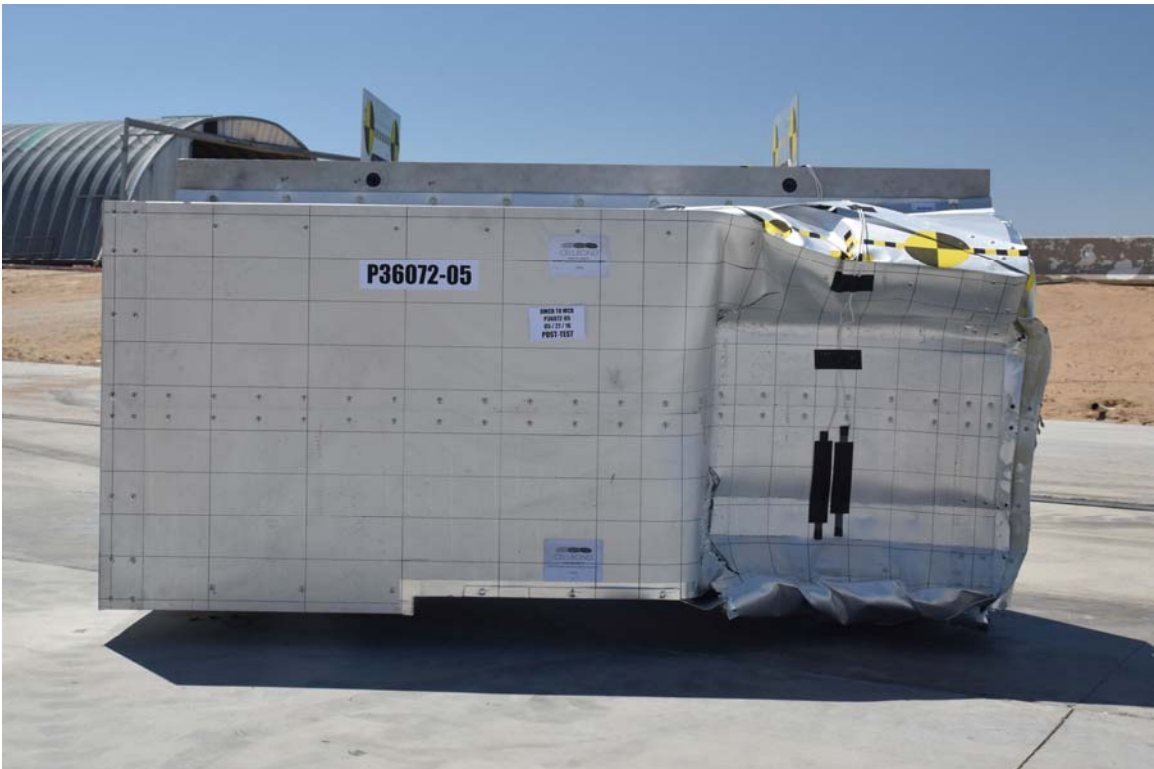
FIGURE 24. Post-Test Front View of OMDB Impactor Face
