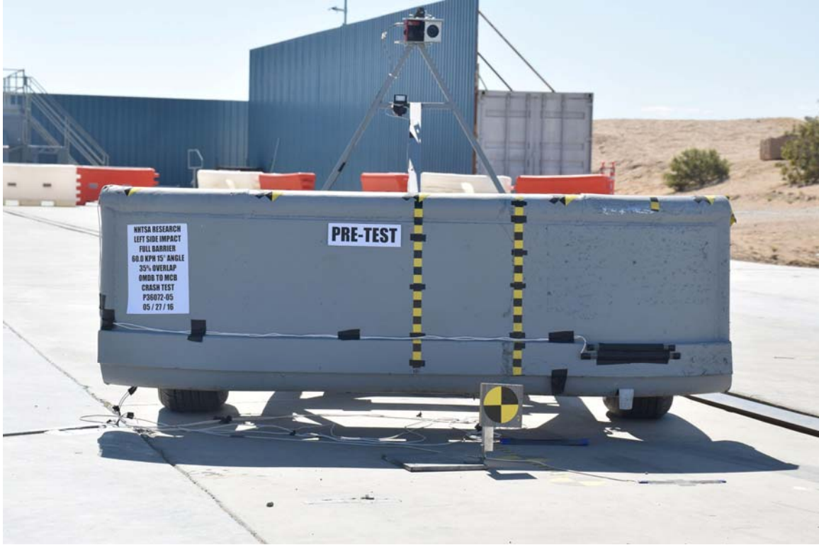
FIGURE 11. Pre-Test Front View of MCB
