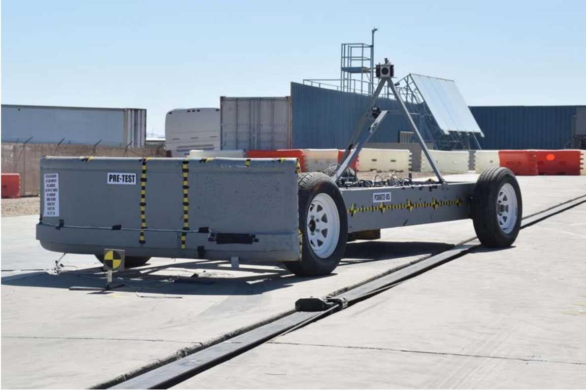
FIGURE 13. Pre-Test Left Front \frac{3}{4} View of MCB
