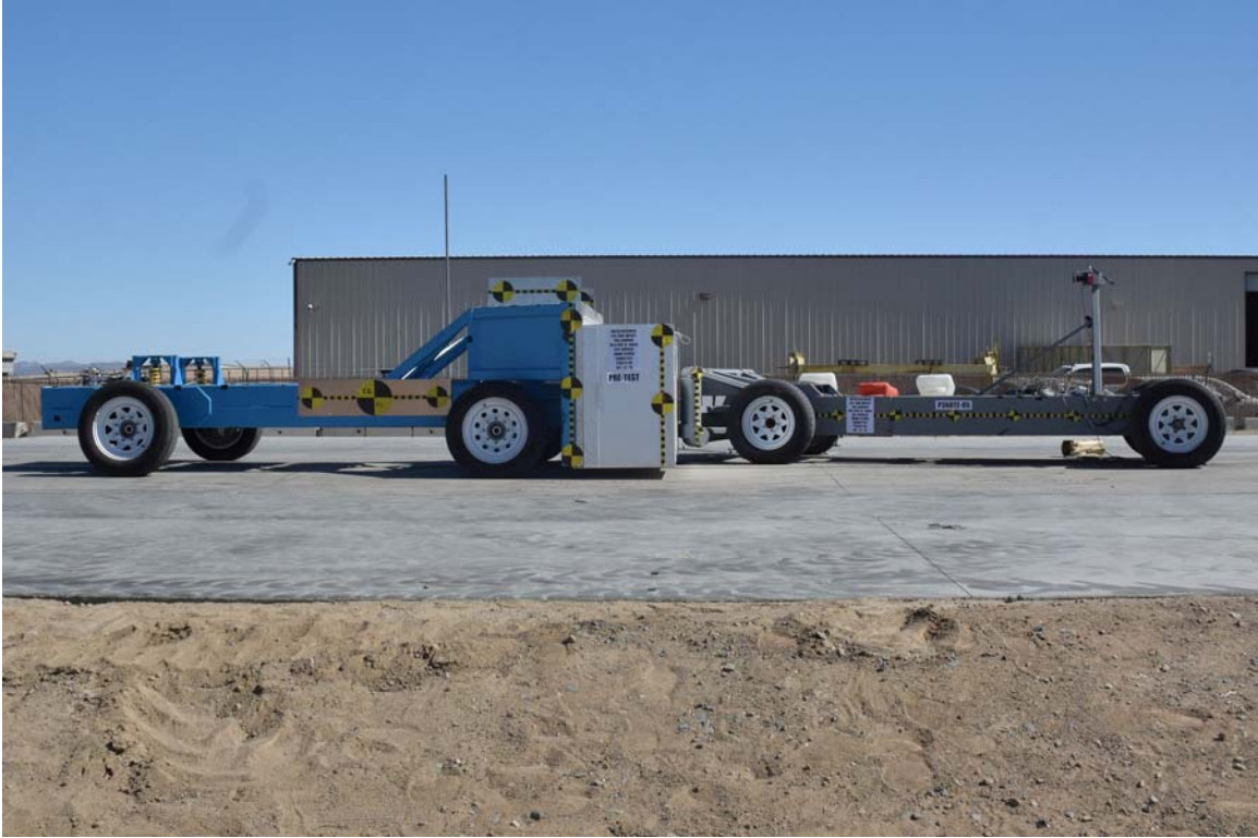
FIGURE 1. Pre-Test Right View of OMDB and MCB
