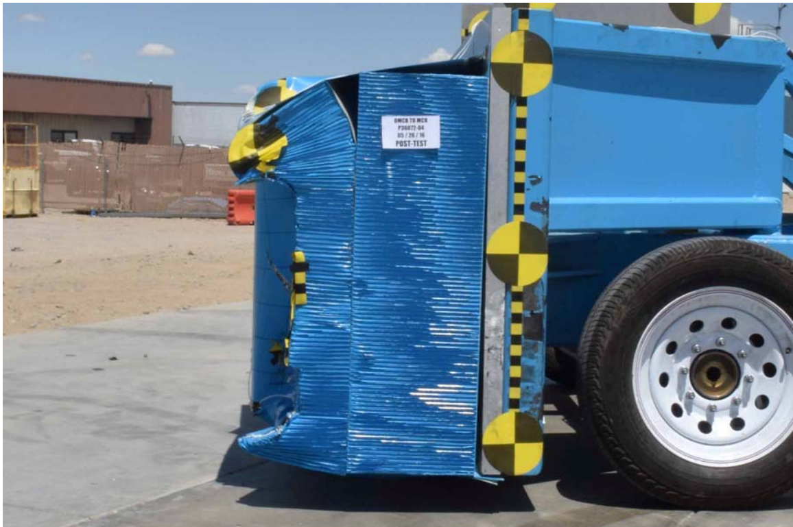
FIGURE 18. Post-Test Left View of OMDB Impactor Face
