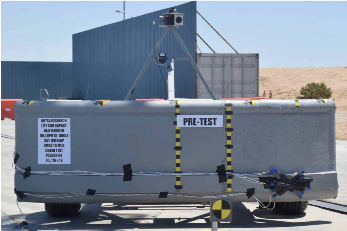
FIGURE 11. Pre-Test Front View of MCB
