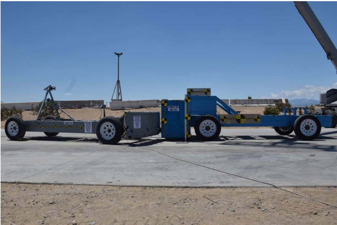
FIGURE 2. Pre-Test Left View of OMDB and MCB
