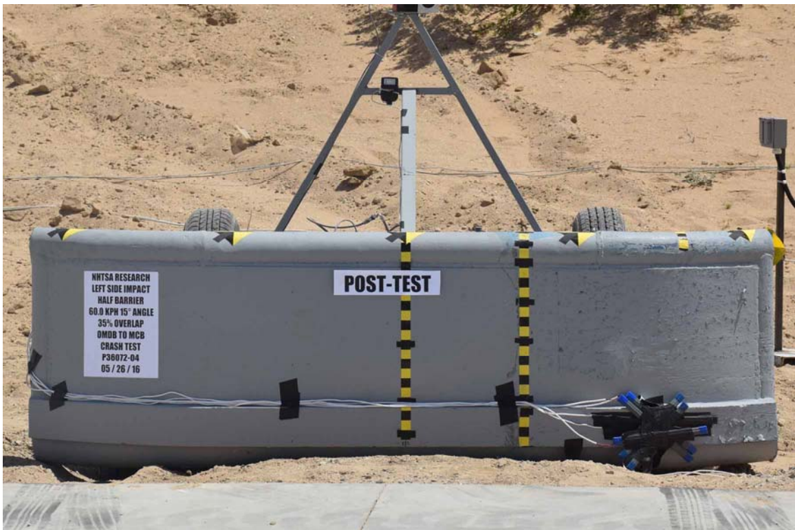
FIGURE 12. Post-Test Front View of MCB
