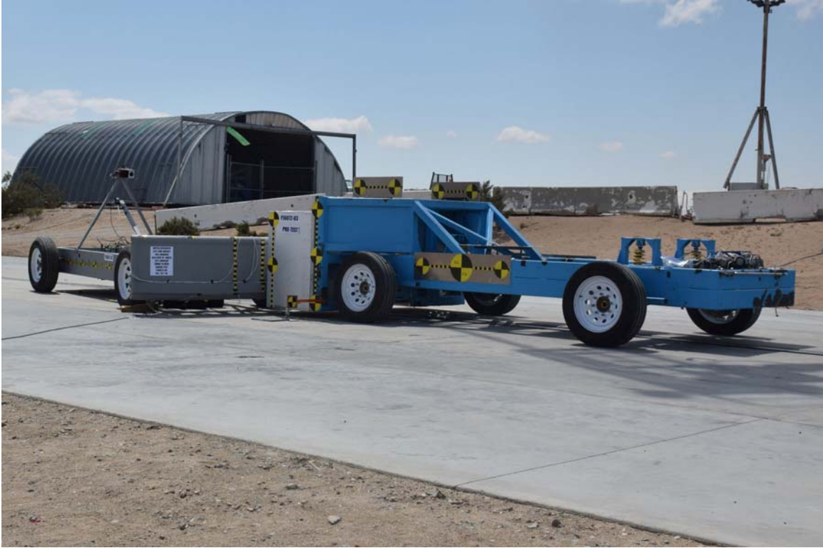
FIGURE 29. Pre-Test OMDB and MCB Alignment
