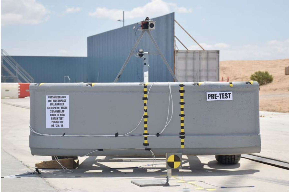
FIGURE 11. Pre-Test Front View of MCB
