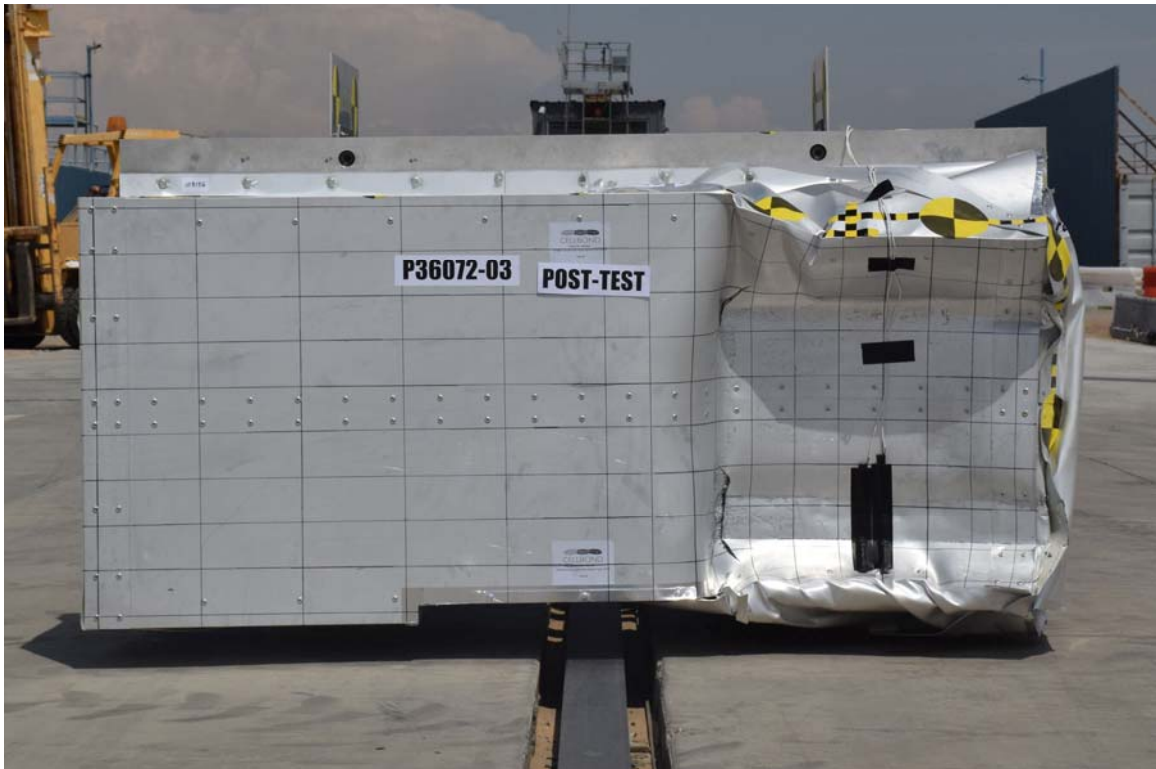
FIGURE 24. Post-Test Front View of OMDB Impactor Face
