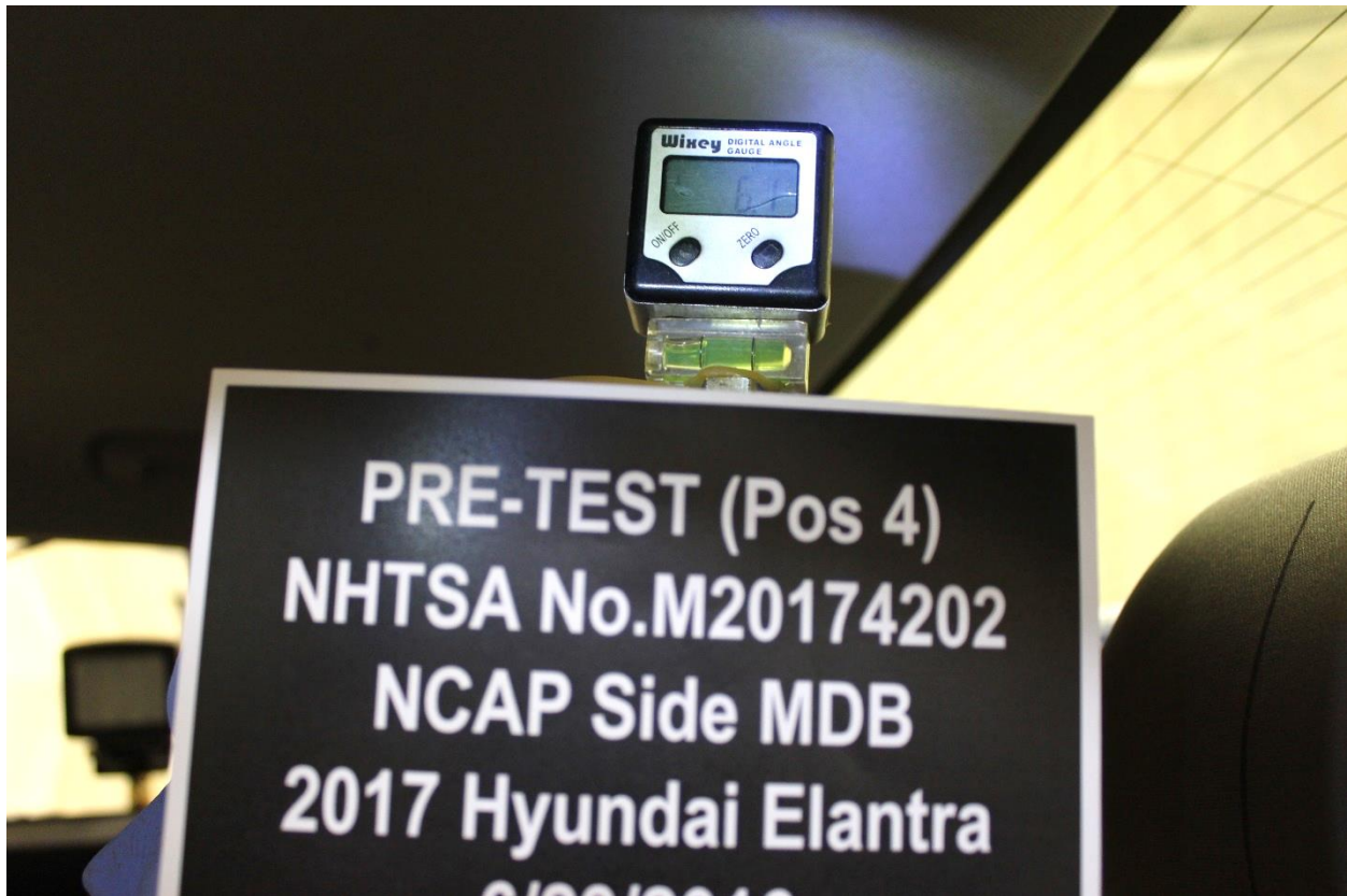
Figure A-63: Pre-Test View of Rear Passenger Dummy's Head Showing Dummy's Head is Level
