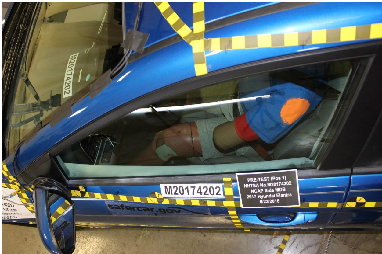
Figure A-42: Pre-Test Driver Dummy and Door Clearance View
