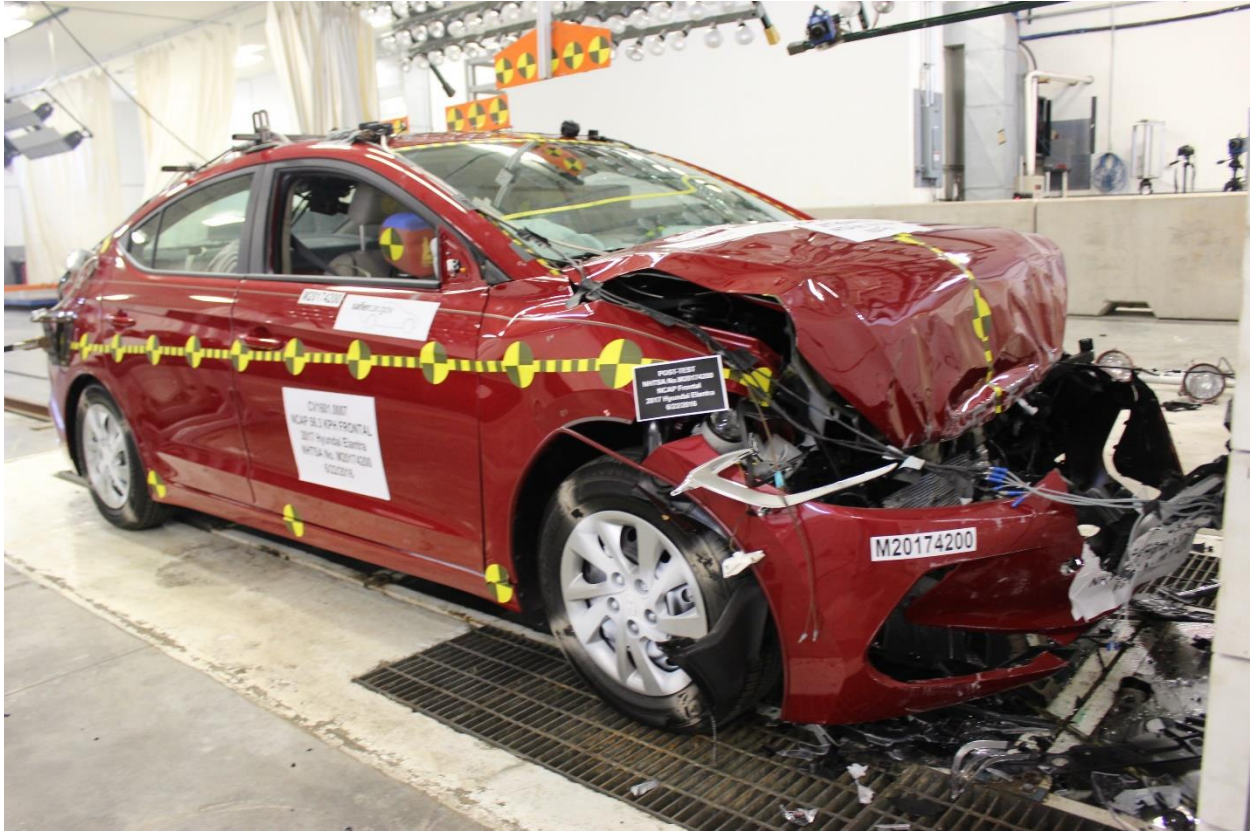
Figure A-15: Post-Test Right Front 3-4 View
