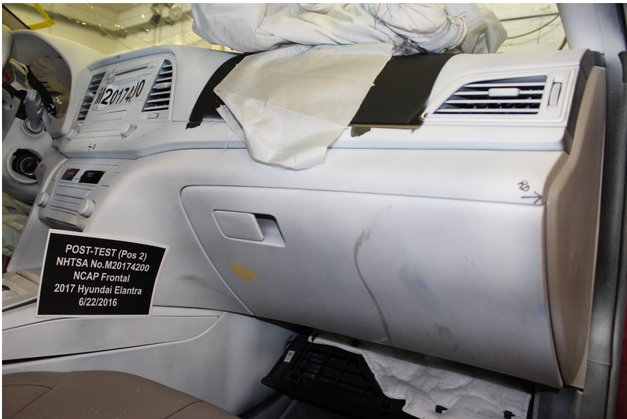
Figure A-64: Post-Test Passenger's Side Knee Bolster
