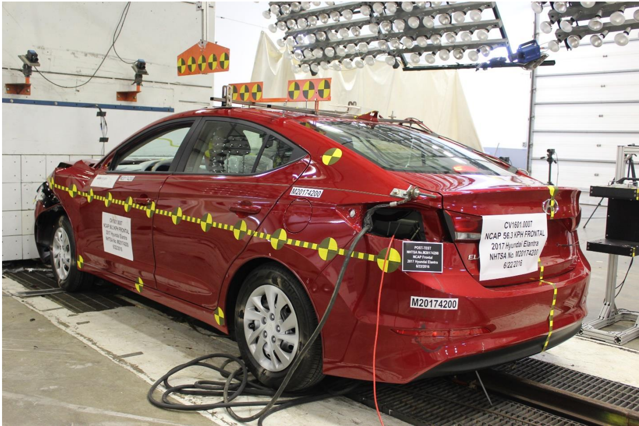
Figure A-17: Post-Test Left Rear 3-4 View
