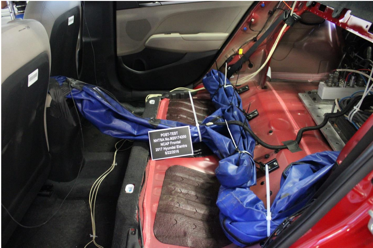
Figure A-29: Post-Test Dummy Cable Routing
