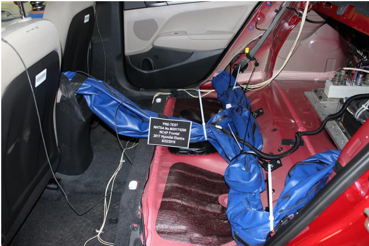
Figure A-28: Pre-Test Dummy Cable Routing
