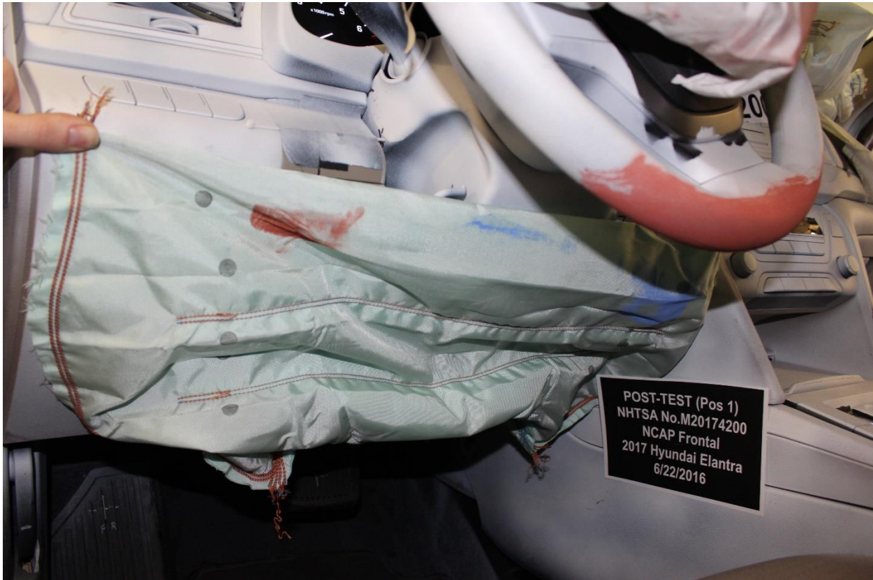
Figure A-43: Post-Test Driver's Side Knee Bolster
