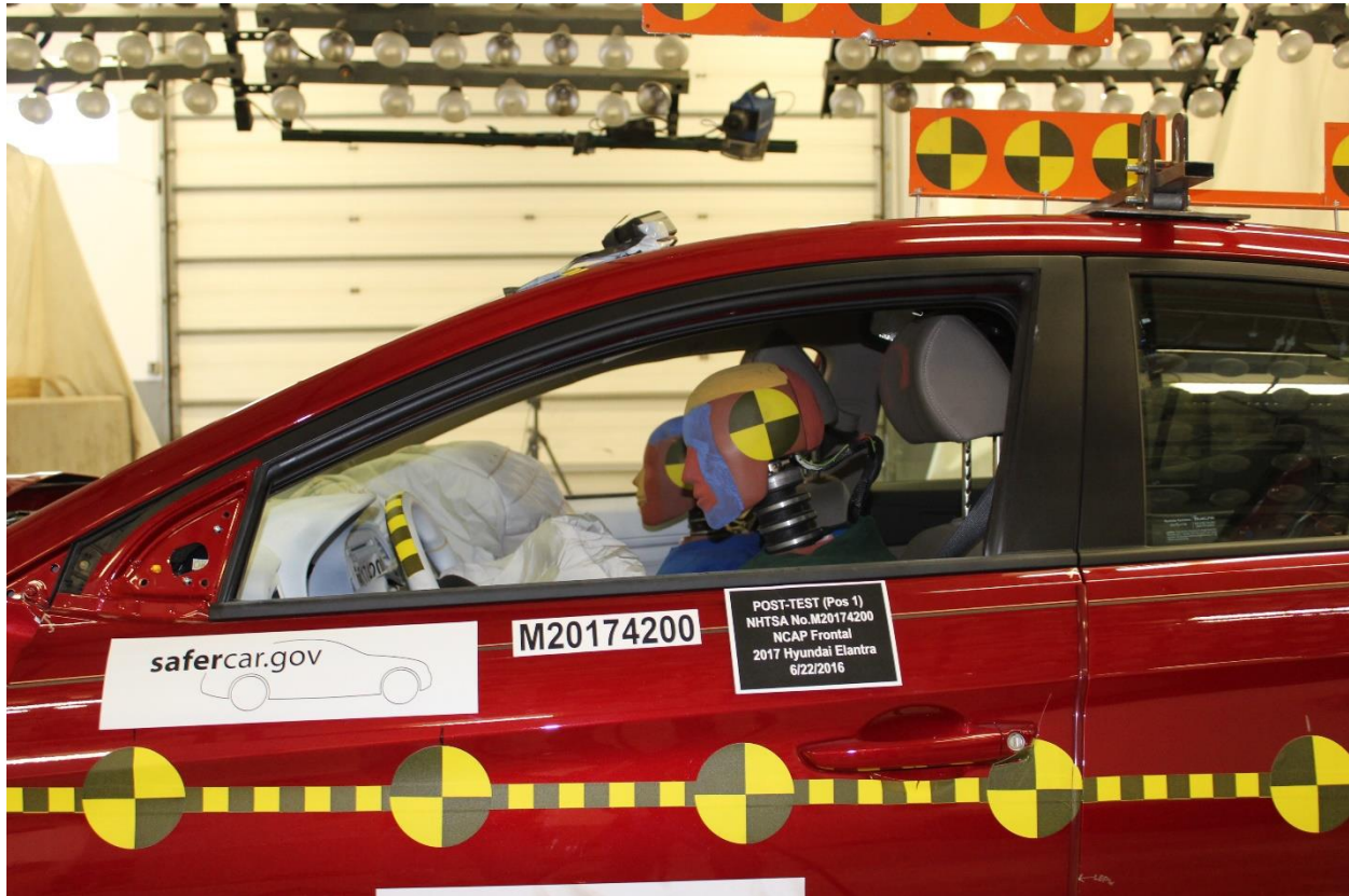
Figure A-33: Post-Test Driver Dummy Window View
