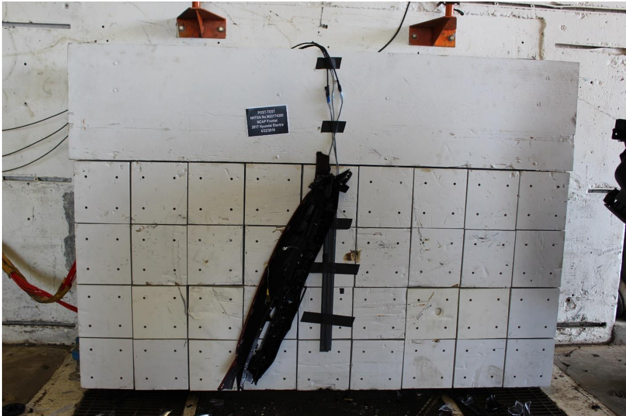
Figure A-3: Post-Test Load Cell Wall
