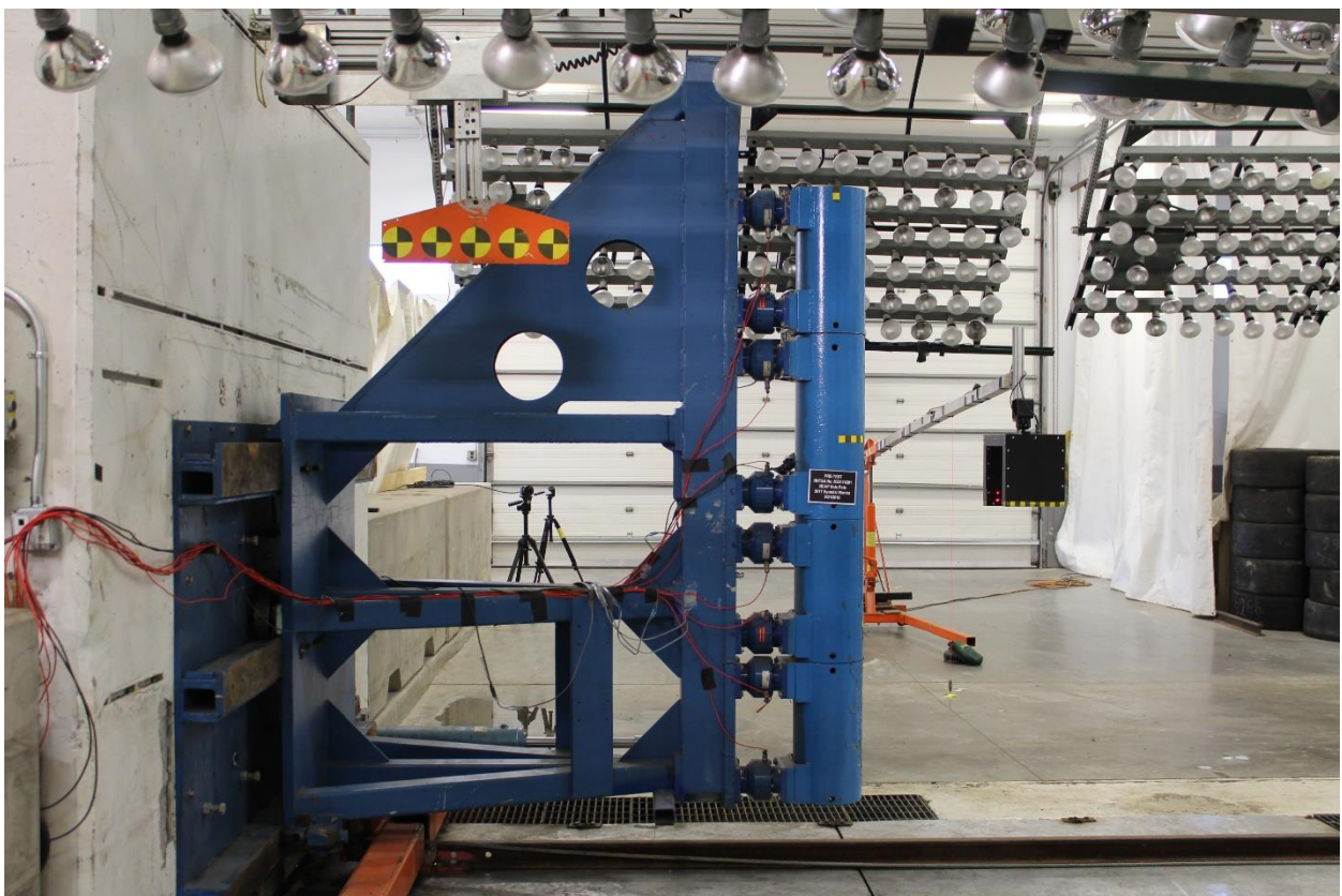
Figure A-59: Pre-Test Pole Barrier Side View
