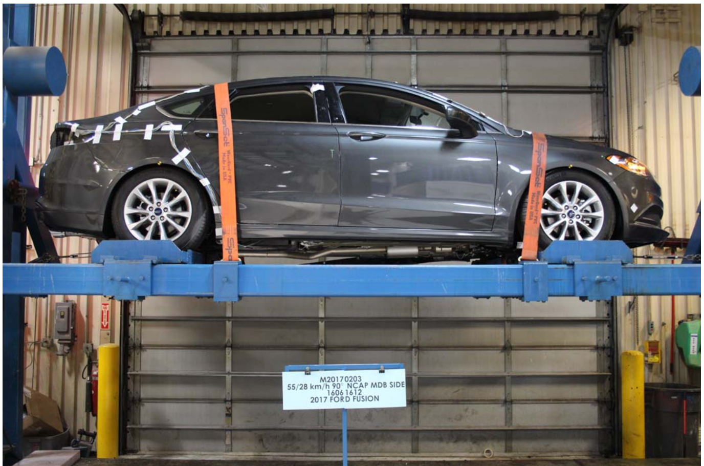
Photo No. 096 - FMVSS No. 301 Static Rollover 0 Degrees
