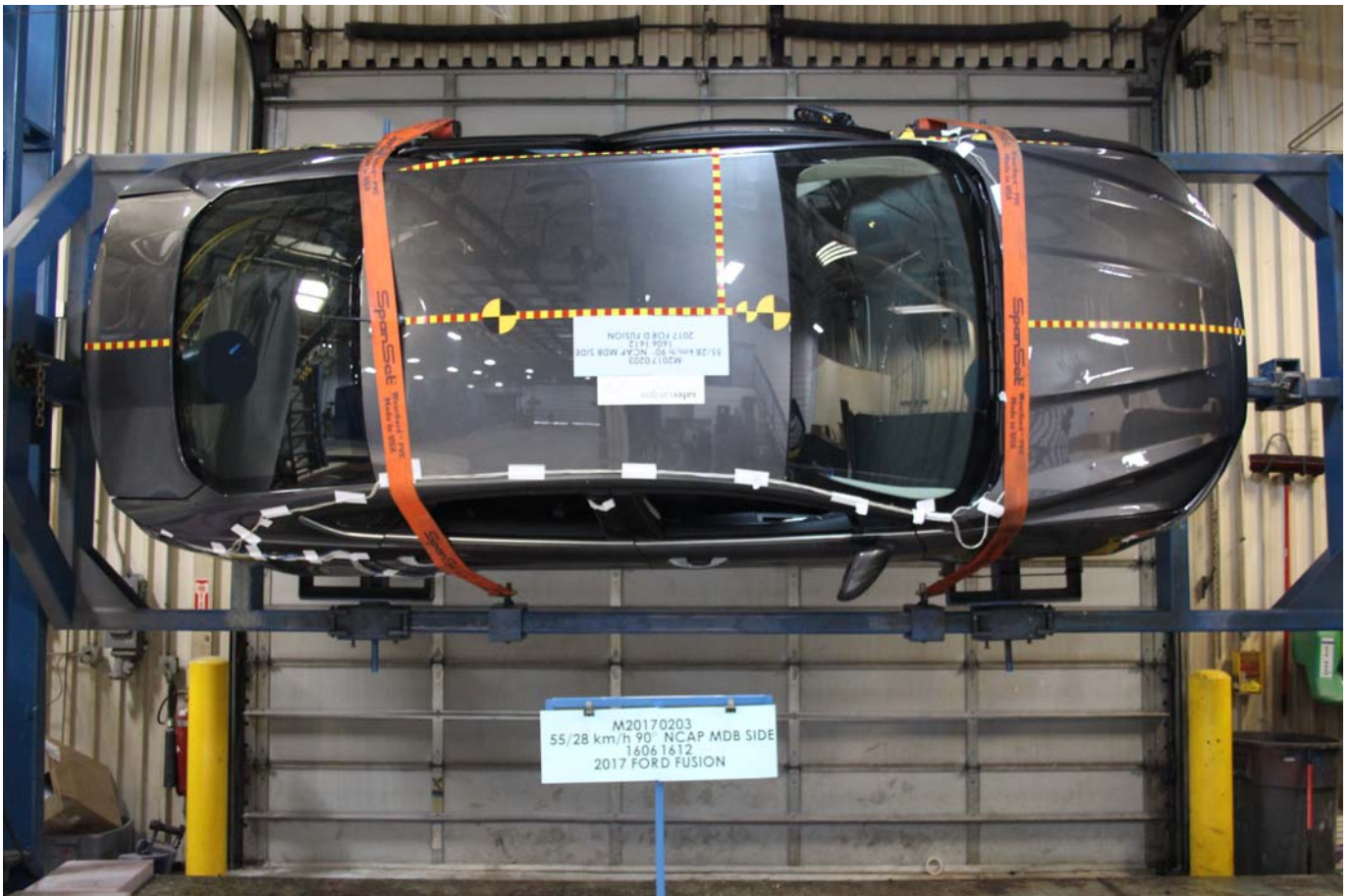
Photo No. 099 - FMVSS No. 301 Static Rollover 270 Degrees
