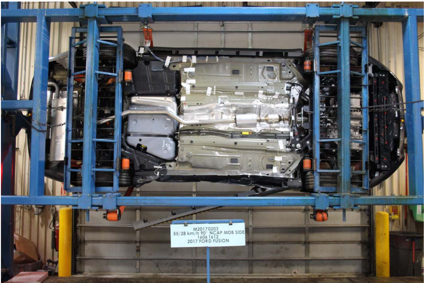
Photo No. 097 - FMVSS No. 301 Static Rollover 90 Degrees
