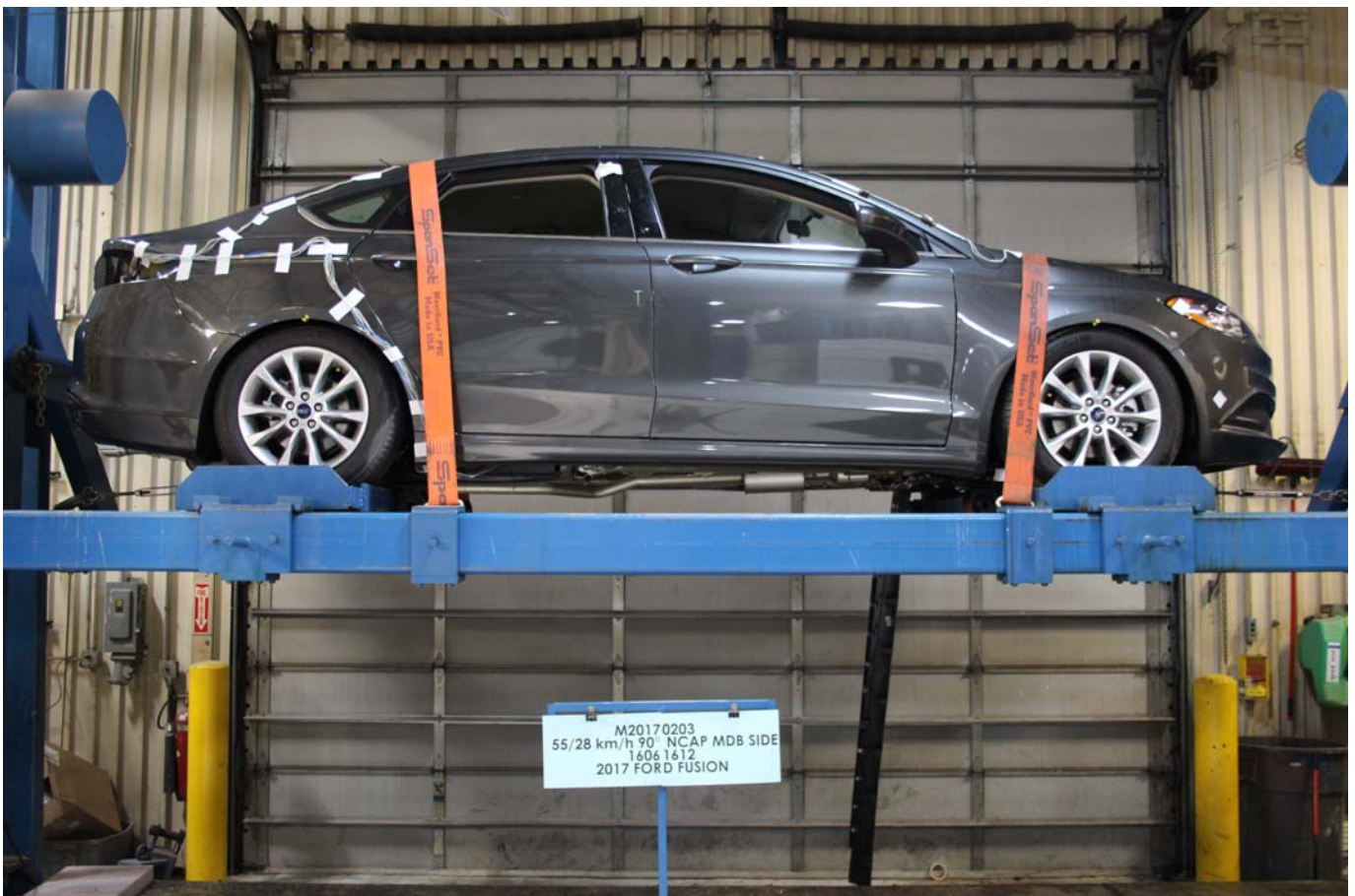
Photo No. 100 - FMVSS No. 301 Static Rollover 360 Degrees
