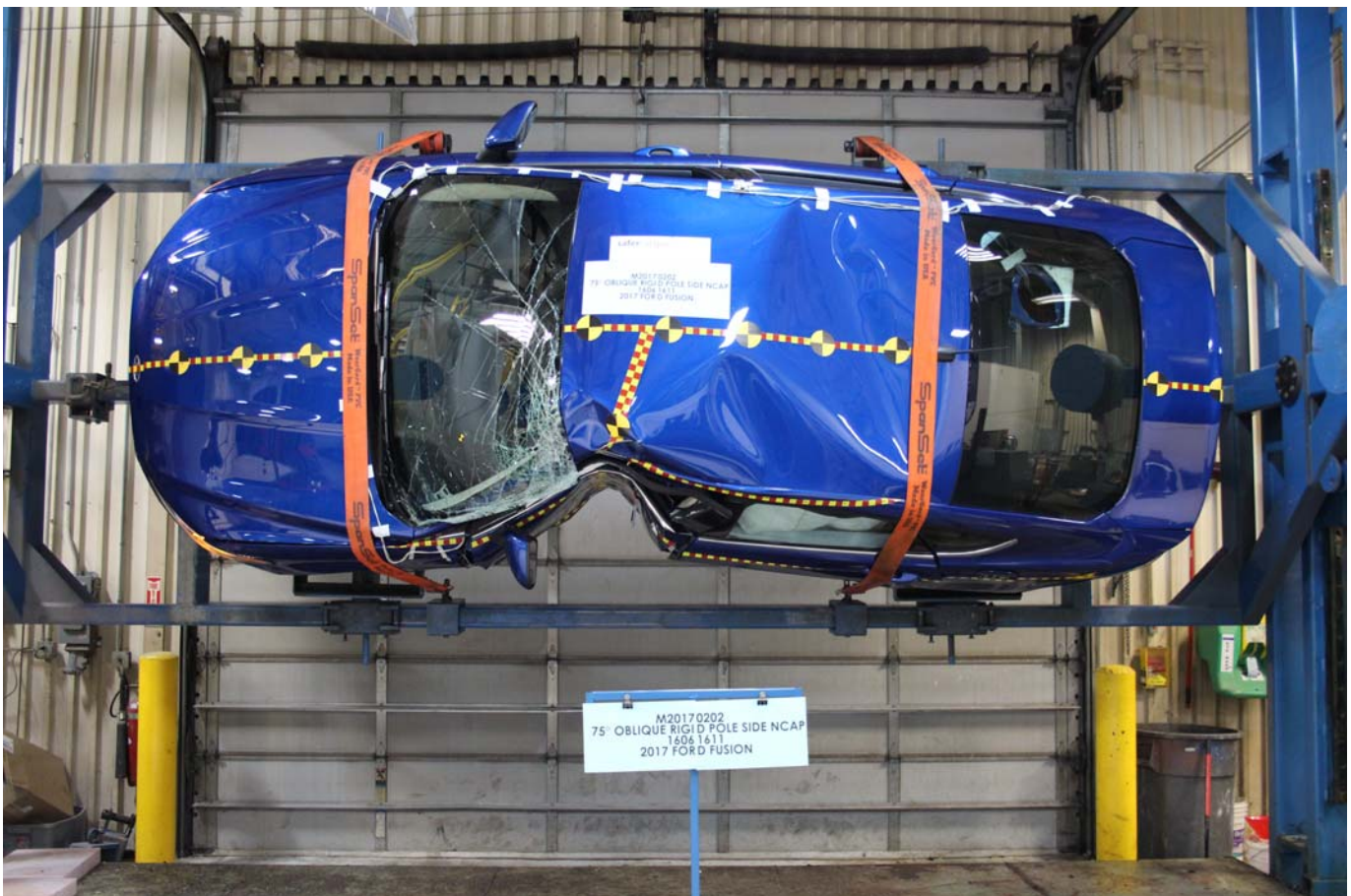
Photo No. 064 - FMVSS No. 301 Static Rollover 90 Degrees
