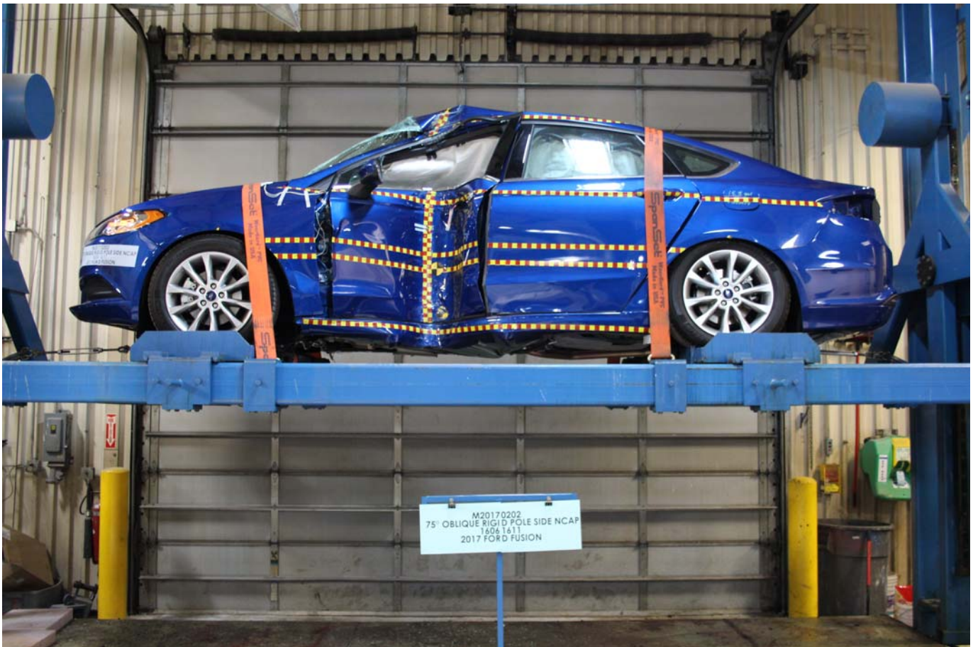
Photo No. 067 - FMVSS No. 301 Static Rollover 360 Degrees
