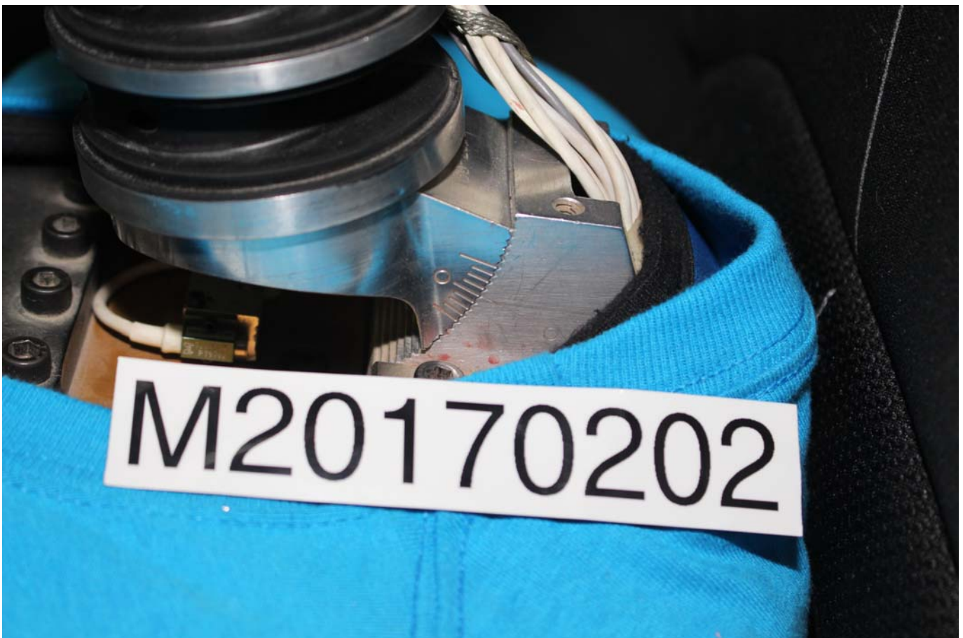
Photo No. 030 - Pre-Test Left Side View of Dummy's Neck Showing Position of Adjustable Neck Bracket
