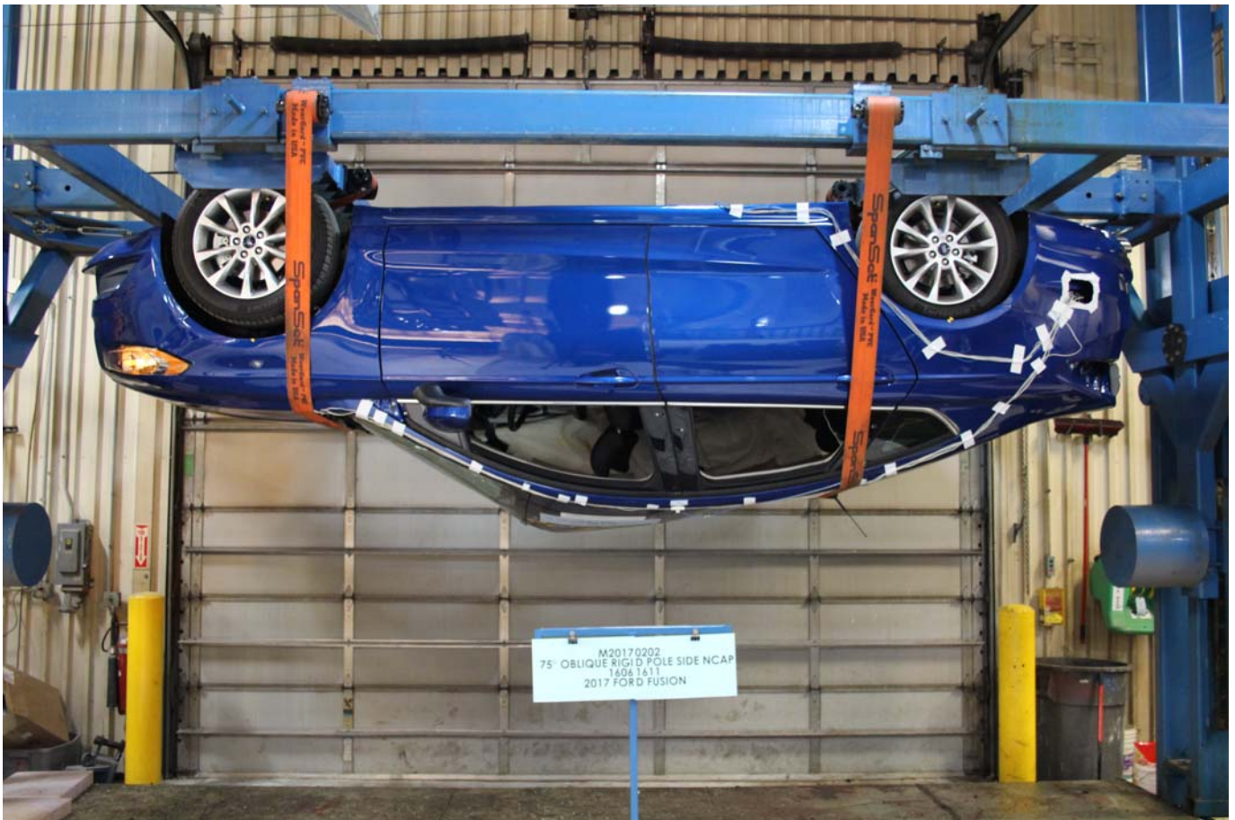
Photo No. 065 - FMVSS No. 301 Static Rollover 180 Degrees
