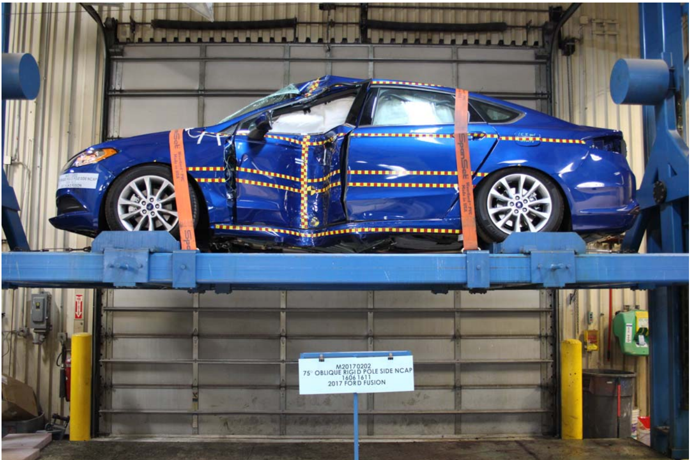
Photo No. 063 - FMVSS No. 301 Static Rollover 0 Degrees
