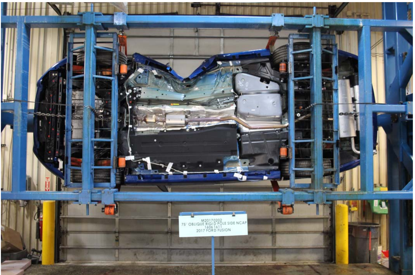
Photo No. 066 - FMVSS No. 301 Static Rollover 270 Degrees
