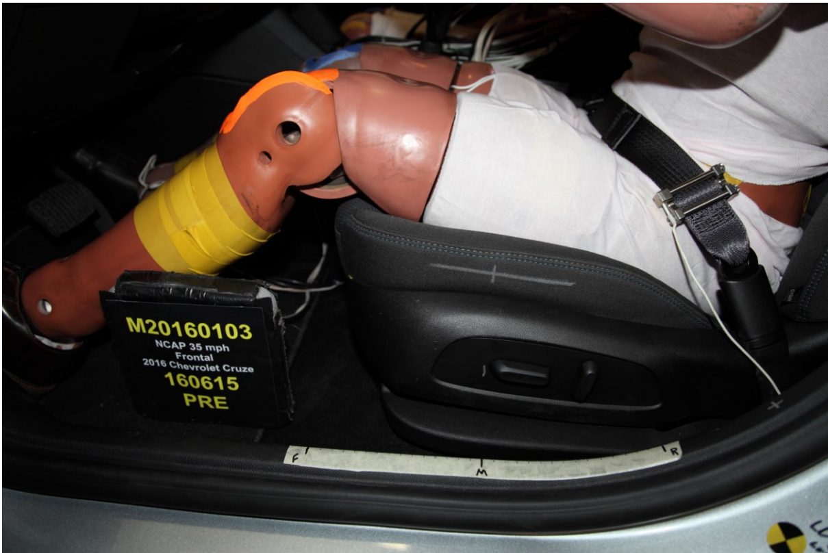
036 Pre-Test Driver's Seat Fore-Aft Markings
