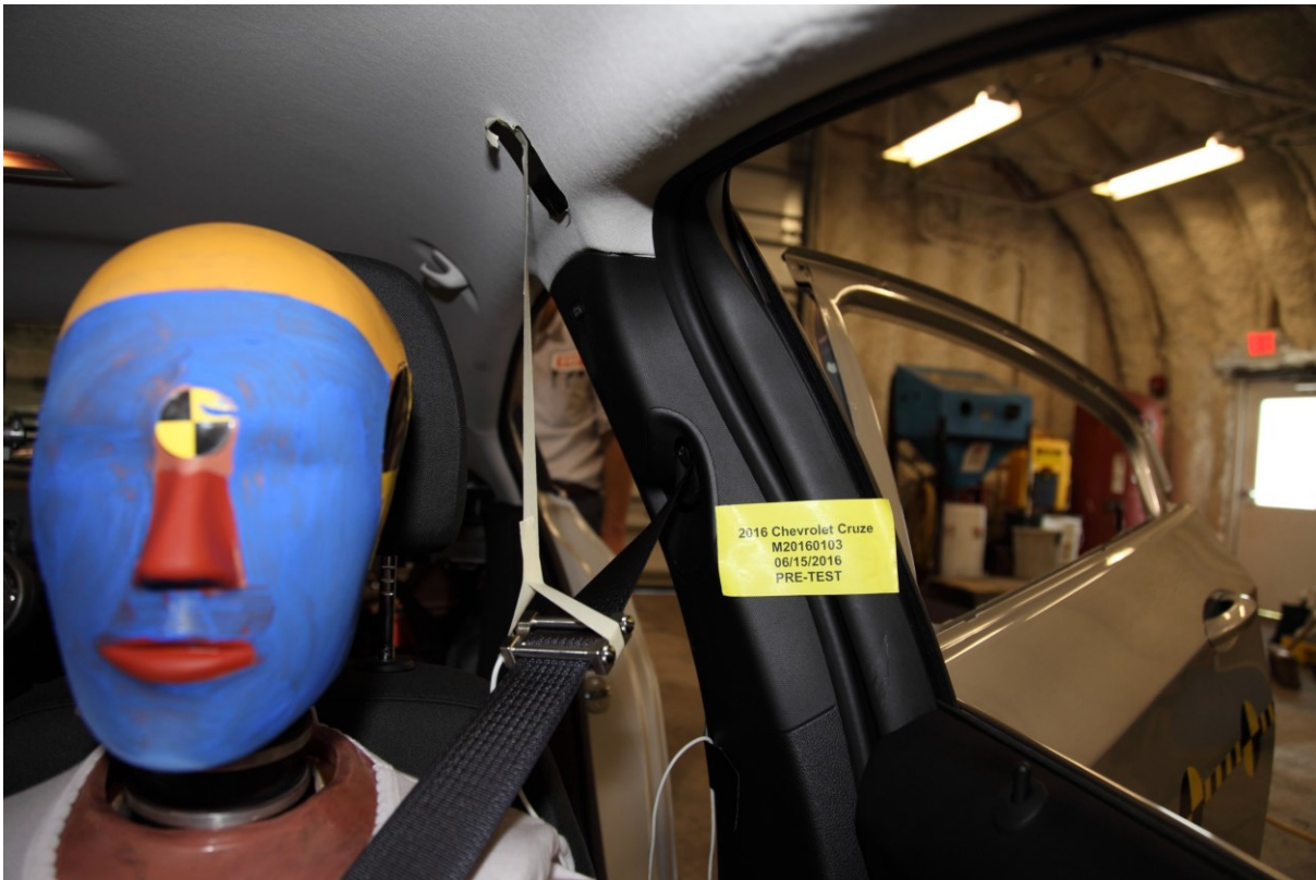
038 Pre-Test View of Belt Anchorage for Driver Dummy
