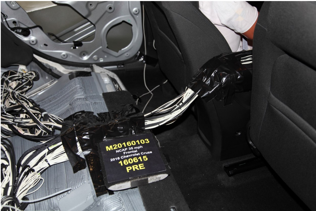
028 Pre-Test Dummy Cable Routing
