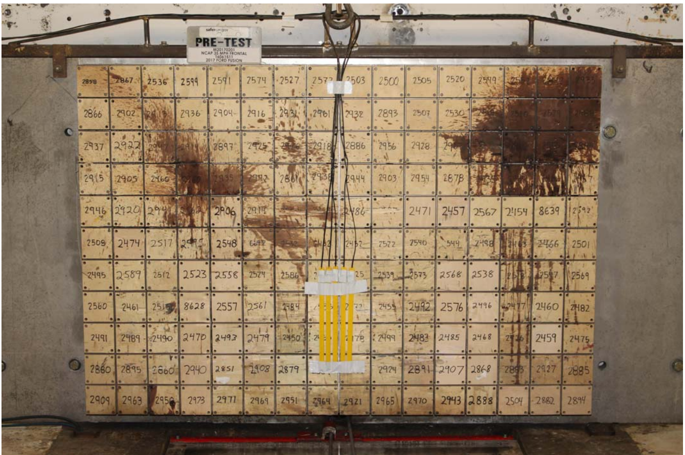
Photo No. 002 - Pre-Test Load Cell Wall
