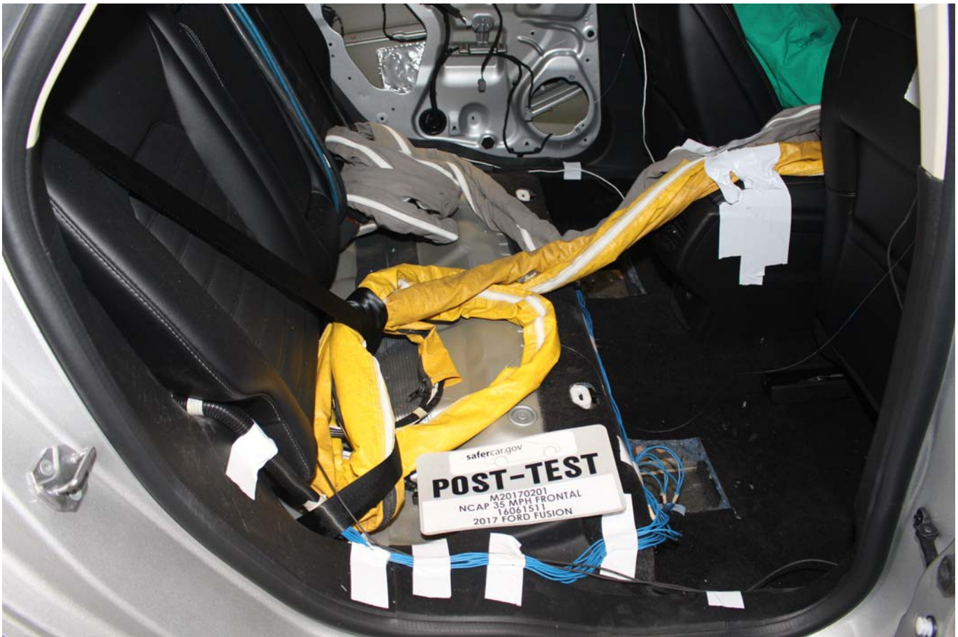
Photo No. 029 - Post-Test Dummy Cable Routing
