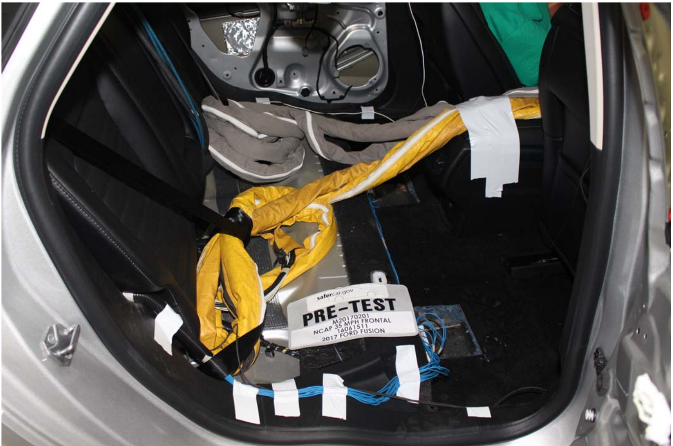
Photo No. 028 - Pre-Test Dummy Cable Routing
