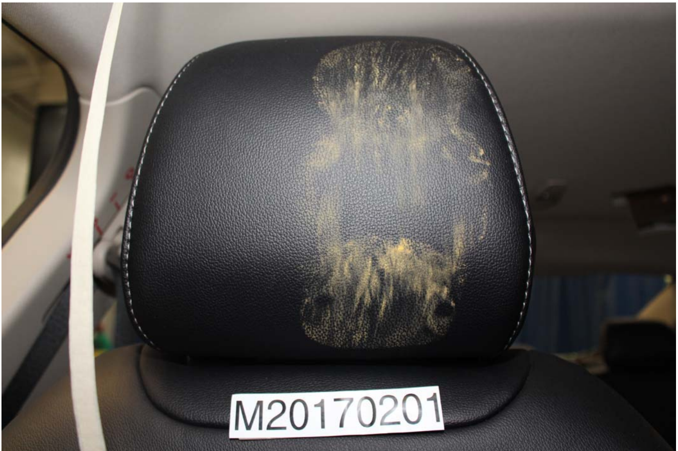
Photo No. 069 - Post-Test Passenger Dummy Contact with Headrest
