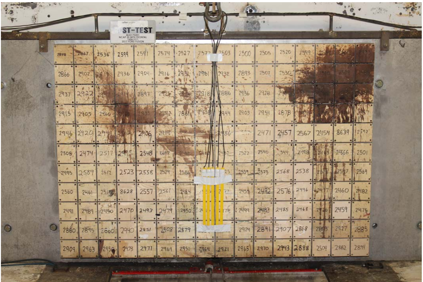
Photo No. 003 - Post-Test Load Cell Wall
