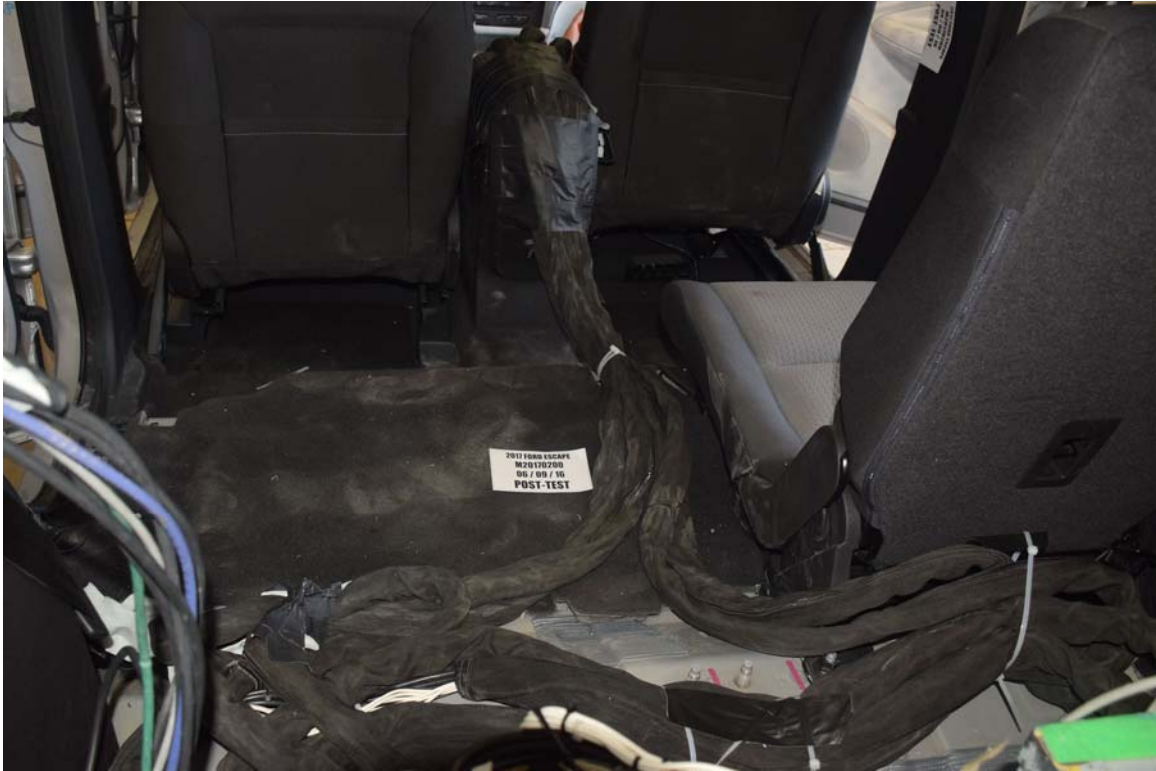
FIGURE 29. Post-Test Dummy Cable Routing
