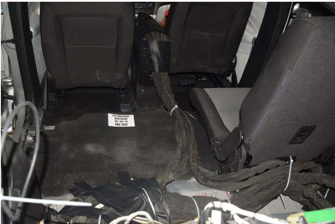
FIGURE 28. Pre-Test Dummy Cable Routing
