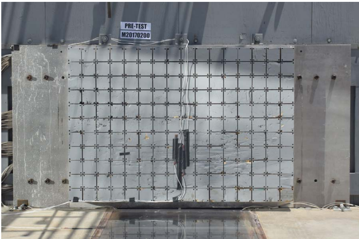
FIGURE 2. Pre-Test Load Cell Wall
