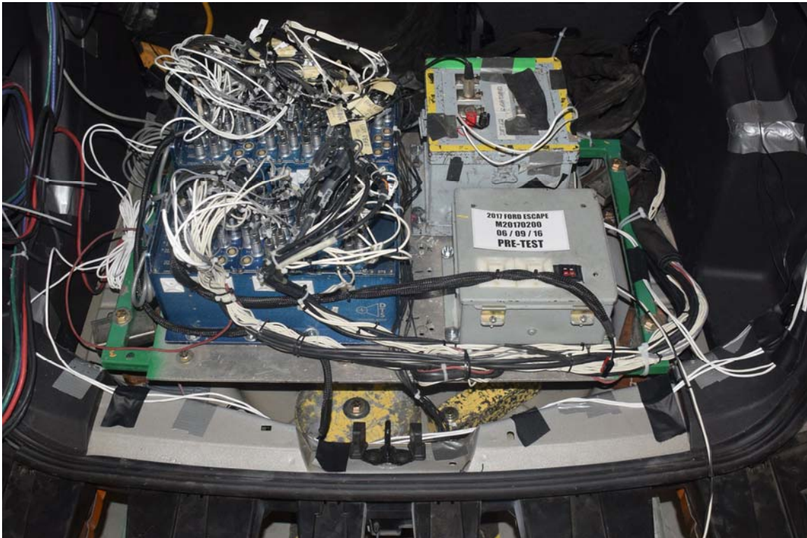
FIGURE 70. Photograph of Ballast Installed in Vehicle
