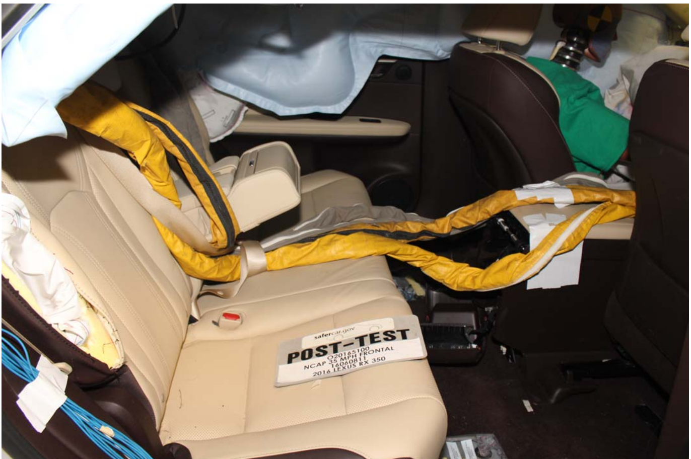
Photo No. 029 - Post-Test Dummy Cable Routing
