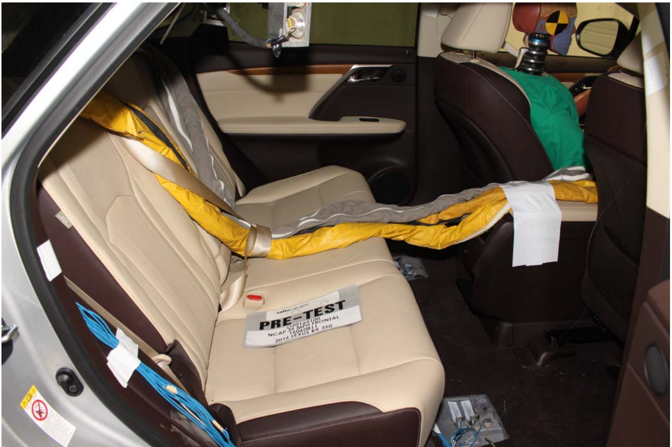
Photo No. 028 - Pre-Test Dummy Cable Routing
