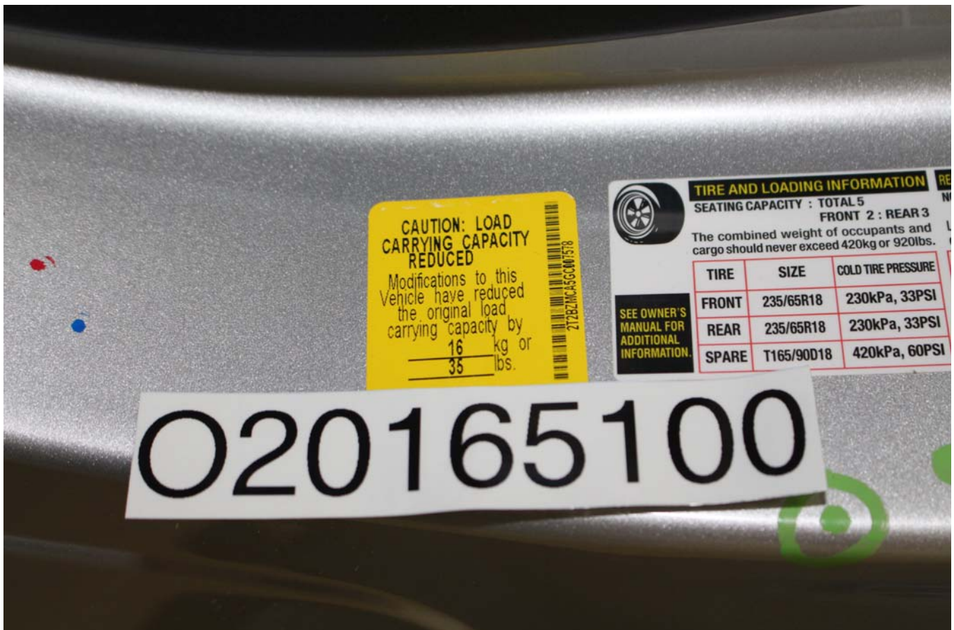
Photo No. 005a - Capacity Reduction Label
