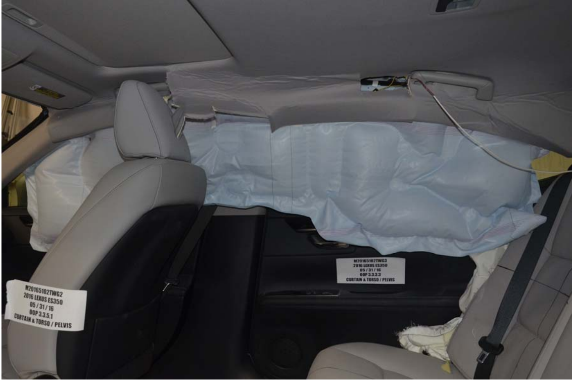
FIGURE 15. Post-Test Airbags, Left Side View
