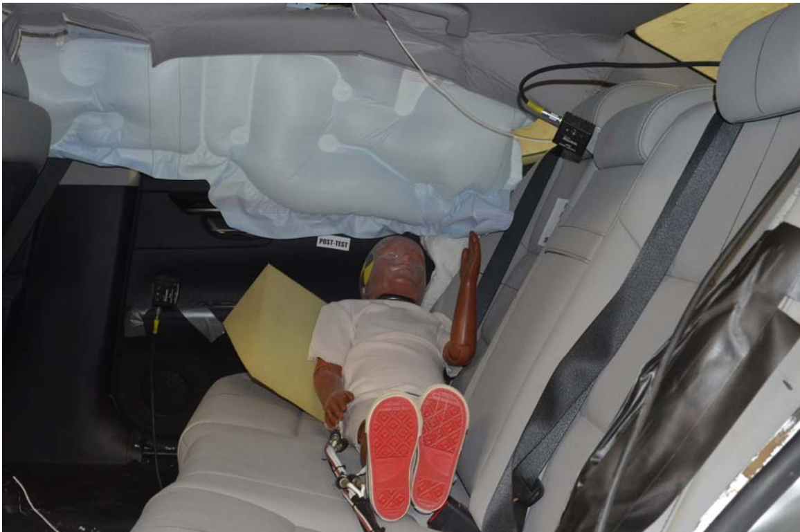
FIGURE 8. Post-Test Dummy Position, Left View
