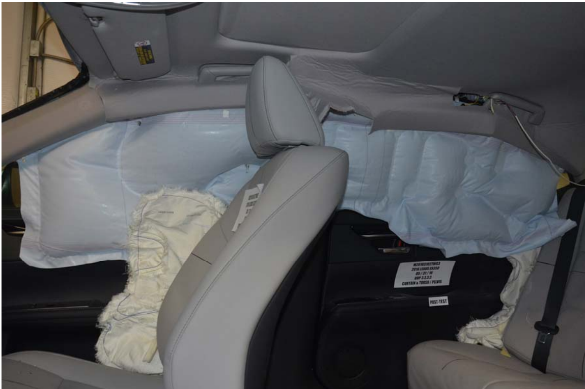
FIGURE 16. Post-Test Airbags, Left Front \frac{3}{4} View
