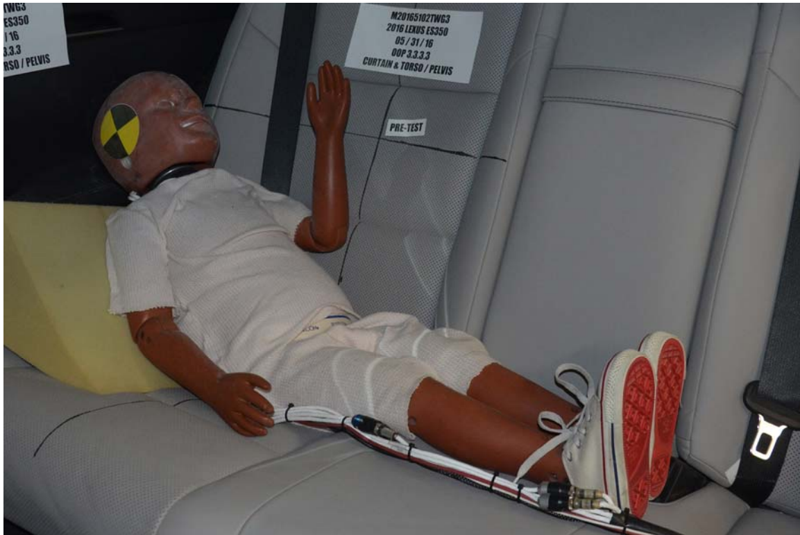
FIGURE 9. Pre-Test Dummy Position, \frac{3}{4} View
