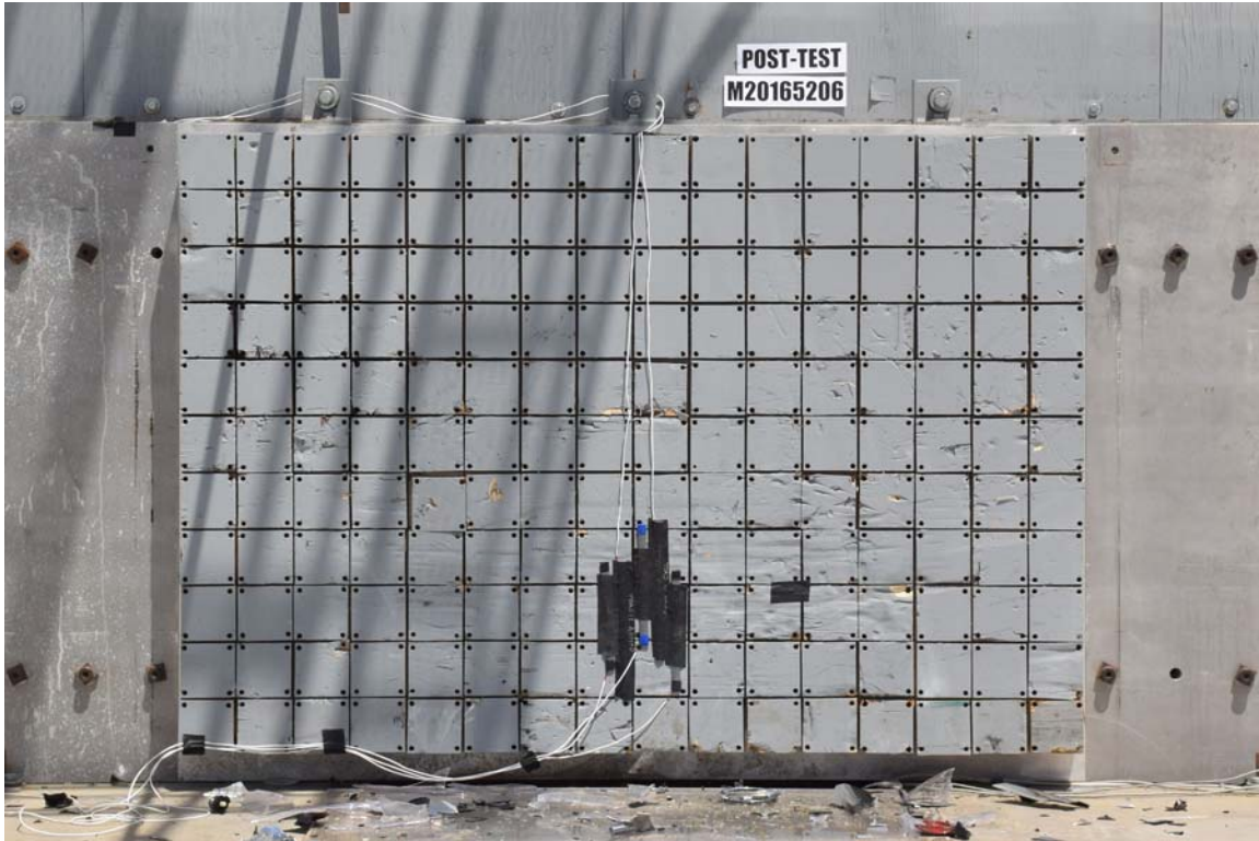
FIGURE 3. Post-Test Load Cell Wall
