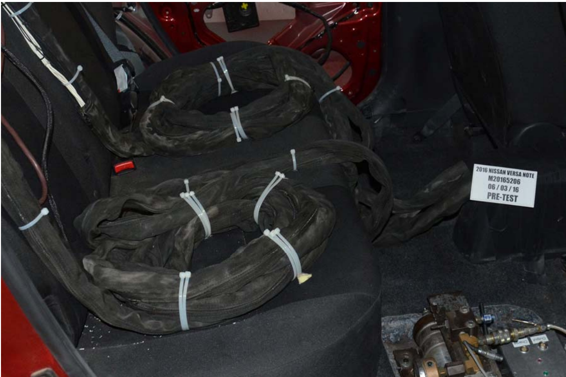
FIGURE 28. Pre-Test Dummy Cable Routing
