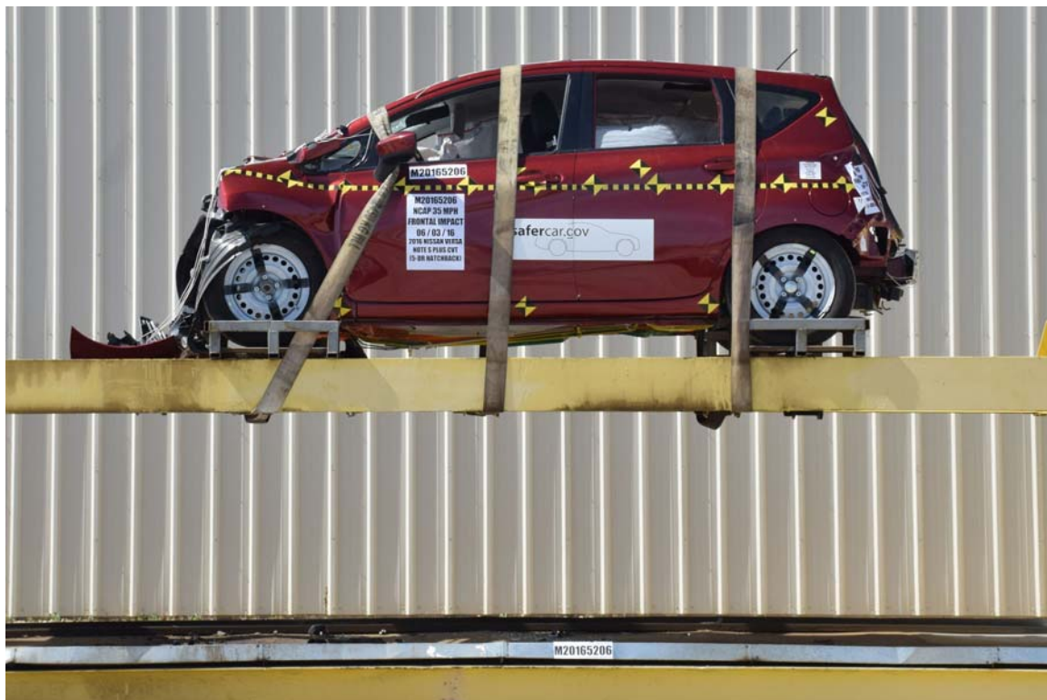
FIGURE 73. Vehicle at 0° on Static Rollover Device
