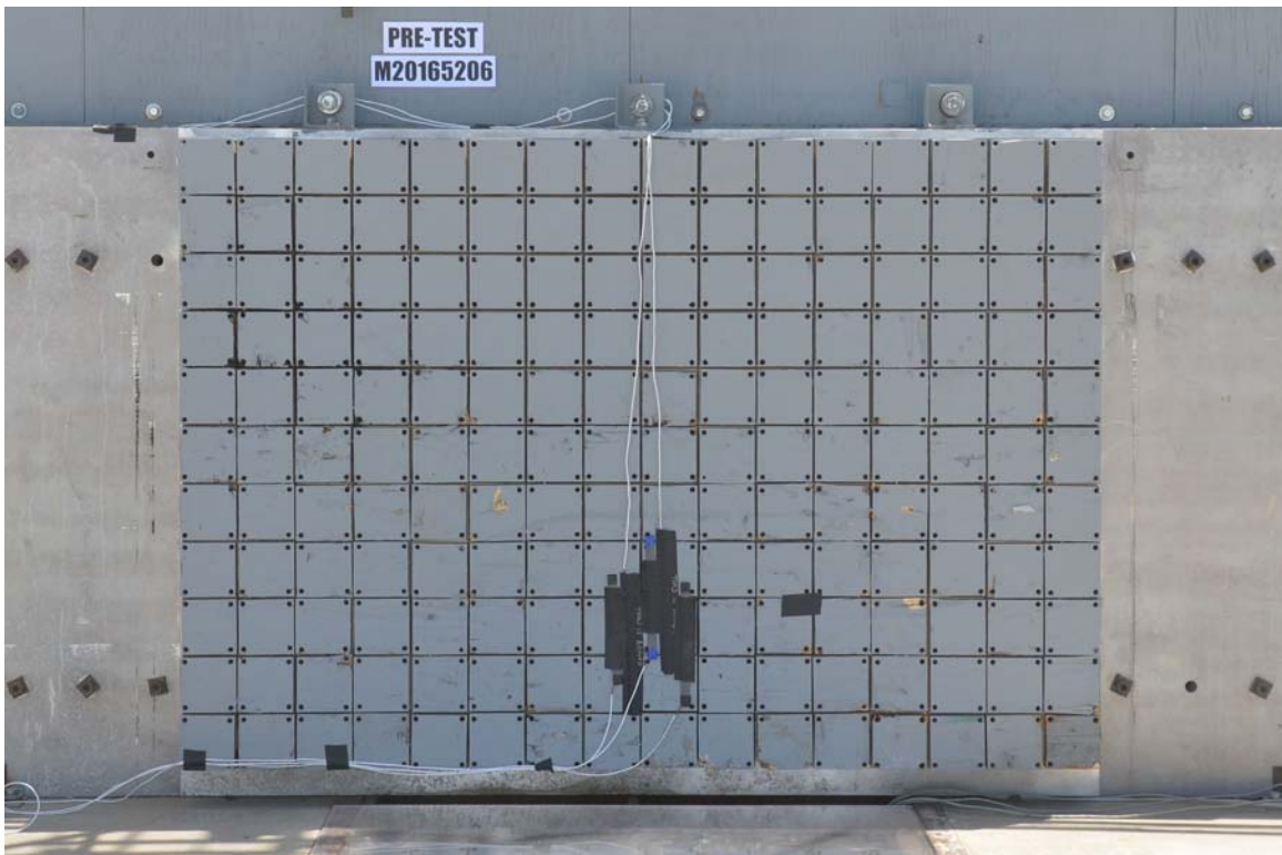
FIGURE 2. Pre-Test Load Cell Wall
