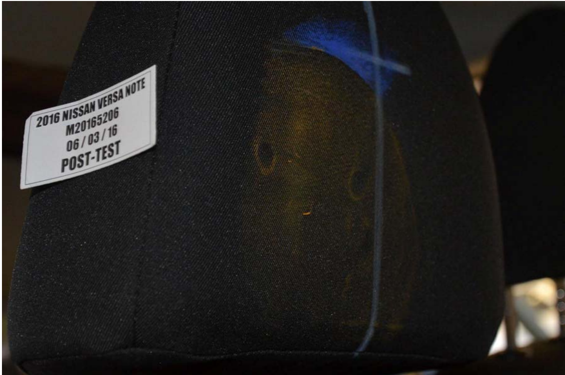
FIGURE 69. Post-Test Passenger Dummy Contact with Headrest
