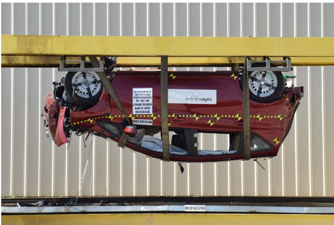
FIGURE 75. Vehicle at 180° on Static Rollover Device
