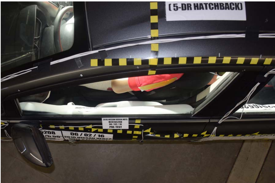
FIGURE 42. Pre-Test Driver Dummy and Door Clearance View
