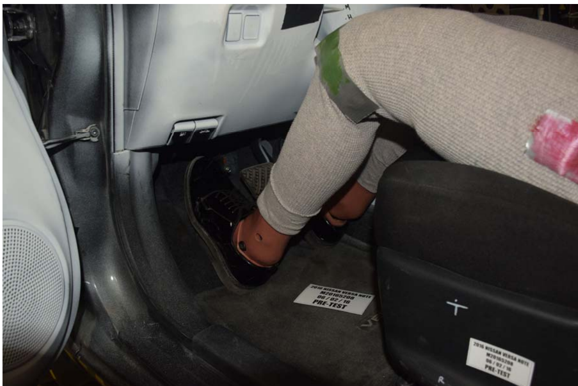
FIGURE 34. Pre-Test Placement of Driver Dummy's Feet
