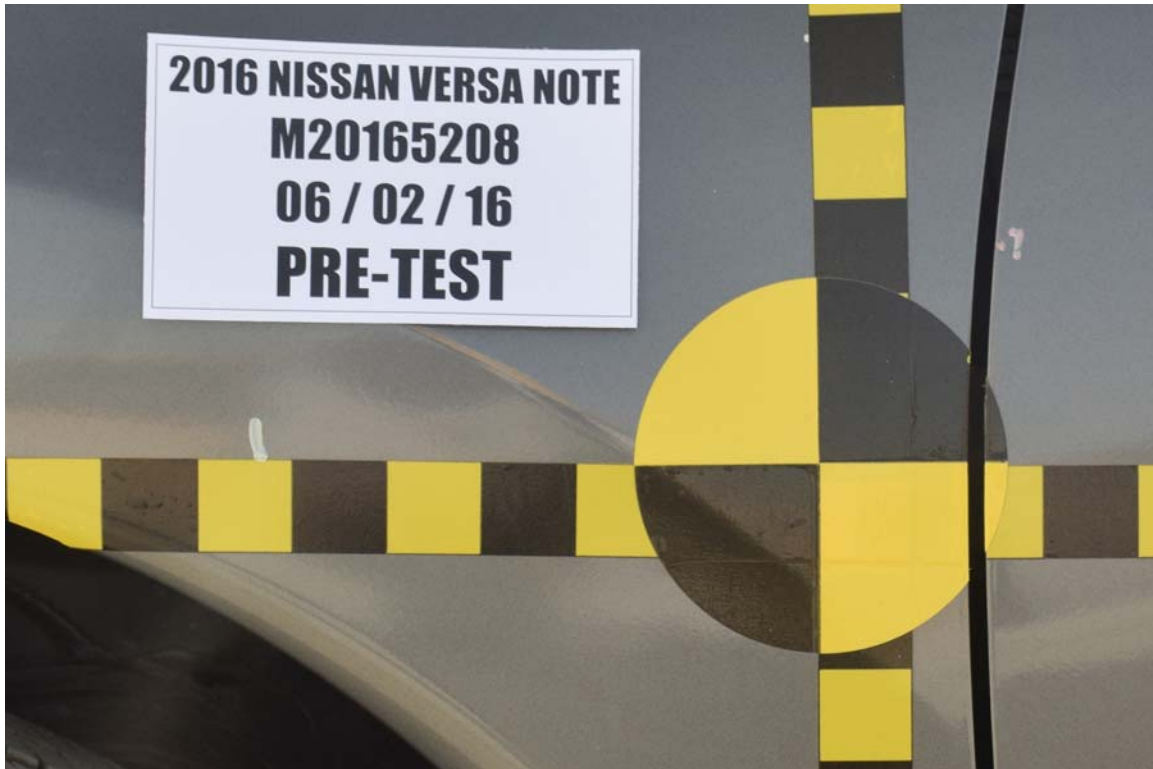
FIGURE 19. Pre-Test Close-Up View of Impact Point Target
