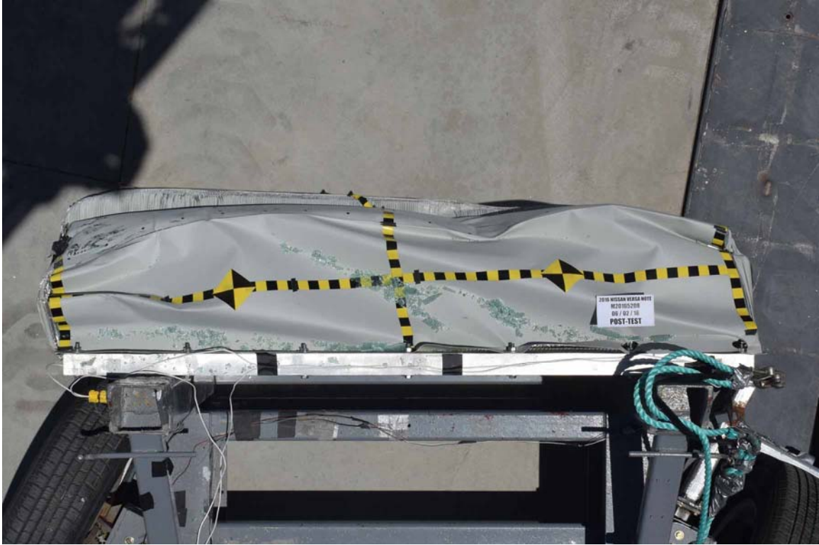
FIGURE 87. Post-Test Top View of MDB Impactor Face
