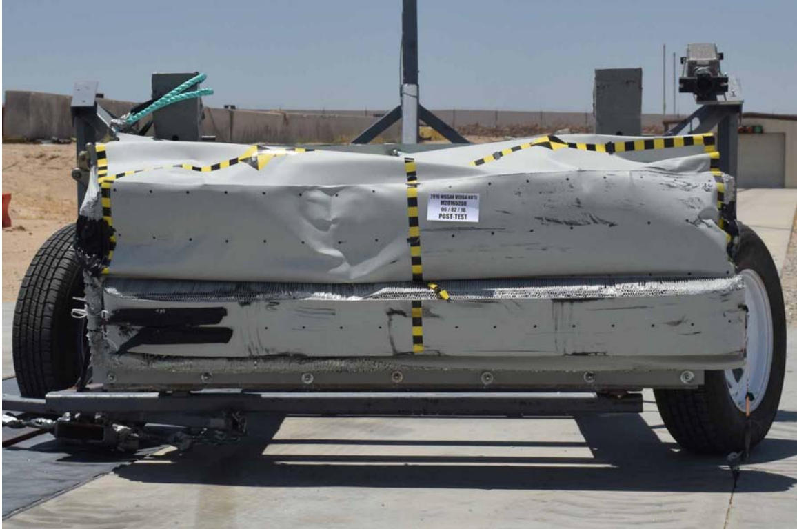
FIGURE 85. Post-Test Front View of MDB Impactor Face
