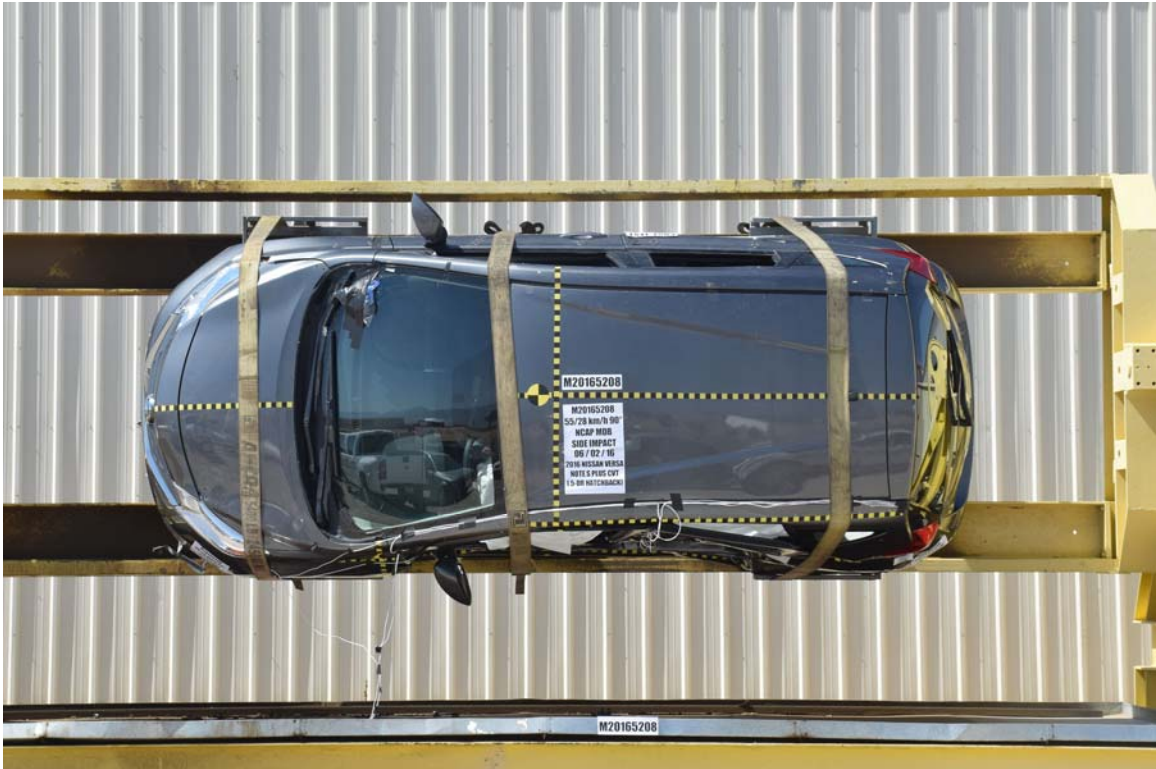
FIGURE 97. FMVSS No. 301 Static Rollover 90 Degrees
