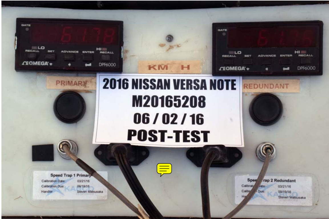
FIGURE 95. Post-Test Primary and Redundant Speed Trap Read-Out
