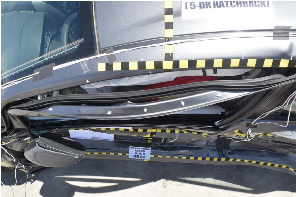
FIGURE 43. Post-Test Driver Dummy and Door Clearance View
