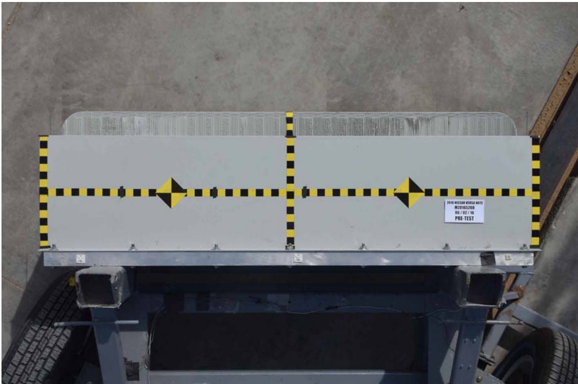
FIGURE 86. Pre-Test Top View of MDB Impactor Face
