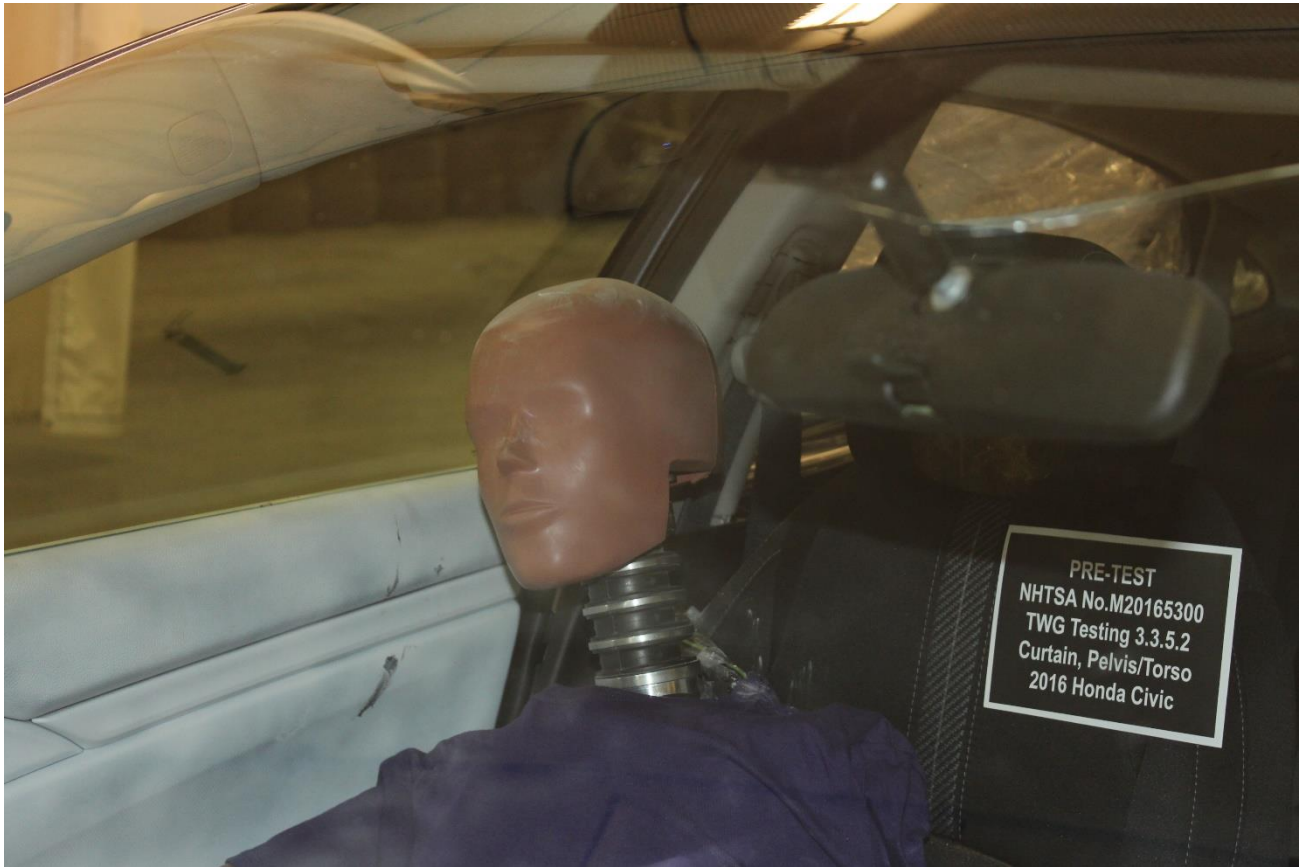
Figure A-9: Pre-Test SID-IIs 5th Female Left \frac{3}{4} Front Close-up View
