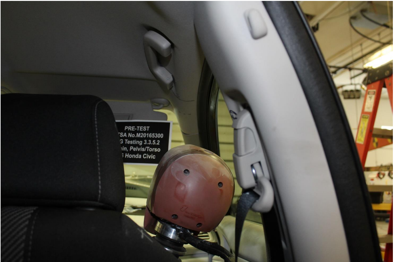
Figure A-17: Pre-Test SID-IIs 5th Female Rear Clearance View
