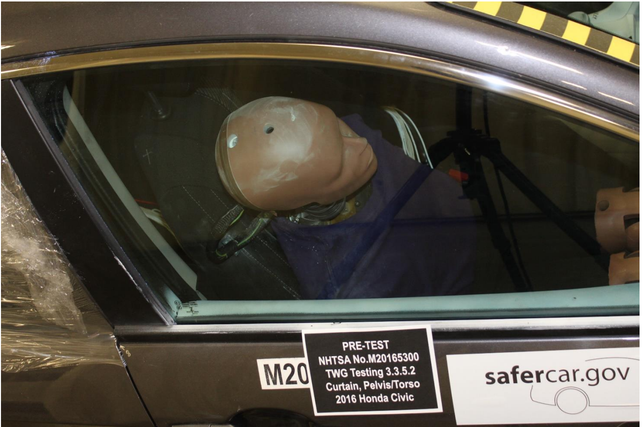
Figure A-15: Pre-Test SID-IIs 5th Female Right Side Clearance View
