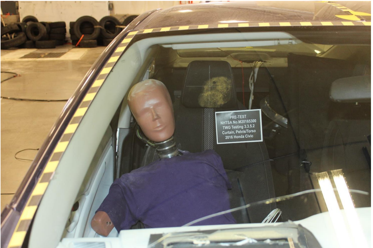
Figure A-11: Pre-Test SID-IIs 5th Female Front View
