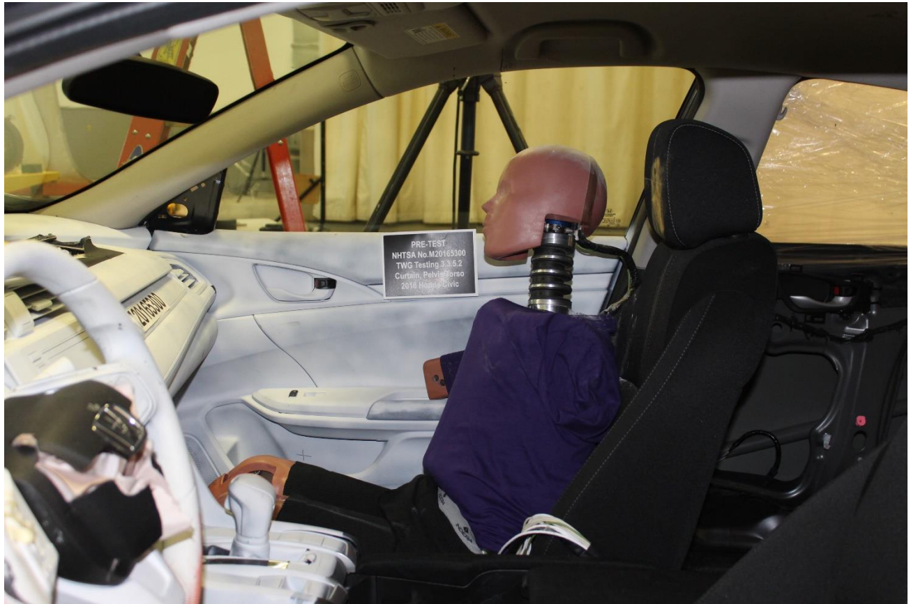
Figure A-3: Pre-Test SID-IIs 5th Female Left Side View
