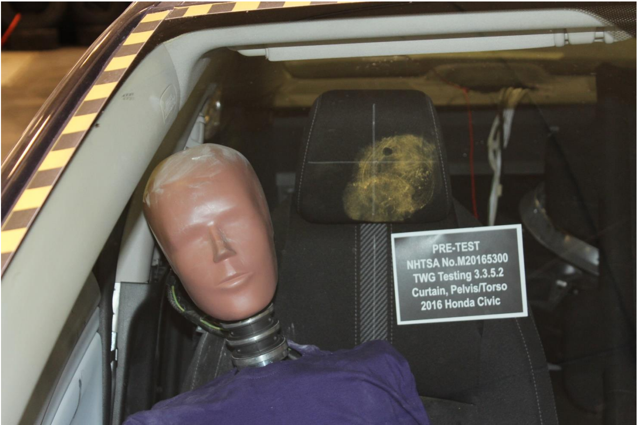
Figure A-13: Pre-Test SID-IIs 5th Female Front Close-up View
