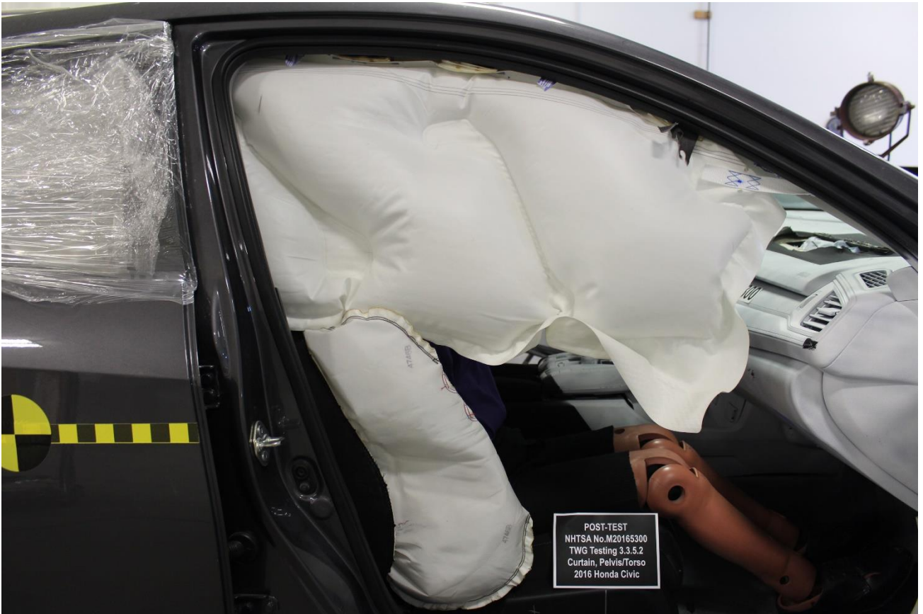
Figure A-19: Post-Test Torso and Curtain Airbag(s) Right Side View
