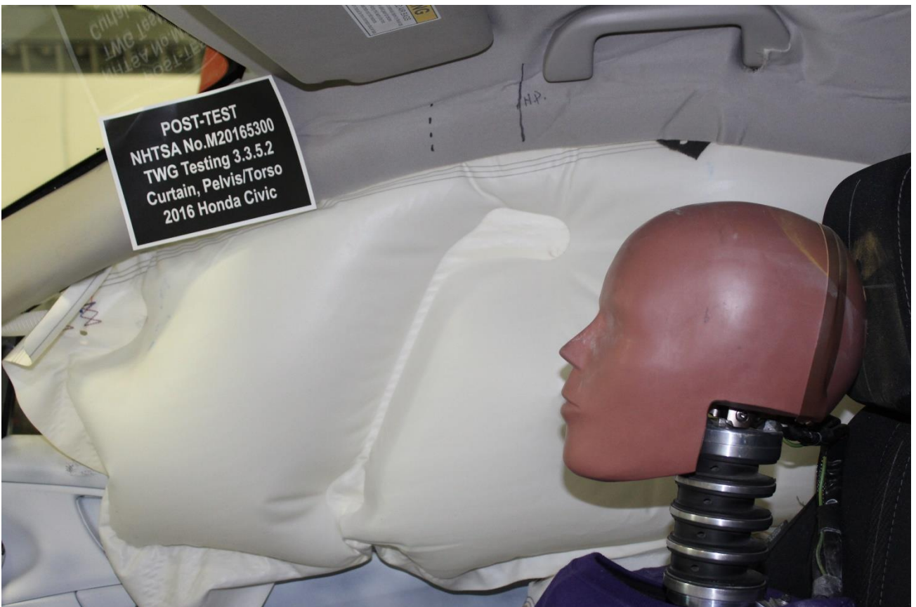
Figure A-18: Post-Test Curtain Airbag Left Side View
