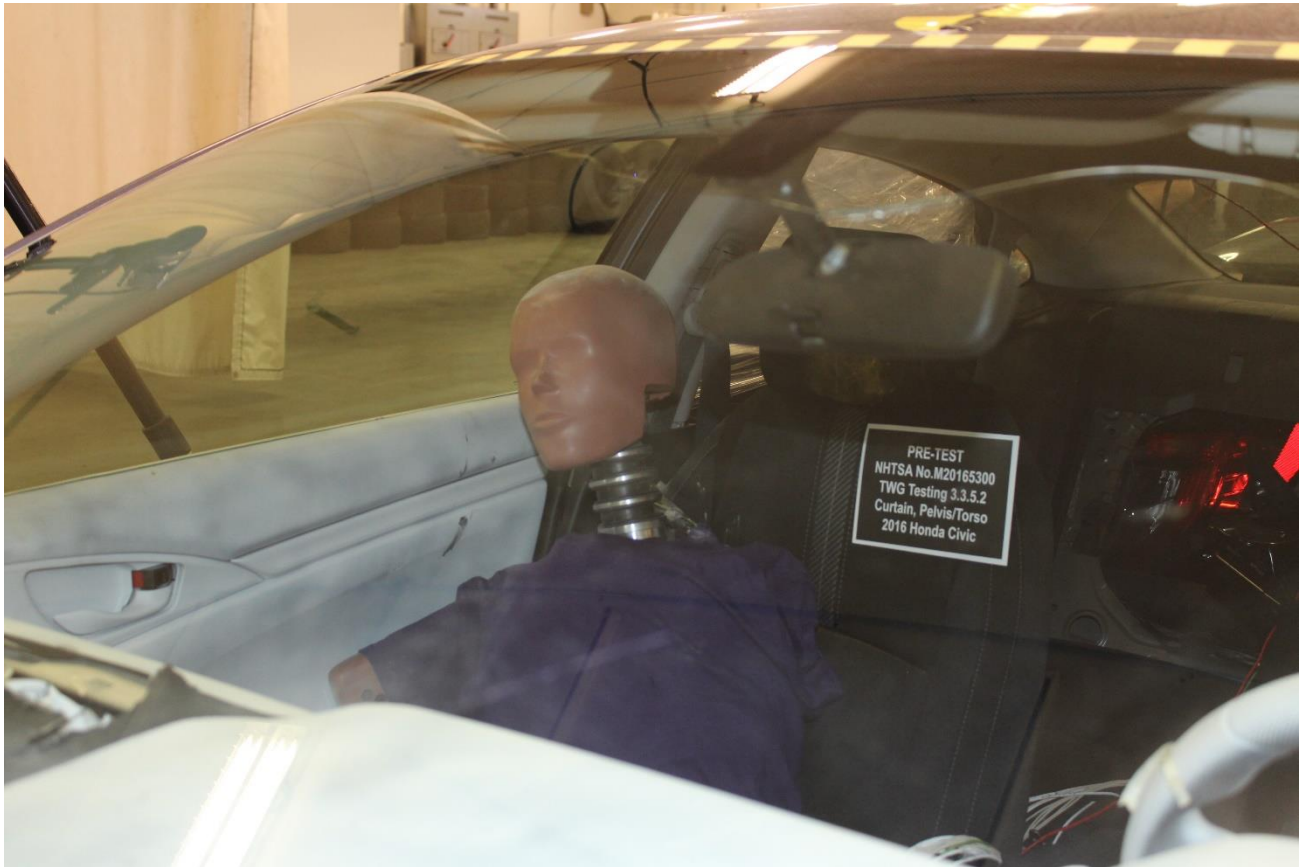
Figure A-7: Pre-Test SID-IIs 5th Female Left \frac{3}{4} Front View
