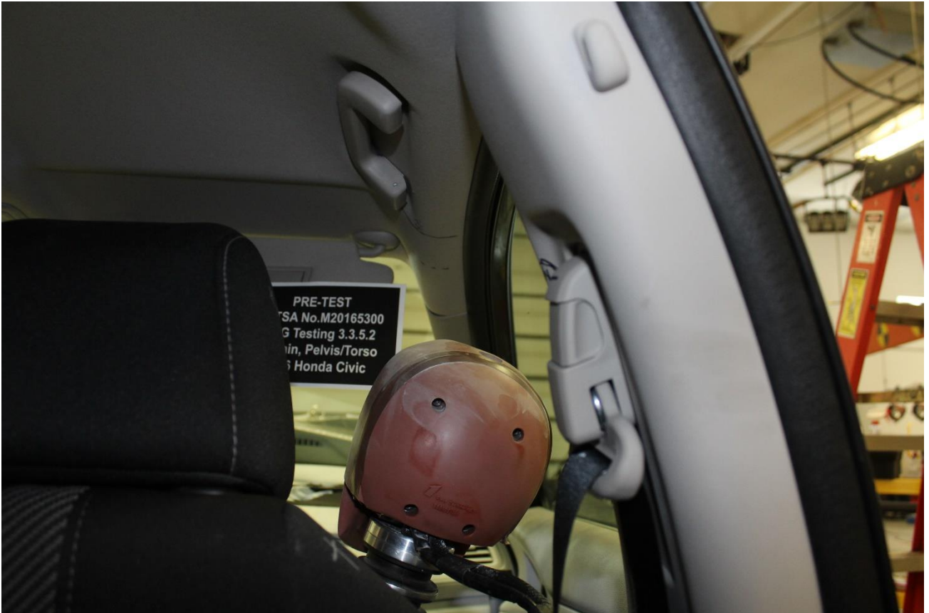
Figure A-14: Pre-Test SID-IIs 5th Female Rear View
