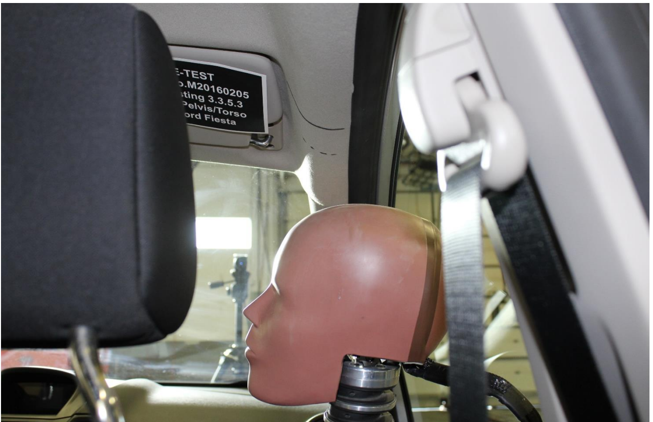
Figure A-16: Pre-Test SID-IIs 5th Female Rear Clearance View
