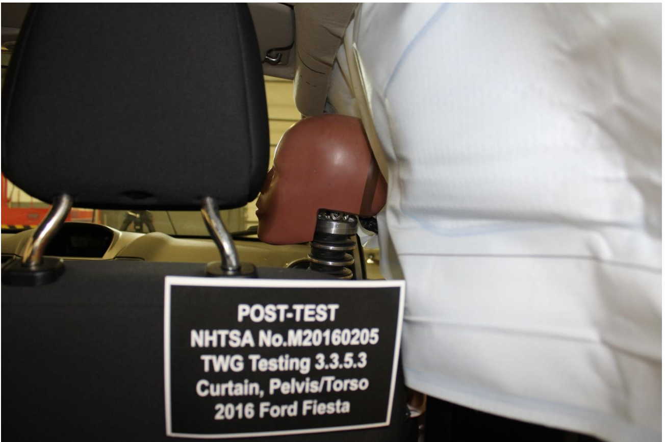
Figure A-17: Post-Test SID-IIs 5th Female Rear Clearance View
