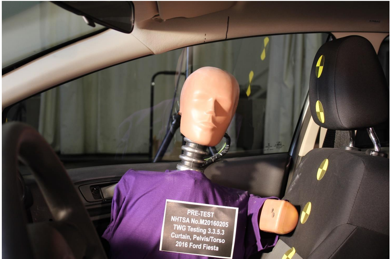
Figure A-5: Pre-Test SID-IIs 5th Female Left Side Close-up View
