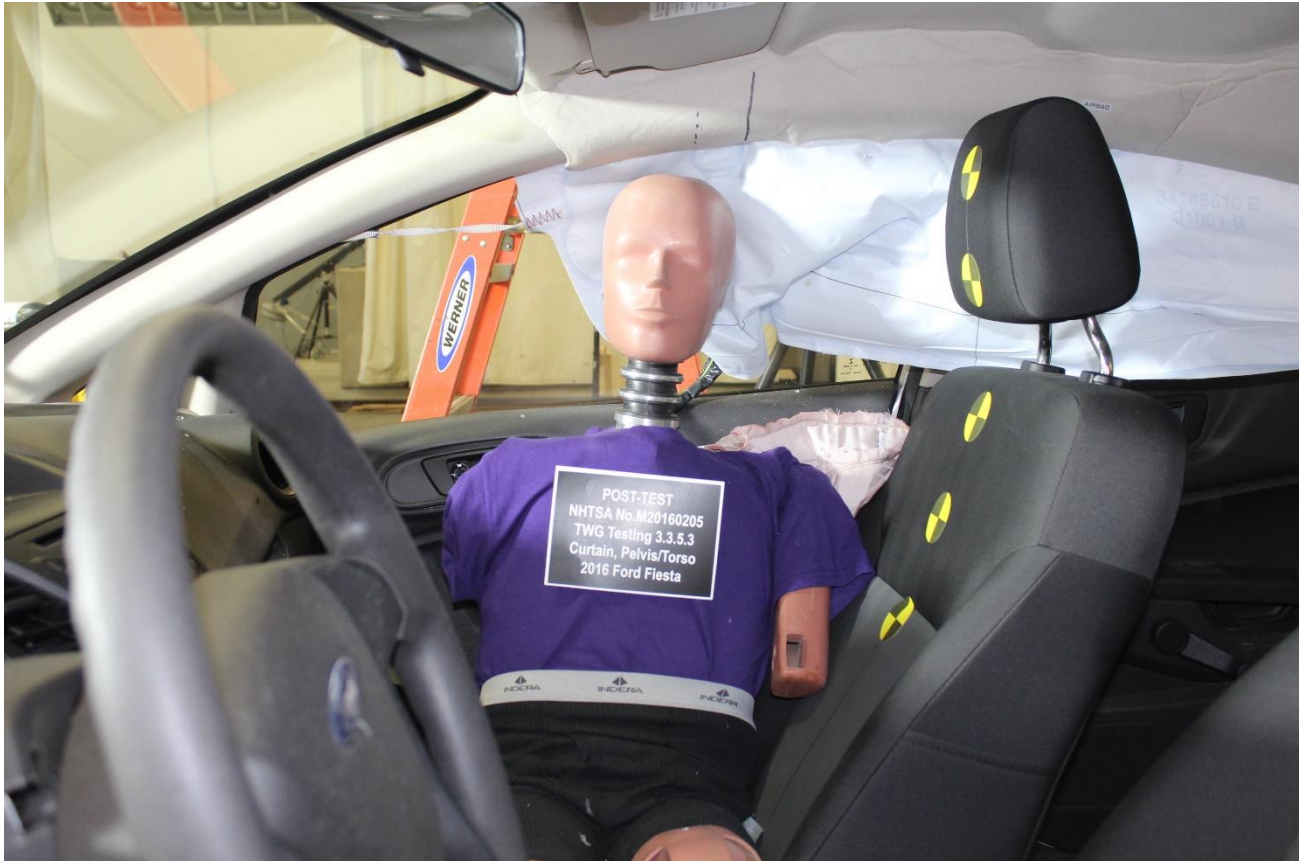
Figure A-4: Post-Test SID-IIs 5th Female Left Side View
