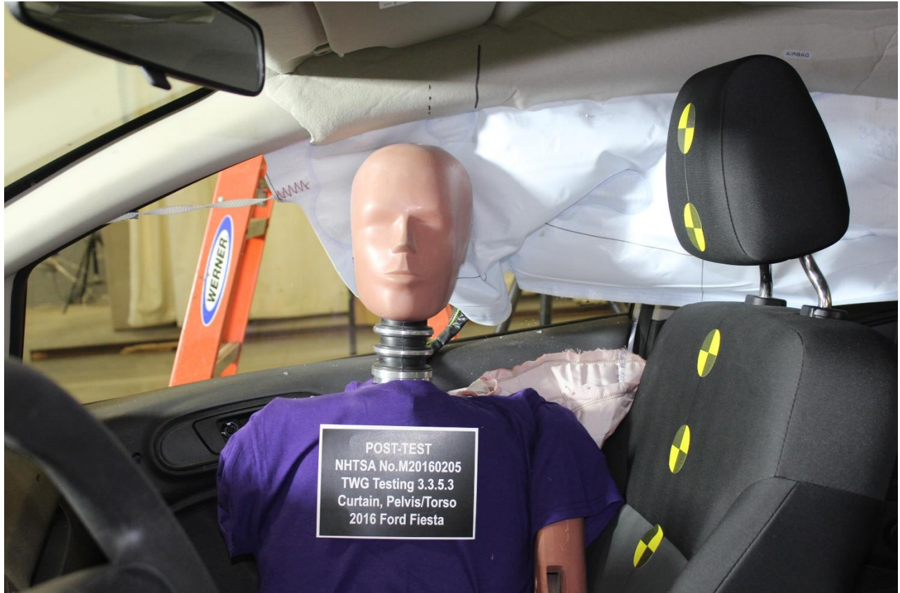
Figure A-6: Post-Test SID-IIs 5th Female Left Side Close-up View
