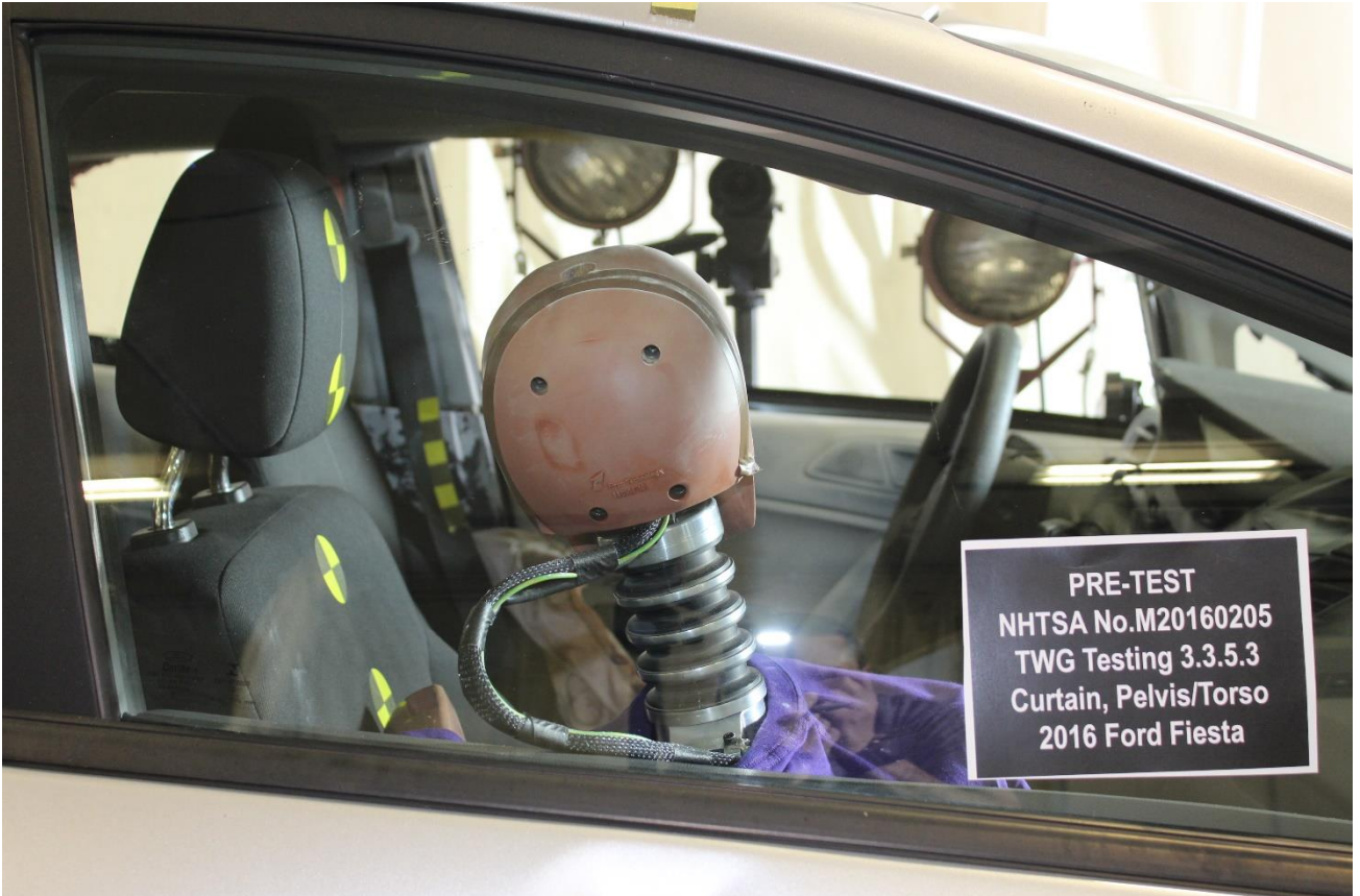
Figure A-14: Pre-Test SID-IIs 5th Female Right Side View
