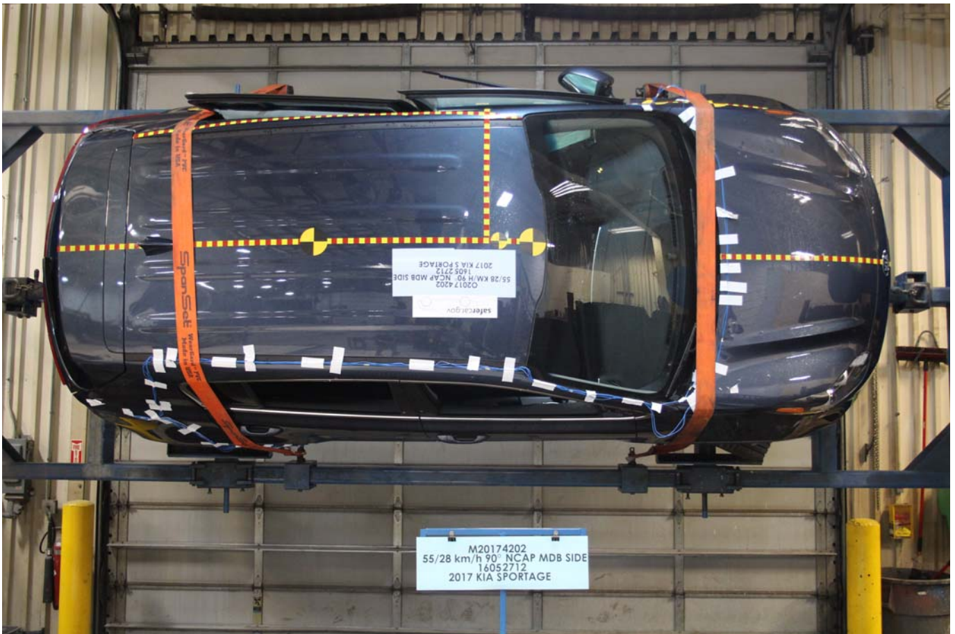
Photo No. 099 - FMVSS No. 301 Static Rollover 270 Degrees
