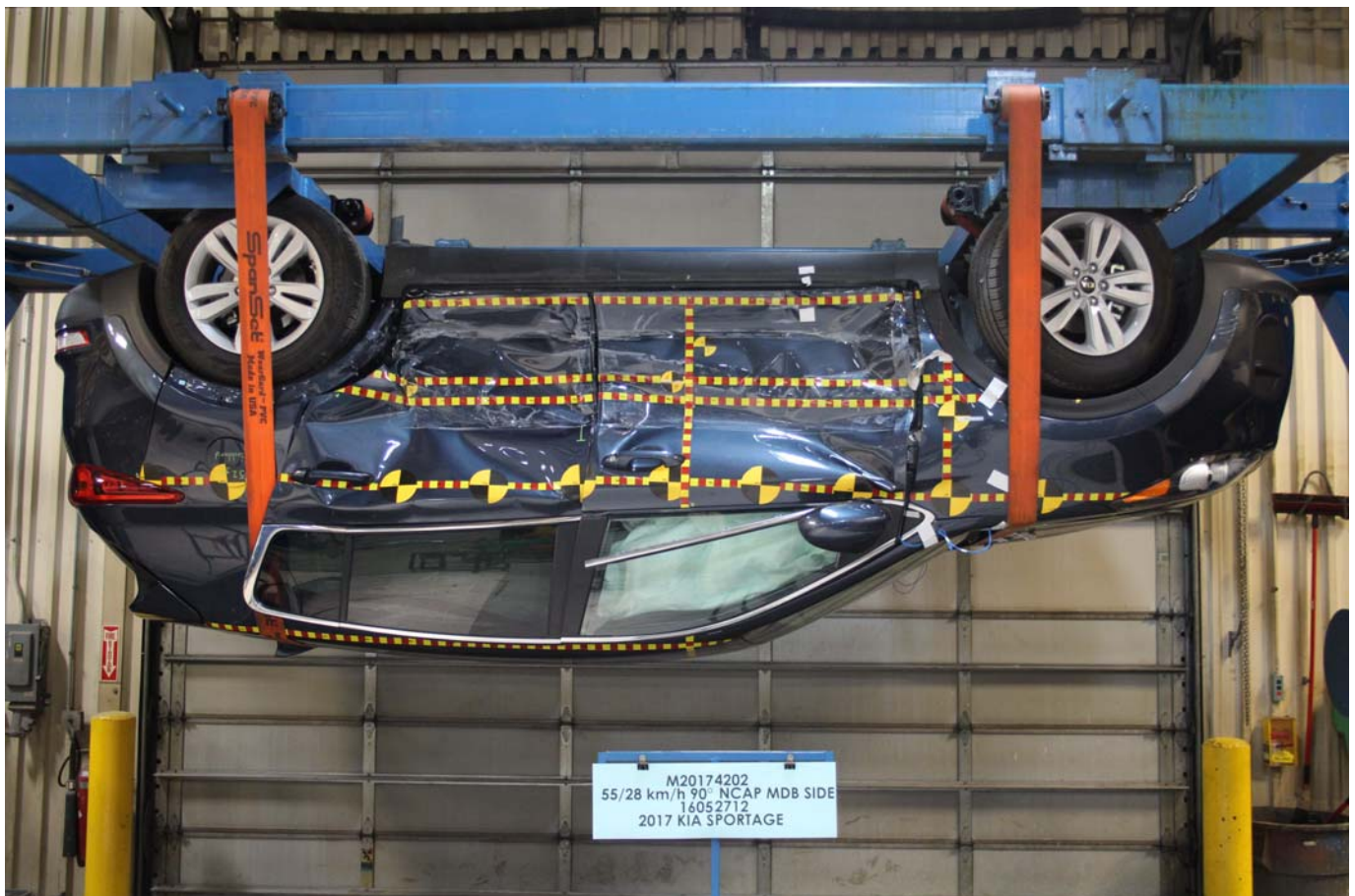
Photo No. 098 - FMVSS No. 301 Static Rollover 180 Degrees
