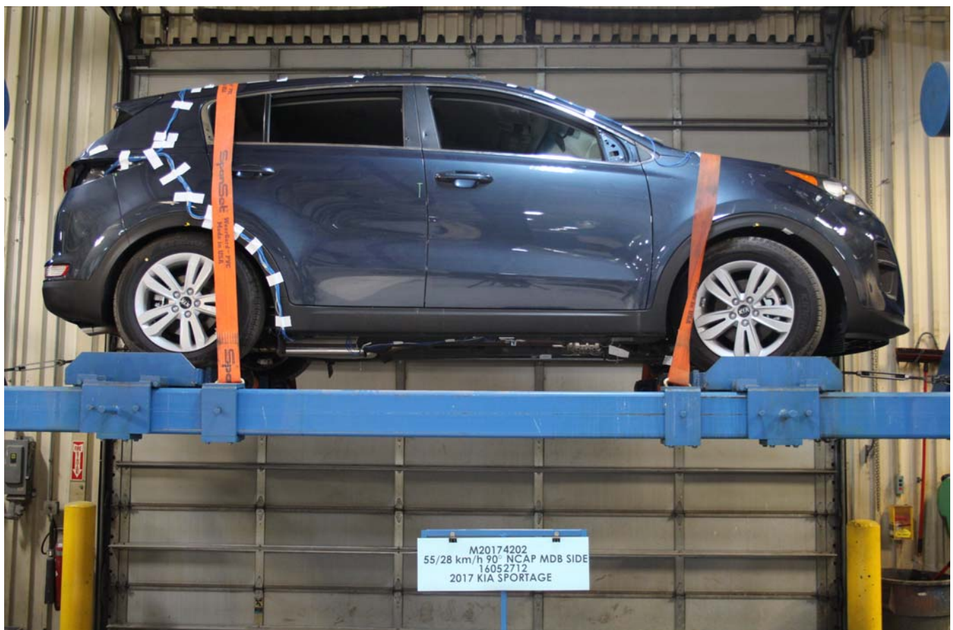
Photo No. 096 - FMVSS No. 301 Static Rollover 0 Degrees
