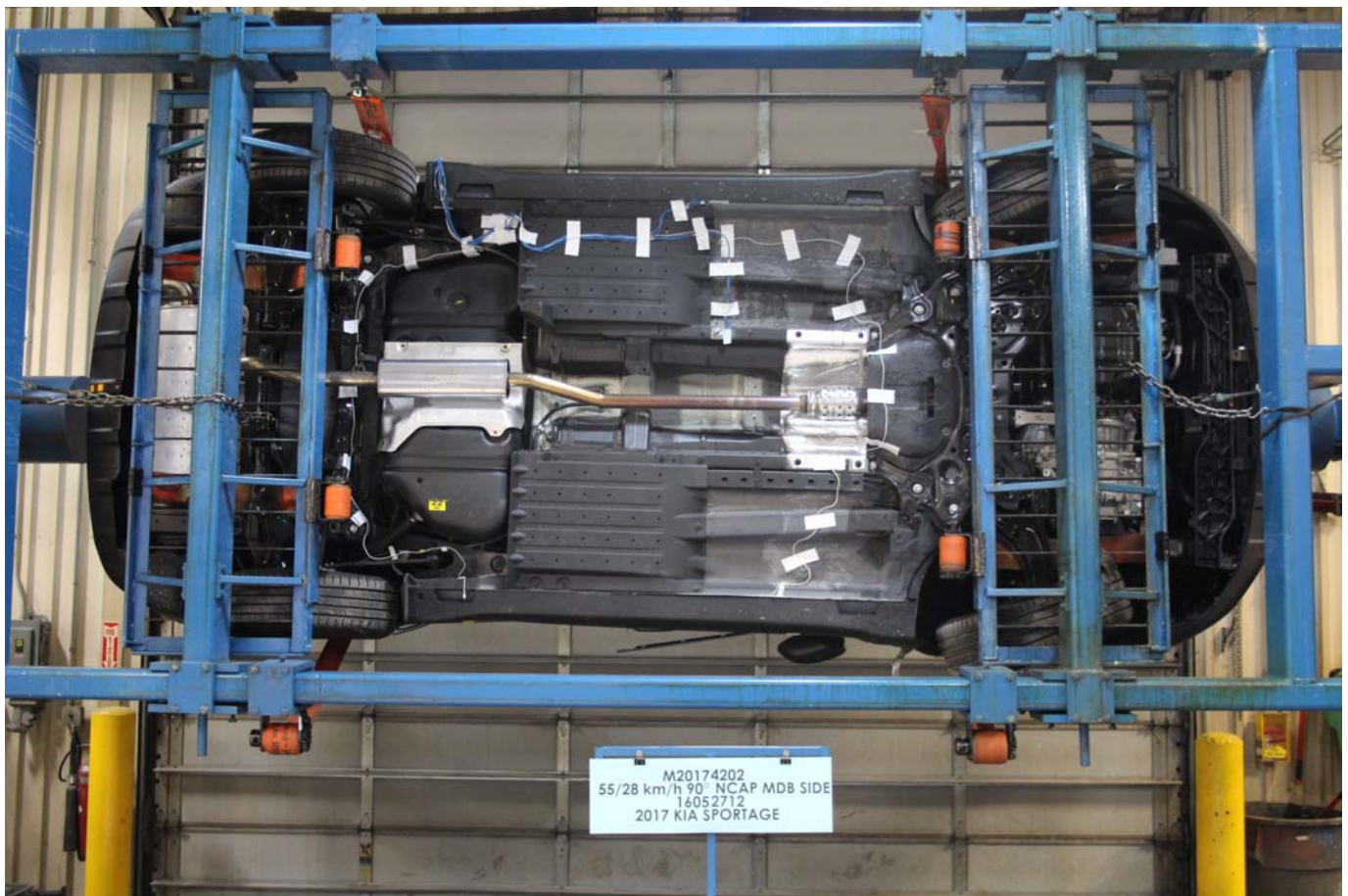
Photo No. 097 - FMVSS No. 301 Static Rollover 90 Degrees
