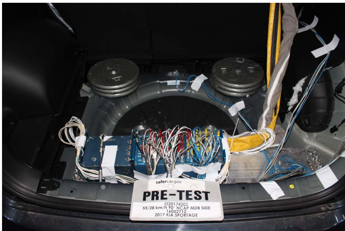
Photo No. 094 - Pre-Test Ballast View
