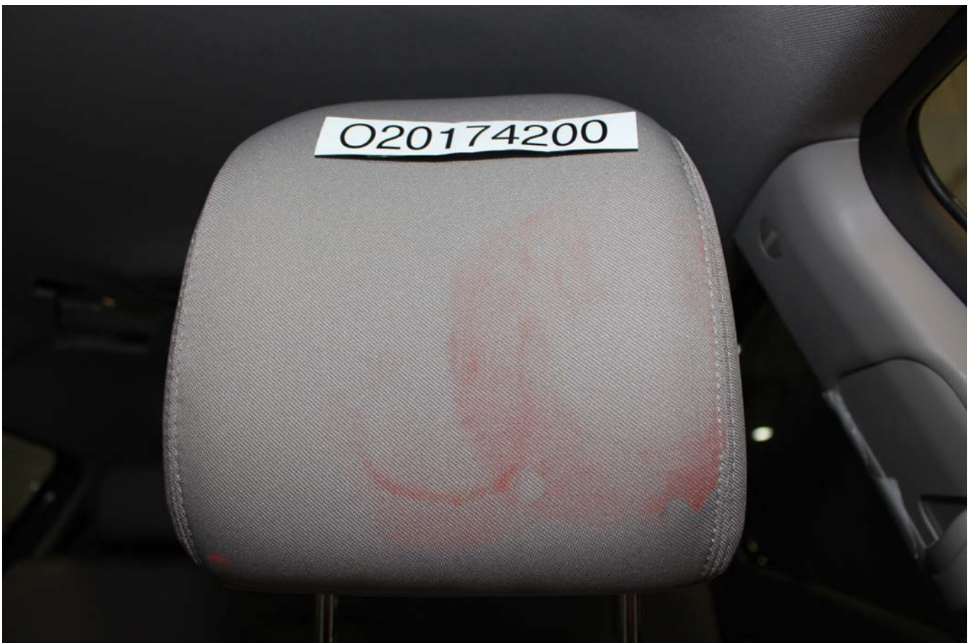
Photo No. 048 - Post-Test Driver Dummy Contact with Headrest
