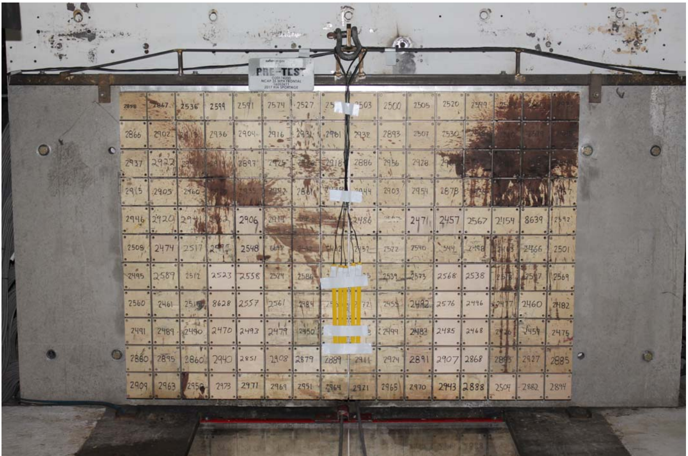
Photo No. 002 - Pre-Test Load Cell Wall
