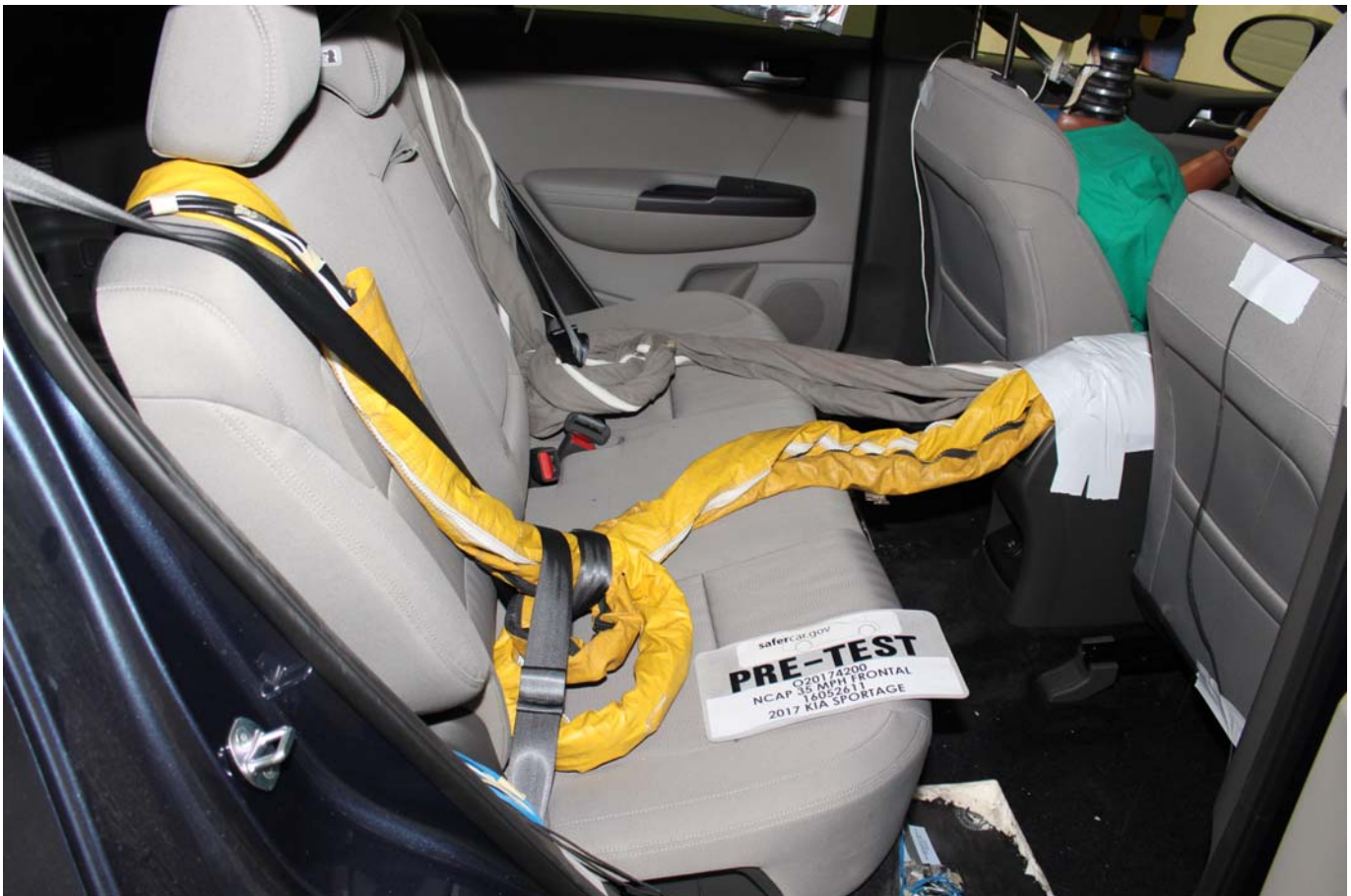
Photo No. 028 - Pre-Test Dummy Cable Routing
