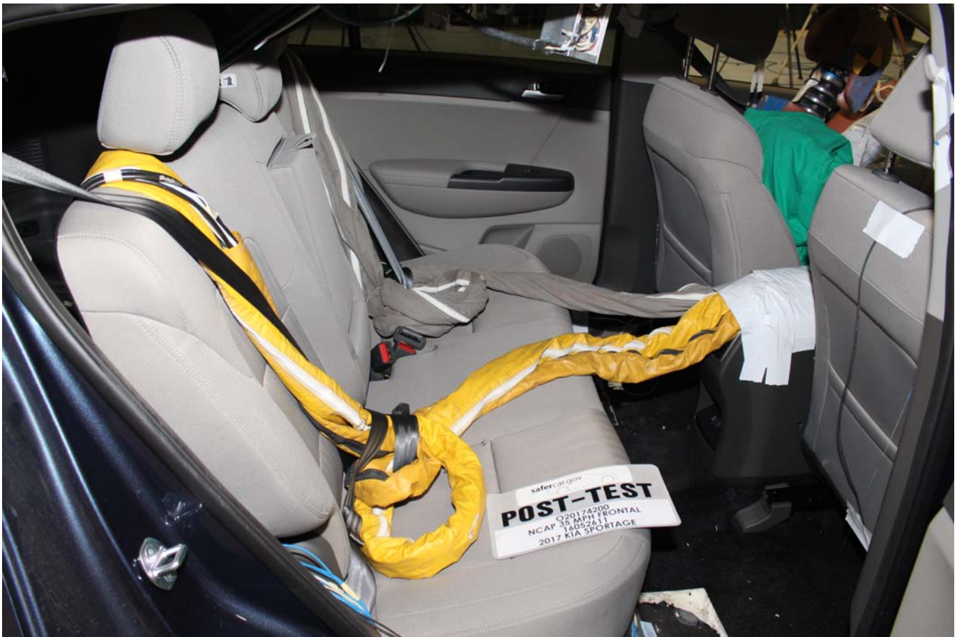
Photo No. 029 - Post-Test Dummy Cable Routing
