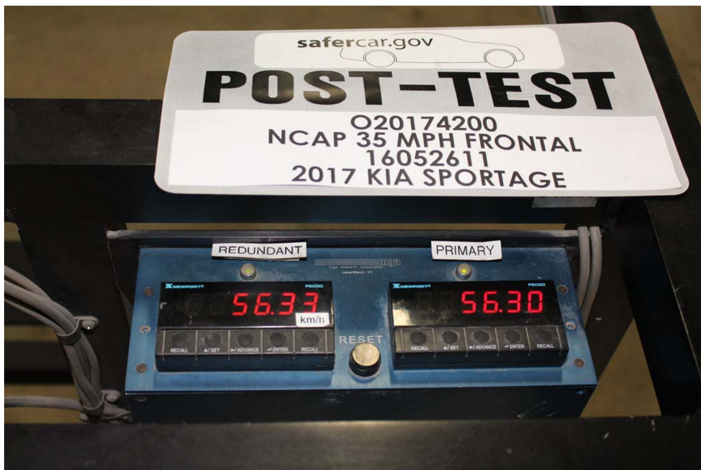
Photo No. 072 - Post-Test Speed Trap Read-Out
