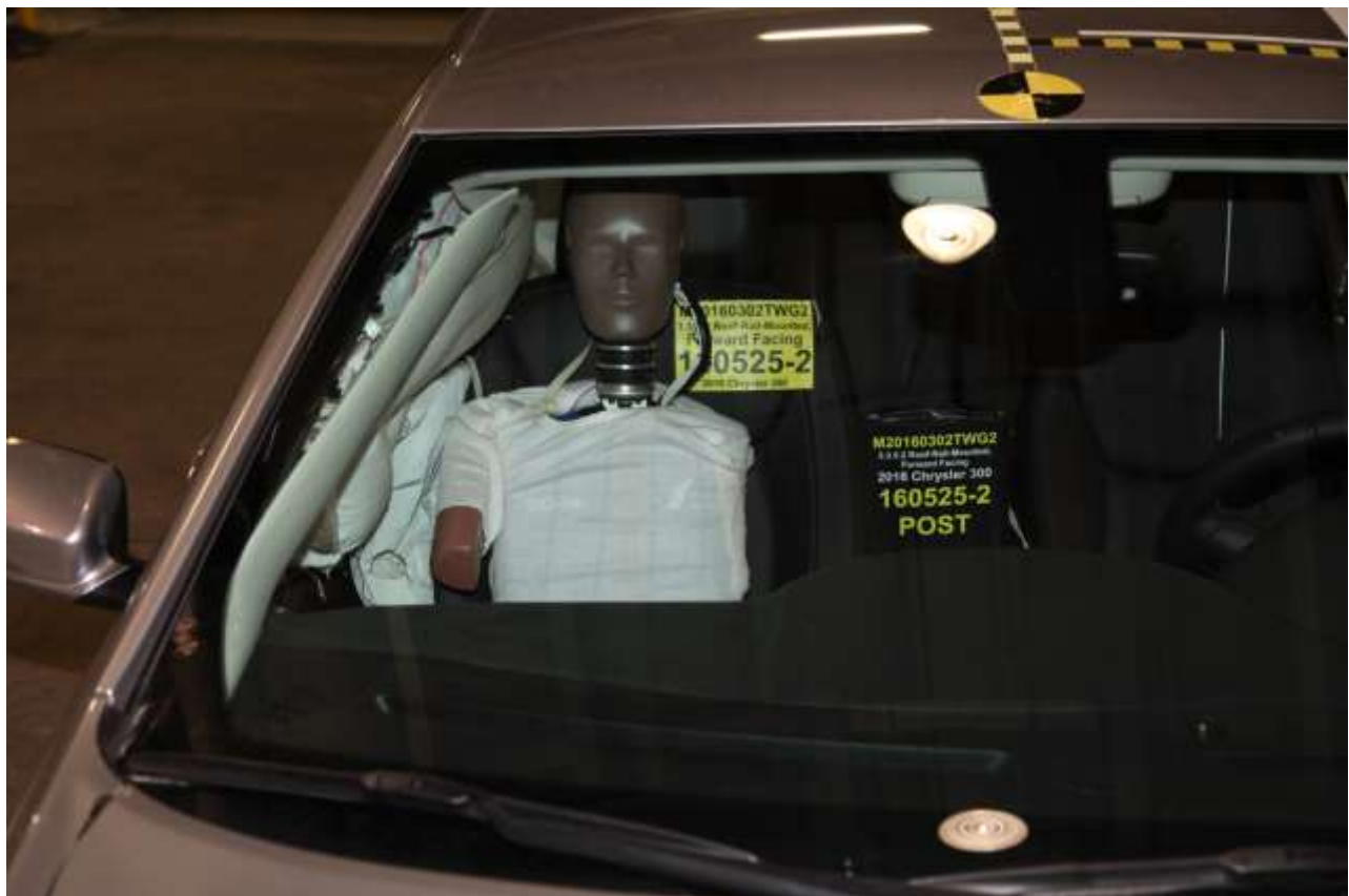
Figure A-18 Post-Test SIDI Dummy - Front View
