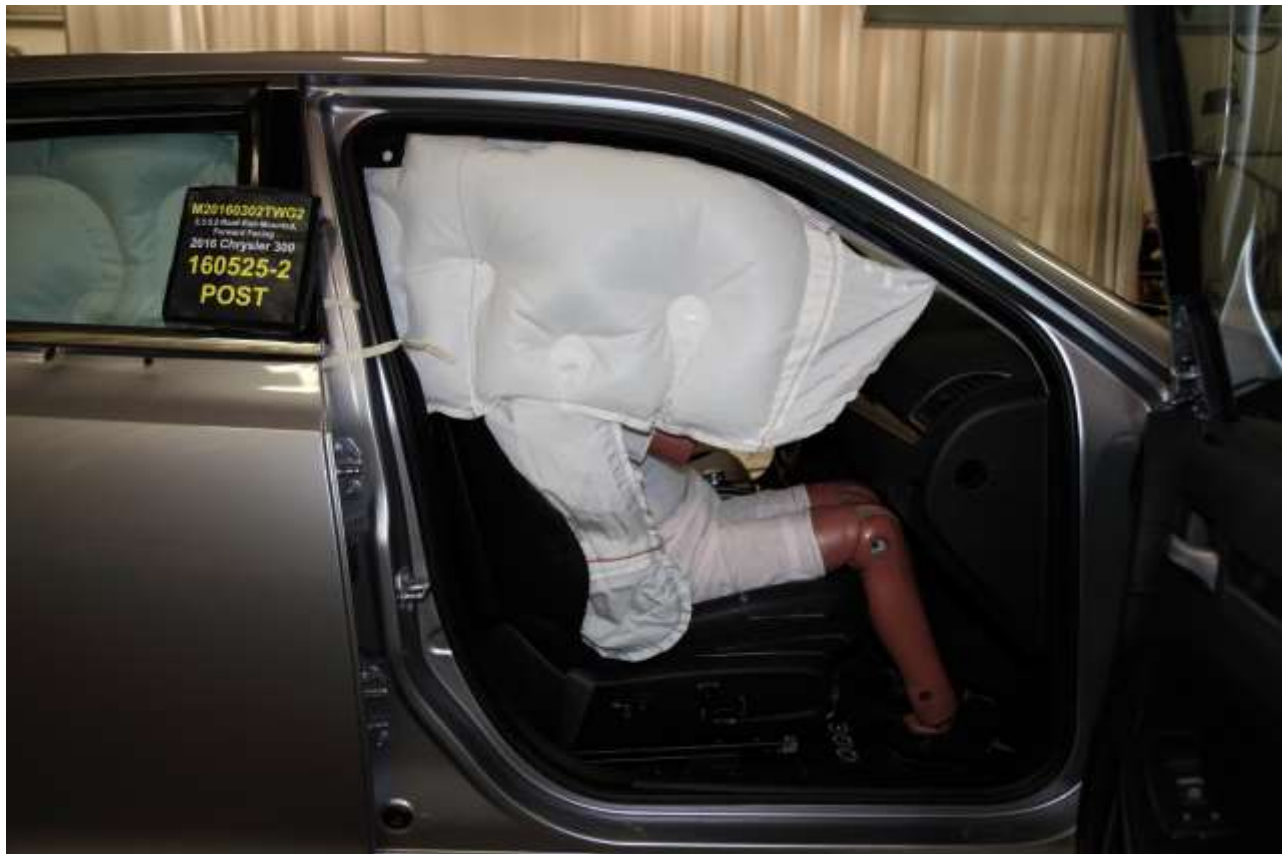
Figure A-25 Post-Test SIDII Dummy - Right Side View (Door Open)
