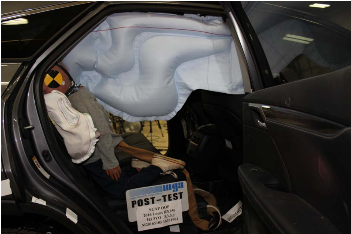
Photo No. 21. Post-Test 3-Year-Old Child Dummy Right Side View (Door Open)
