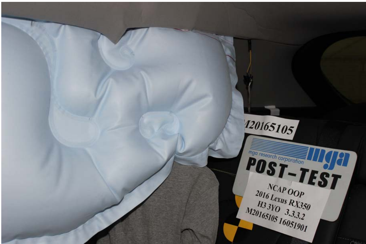
Photo No. 12. Post-Test 3-Year-Old Child Dummy Left \frac{3}{4} Front Closeup View
