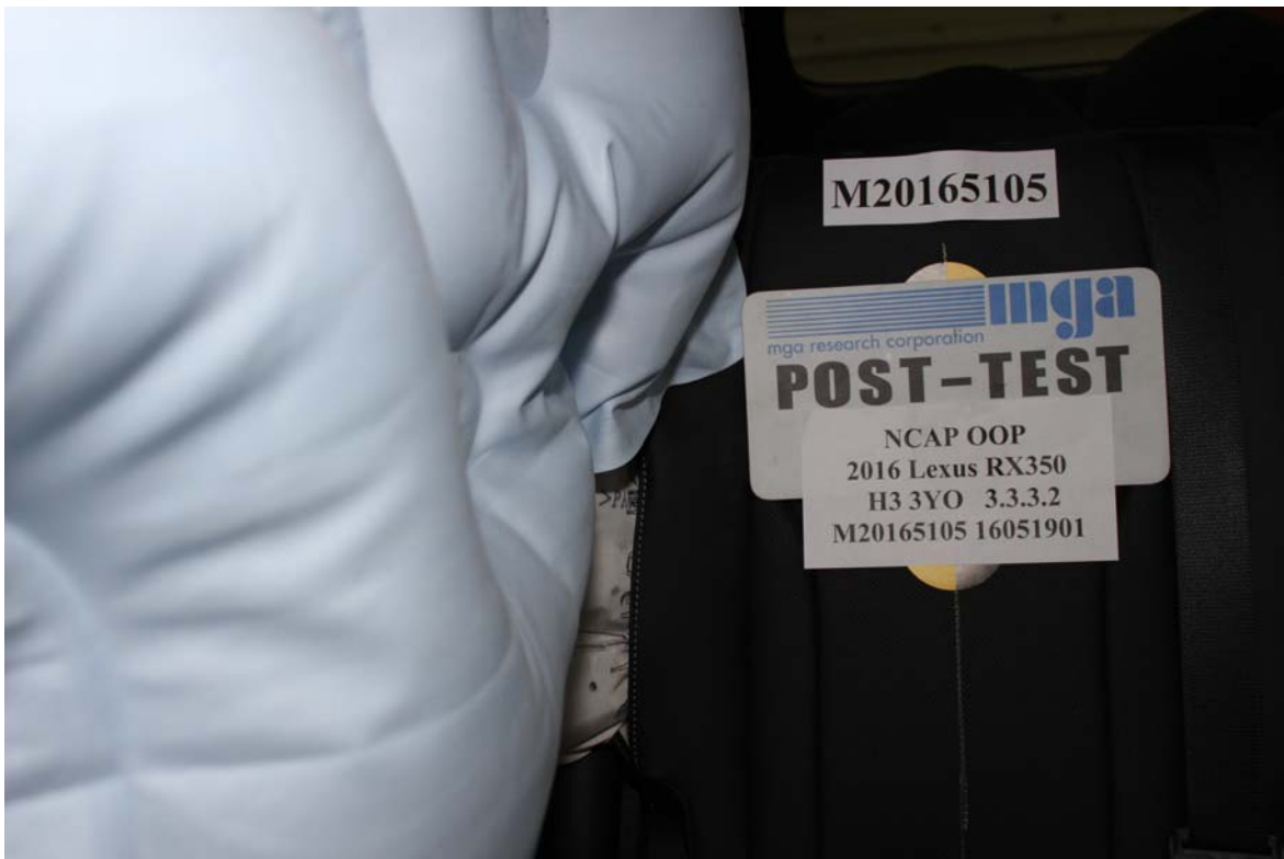
Photo No. 24. Post-Test Curtain Airbag Front View
