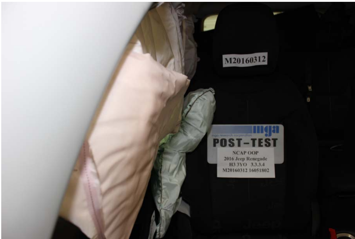
Photo No. 24. Post-Test Curtain Airbag Front View
