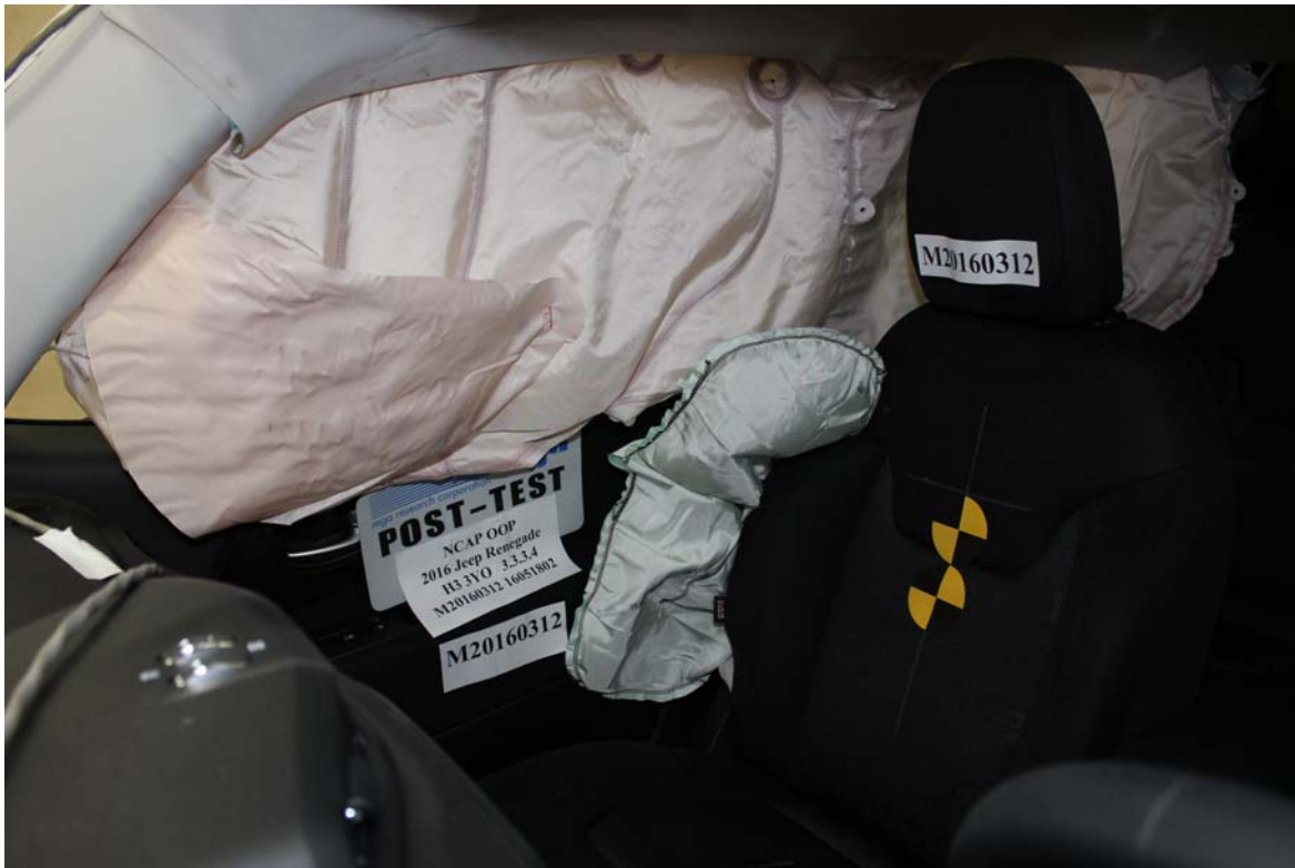
Photo No. 23. Post-Test Curtain Airbag Left \frac{3}{4} Front View
