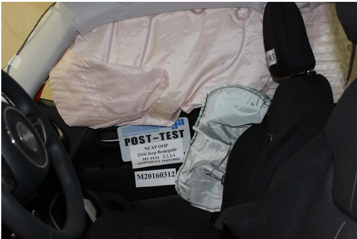
Photo No. 22. Post-Test Curtain Airbag Left Side View
