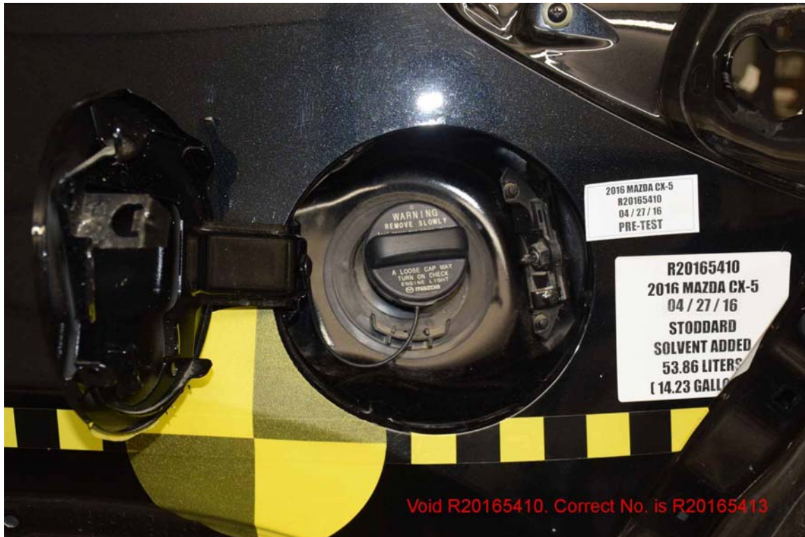
FIGURE 127. Pre-Test View of Fuel Filler Cap
