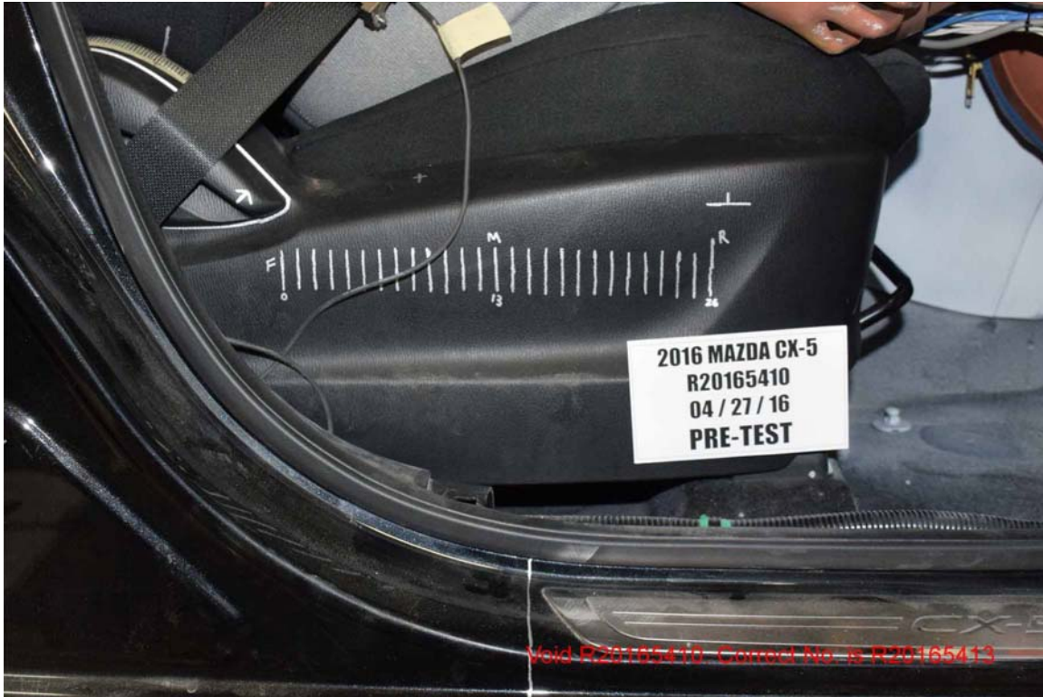
FIGURE 105. Pre-Test Passenger Seat Fore-Aft Markings
