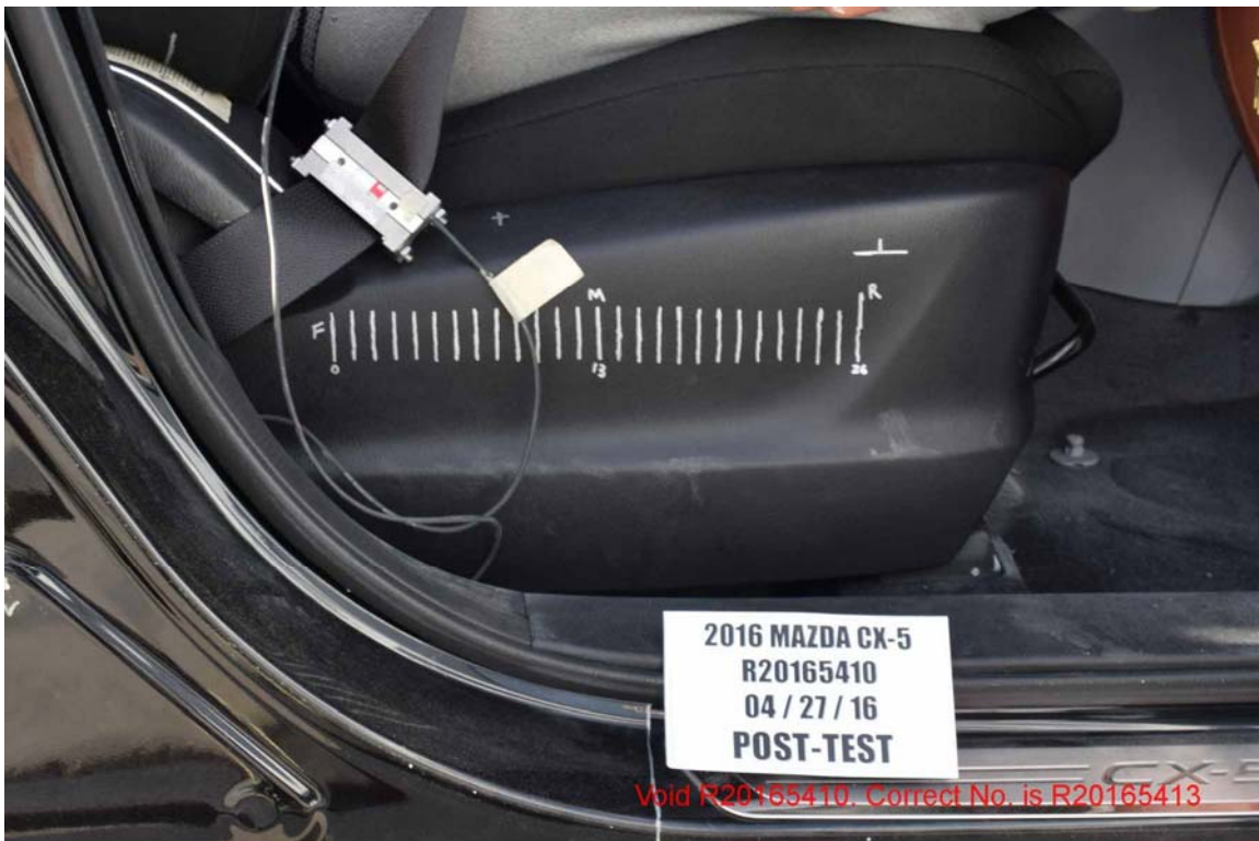
FIGURE 106. Post-Test Passenger Seat Fore-Aft Markings
