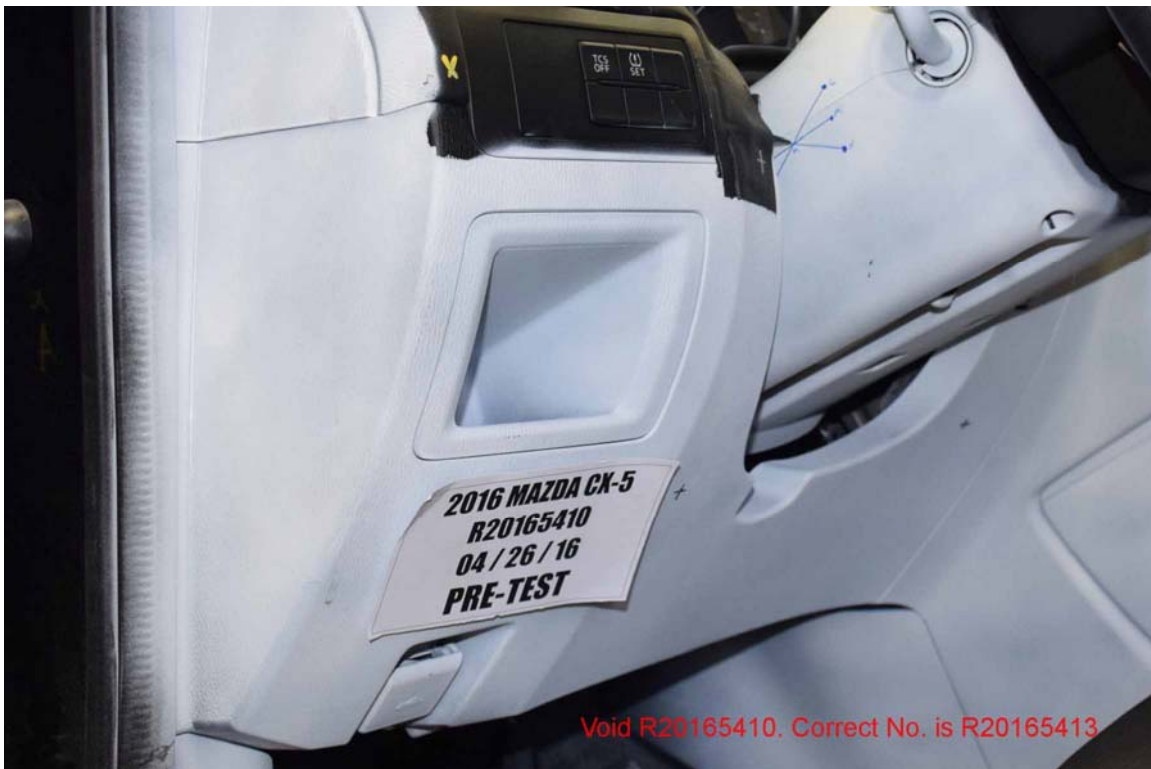
FIGURE 40. Pre-Test Left Side View of Driver Knee Bolster
