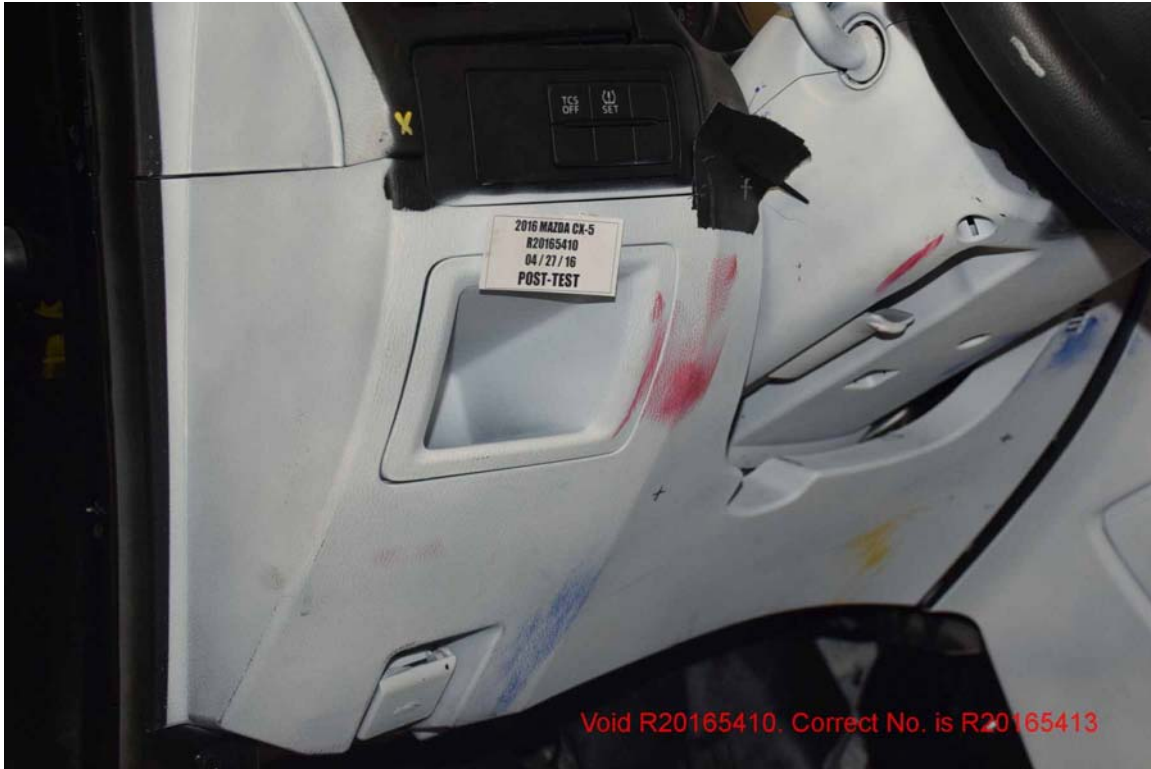
FIGURE 41. Post-Test Left Side View of Driver Knee Bolster
