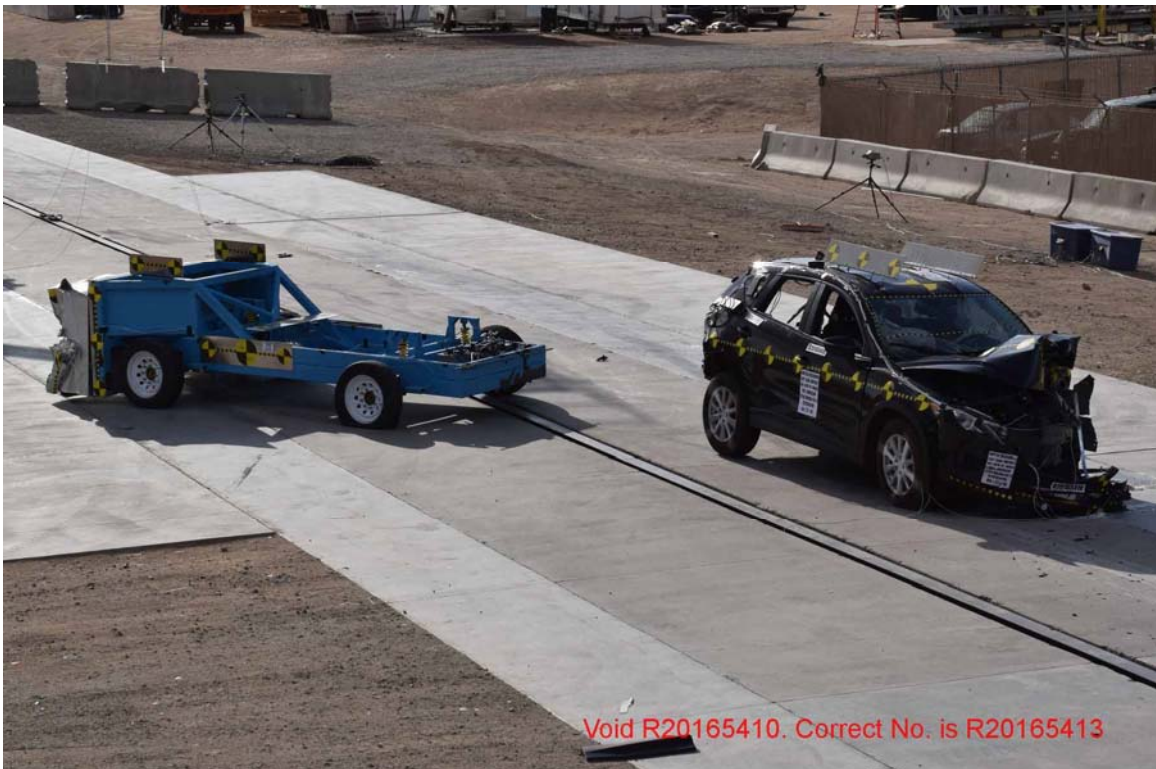
FIGURE 180. Post-Test OMDB & Vehicle, Top View
