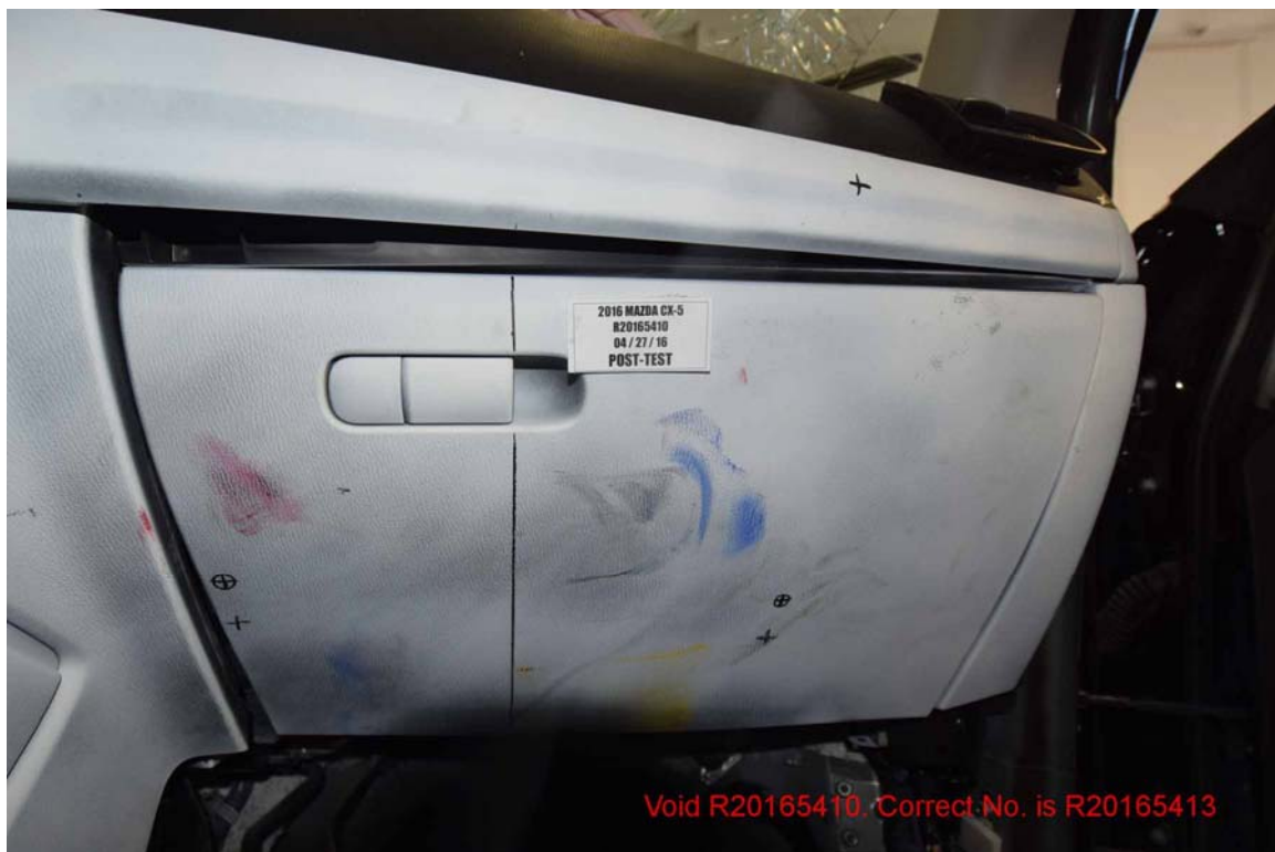
FIGURE 84. Post-Test Overall View of Passenger Knee Bolster
