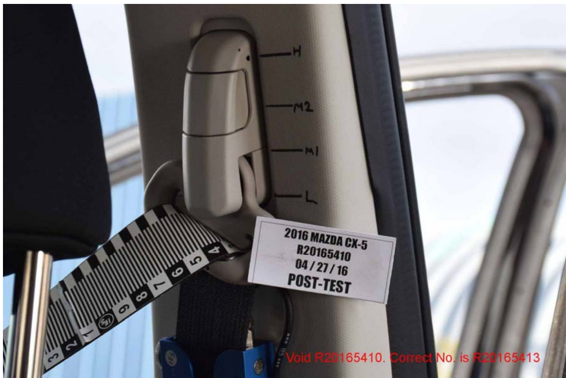
FIGURE 110. Post-Test Passenger Adjustable D-Ring
