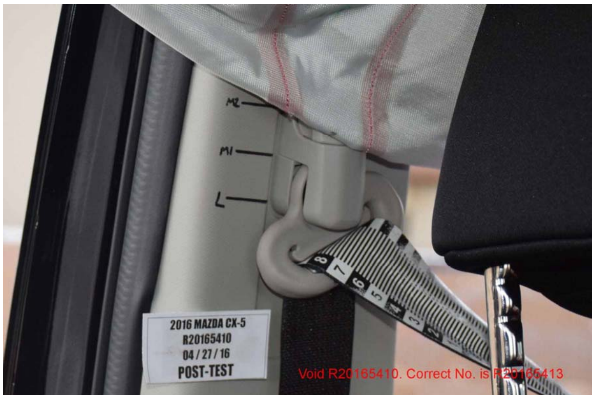
FIGURE 66. Post-Test Driver Adjustable D-Ring
