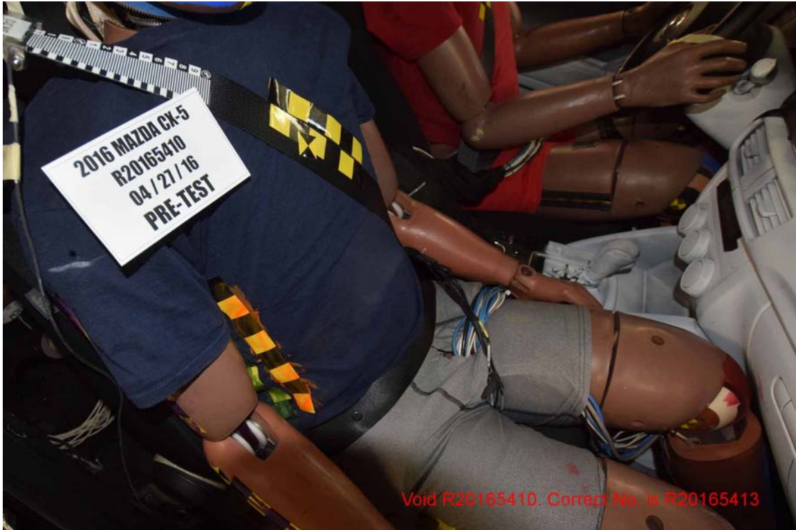
FIGURE 117. Pre-Test View of Passenger Abdomen
