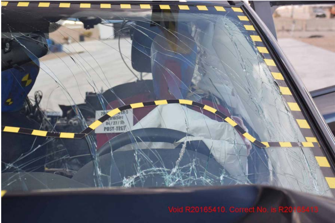
FIGURE 51. Post-Test Driver Front Windshield View
