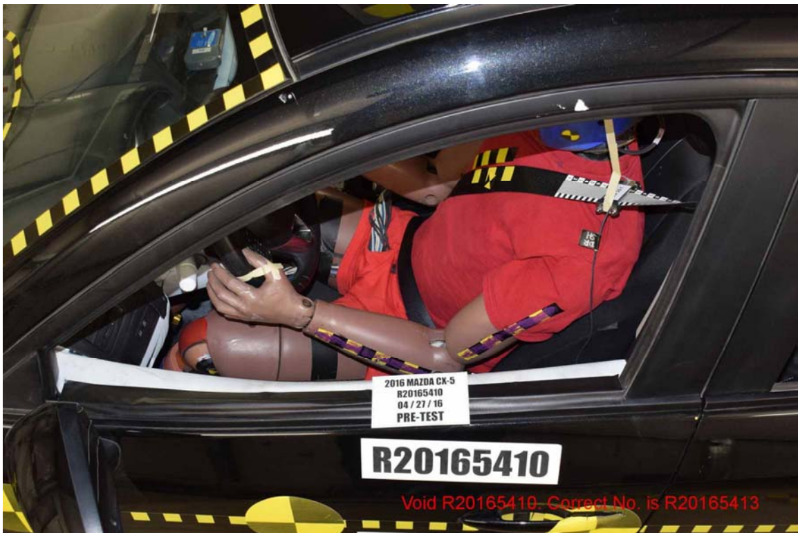
FIGURE 58. Pre-Test View of Driver Door Clearance
