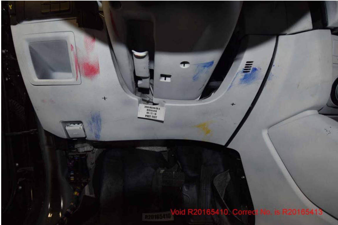
FIGURE 39. Post-Test Overall View of Driver Knee Bolster
