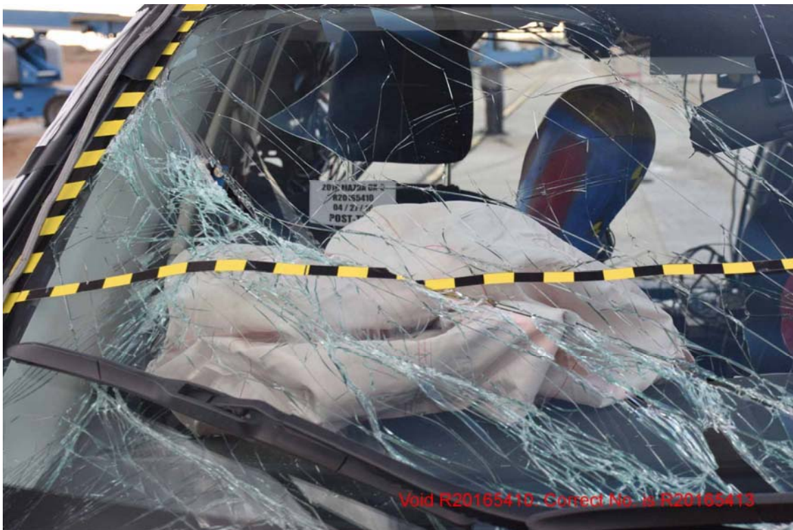
FIGURE 96. Post-Test Passenger Front Windshield View
