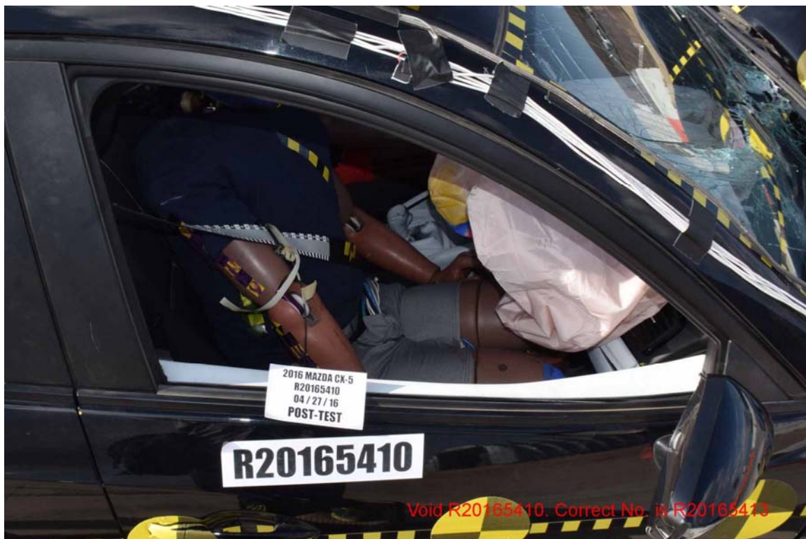
FIGURE 104. Post-Test View of Passenger Door Clearance
