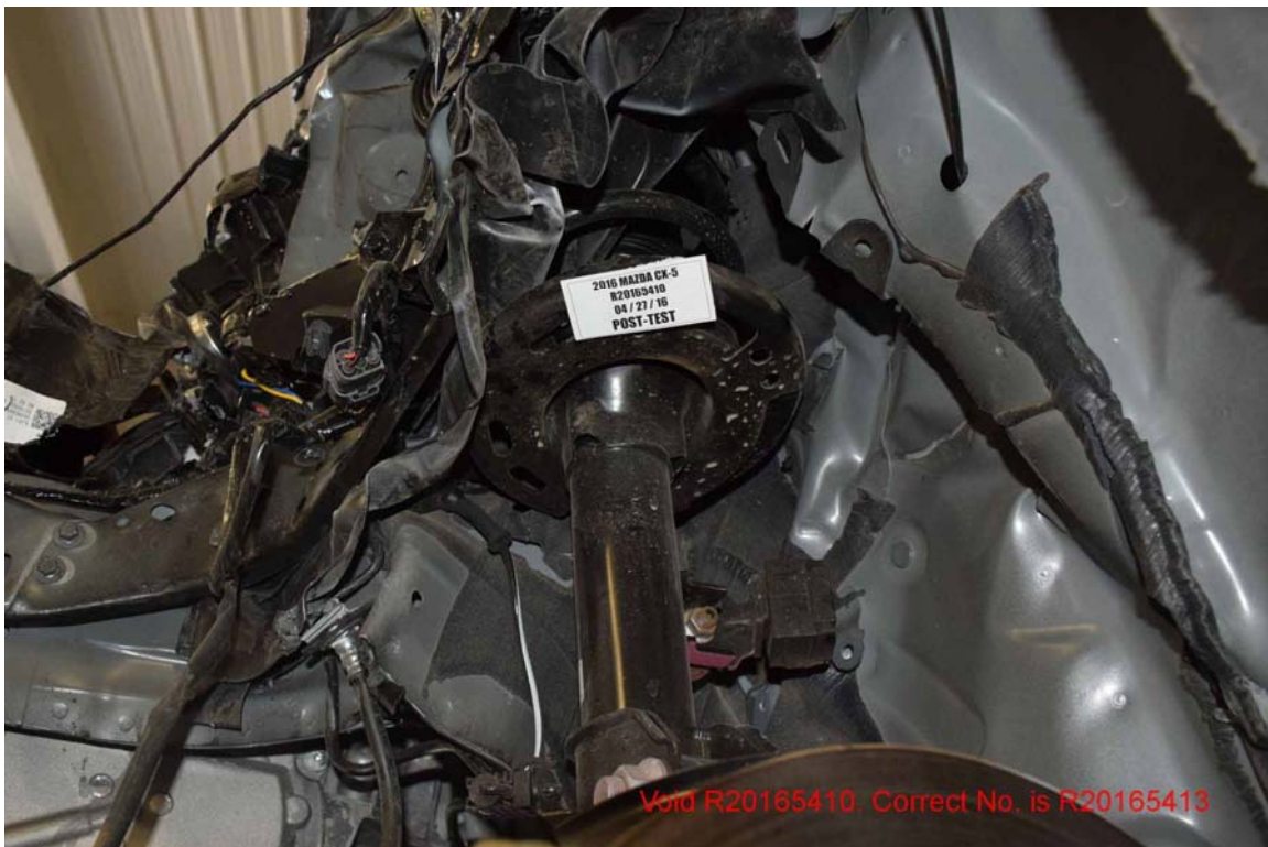
FIGURE 150. Post-Test Driver Close-up View of Suspension
