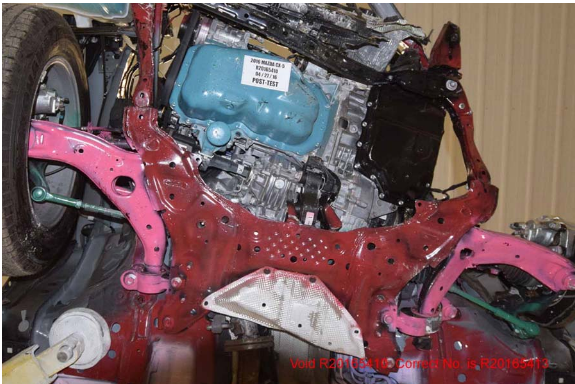
FIGURE 140. Post-Test Bumper to Rail Attachments and Crush Initiators
