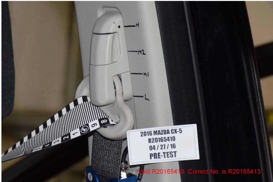
FIGURE 109. Pre-Test Passenger Adjustable D-Ring
