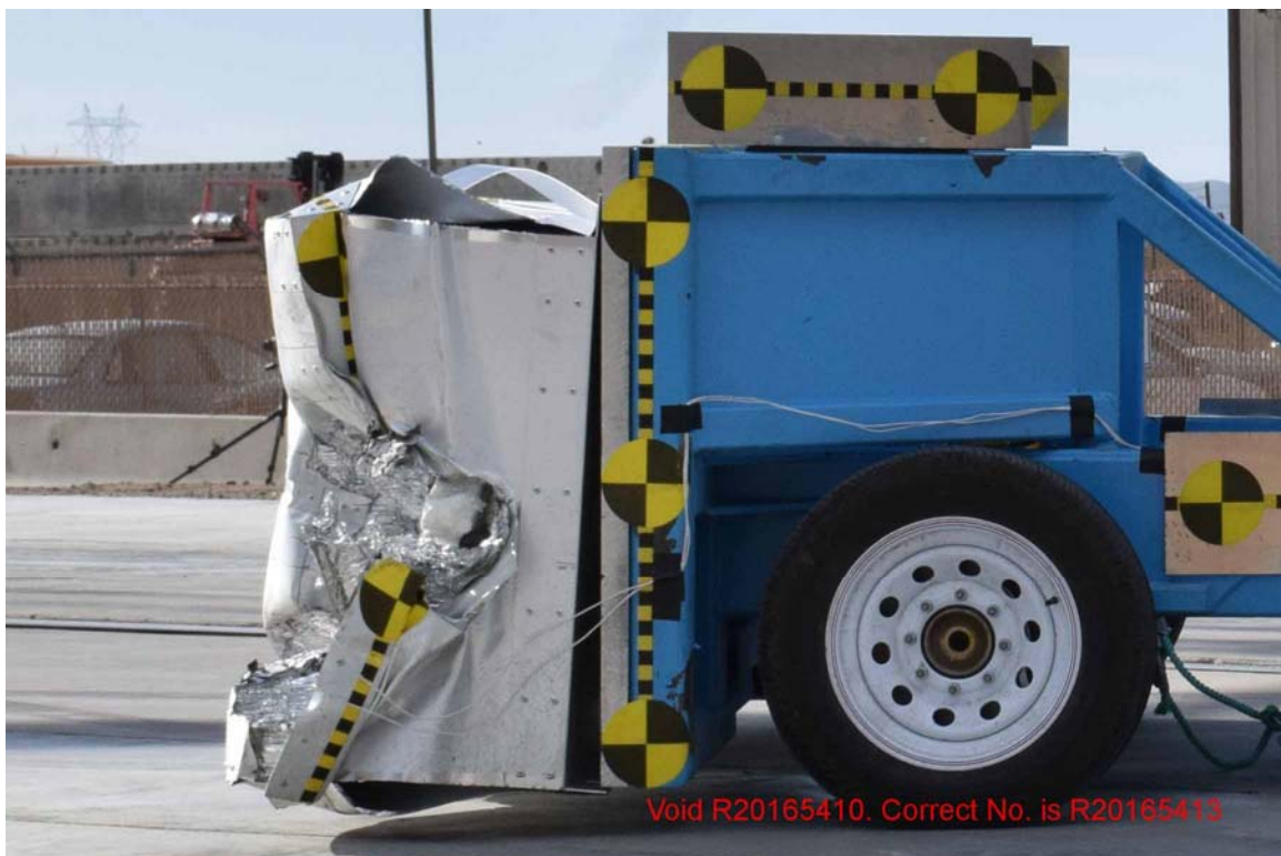
FIGURE 164. Post-Test Left Side View of OMDB Impactor Face
