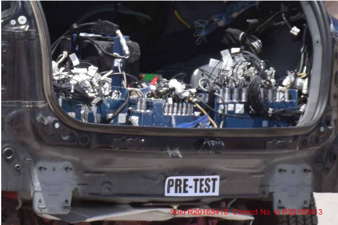
FIGURE 125. Pre-Test Ballast Locations
