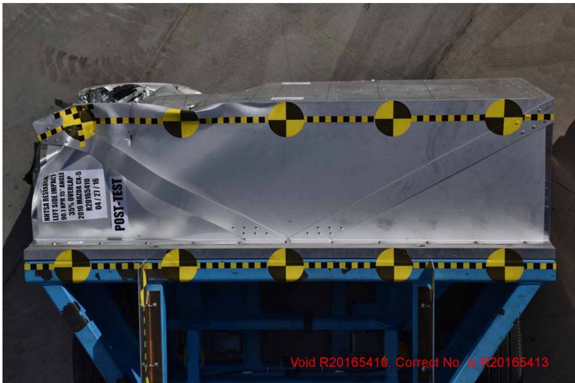
FIGURE 168. Post-Test Top View of OMDB Impactor Face
