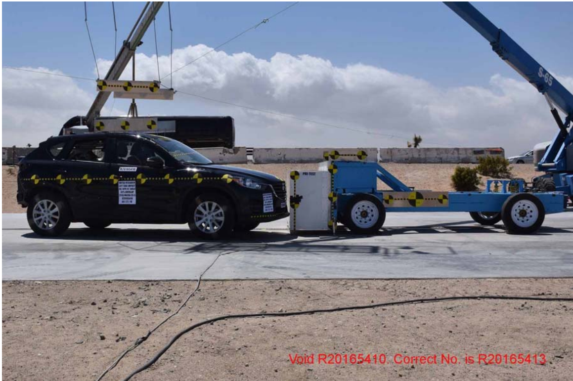
FIGURE 177. Pre-Test OMDB & Vehicle, Left Side
