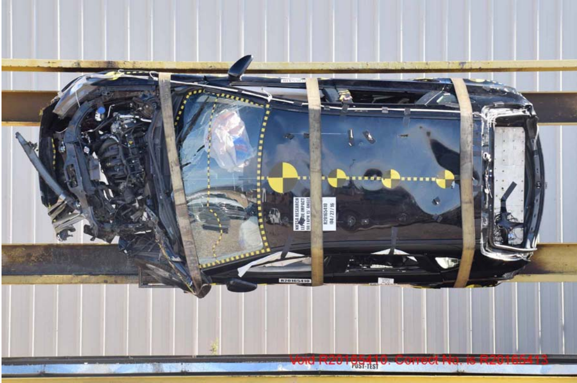
FIGURE 183. FMVSS No. 301 Static Rollover 90 Degrees
