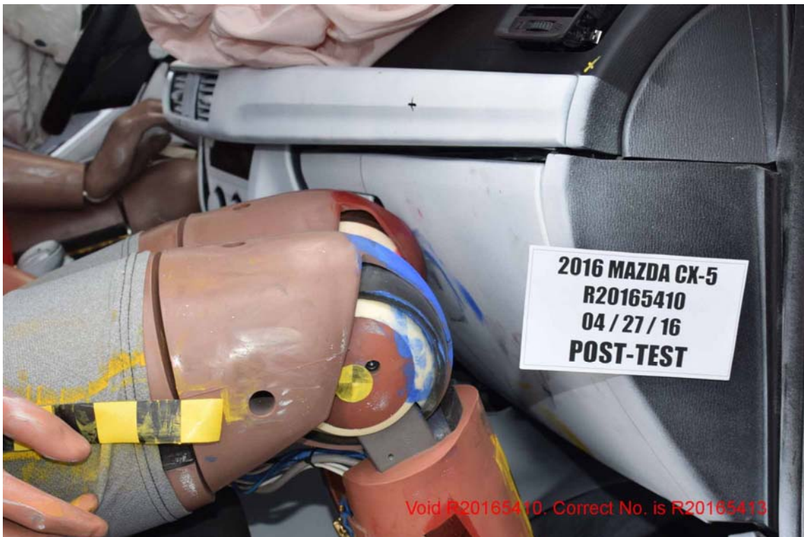
FIGURE 114. Post-Test View of Passenger Right Knee and Bolster
