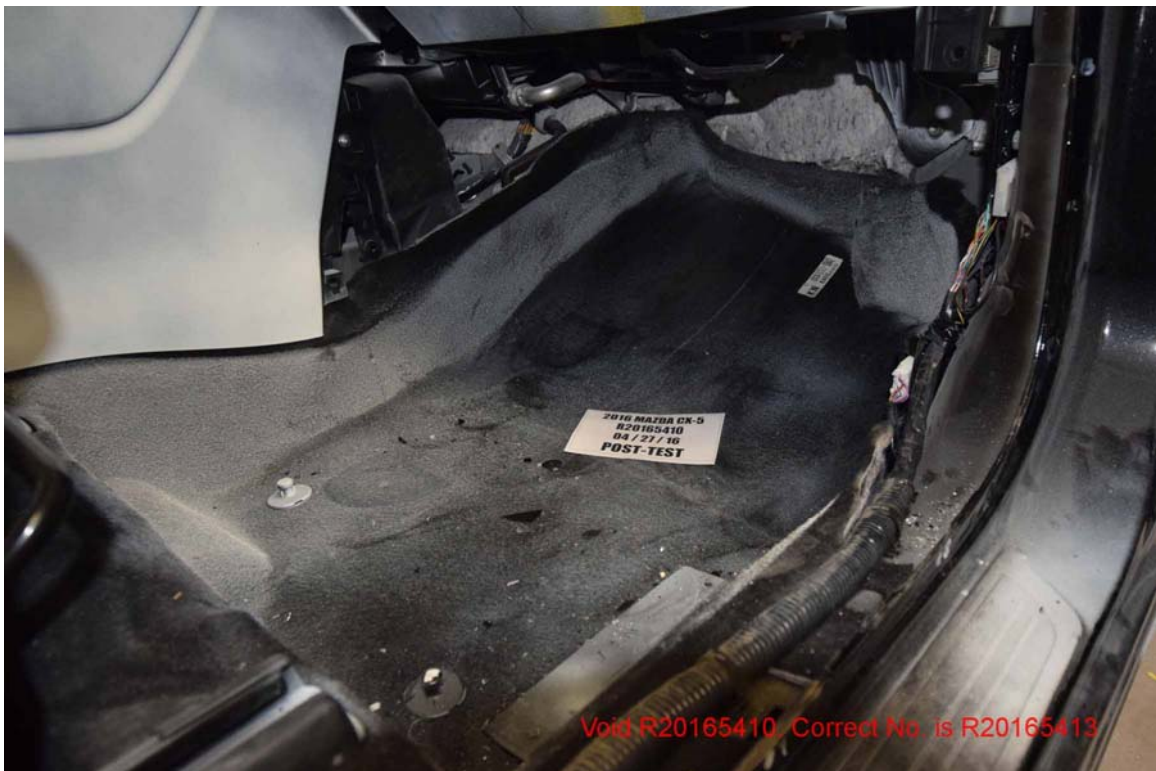
FIGURE 90. Post-Test View of Passenger Floor Pan at Right Sill Level
