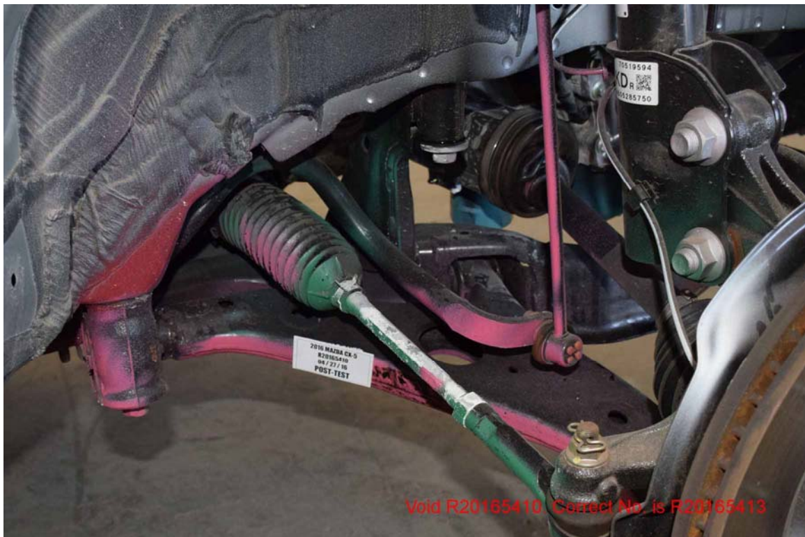
FIGURE 162. Post-Test Right Side Tie Rod and Sway Bar Attachment Points
