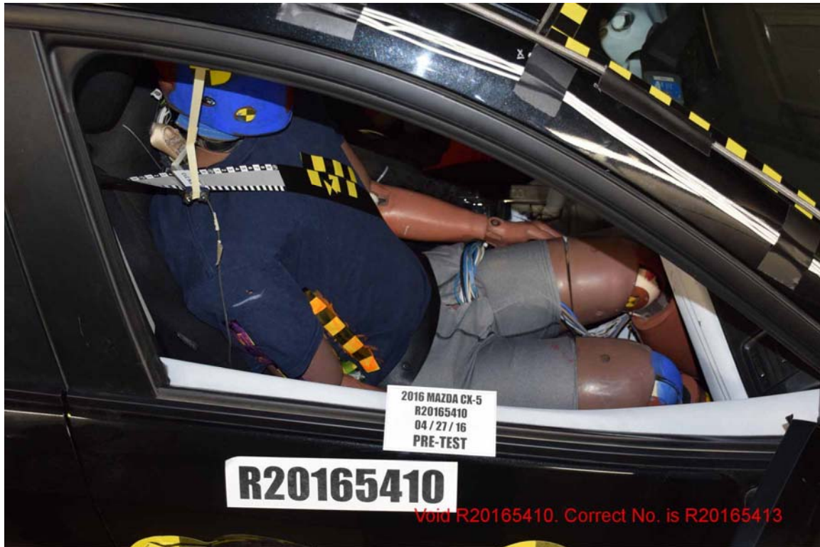
FIGURE 103. Pre-Test View of Passenger Door Clearance
