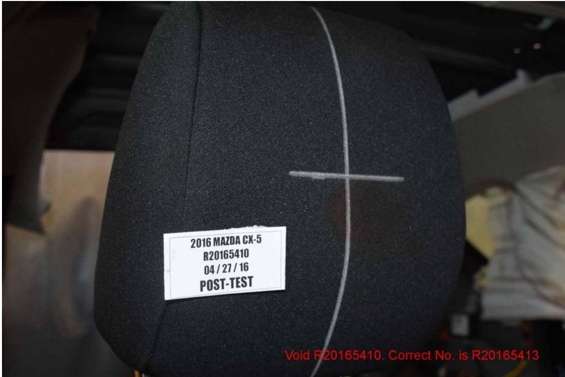
FIGURE 121. Post-Test View of Passenger Head contact with Interior
