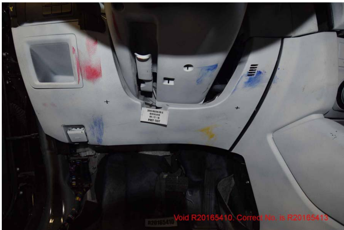
FIGURE 82. Post-Test View of Driver Leg Contact with Vehicle Interior
