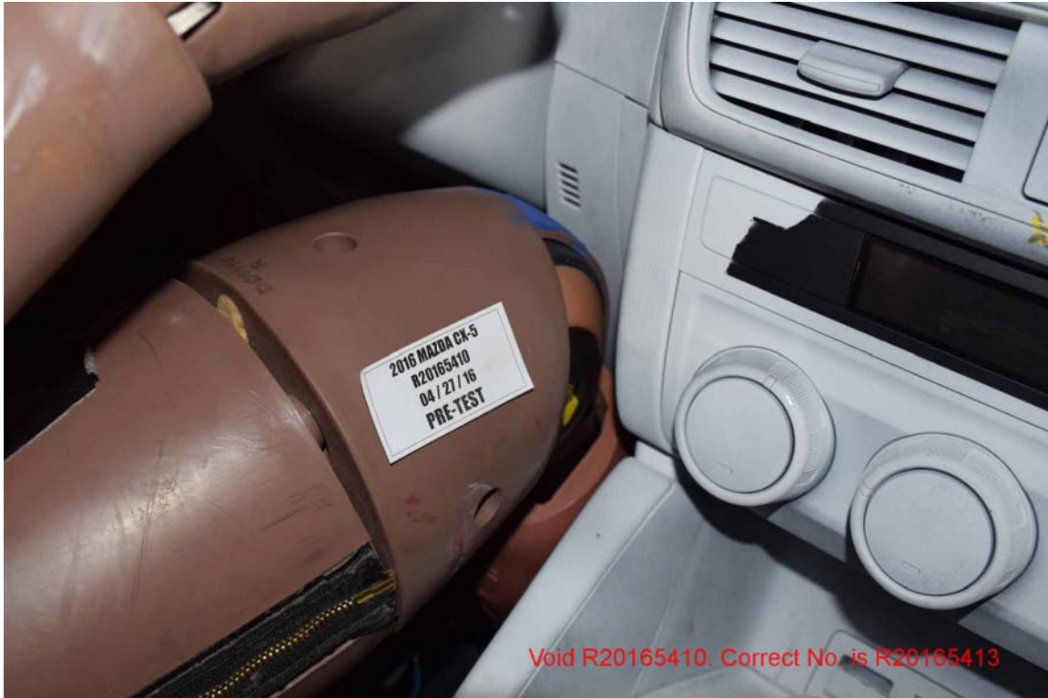
FIGURE 69. Pre-Test View of Driver Right Knee and Bolster
