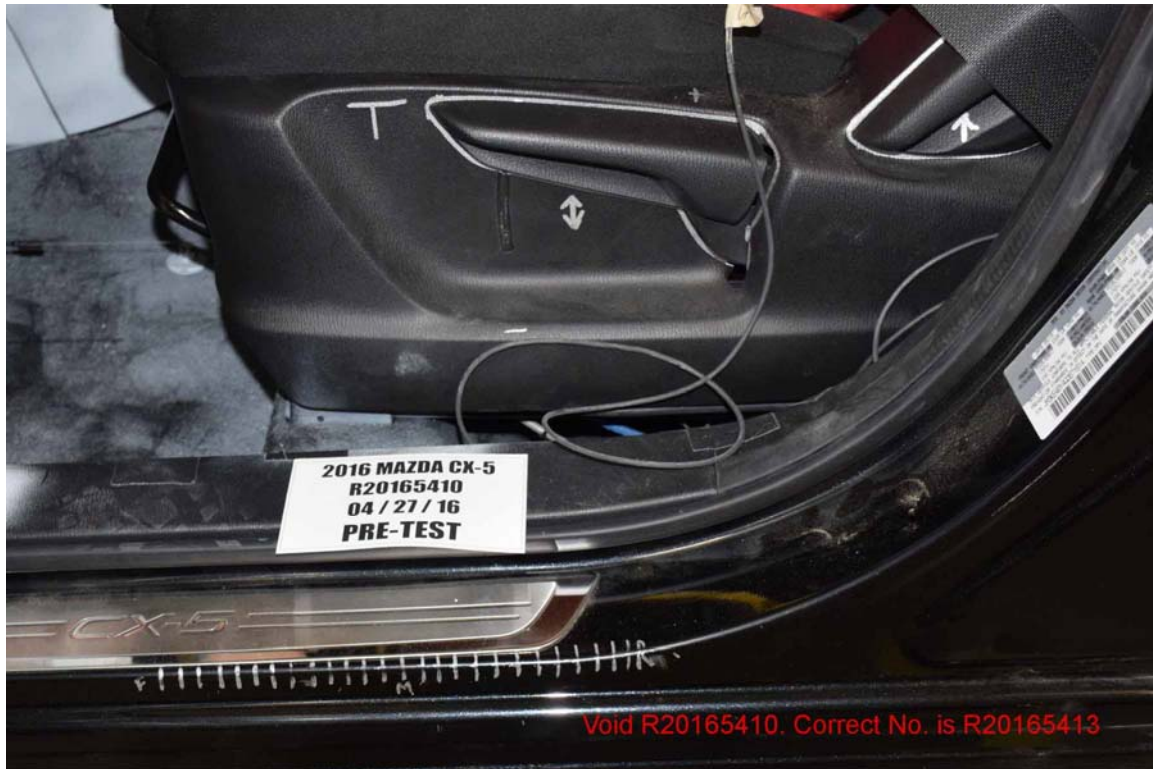
FIGURE 61. Pre-Test Driver Seat Fore Aft Markings
