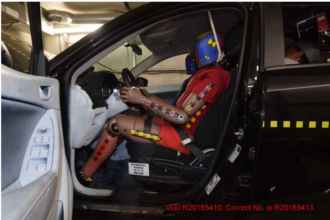
FIGURE 52. Pre-Test Left Side View of Driver and Interior
