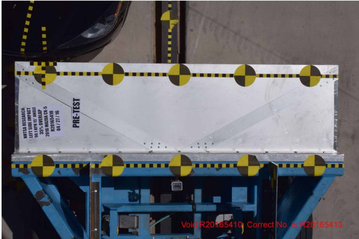
FIGURE 167. Pre-Test Top View of OMDB Impactor Face
