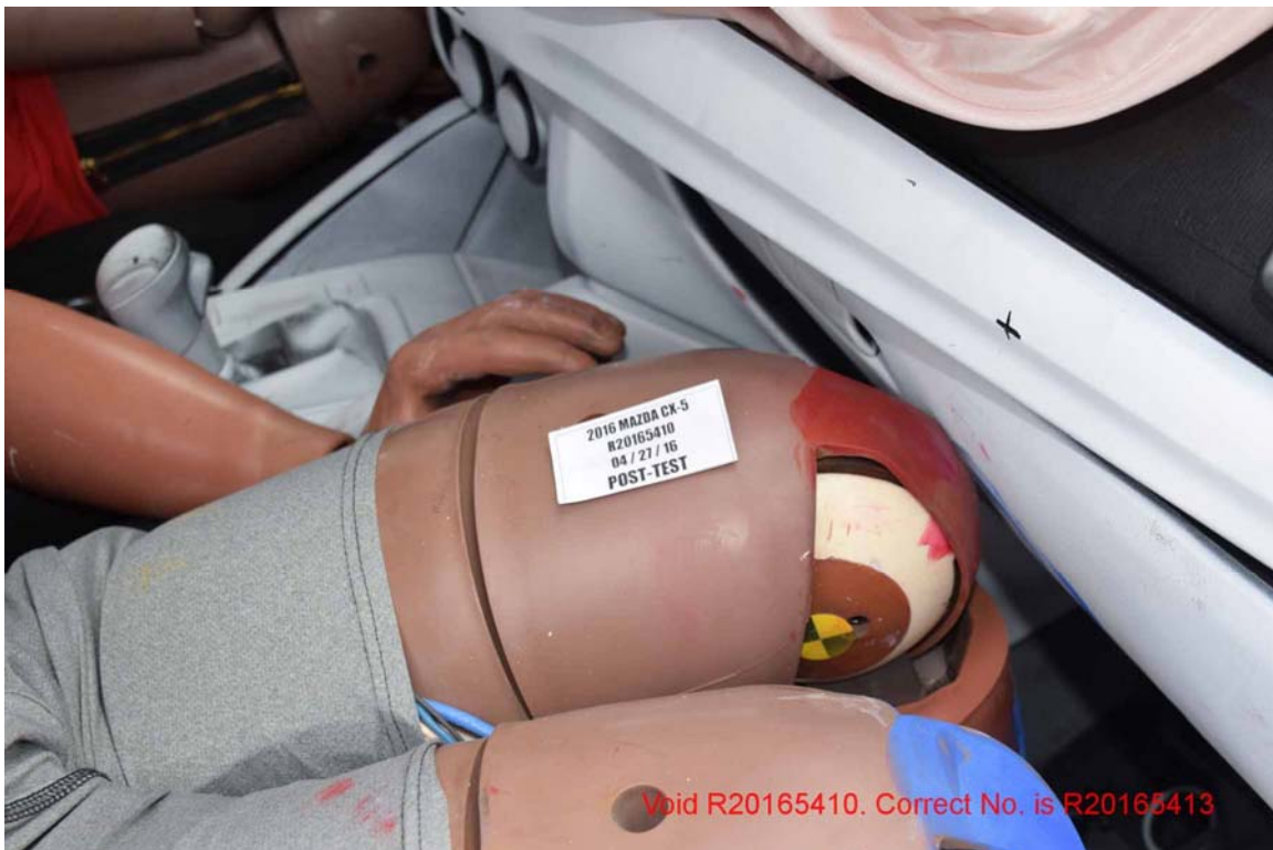
FIGURE 116. Post-Test View of Passenger Left Knee and Bolster
