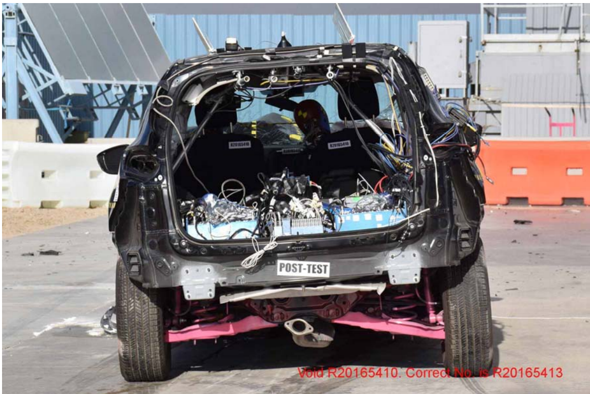
FIGURE 14. Post-Test Rear View of Test Vehicle
