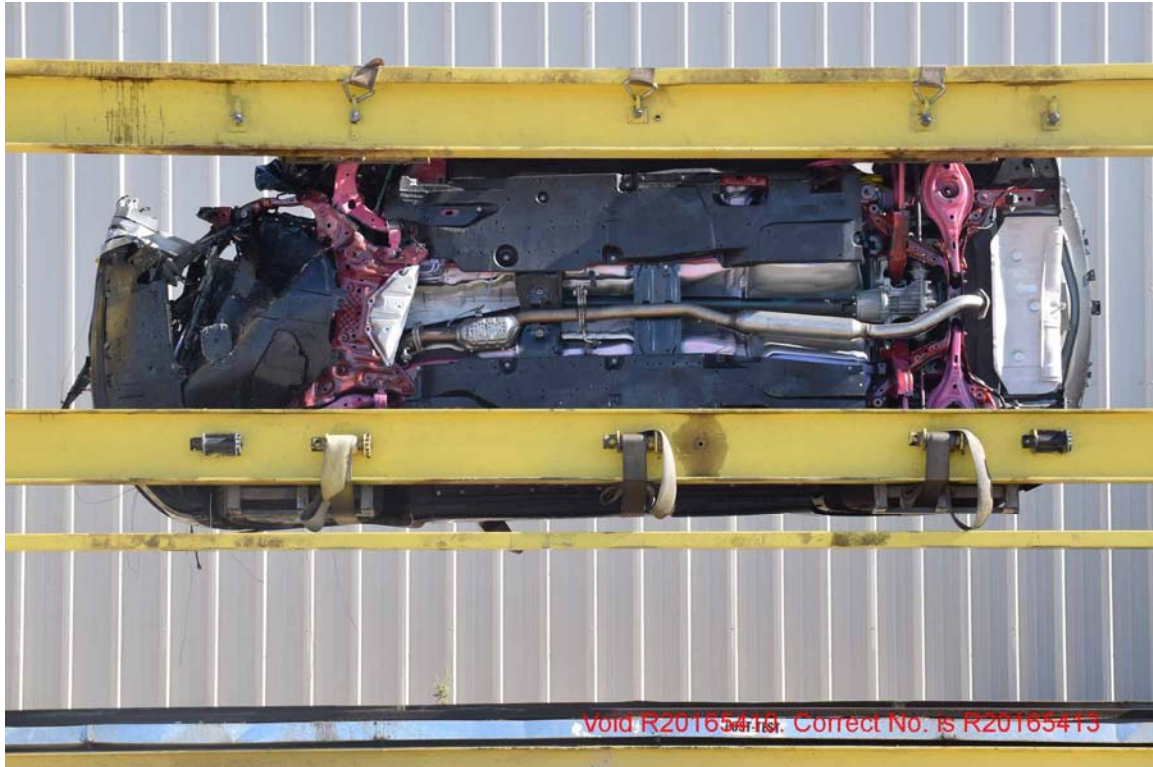
FIGURE 185. FMVSS No. 301 Static Rollover 270 Degrees
