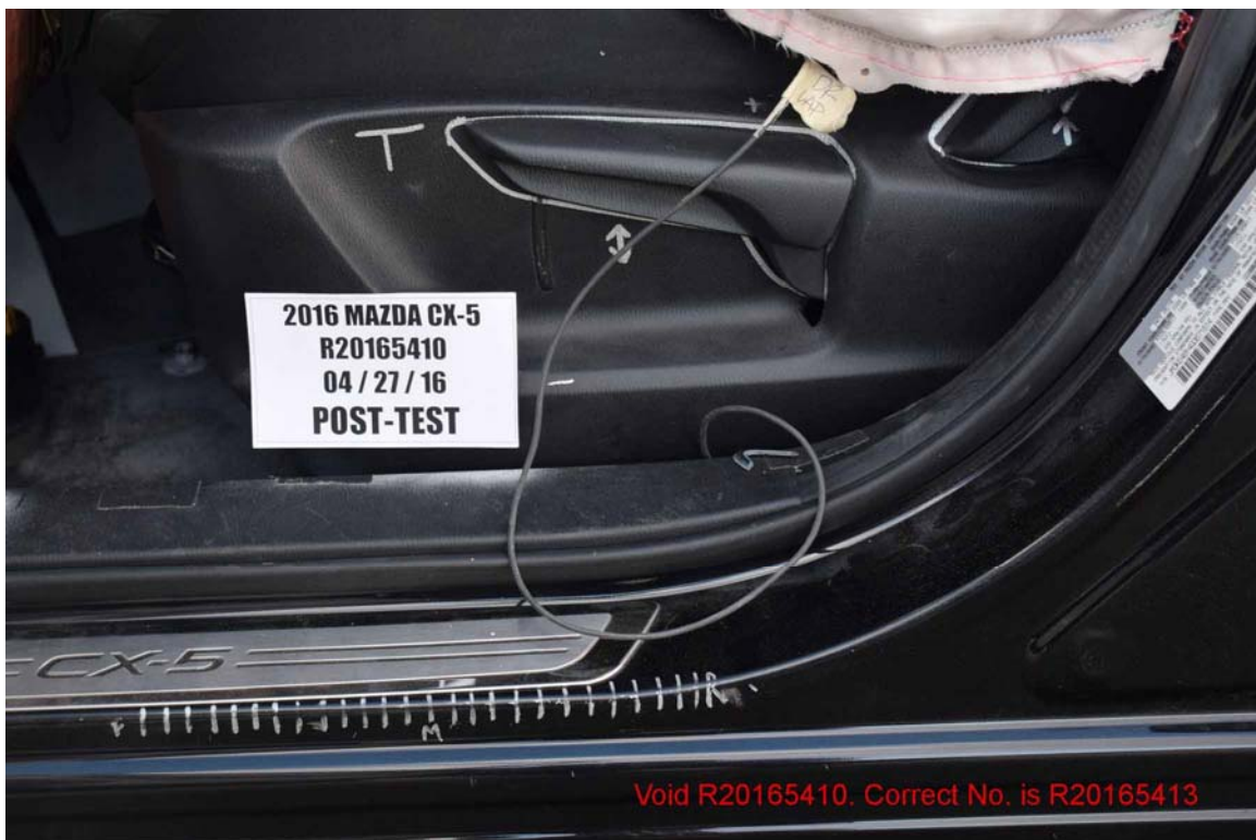
FIGURE 62. Post-Test Driver Seat Fore Aft Markings
