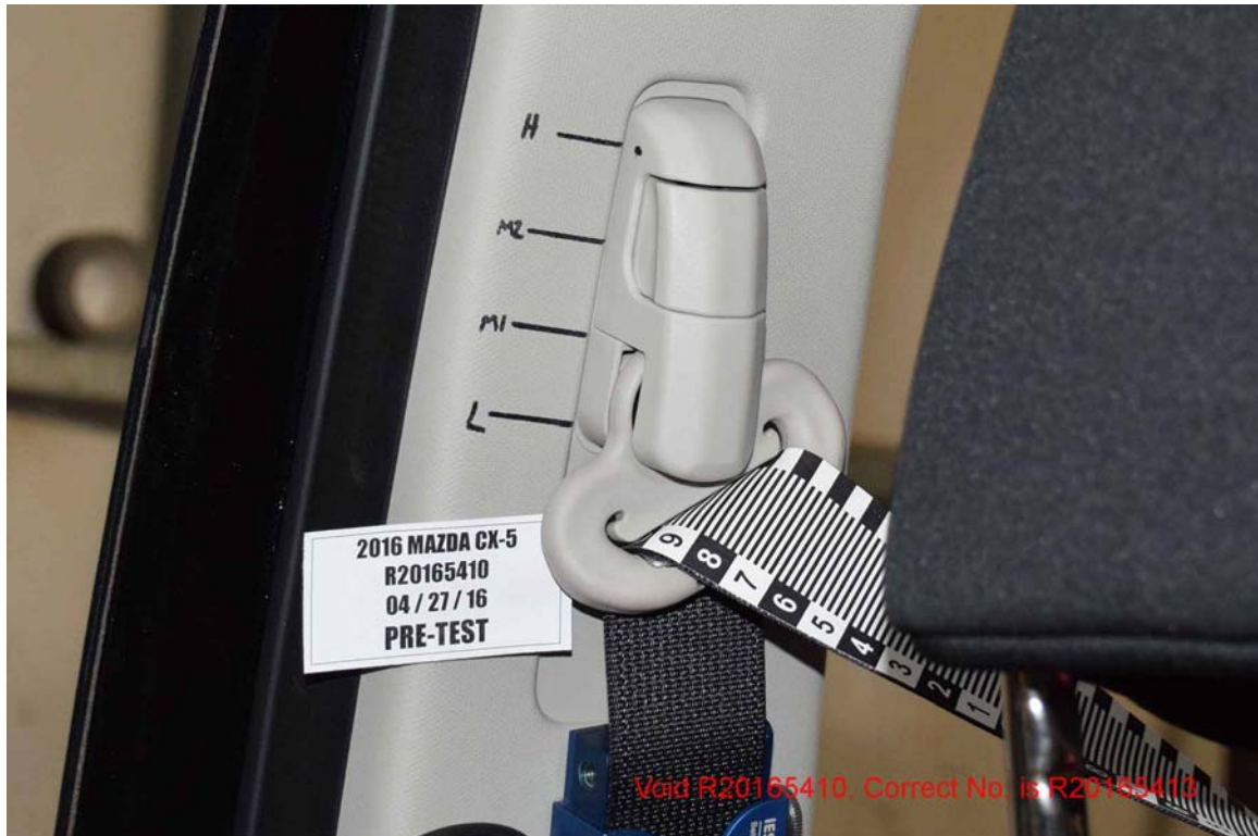
FIGURE 65. Pre-Test Driver Adjustable D-Ring
