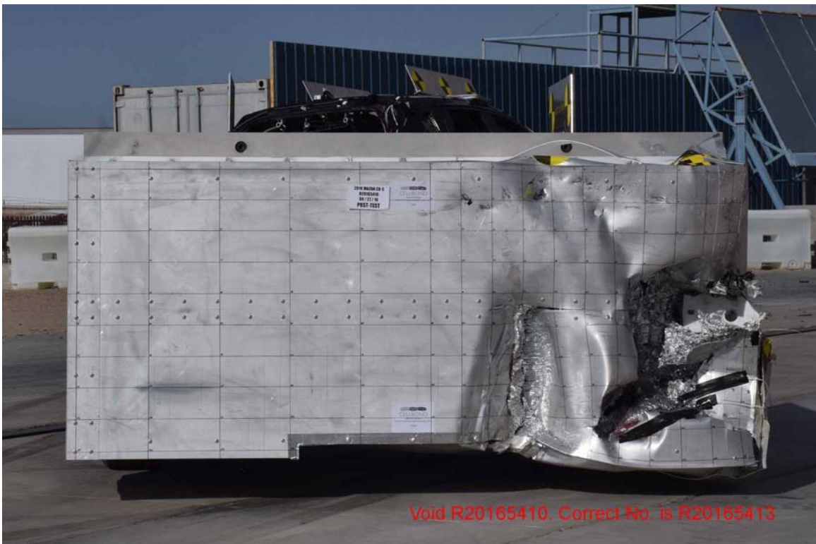
FIGURE 170. Post-Test Front View of OMDB Impactor Face
