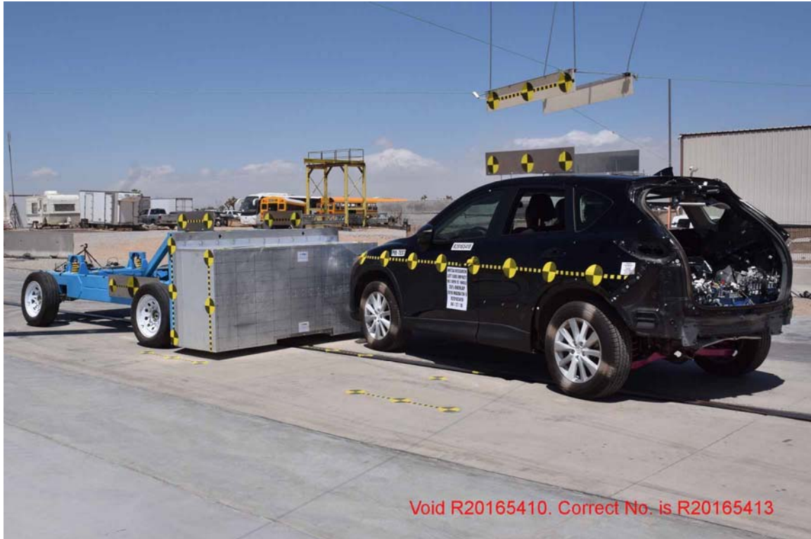
FIGURE 181. Pre-Test OMDB & Vehicle Alignment
