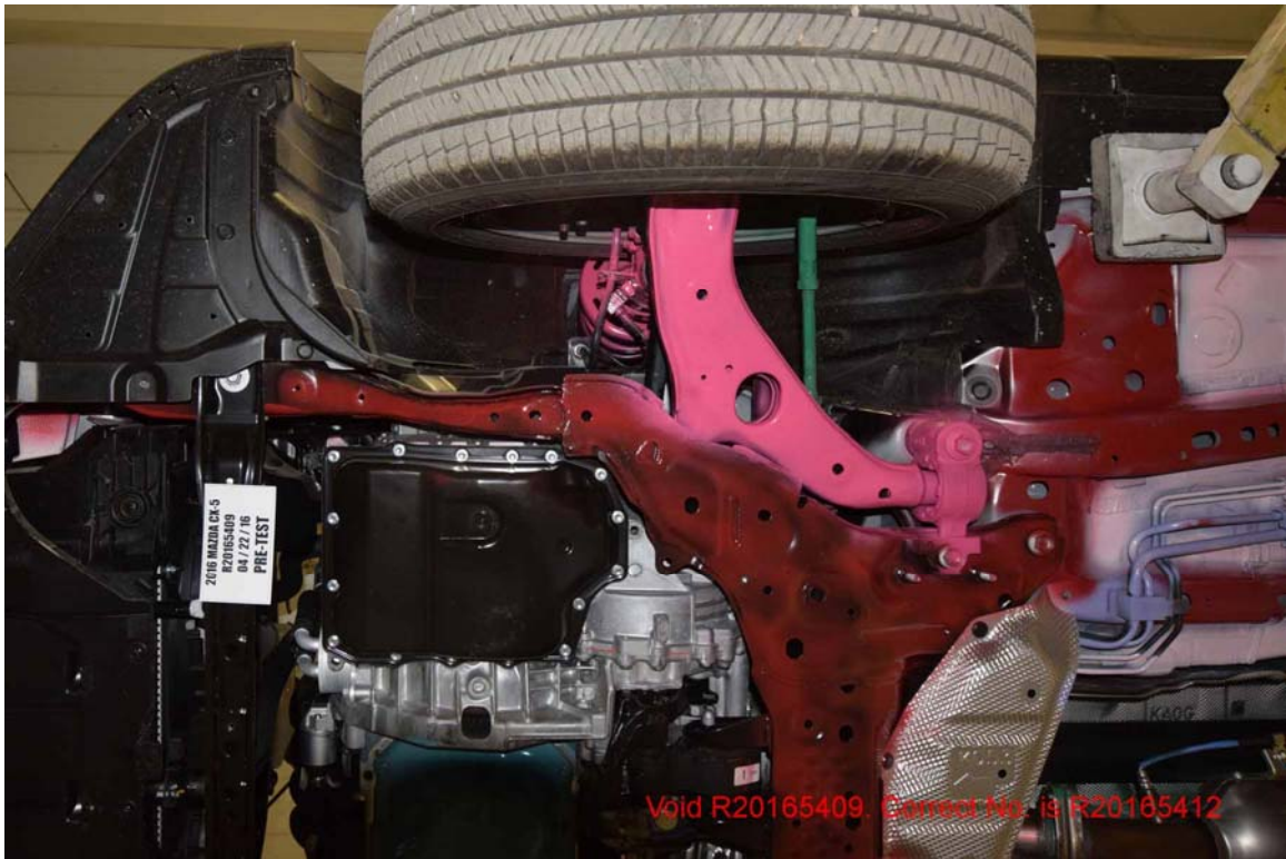
FIGURE 141. Pre-Test Left Side Impact Rail
