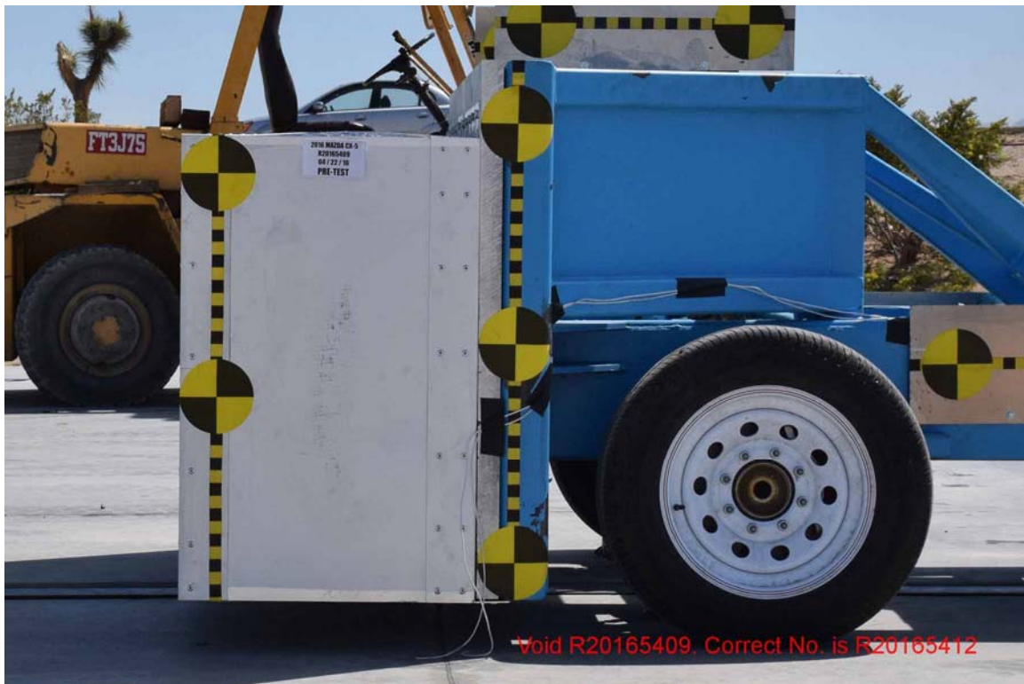
FIGURE 163. Pre-Test Left Side View of OMDB Impactor Face
