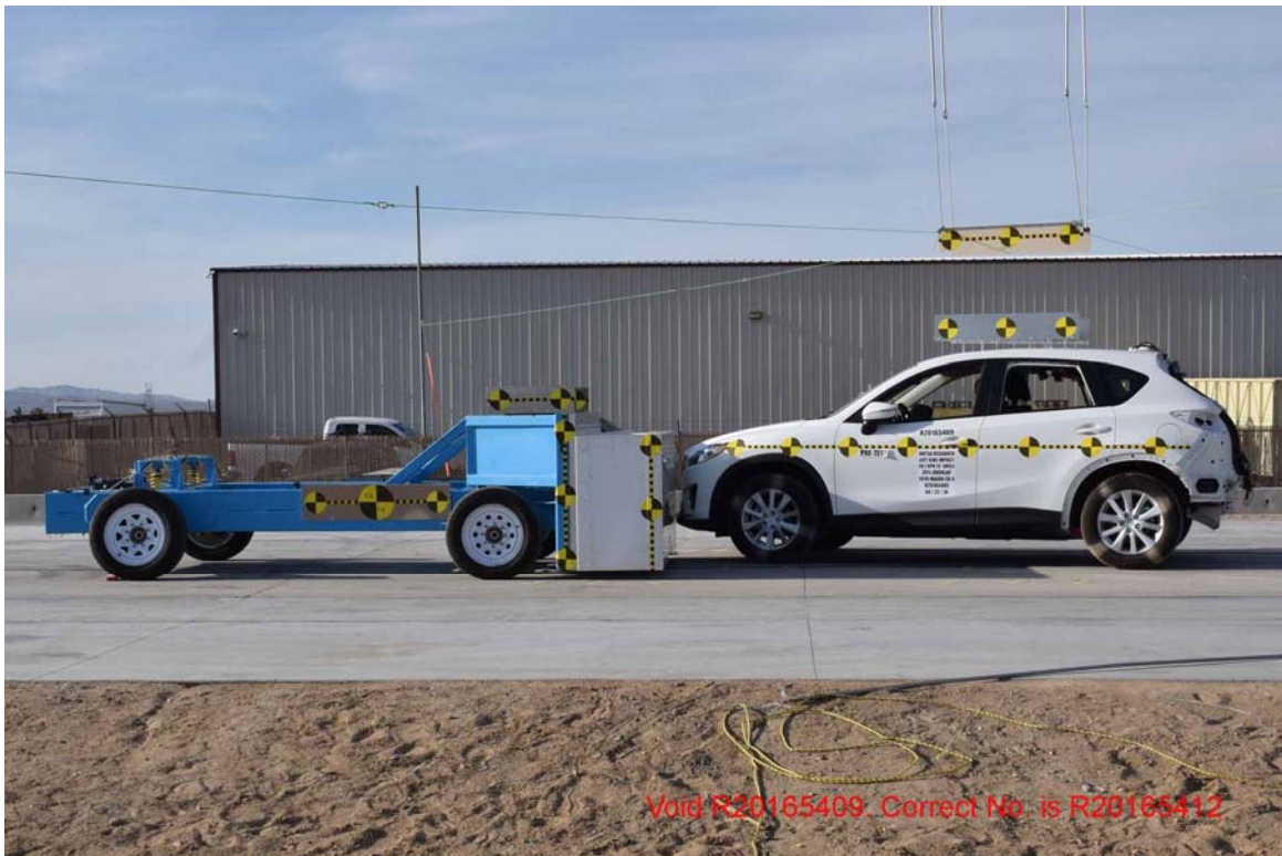
FIGURE 175. Pre-Test OMDB & Vehicle, Right Side
