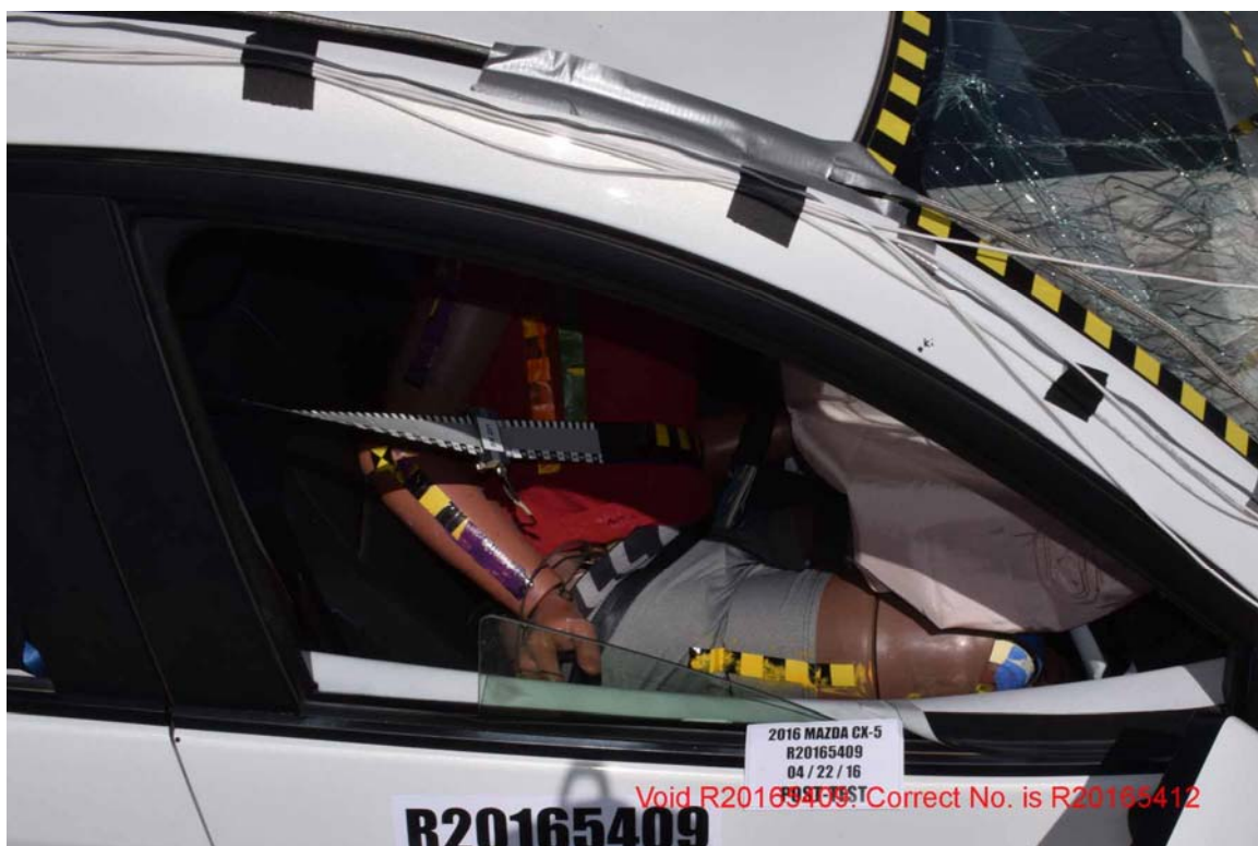
FIGURE 104. Post-Test View of Passenger Door Clearance
