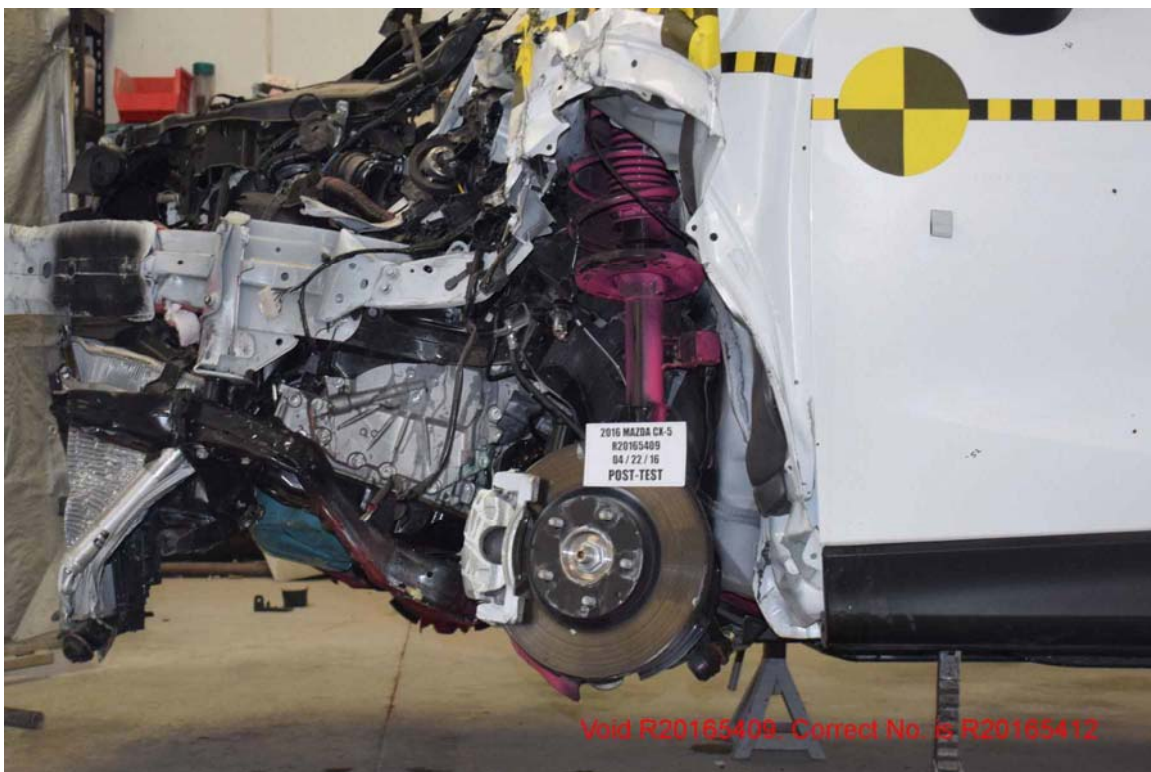
FIGURE 146. Post-Test Left Side View of Driver Wheel Well
