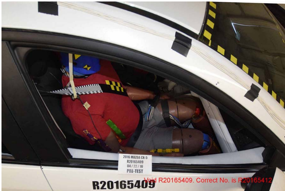
FIGURE 103. Pre-Test View of Passenger Door Clearance
