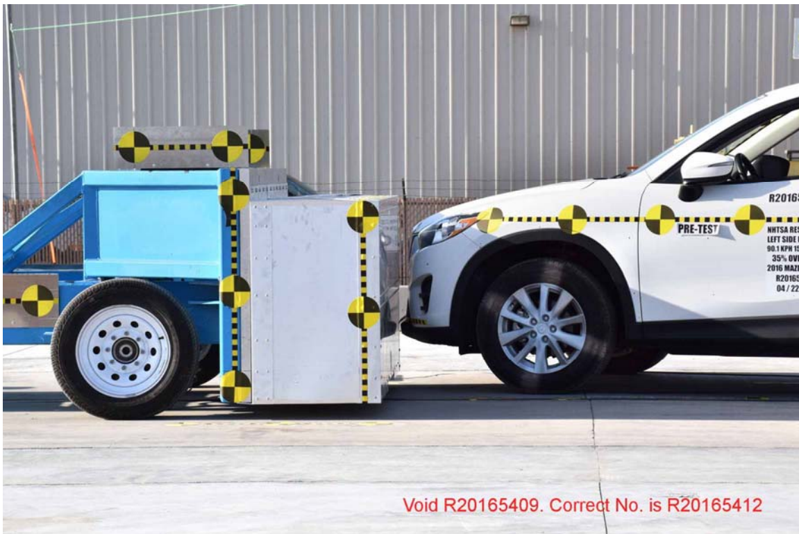
FIGURE 24. Pre-Test Right Side View of OMDB Against Target Vehicle at Ideal Impact Point
