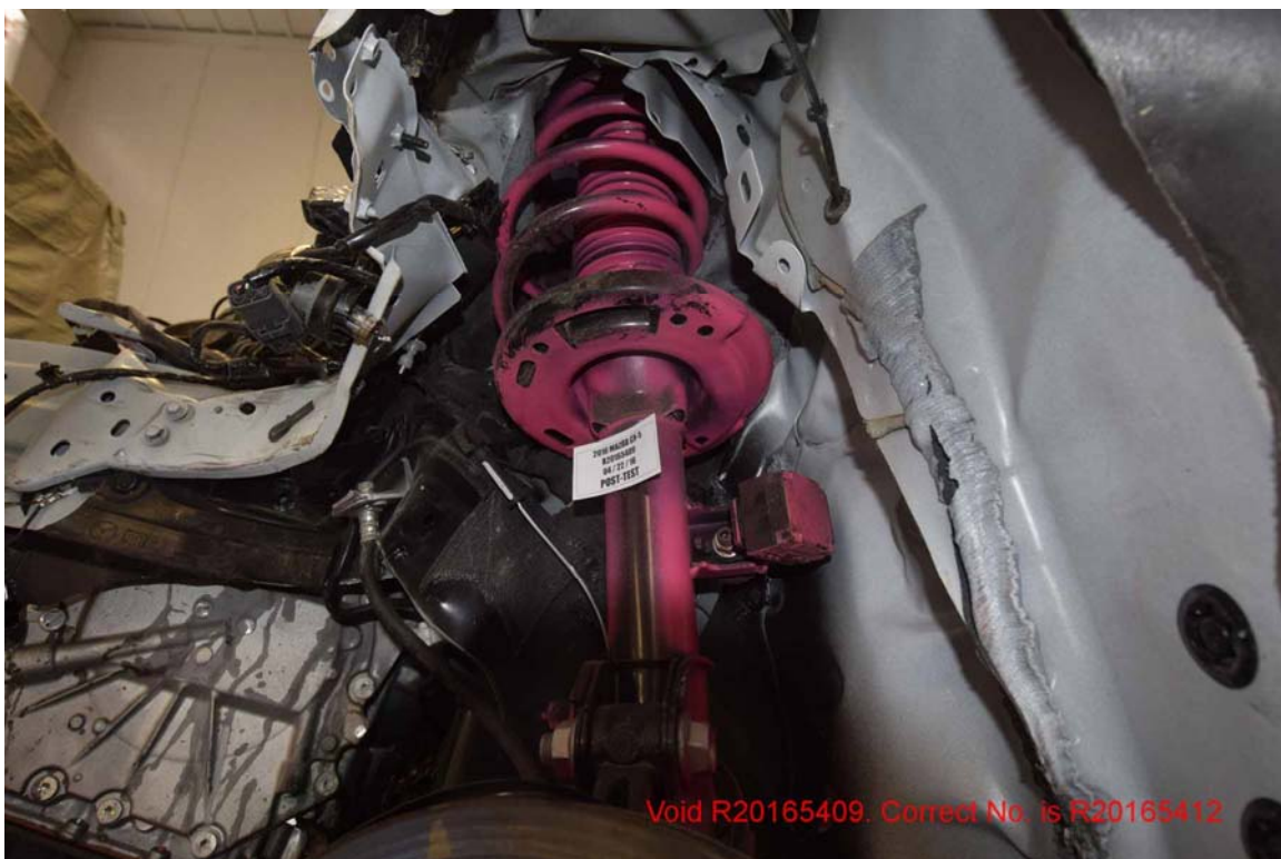
FIGURE 150. Post-Test Driver Close-up View of Suspension
