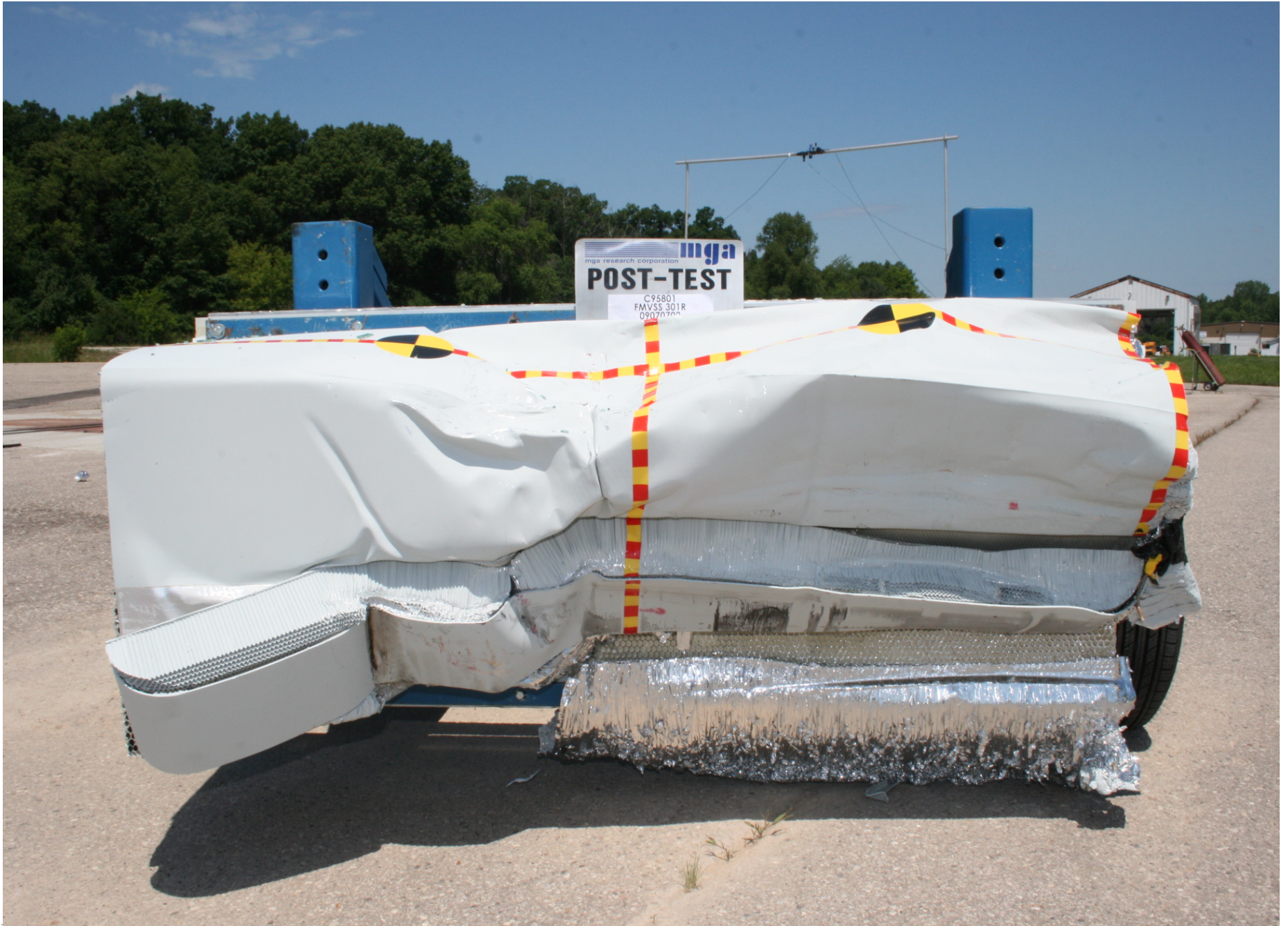
Post-Test Front View of MDB
