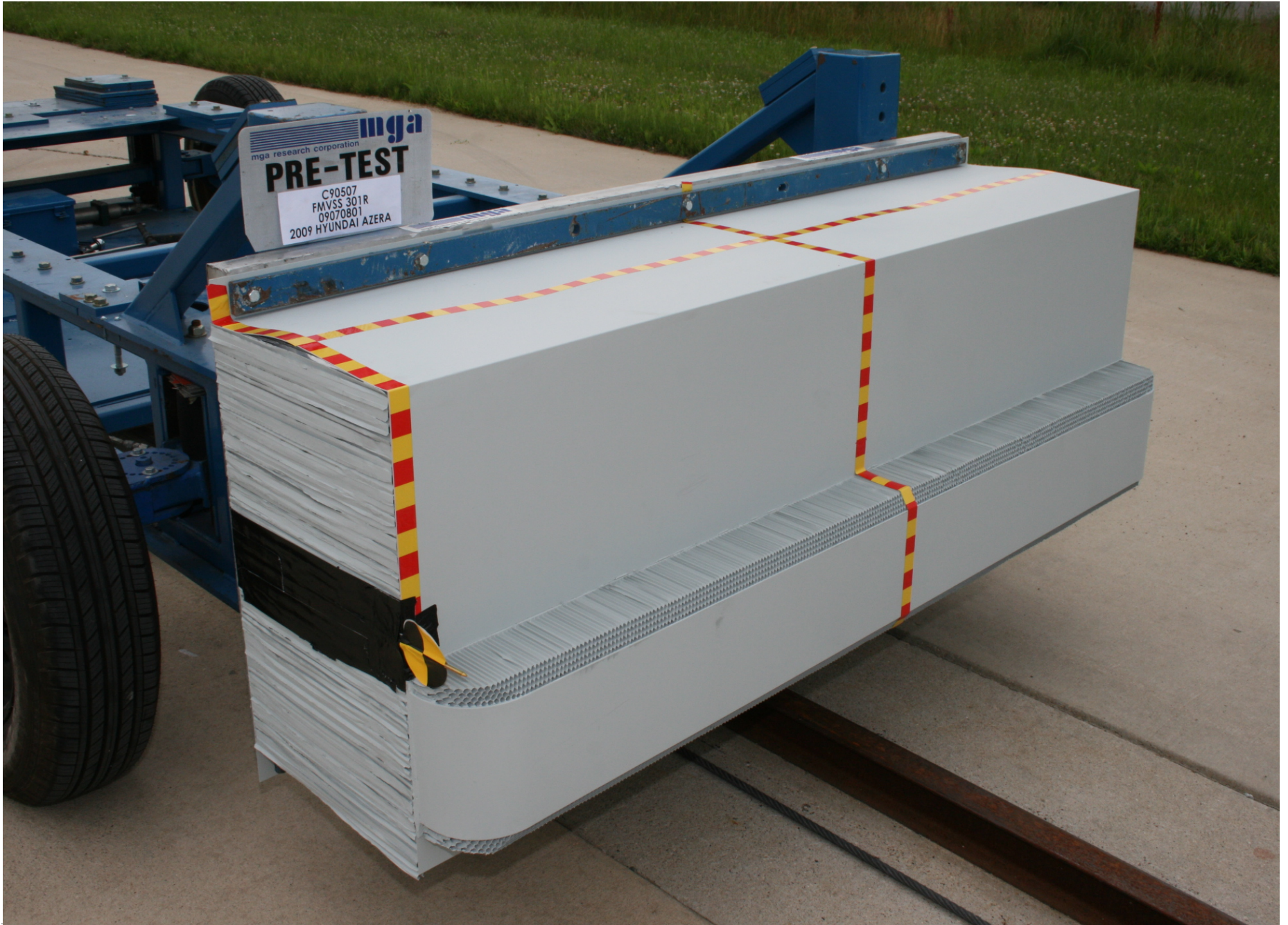
Pre-Test \frac{3}{4} Right Side View of MDB
