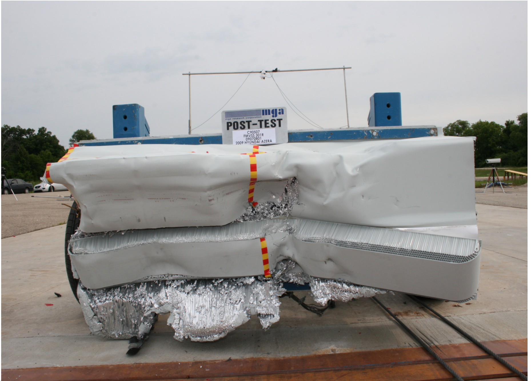
Post-Test Front View of MDB
