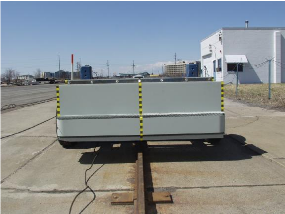
Figure A-19: Pre-Test MDB Front View
