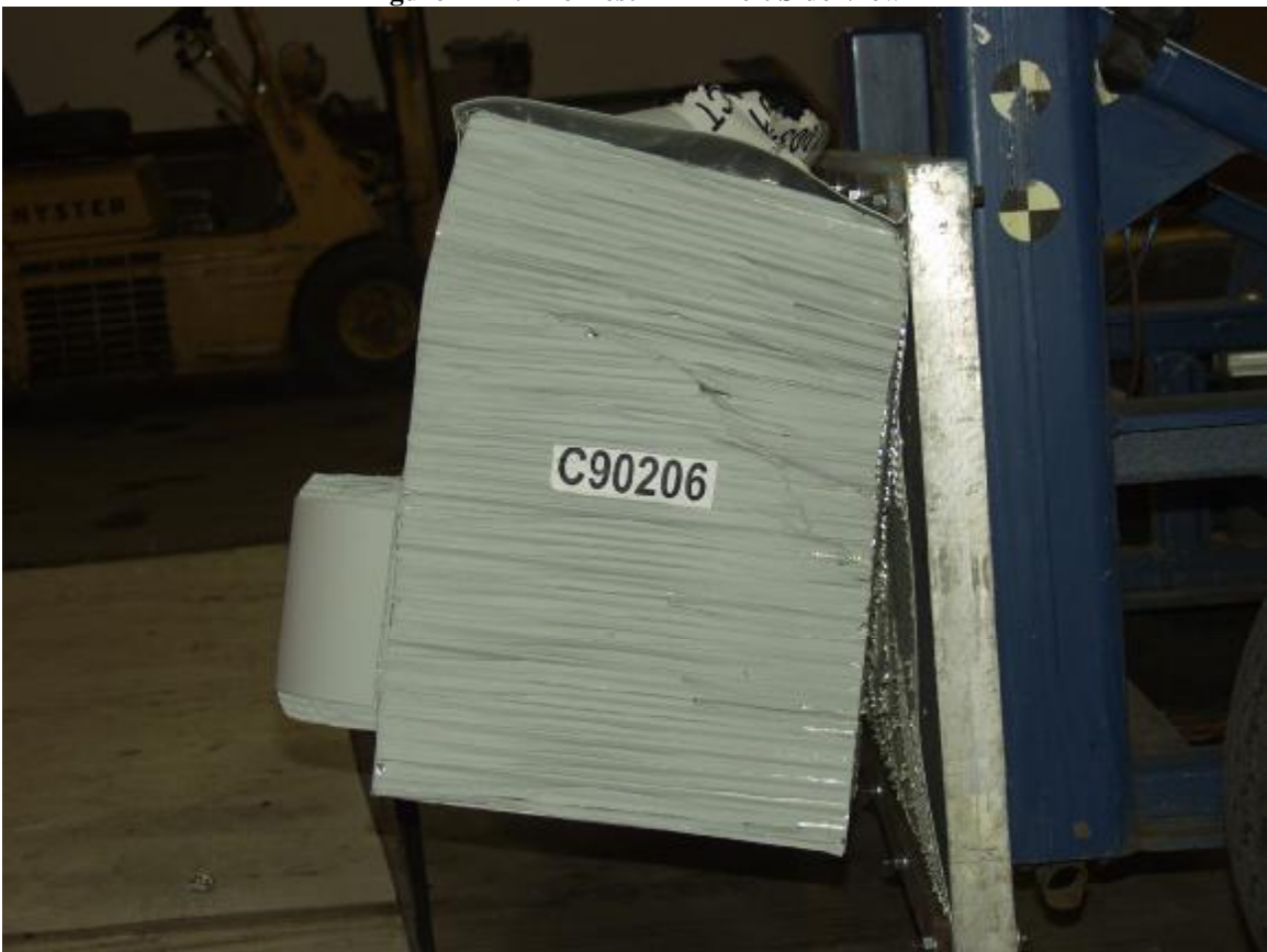
Figure A-22: Post-Test MDB Left Side View
