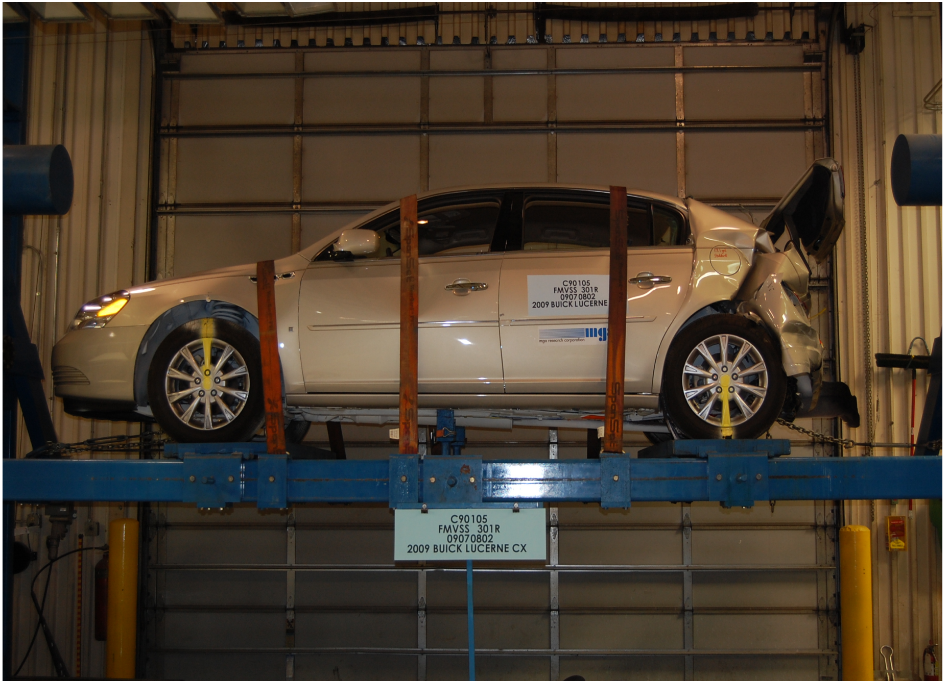
Static Rollover at 360 Degrees
