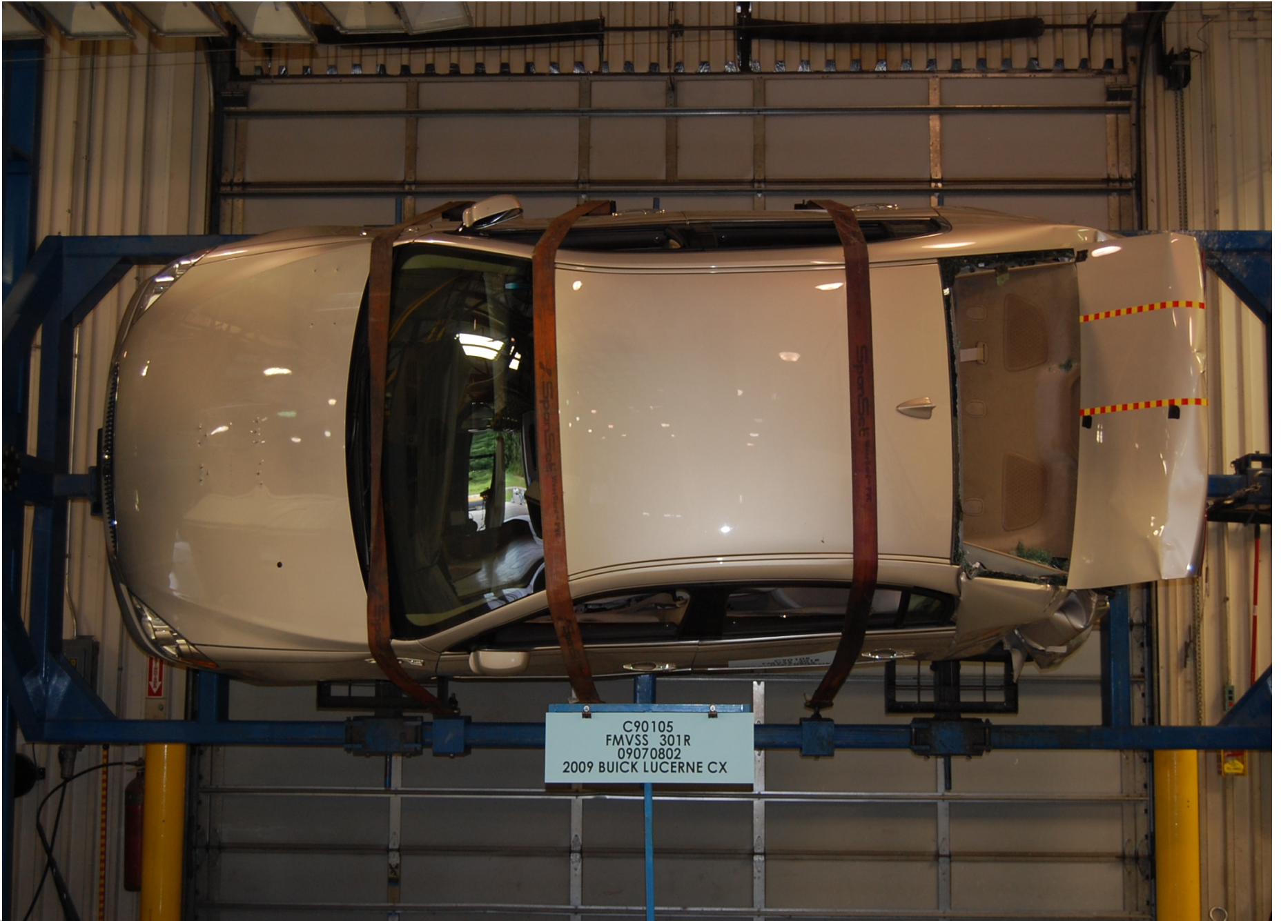
Static Rollover at 90 Degrees
