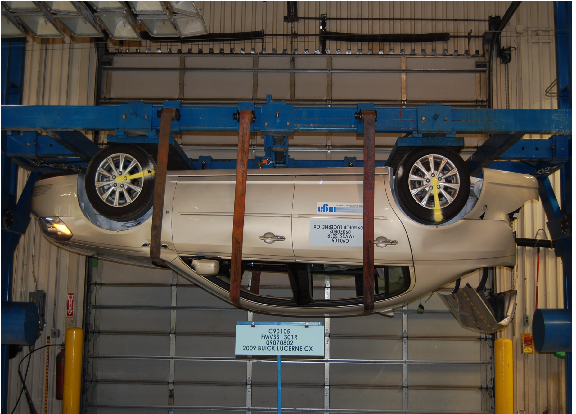
Static Rollover at 180 Degrees
