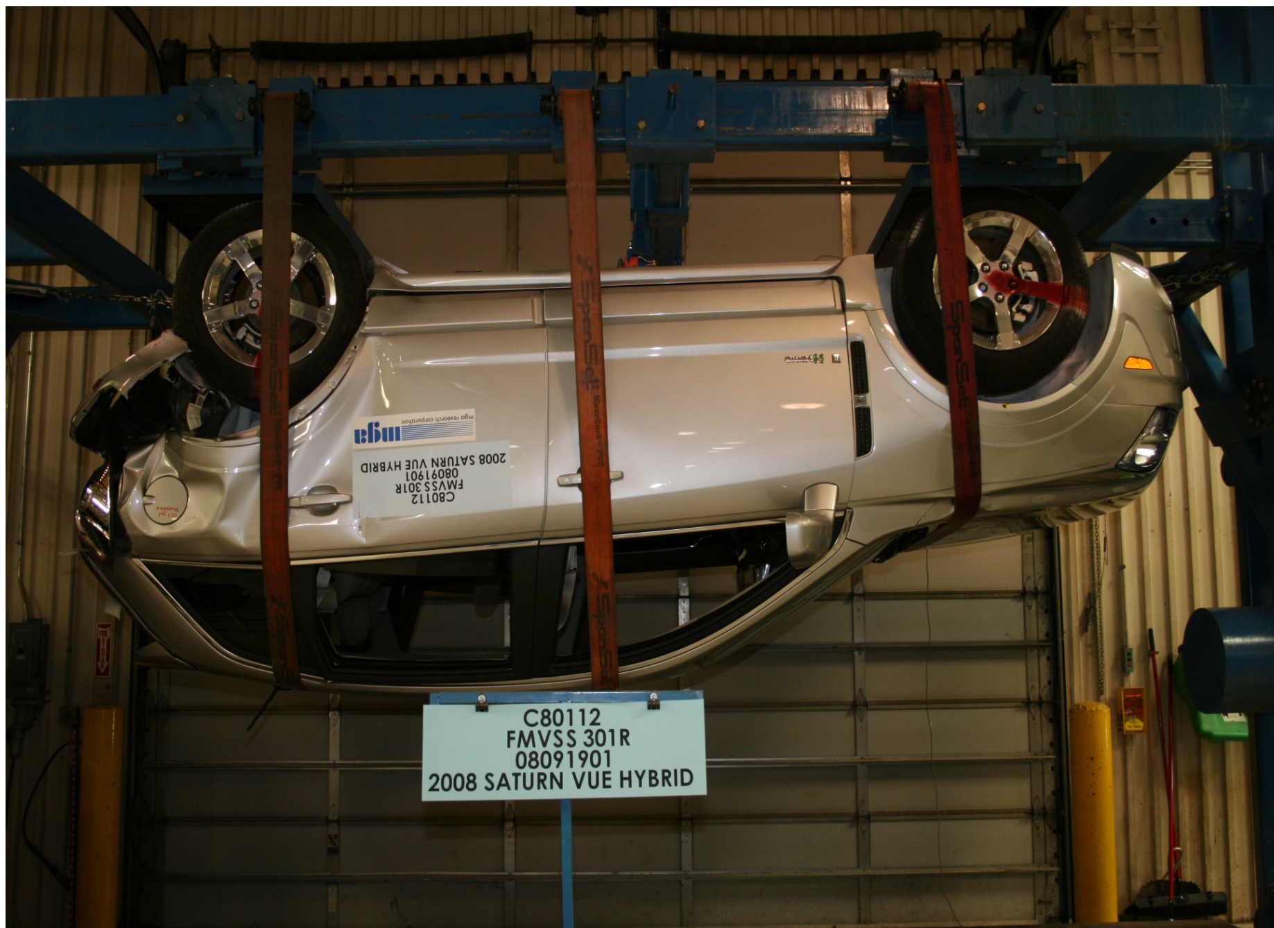
Static Rollover at 180 Degrees
