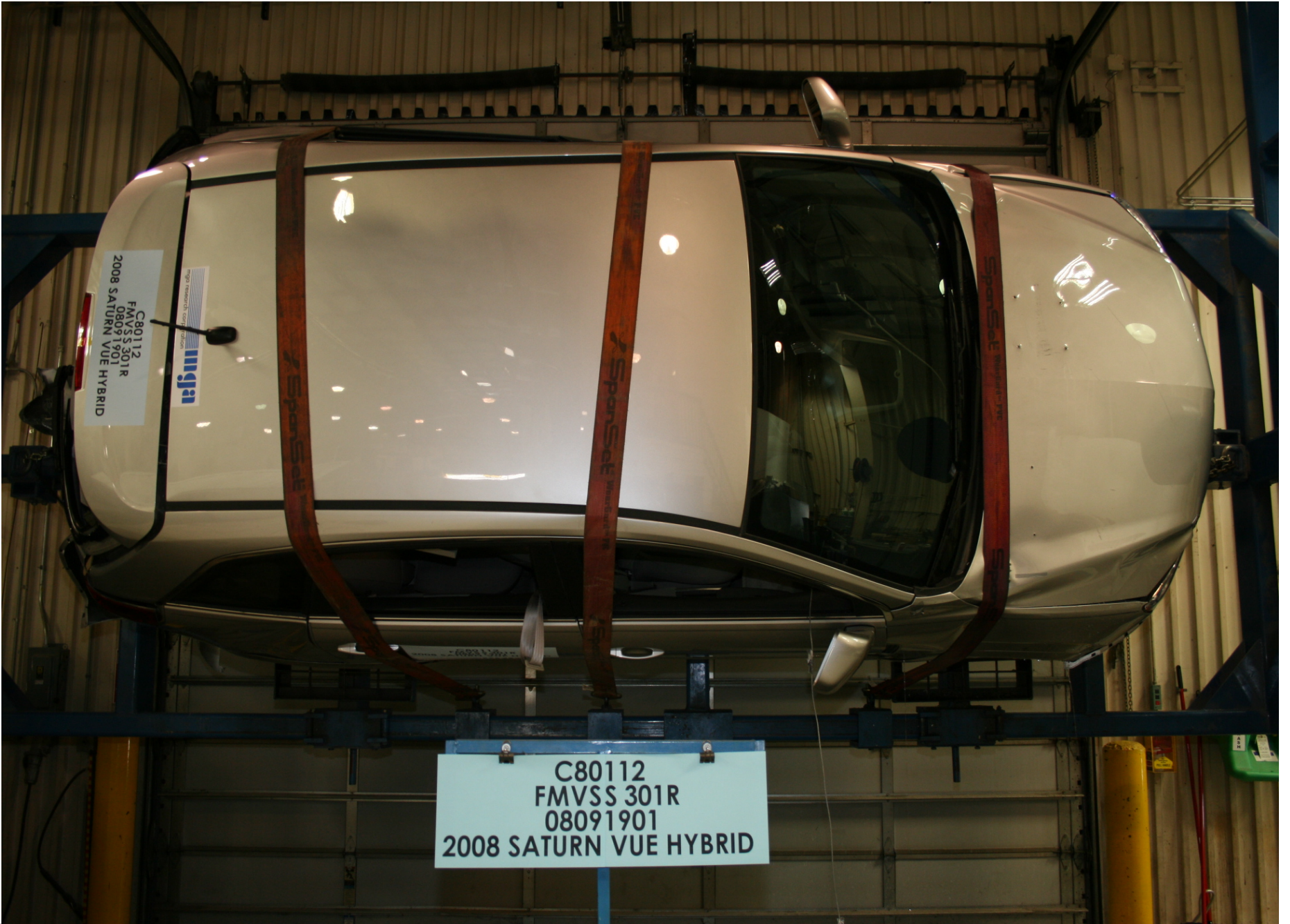
Static Rollover at 270 Degrees
