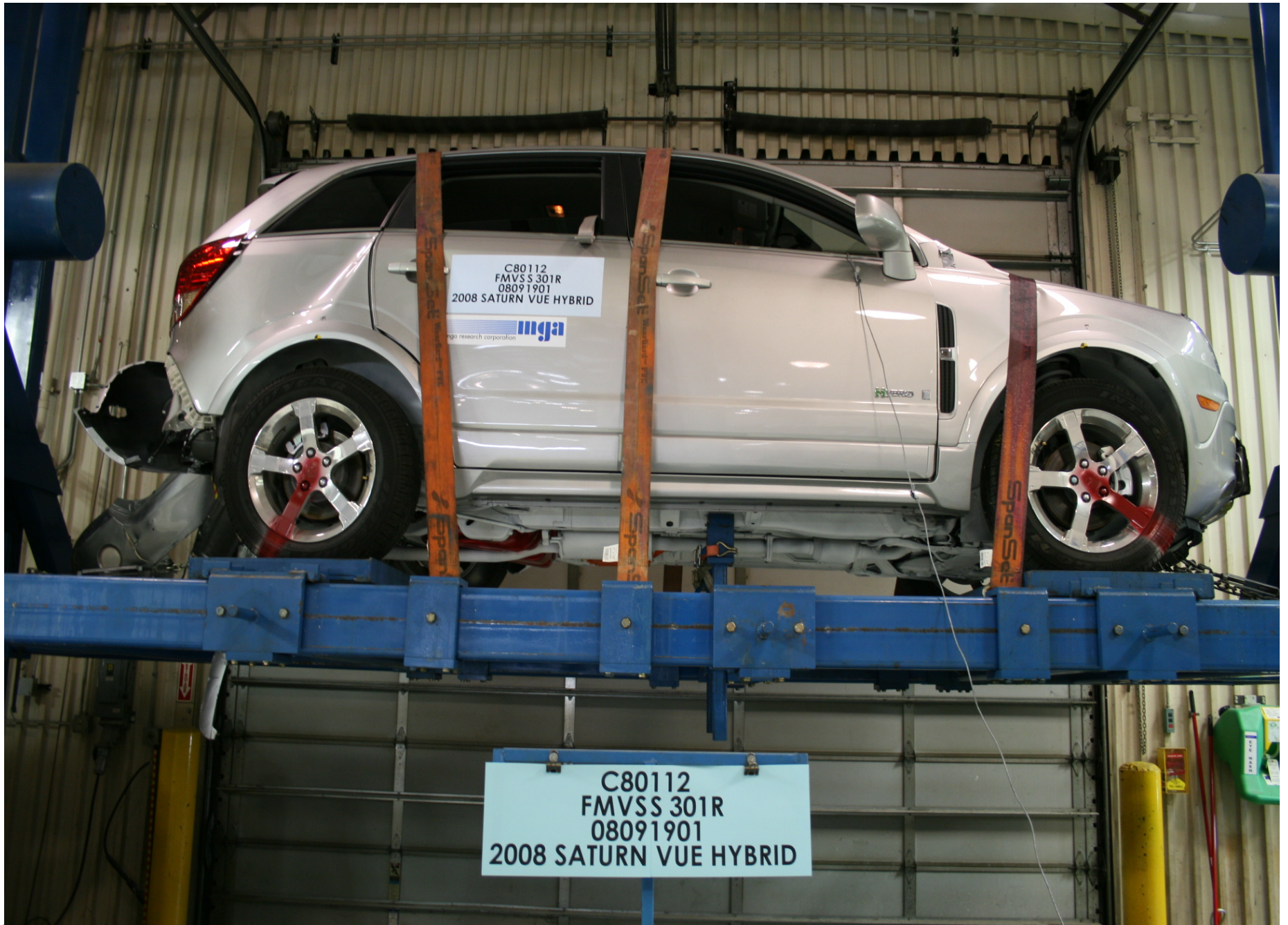
Static Rollover at 360 Degrees
