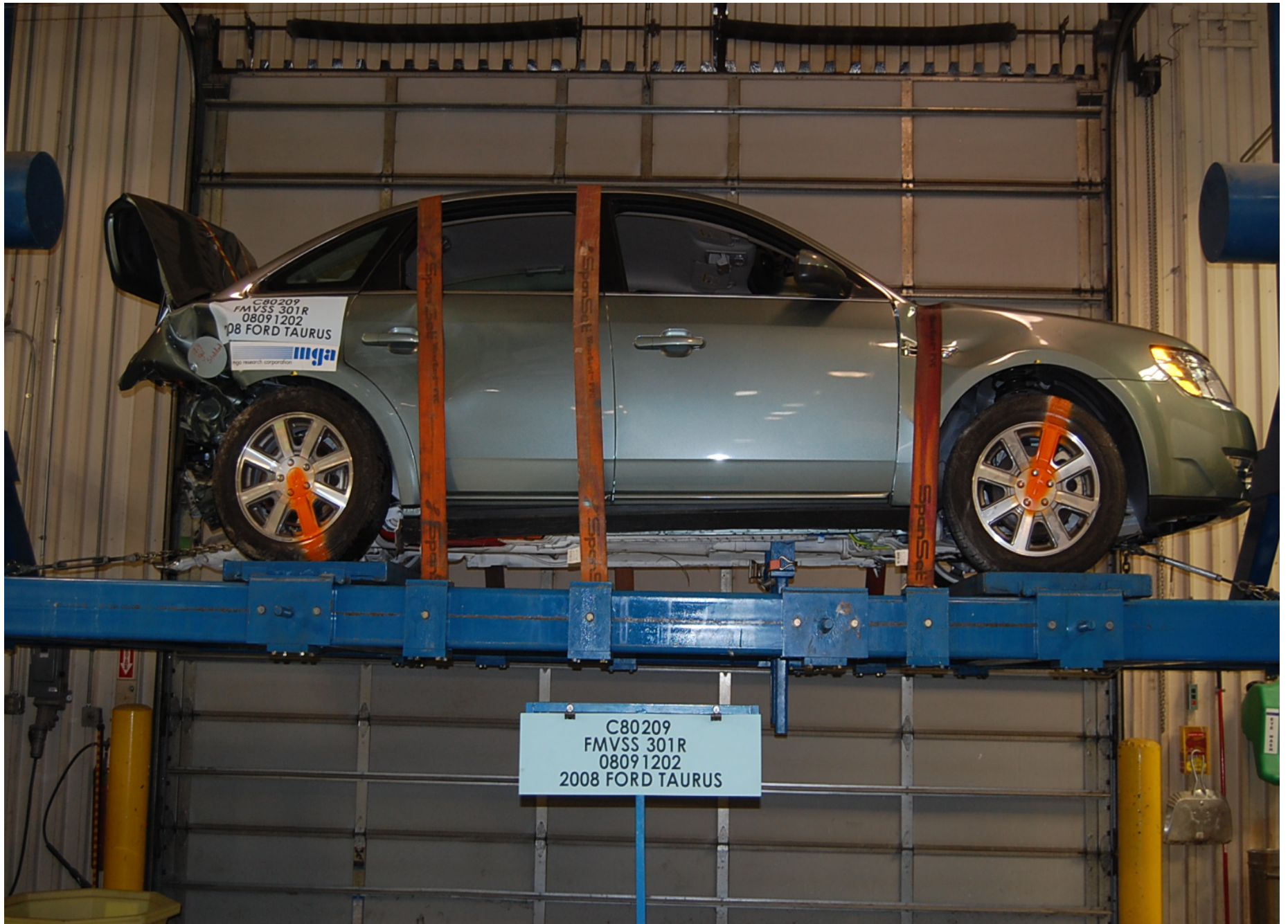
Static Rollover at 360 Degrees
