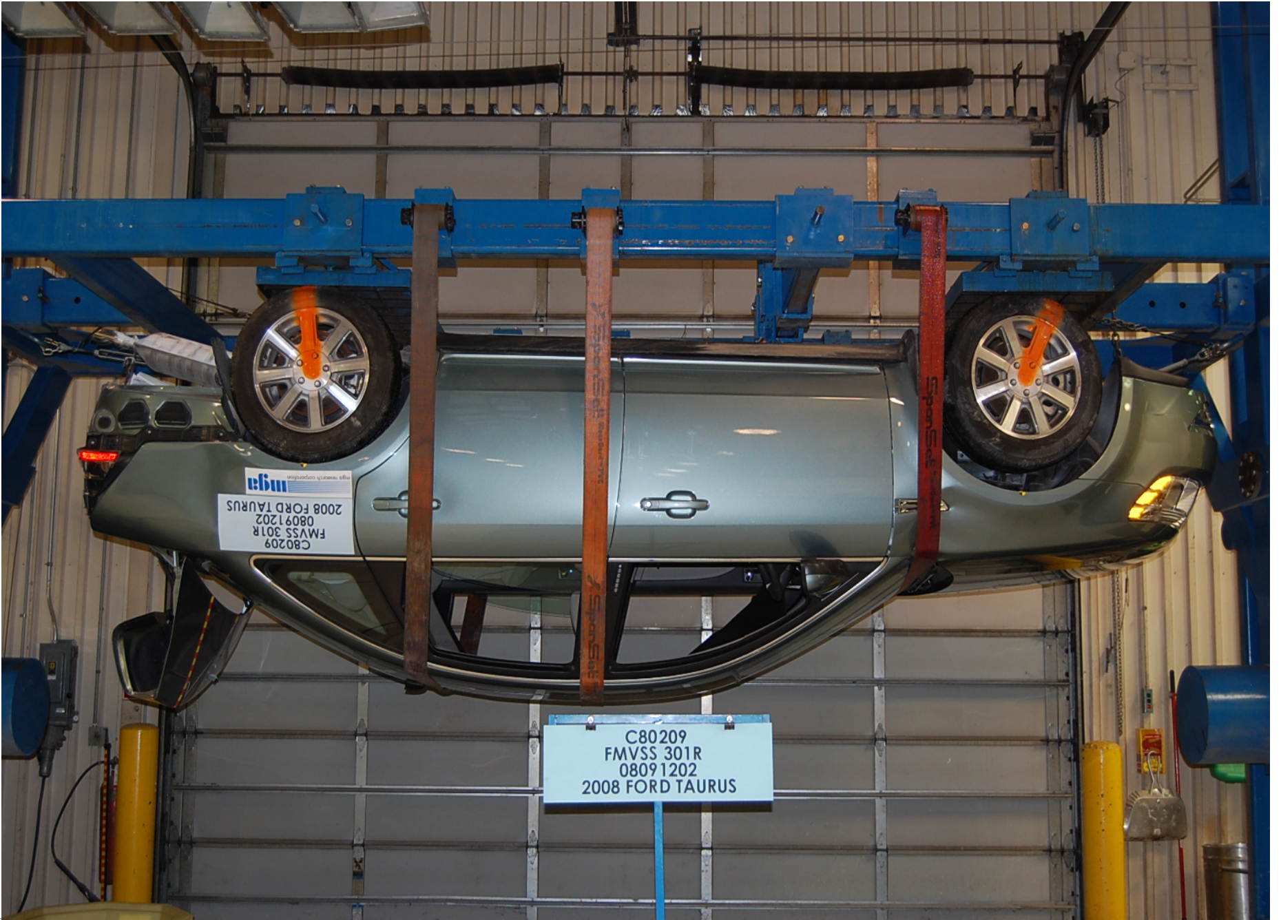
Static Rollover at 180 Degrees
