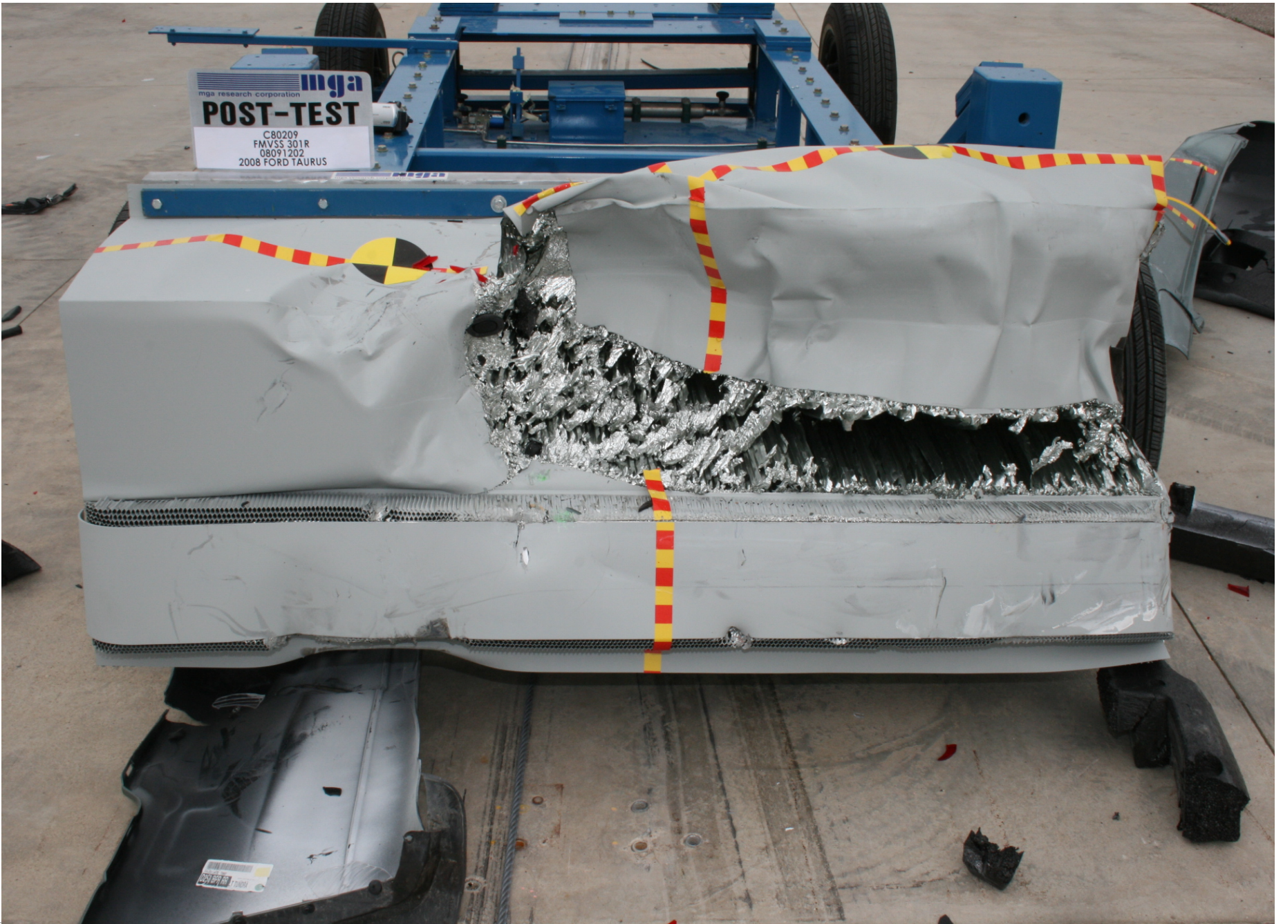
Post-Test Front View of MDB
