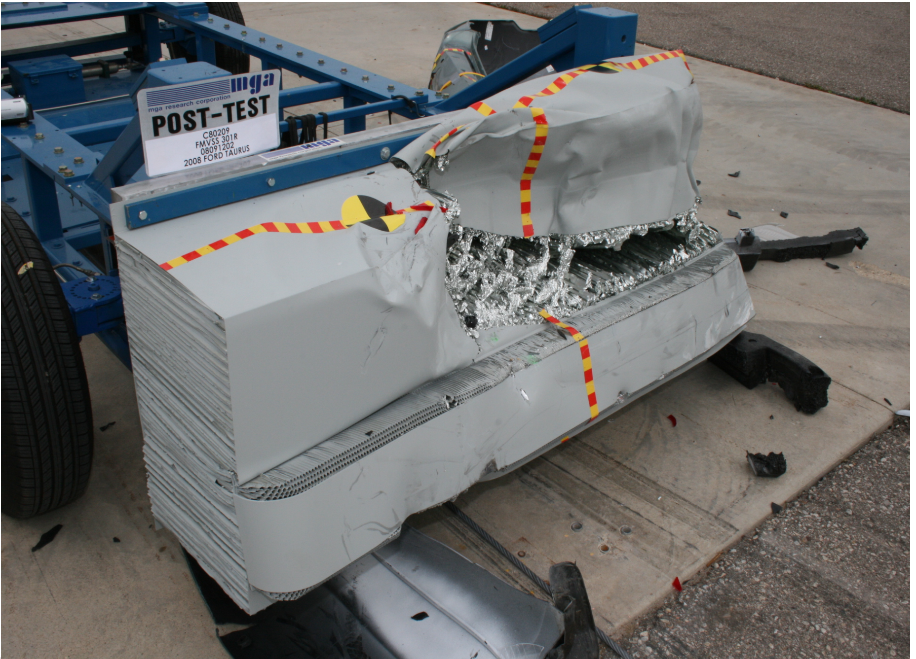
Post-Test ¾ Right Side View of MDB
