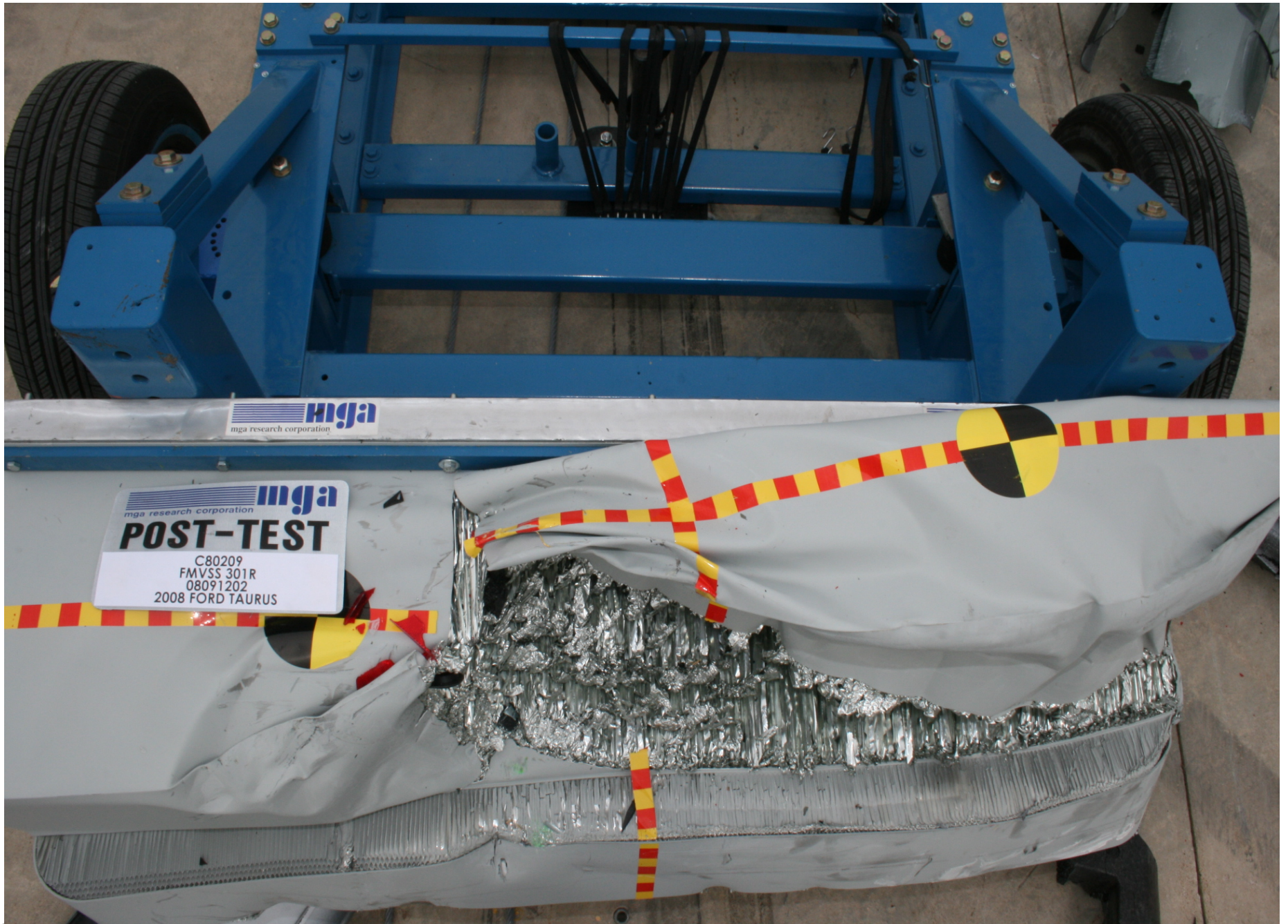
Post-Test Top View of MDB
