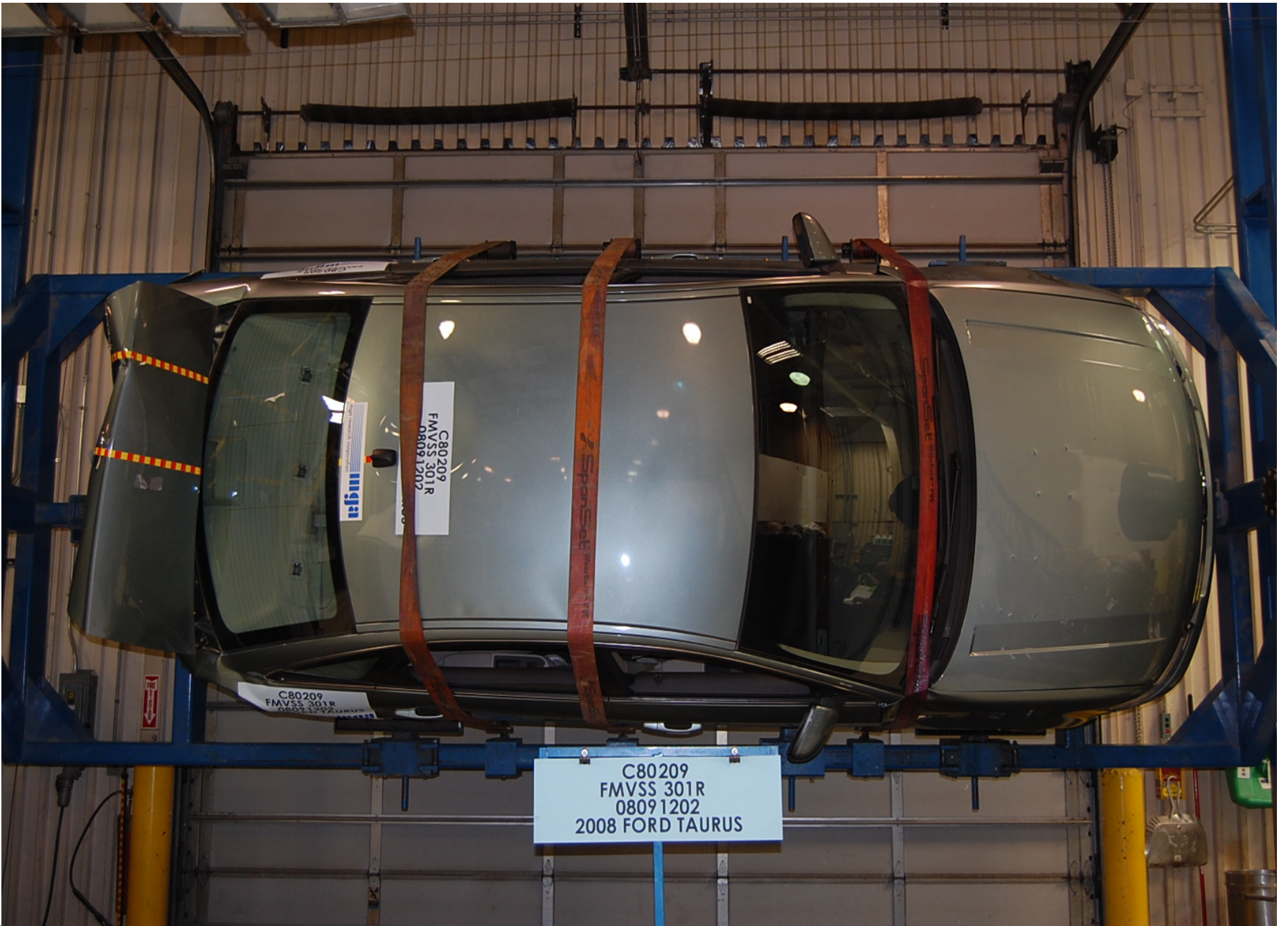
Static Rollover at 90 Degrees
