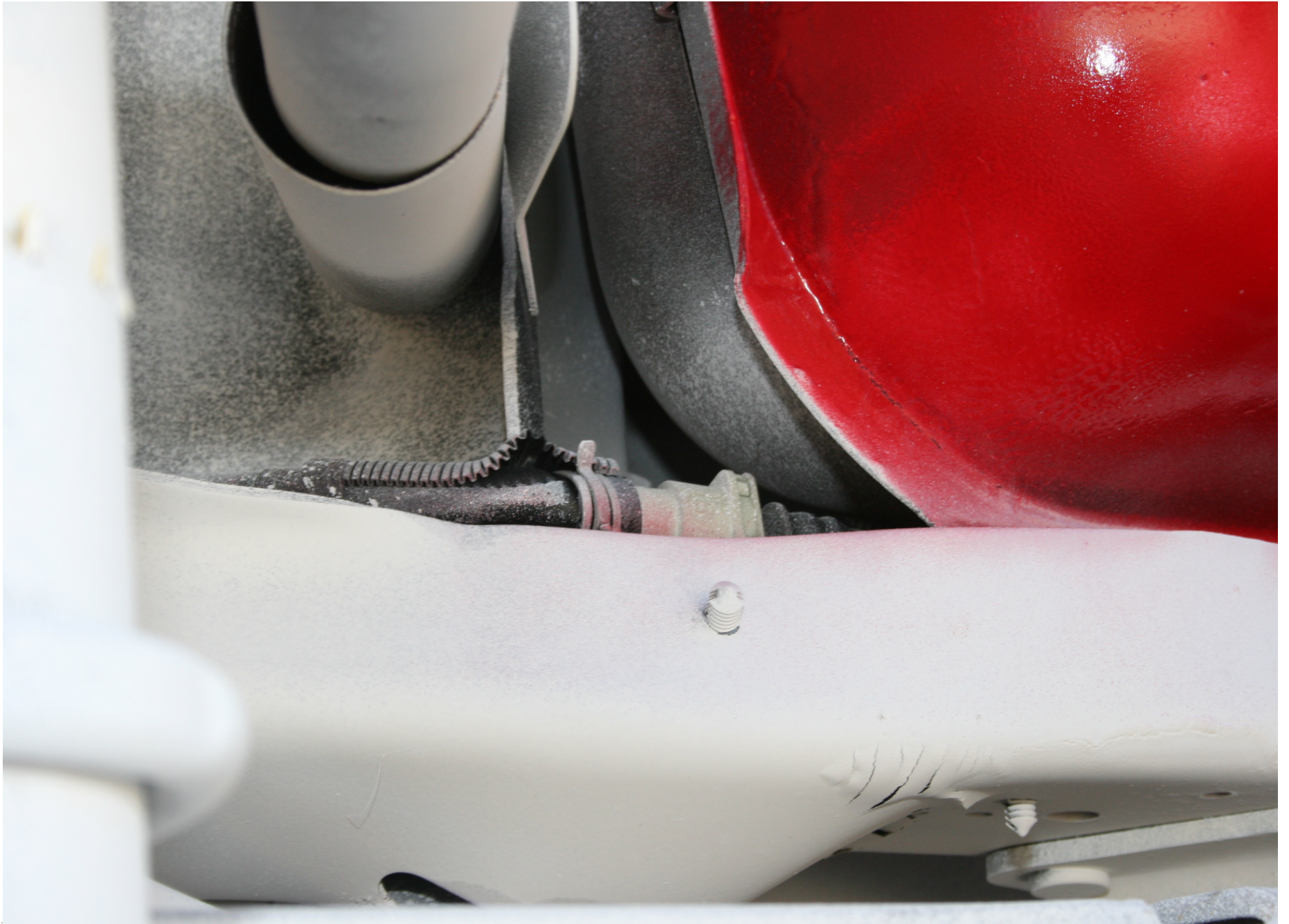
Fuel System Vapor Line Leak
