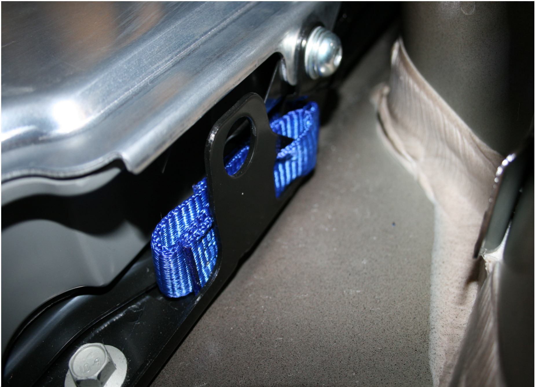
Pre-Test Propulsion Battery Tether
