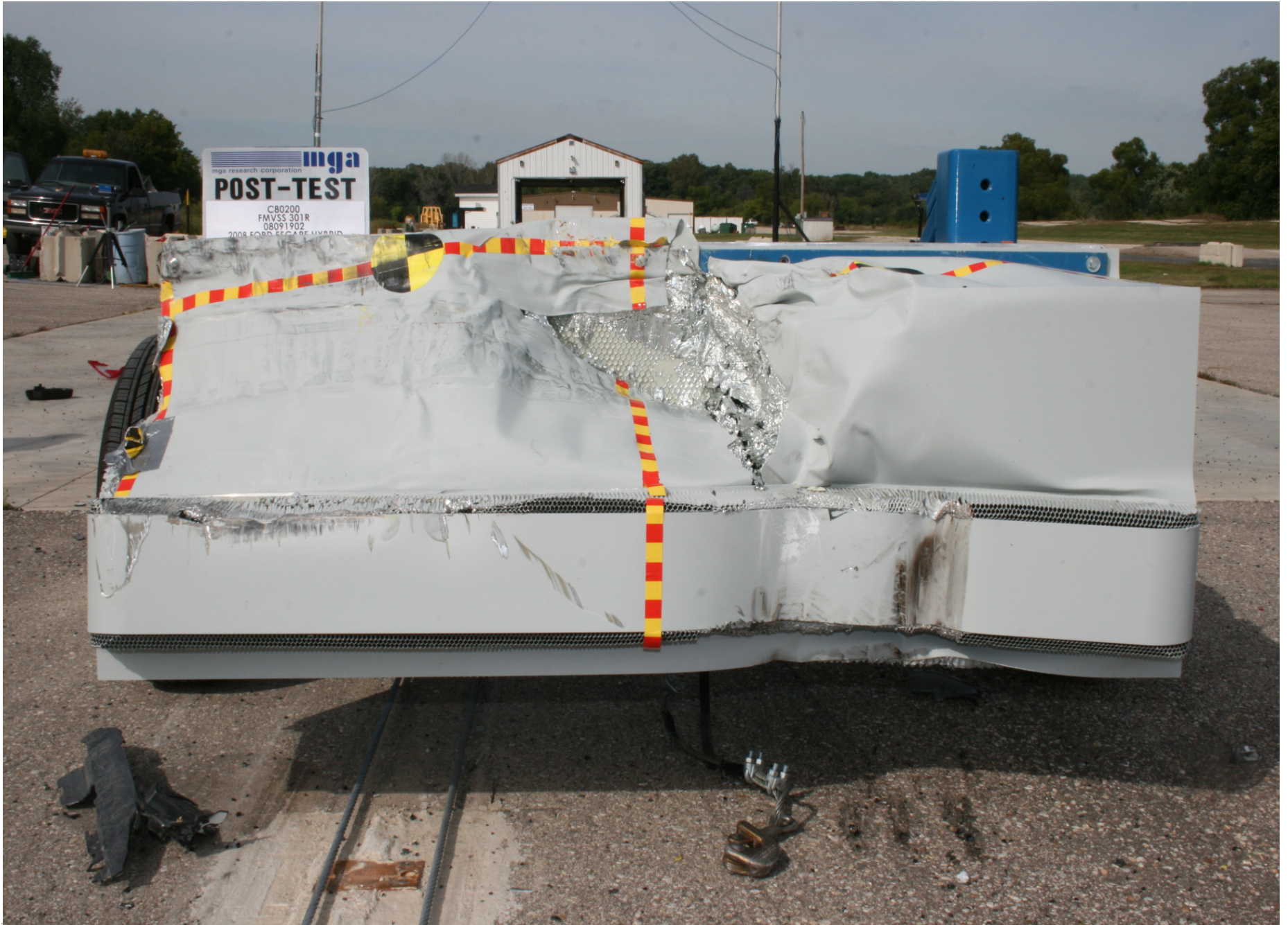
Post-Test Front View of MDB
