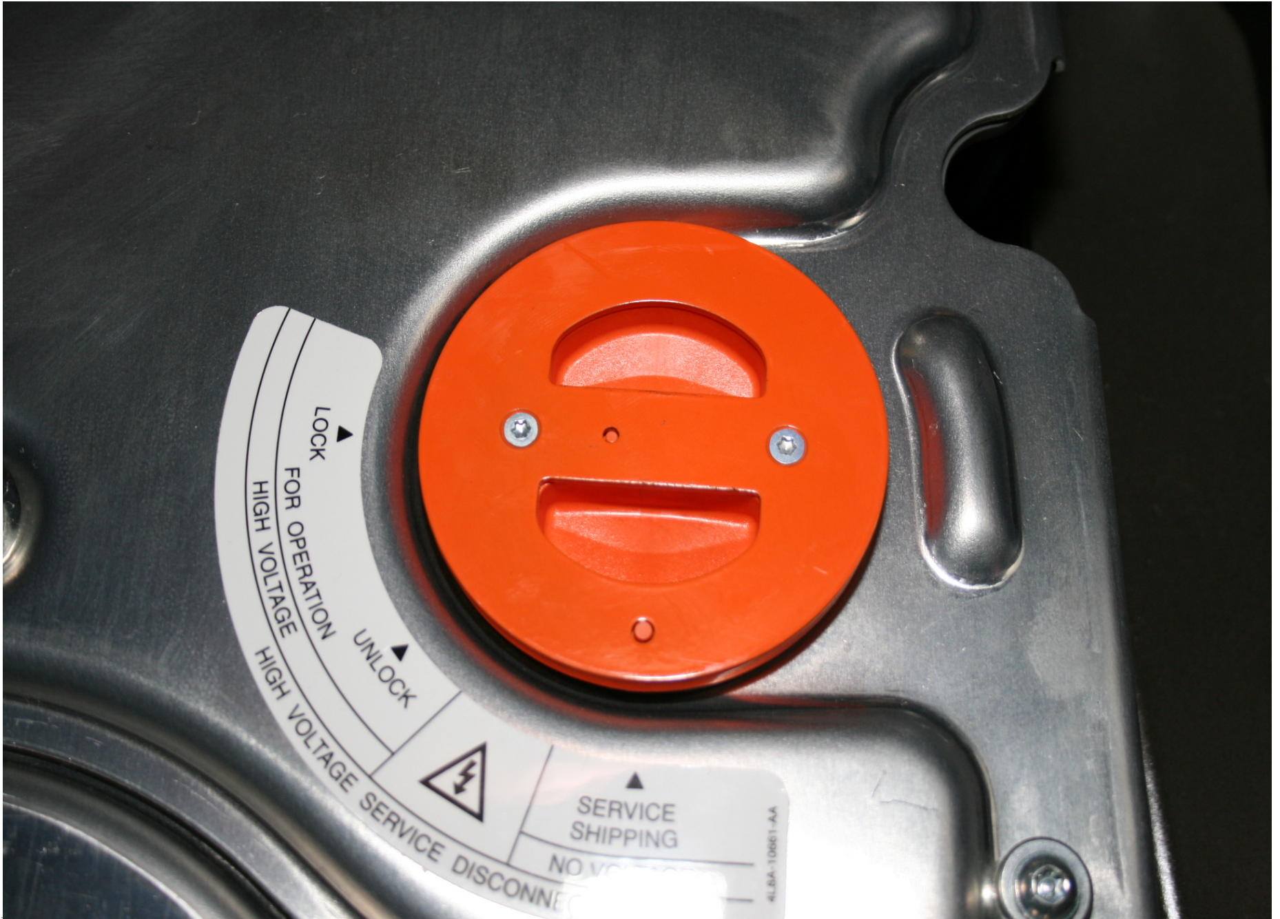
Pre-Test Service Switch Disconnect
