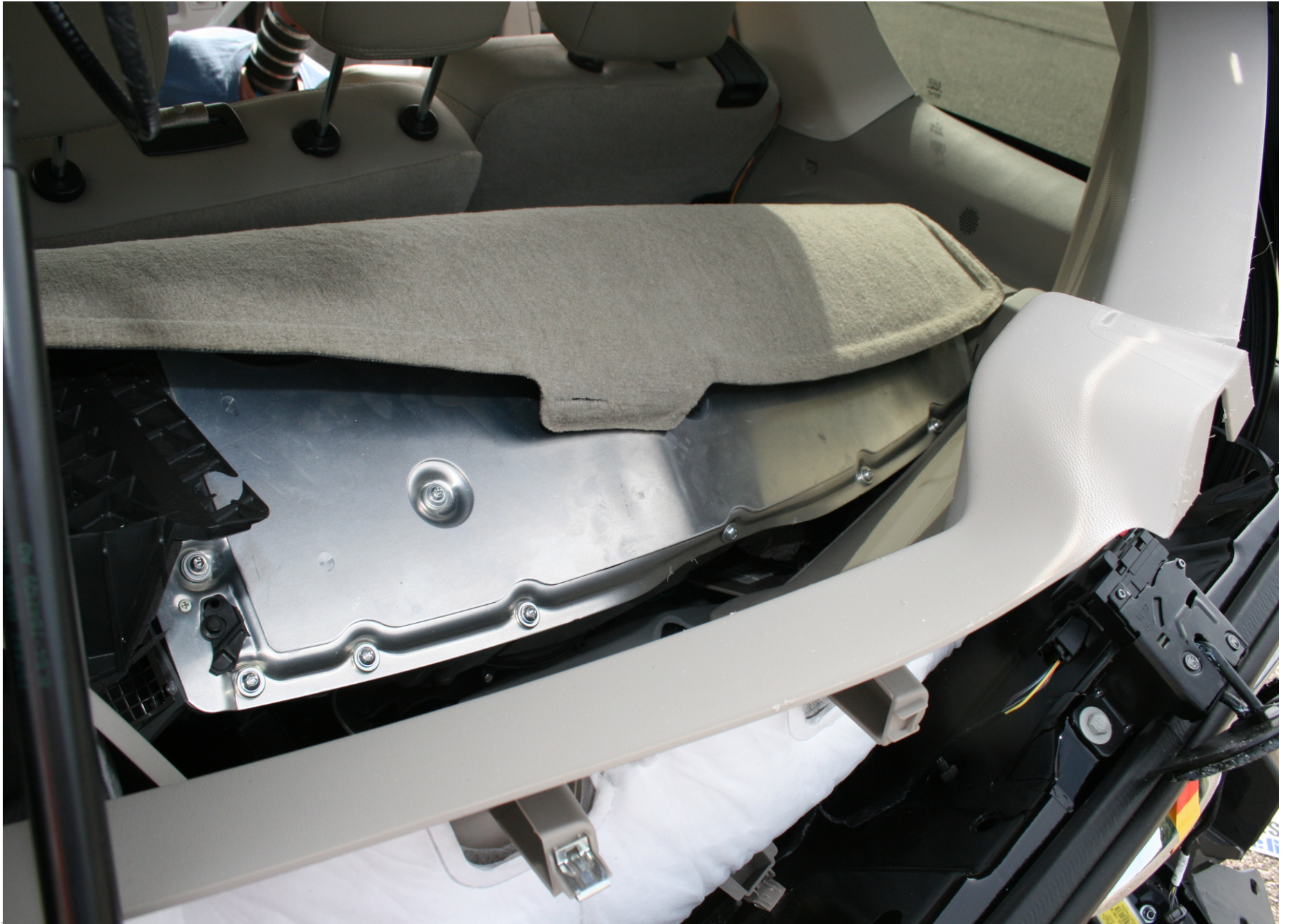
Post-Test Propulsion Battery Module View 2
