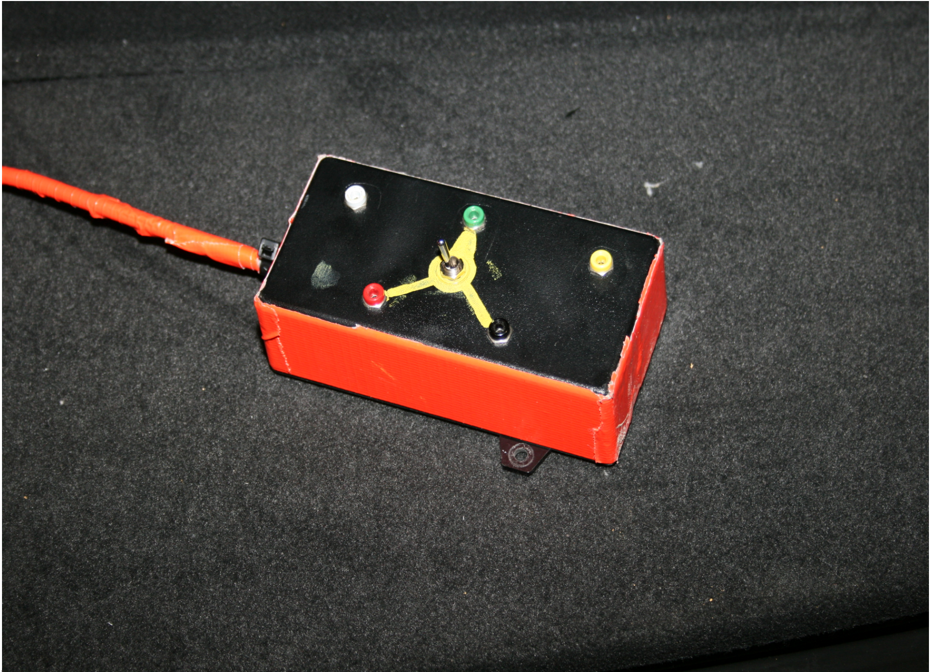
Pre-Test Installed Test Interface Port
