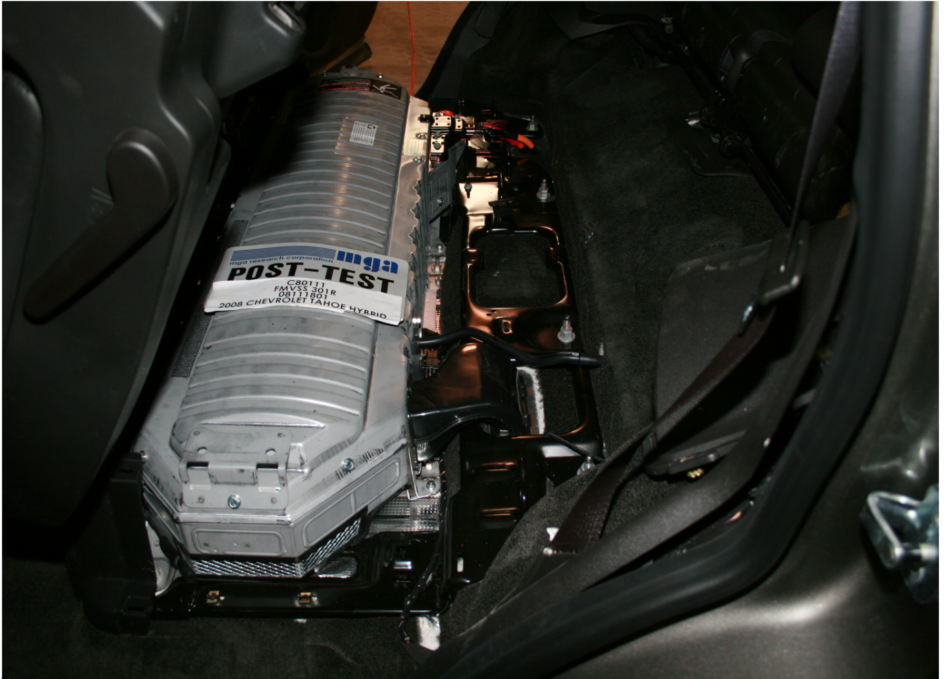
Post-Test Vehicle Pass. Compartment Adjacent to Propulsion Battery
