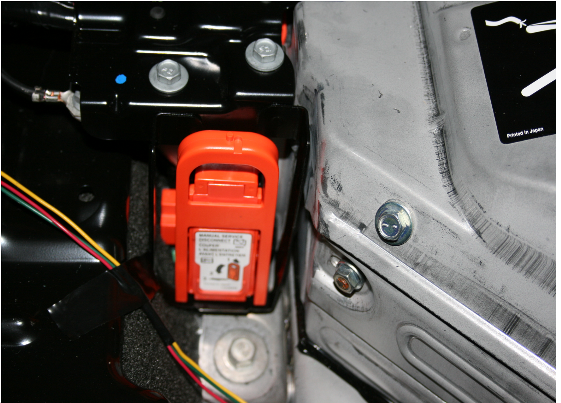
Pre-Test Service Switch Disconnect
