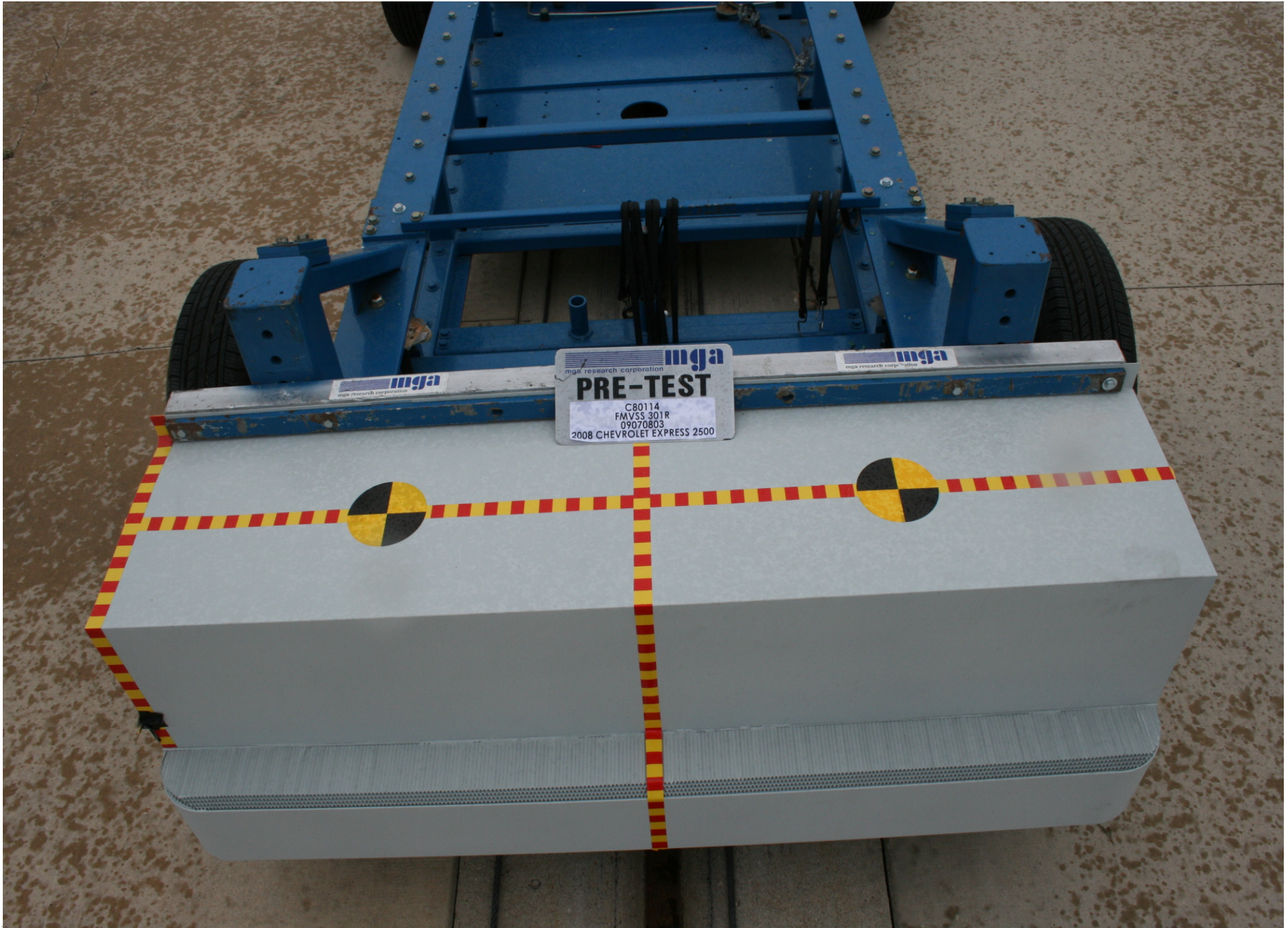
Pre-Test Top View of MDB
