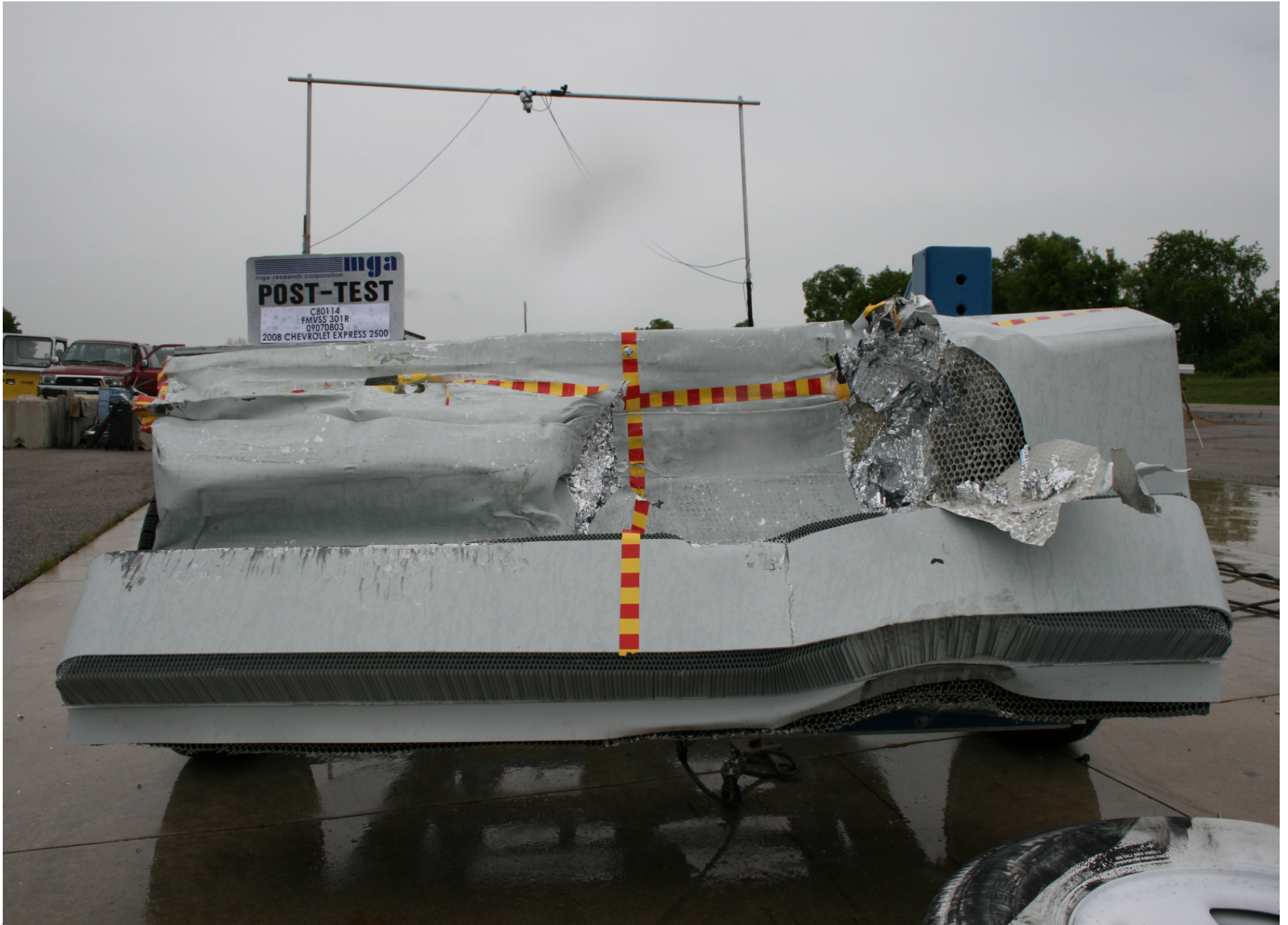
Post-Test Front View of MDB
