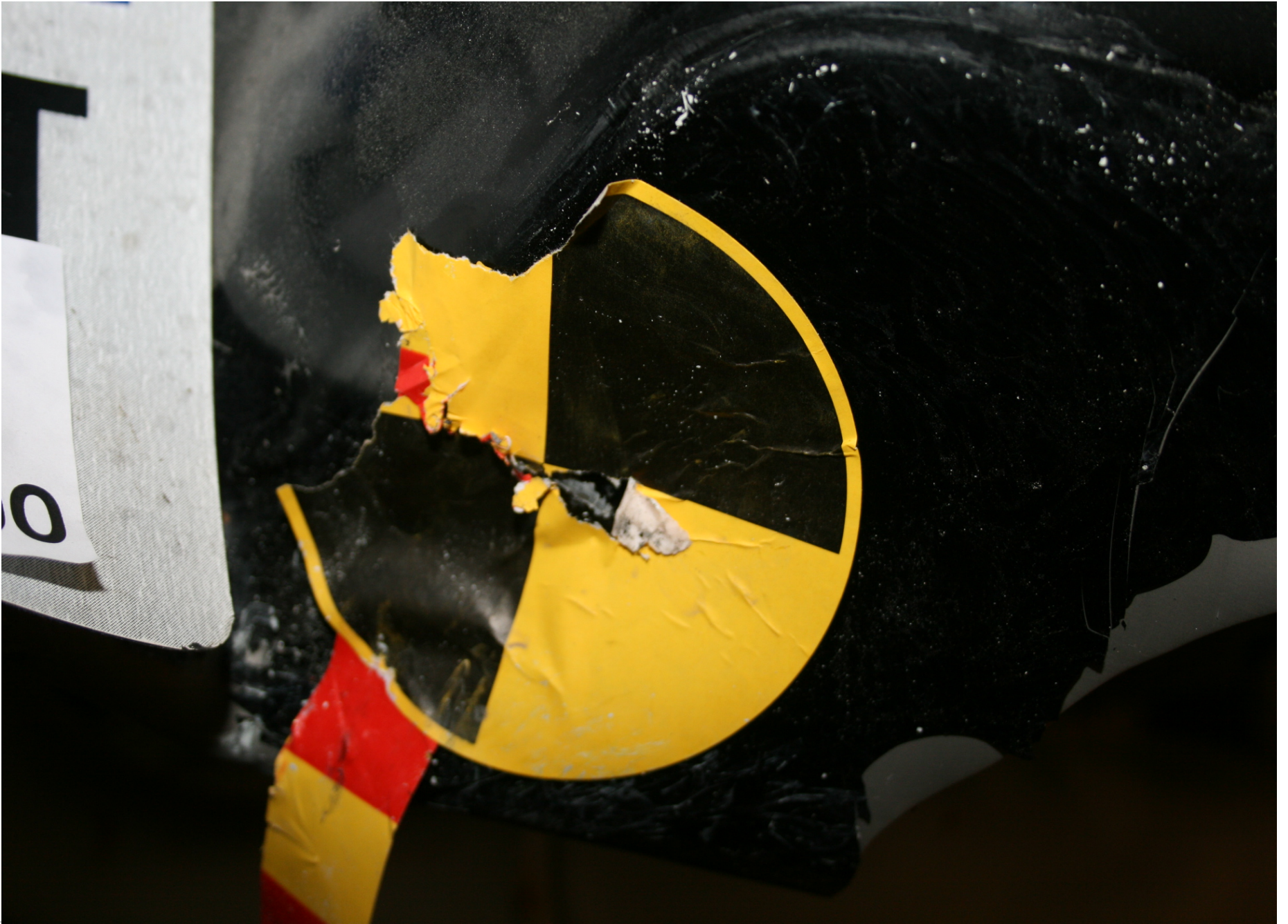
Post-Test Impact Point
