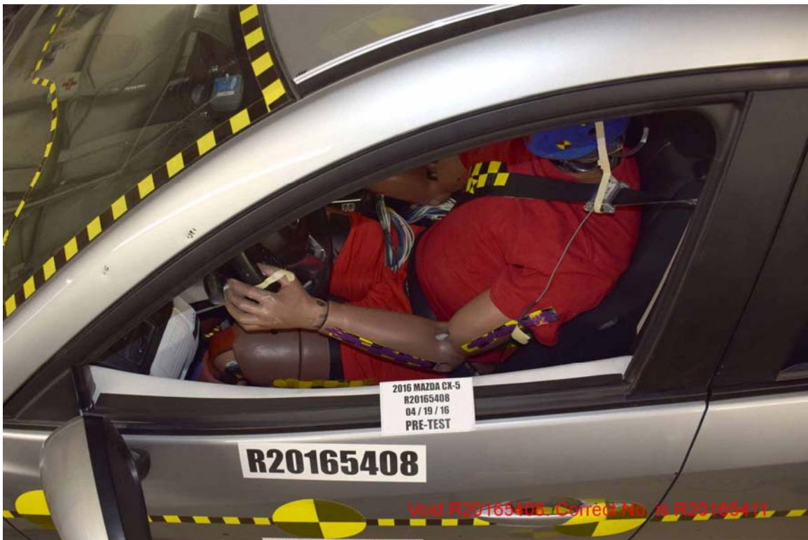
FIGURE 58. Pre-Test View of Driver Door Clearance
