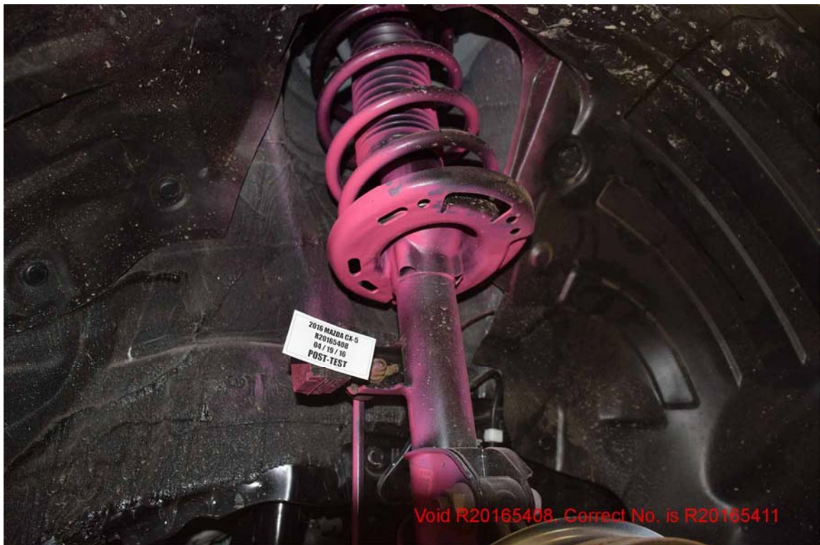
FIGURE 160. Post-Test Passenger Close-up View of Suspension
