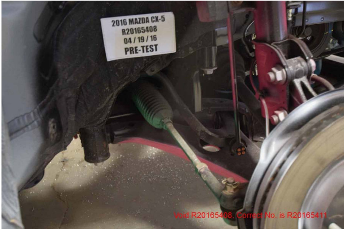
FIGURE 161. Pre-Test Right Side Tie Rod and Sway Bar Attachment Points
