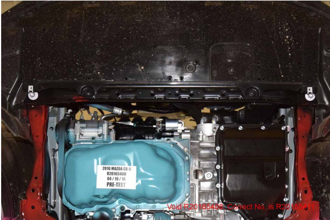
FIGURE 139. Pre-Test Bumper to Rail Attachments and Crush Initiators
