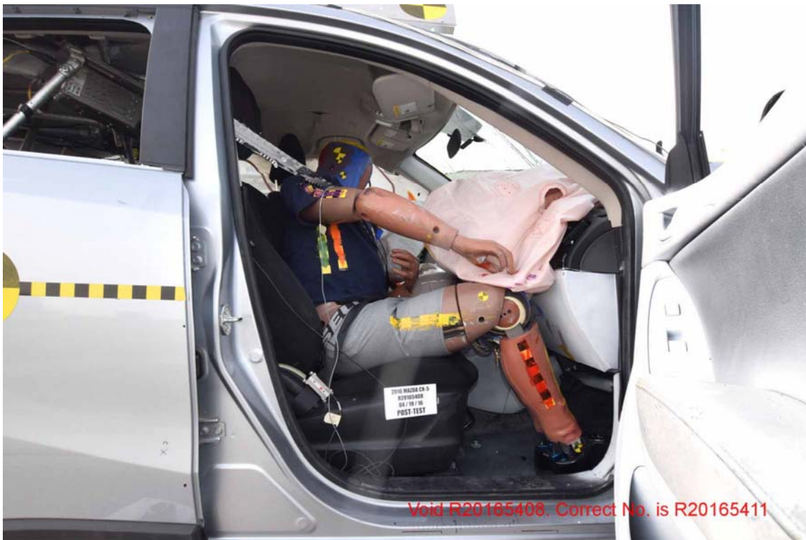
FIGURE 102. Post-Test Right Side Passenger and Interior View
