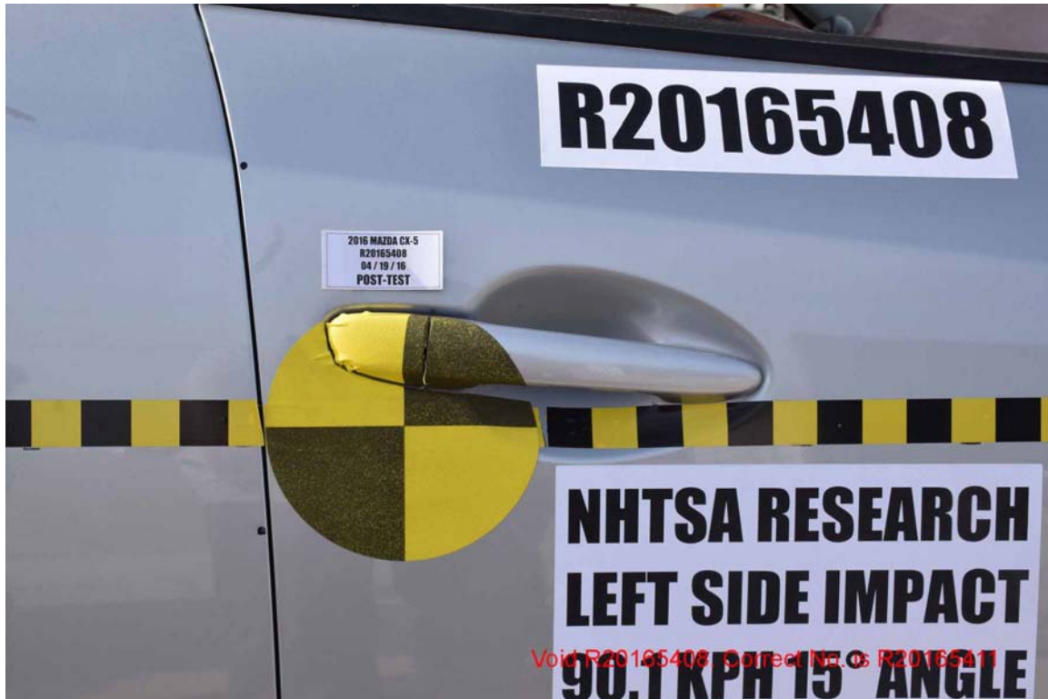
FIGURE 31. Post-Test Close-up View of Passenger Door Latch
