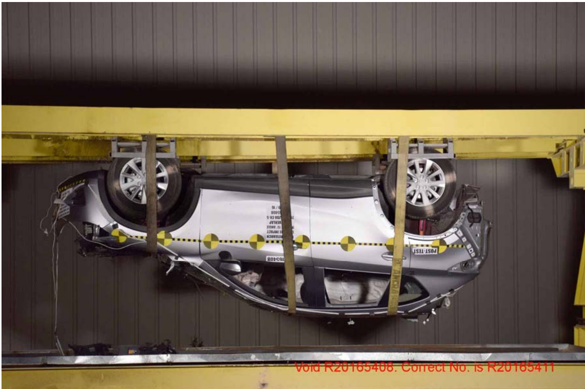
FIGURE 184. FMVSS No. 301 Static Rollover 180 Degrees
