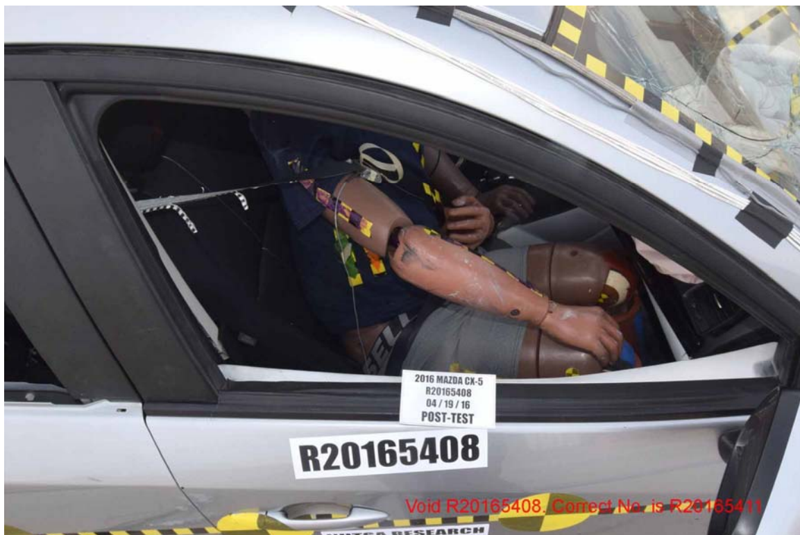
FIGURE 104. Post-Test View of Passenger Door Clearance
