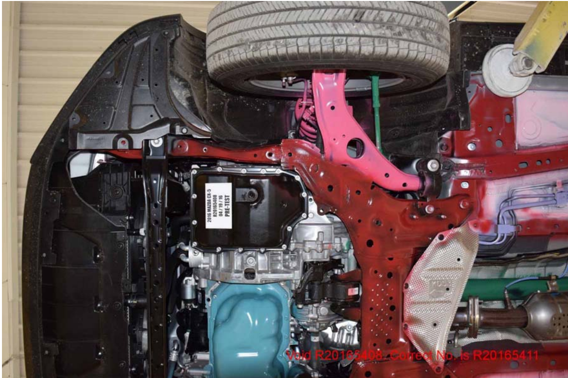
FIGURE 141. Pre-Test Left Side Impact Rail
