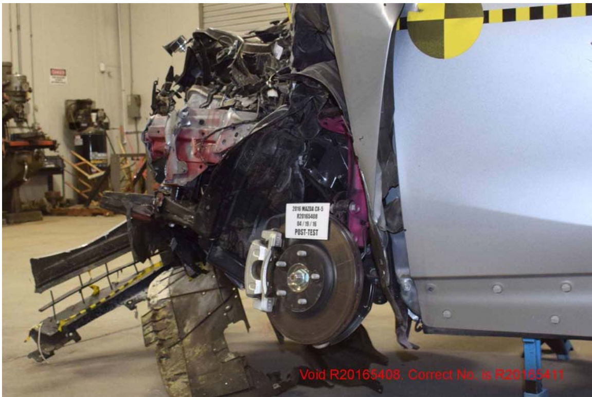
FIGURE 148. Post-Test Left Rear \frac{3}{4} View of the Driver Wheel Well
