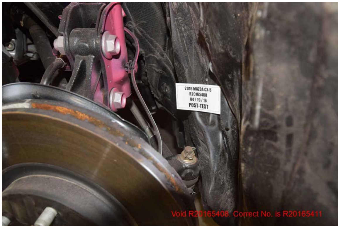
FIGURE 152. Post-Test Left Side Tie Rod and Sway Bar Attachment Points
