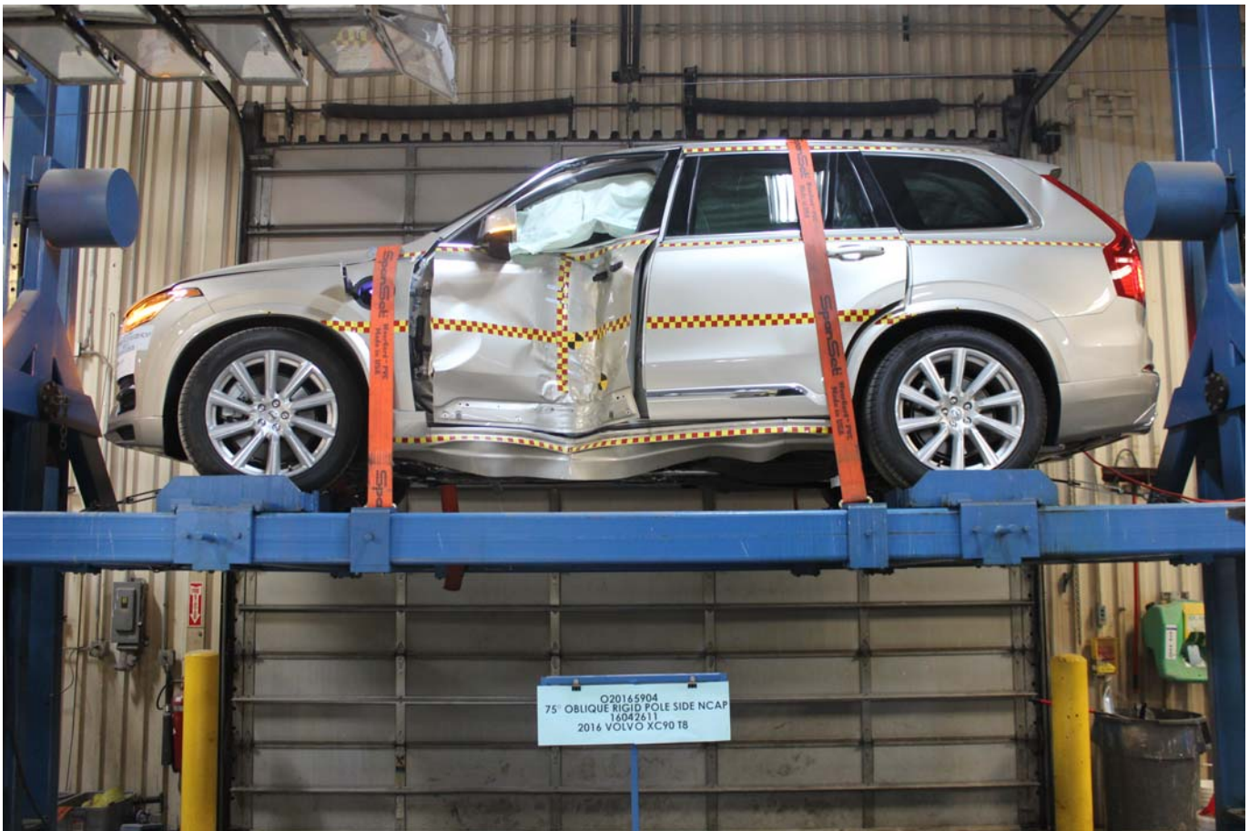
Photo No. 067 - FMVSS No. 301 Static Rollover 360 Degrees
