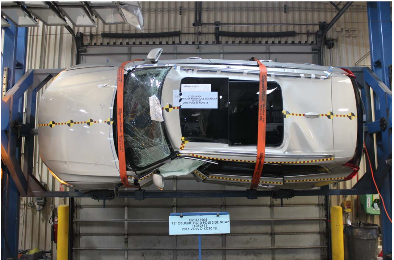
Photo No. 066 - FMVSS No. 301 Static Rollover 270 Degrees
