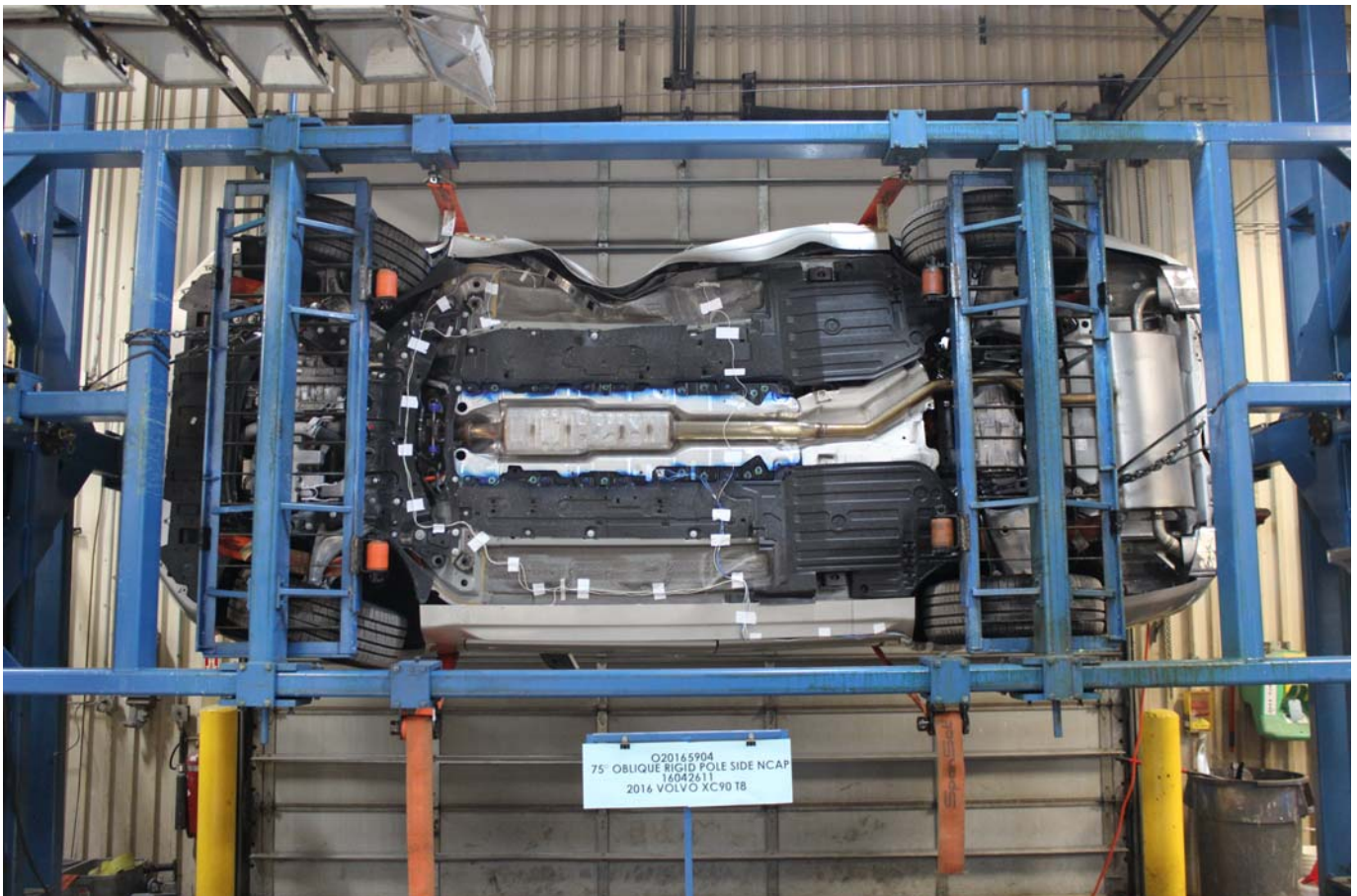
Photo No. 064 - FMVSS No. 301 Static Rollover 90 Degrees
