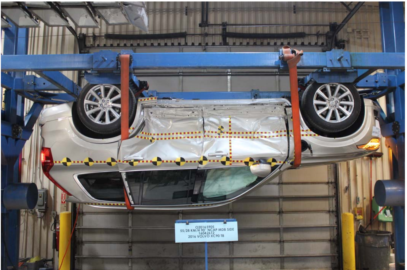
Photo No. 028 - FMVSS No. 305 Static Rollover at 180°
