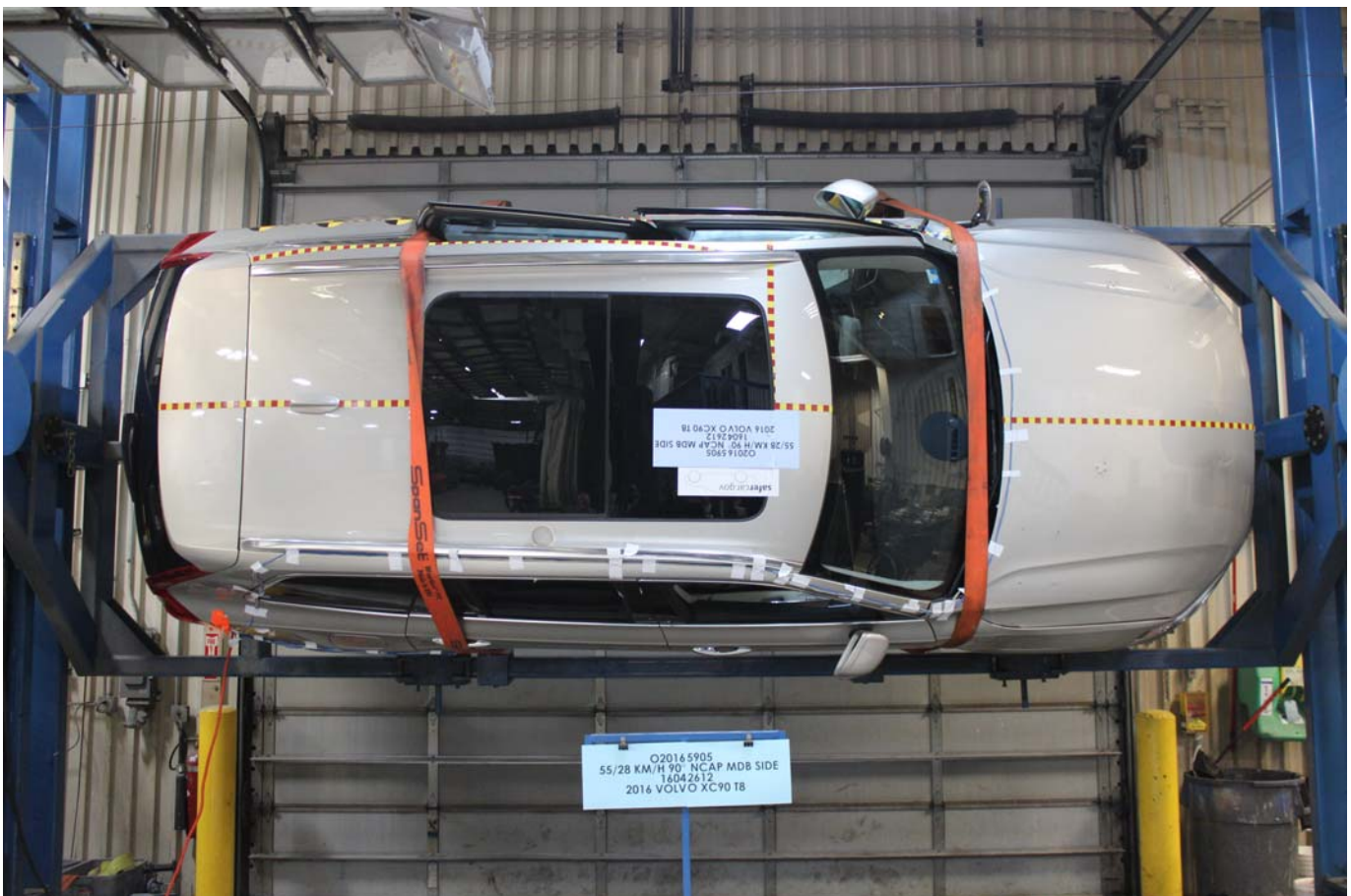
Photo No. 027 - FMVSS No. 305 Static Rollover at 90°
