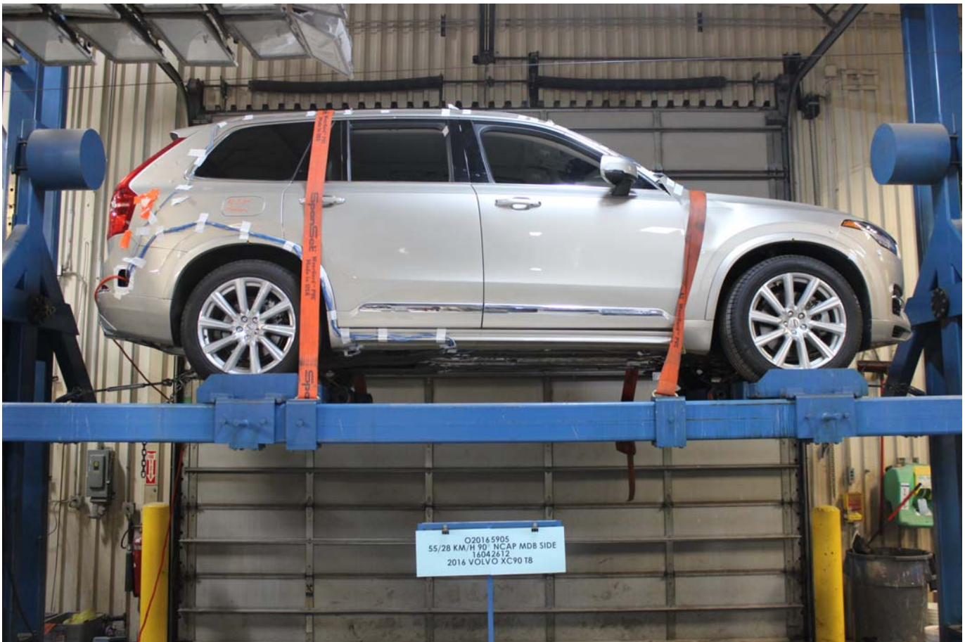
Photo No. 030 - FMVSS No. 305 Static Rollover at 360°
