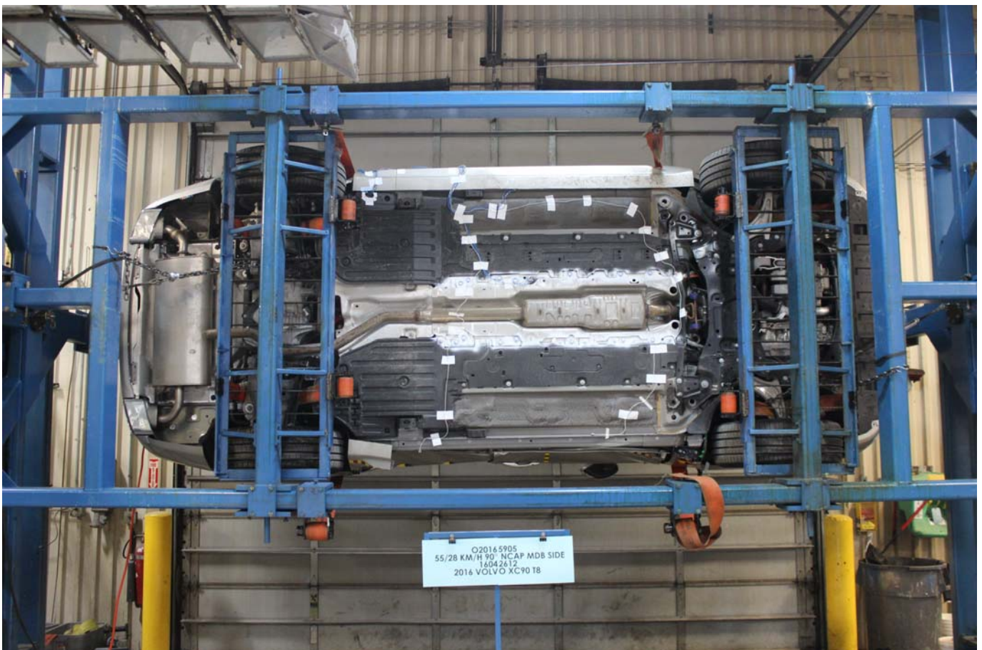
Photo No. 029 - FMVSS No. 305 Static Rollover at 270°
