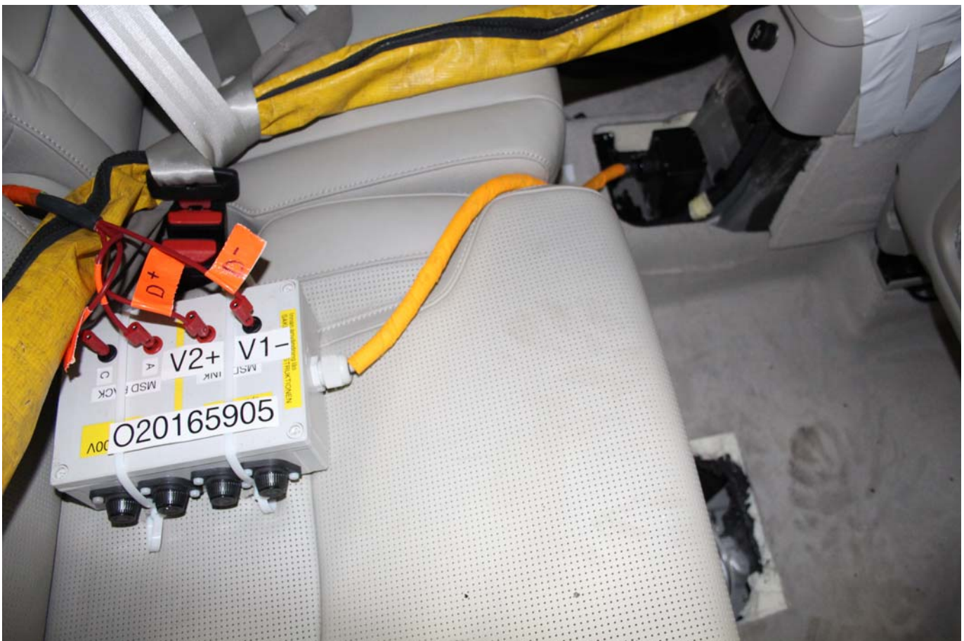
Photo No. 021 - Pre-Impact View of High Voltage Leads Attached
