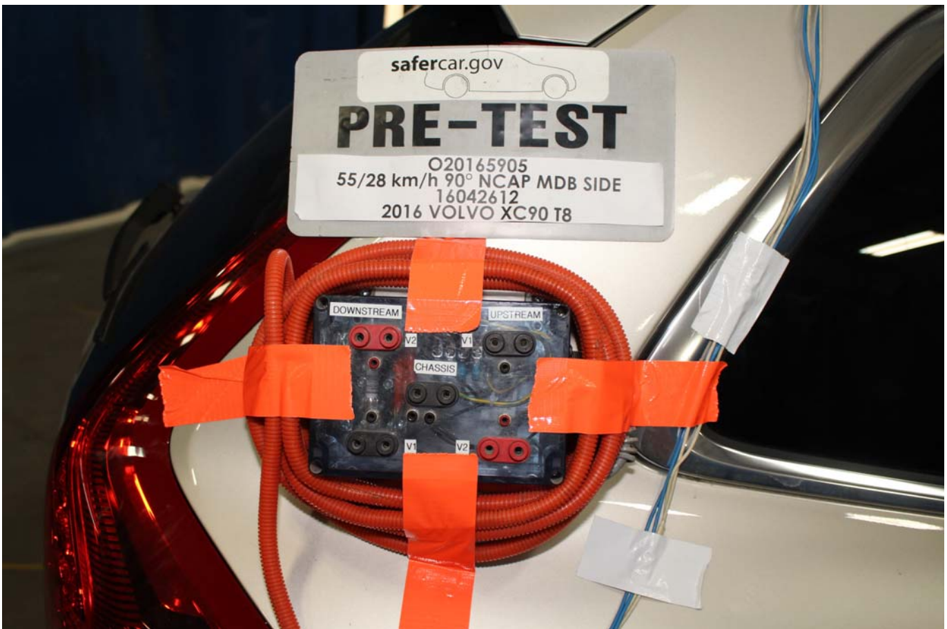
Photo No. 023 - Pre-Impact View of Installed Impact Interface Port
