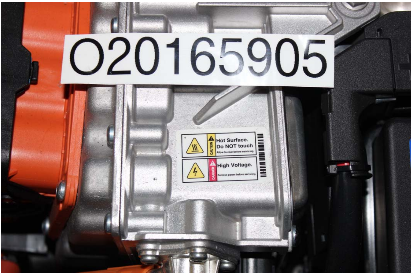
Photo No. 002 - Power Inverter Warning Label
