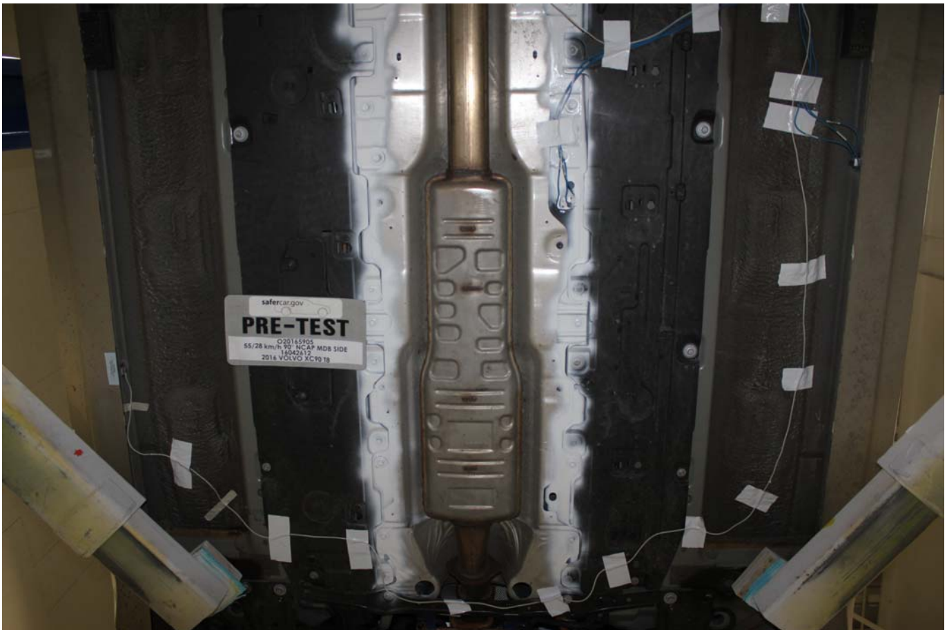
Photo No. 008 - Pre-Impact View of Propulsion Battery
