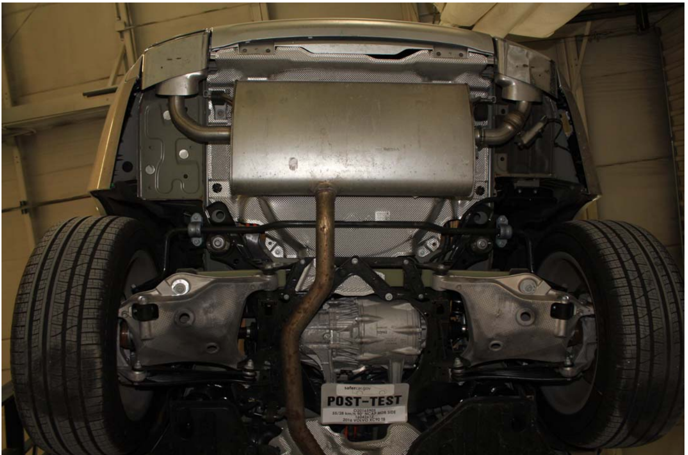
Photo No. 016 - Post-Impact View of Electric Propulsion Drive
