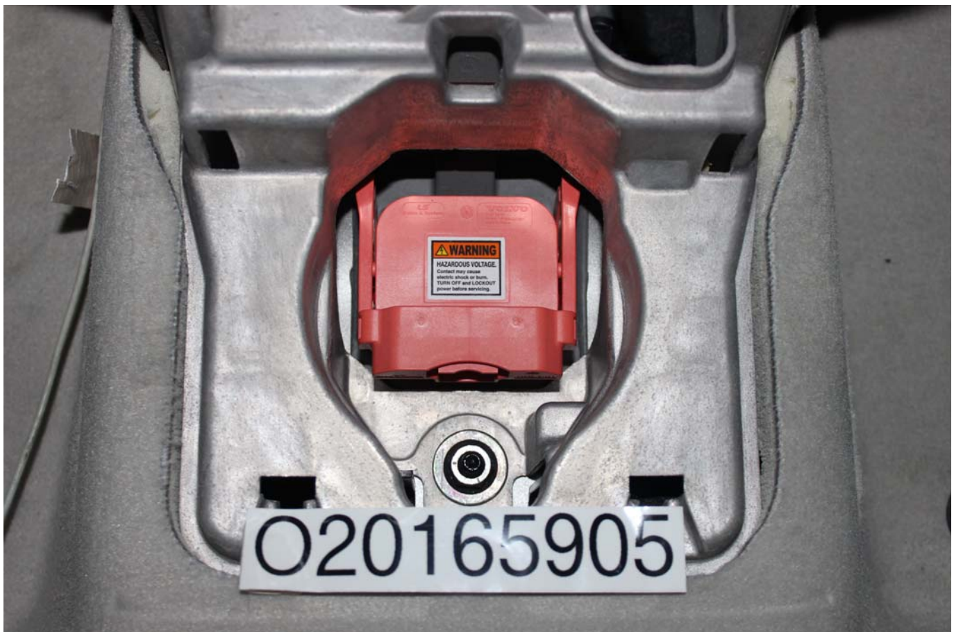
Photo No. 006 - Manual High Voltage Service Disconnect in Place
