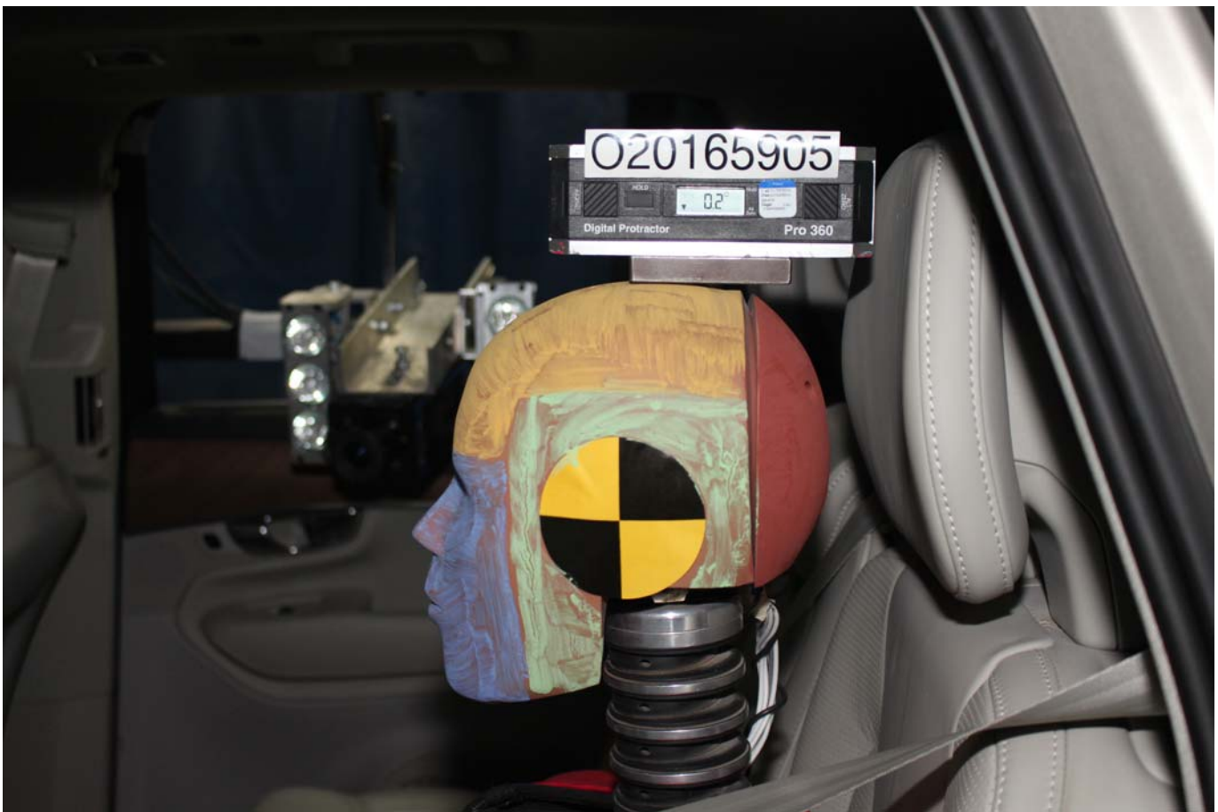
Photo No. 063 - Pre-Test View of Rear Passenger Dummy's Head Showing Dummy's Head is Level
