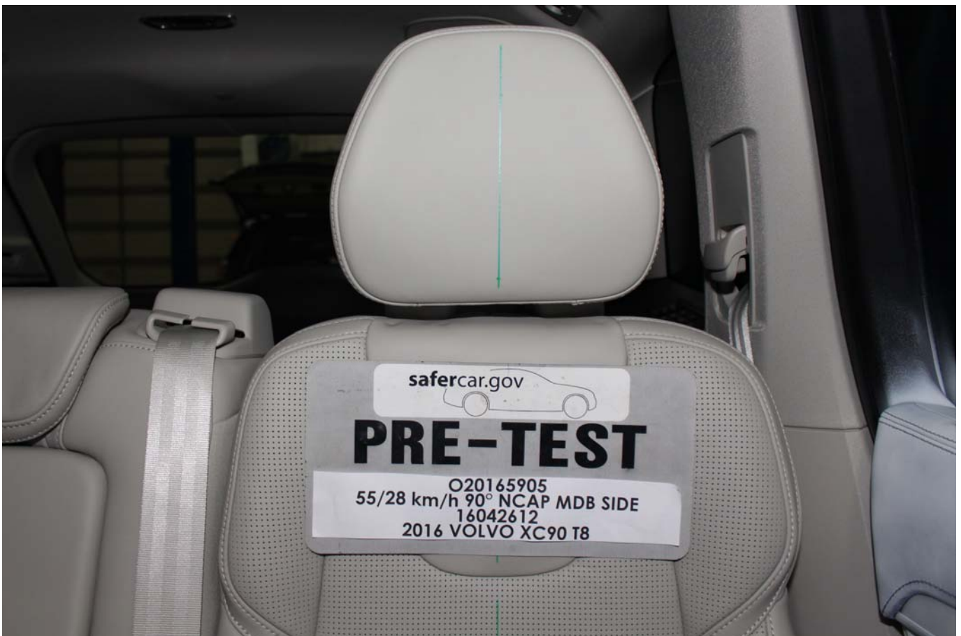
Photo No. 058 - Pre-Test Frontal View of Rear Passenger Seat Back Prior to Dummy Positioning
