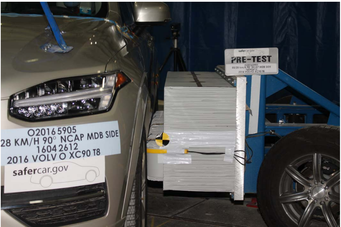
Photo No. 017 - Pre-Test Left Side View of MDB Positioned Against Side of Test Vehicle
