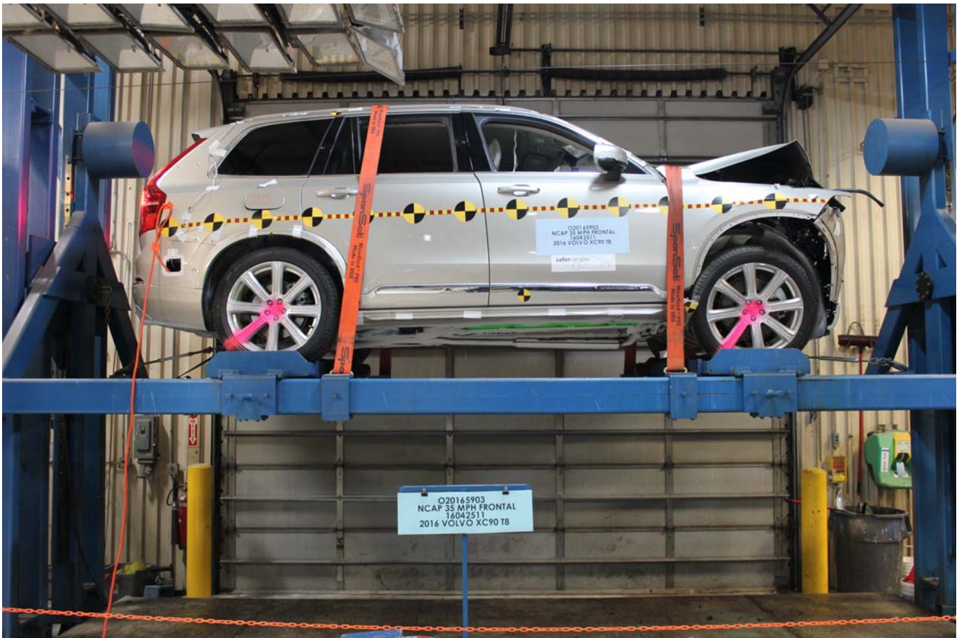
Photo No. 073 - Vehicle at 0 Degree on Static Rollover Device
