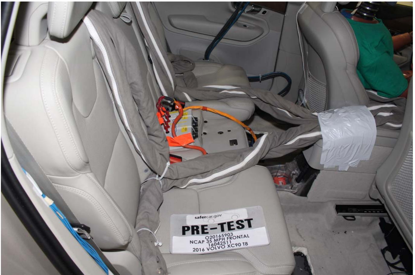
Photo No. 028 - Pre-Test Dummy Cable Routing
