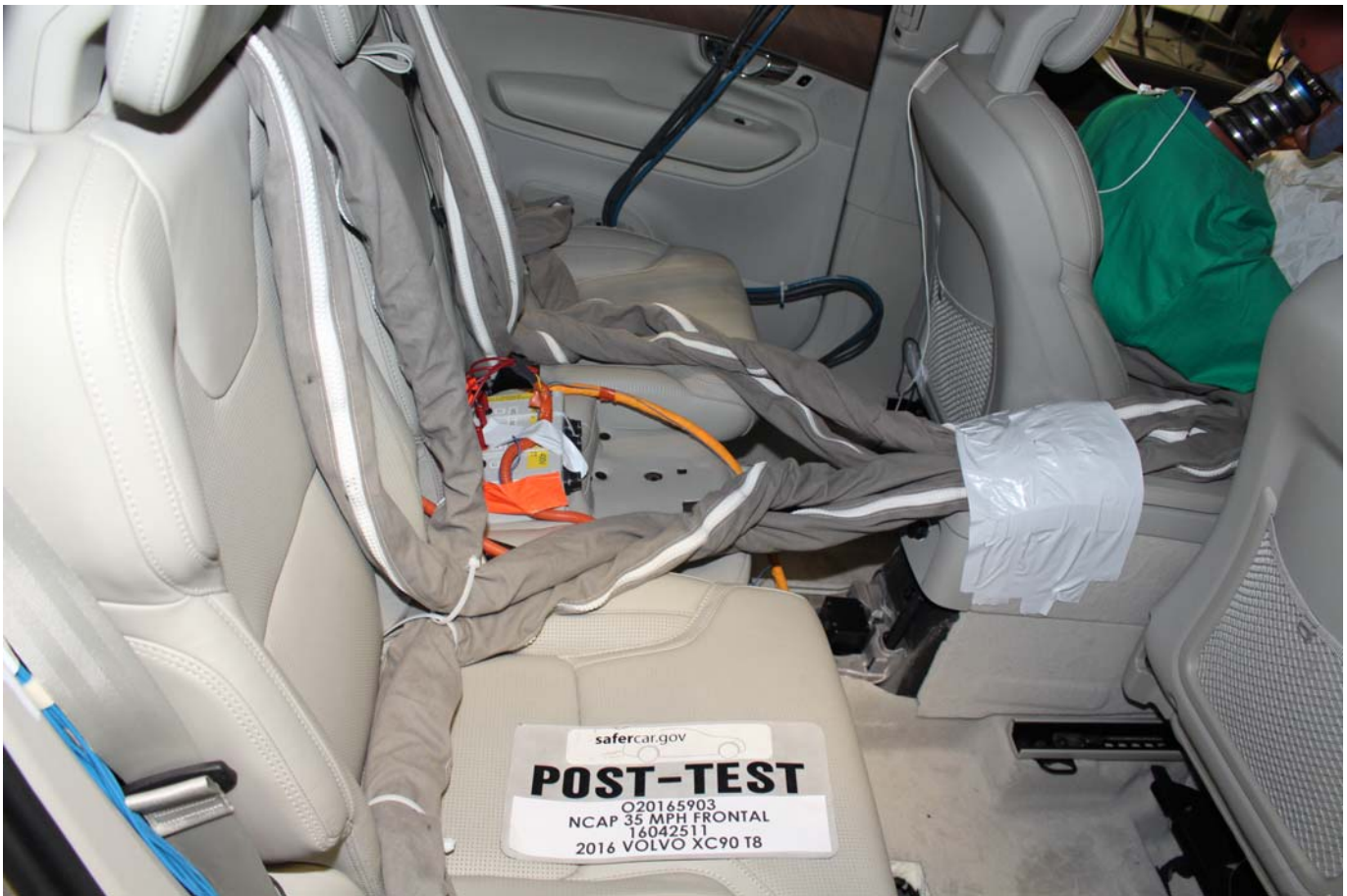
Photo No. 029 - Post-Test Dummy Cable Routing
