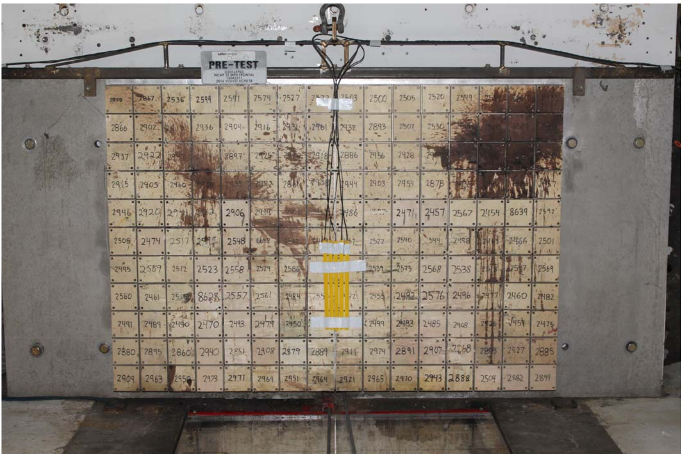
Photo No. 002 - Pre-Test Load Cell Wall
