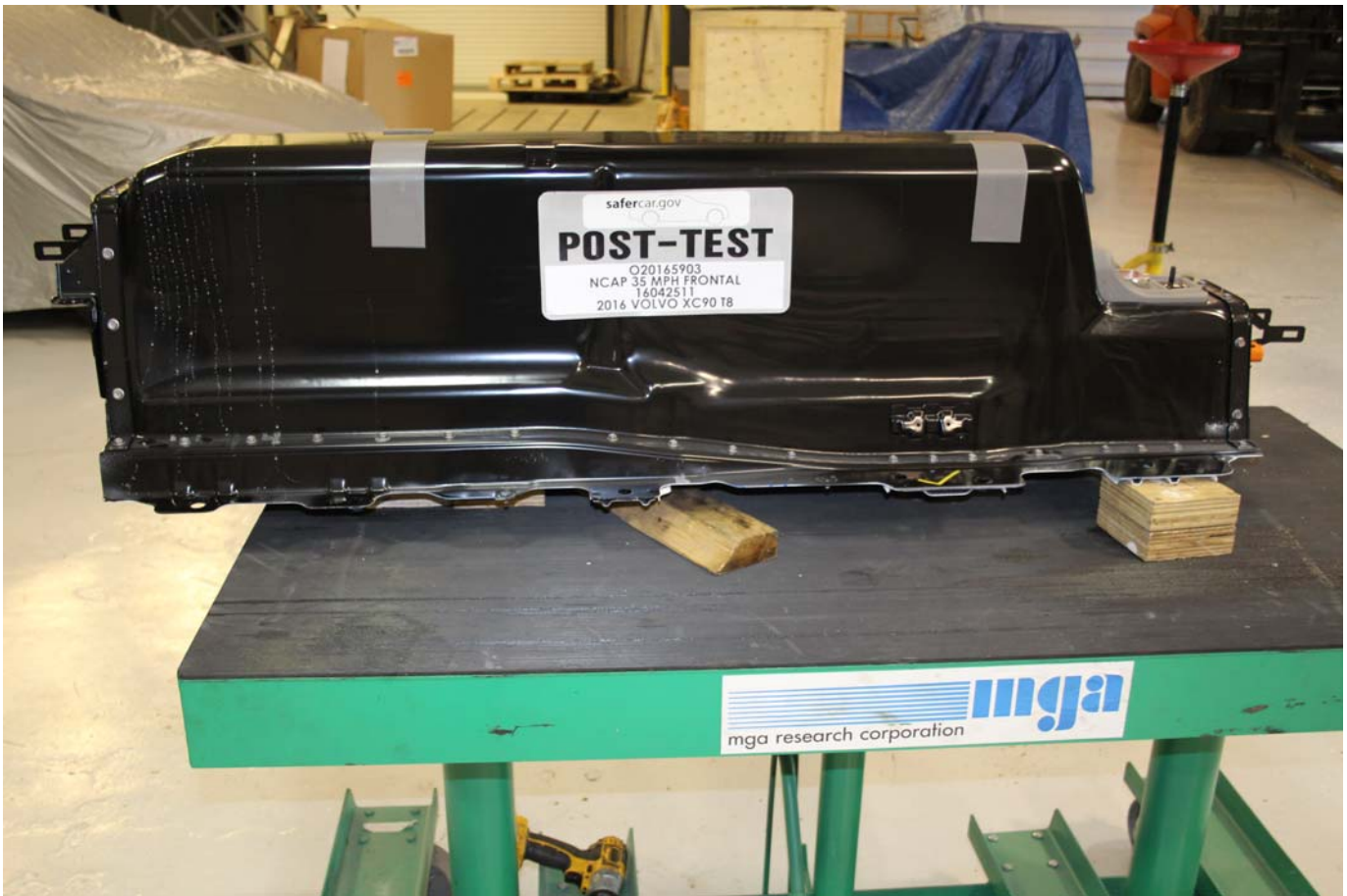
Photo No. 012 - Post-Impact View of Battery Box(s) or Container(s) Which Holds Individual Battery Modules
