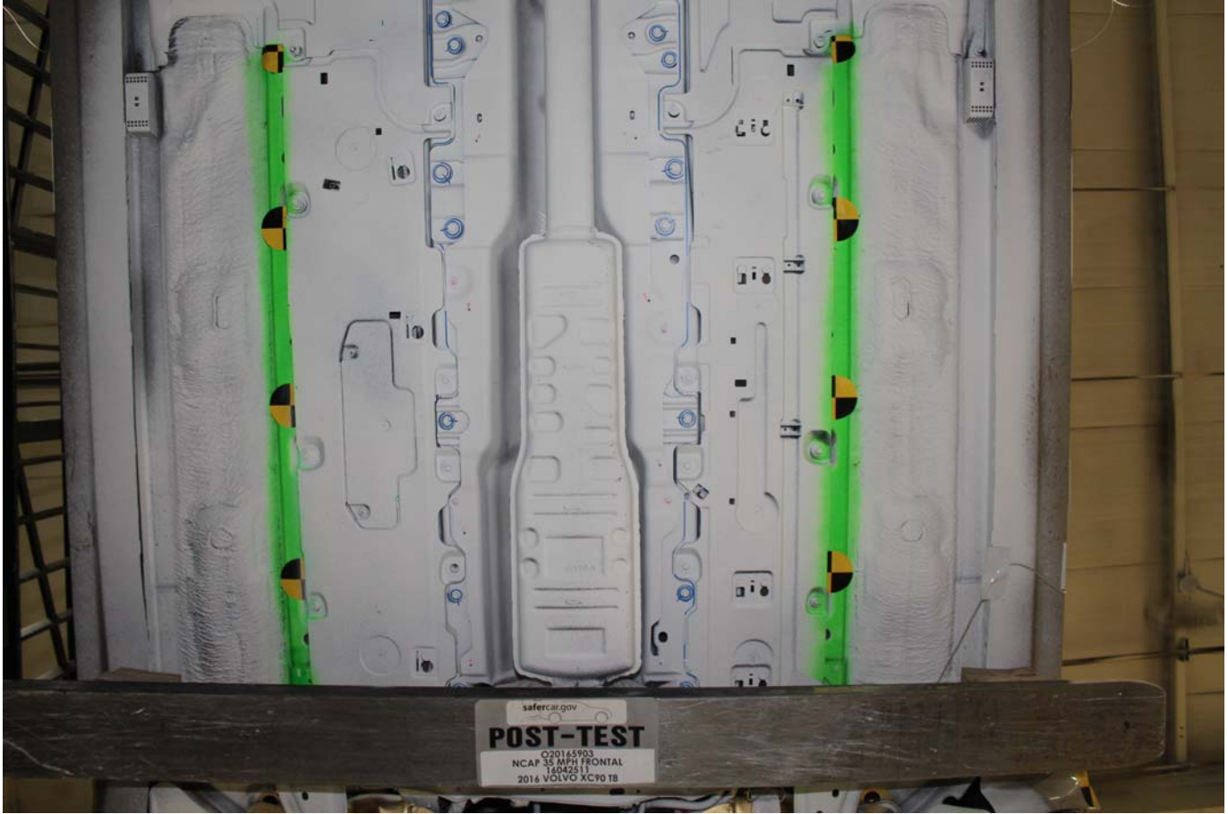
Photo No. 033 - Post-Impact Propulsion Battery System Mounting and-or Intrusion Failure(s)
