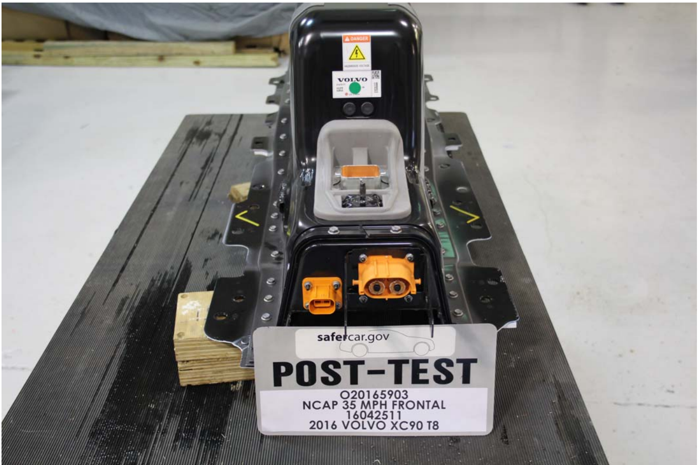
Photo No. 010 - Post-Impact Rear View of Propulsion Battery
