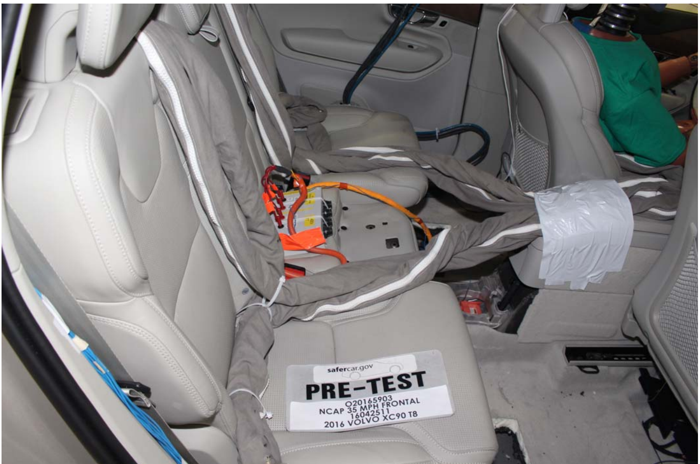
Photo No. 031 - Pre-Impact View of the Vehicle Passenger Compartment Adjacent to Propulsion Battery
