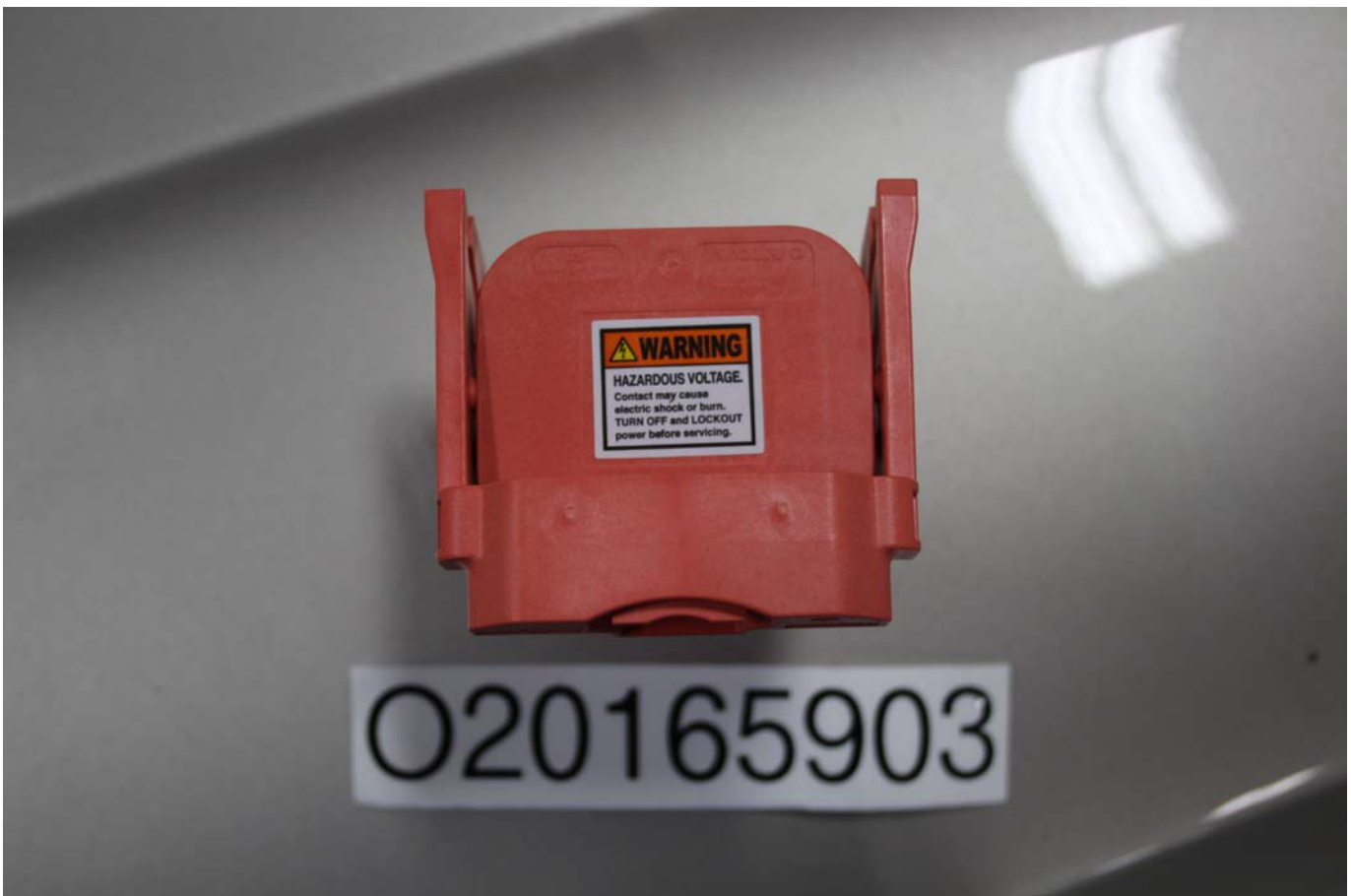
Photo No. 007a - Manual High Voltage Service Disconnect Removed
