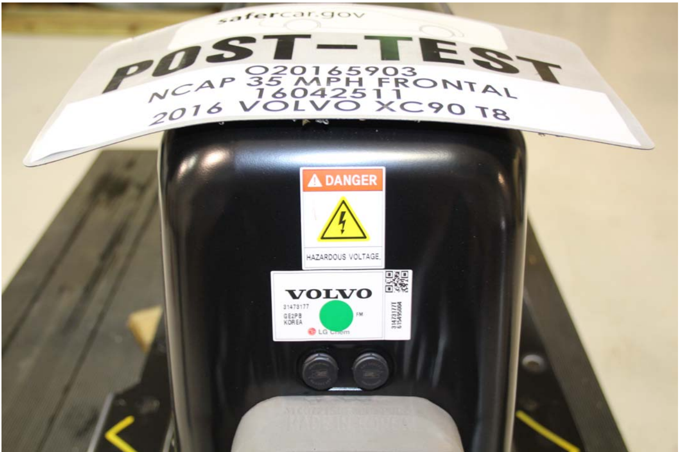
Photo No. 001 - Auxiliary Power Module Warning Label
