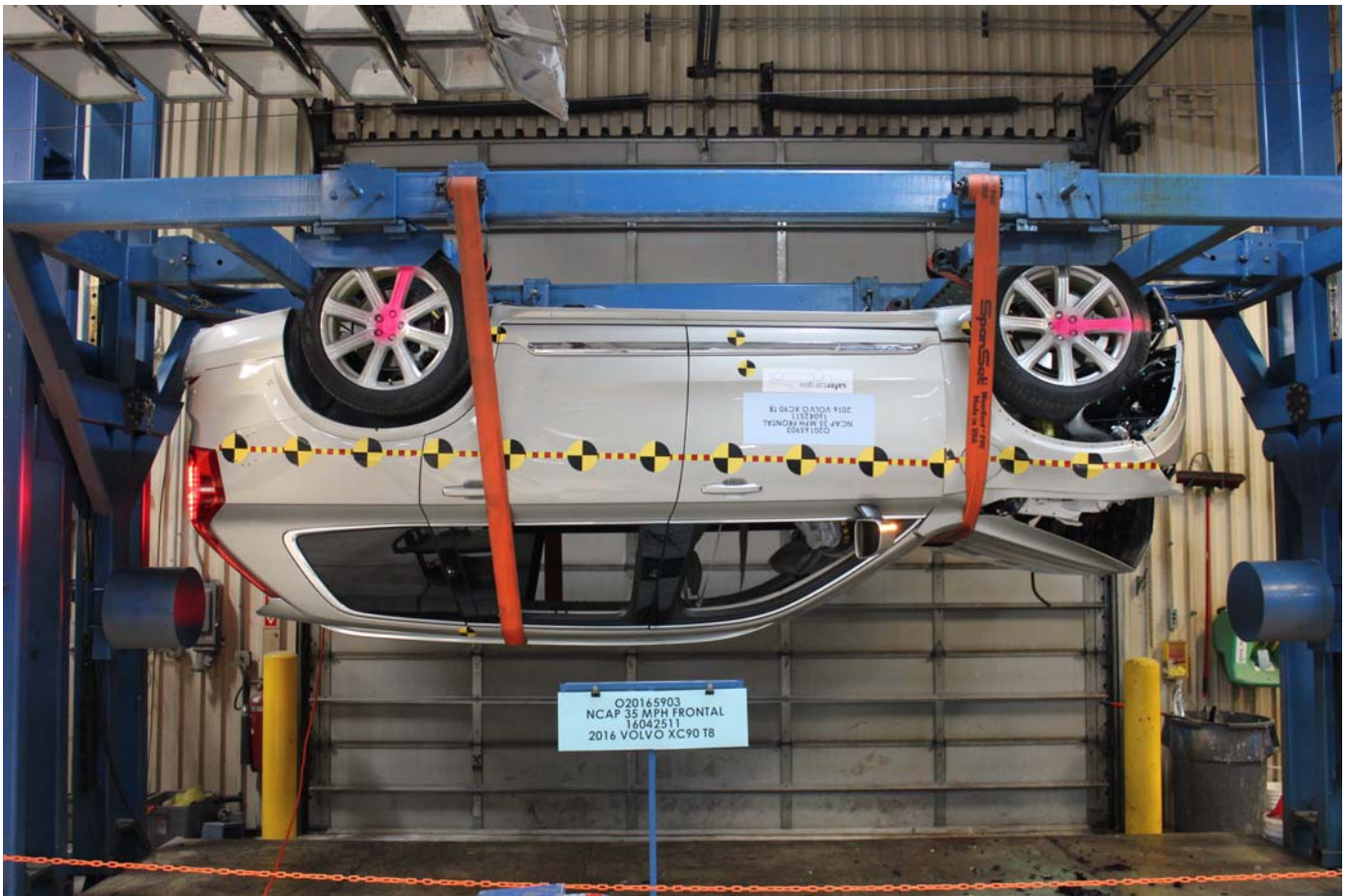
Photo No. 028 - FMVSS No. 305 Static Rollover at 180°
