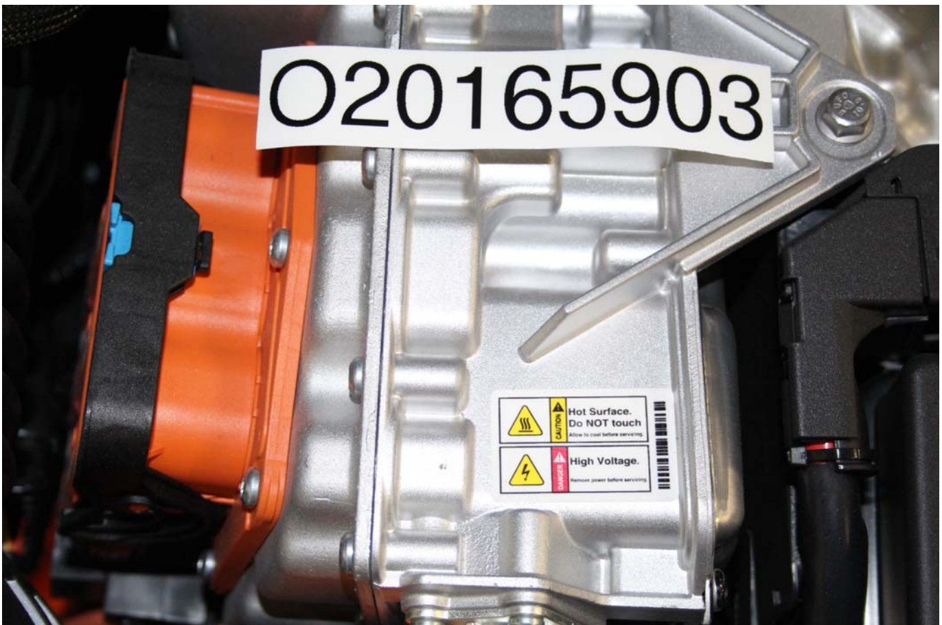
Photo No. 002 - Power Inverter Warning Label
