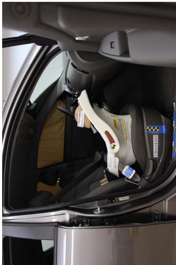
Cosco Arriva WOut Base, Belted, Rear Facing, Middle Seat Track
