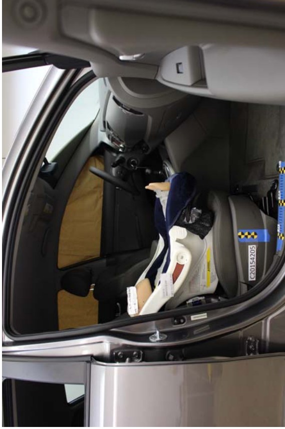
Cosco Arriva WOut Base, Unbelted, Forward Facing, Rearward Seat Track
