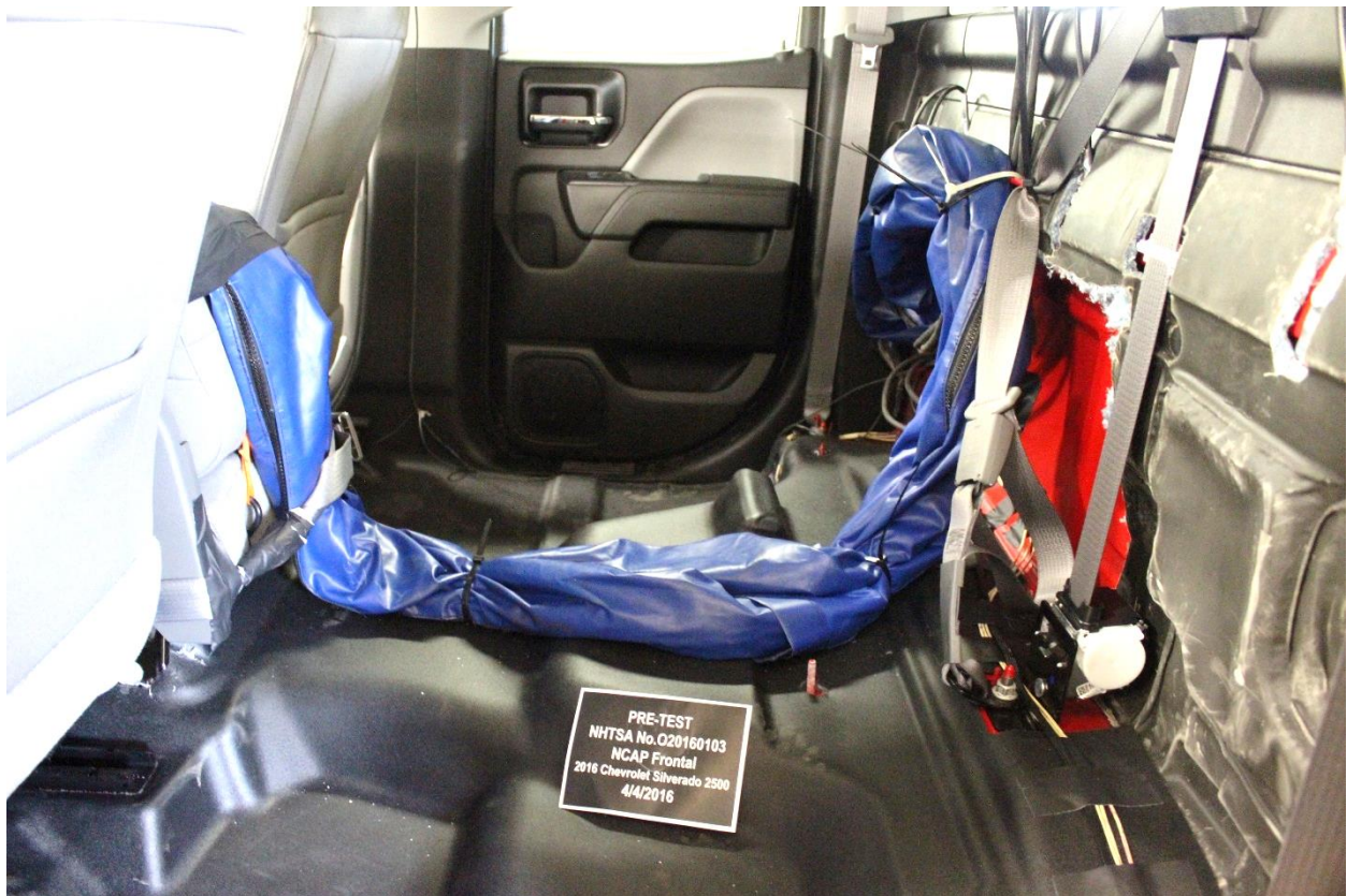
Figure A-28: Pre-Test Dummy Cable Routing
