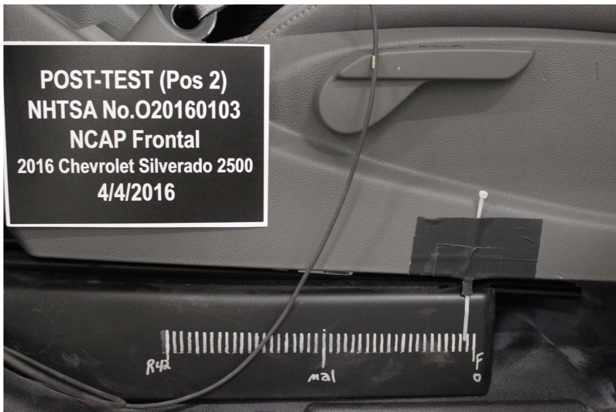
Figure A-58: Post-Test Passenger's Seat Fore-Aft Markings (Plastic Moved not Seat track)
