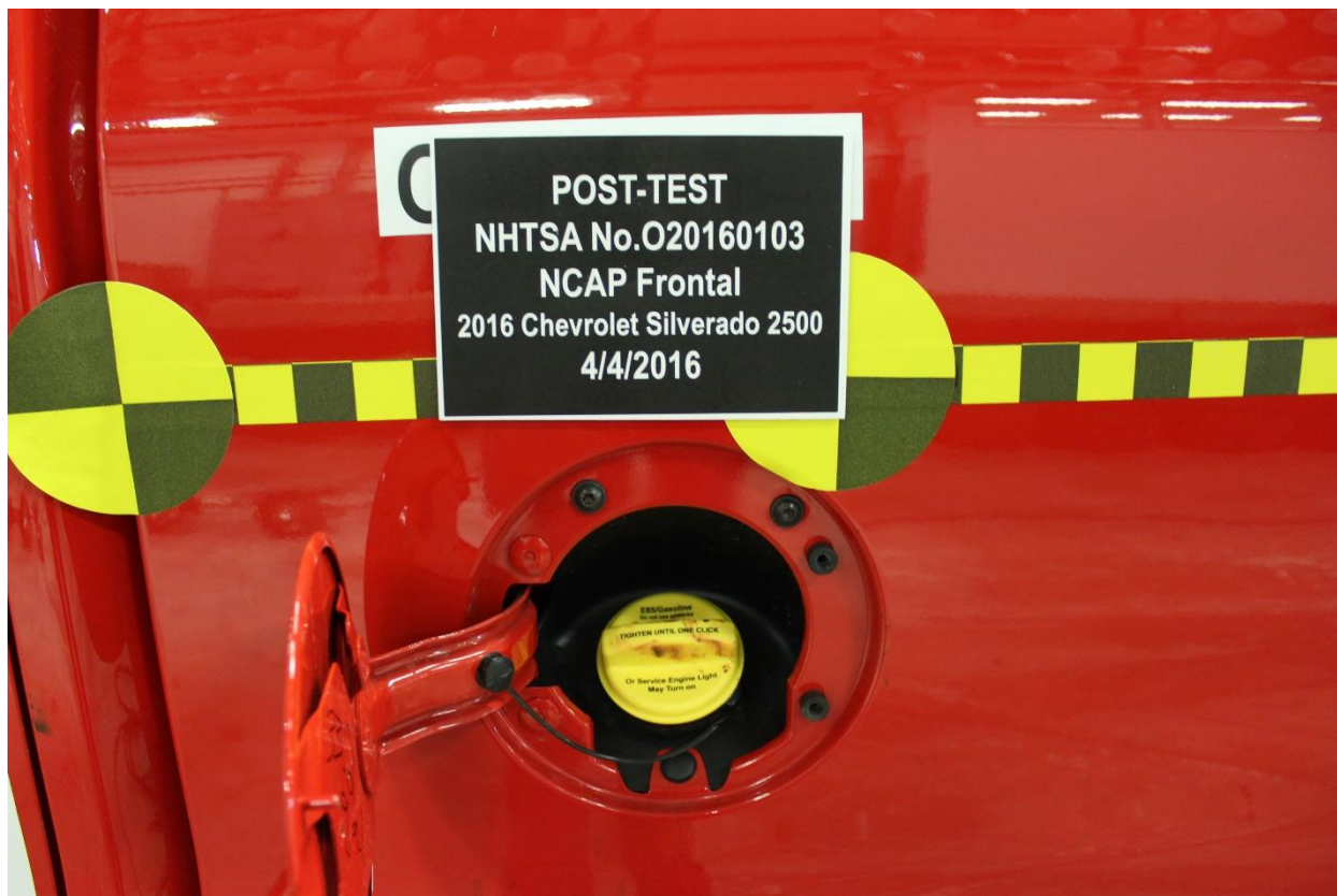
Figure A-23: Post-Test Fuel Filler Cap View
