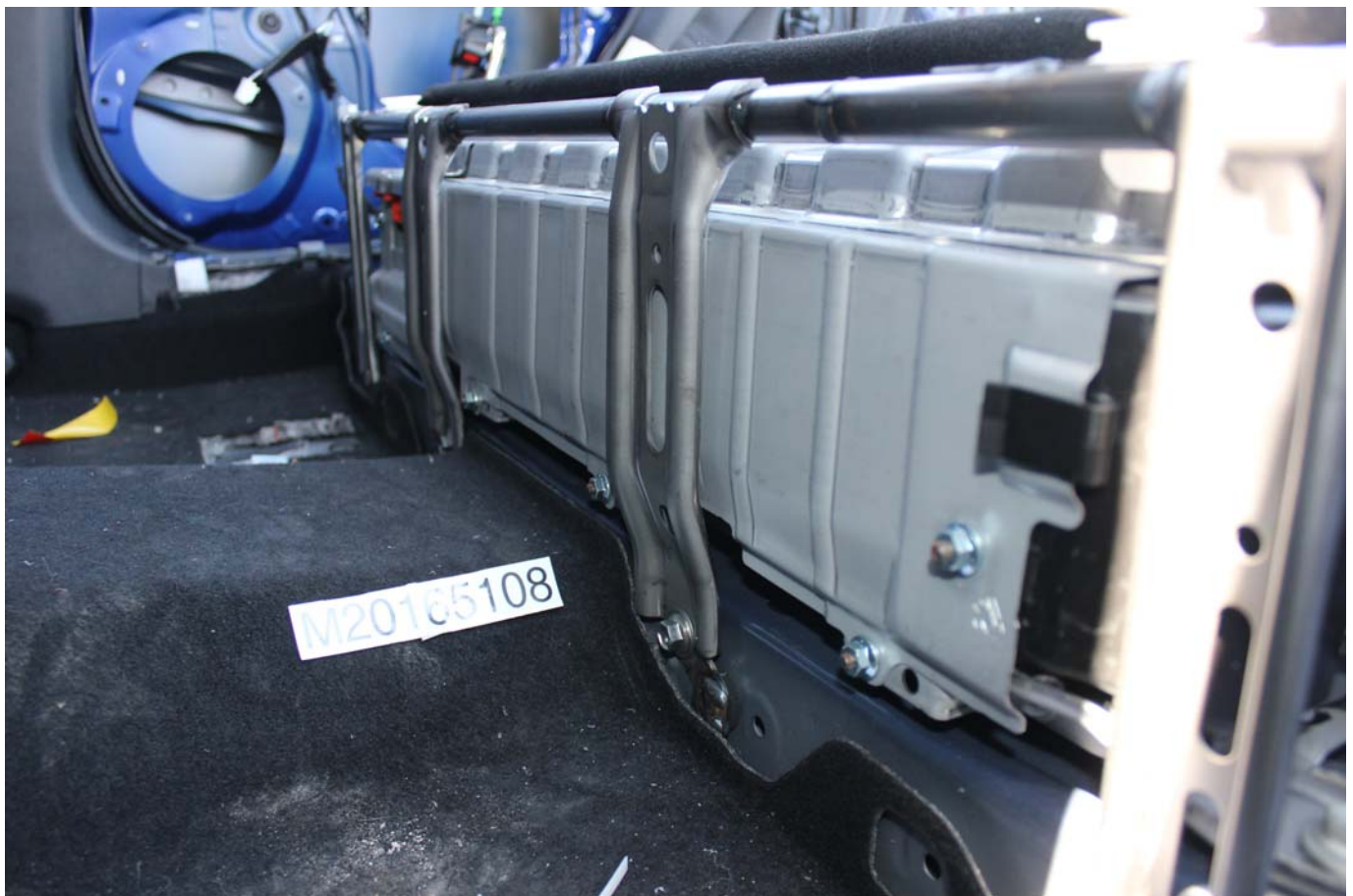
Photo No. 009 - Post-Impact Front View of Propulsion Battery
