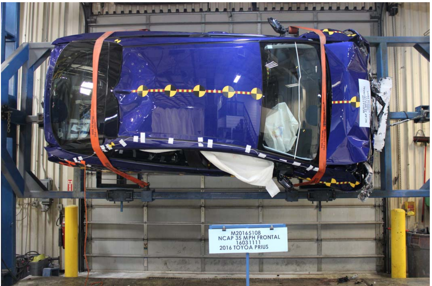
Photo No. 029 - FMVSS No. 305 Static Rollover at 270°
