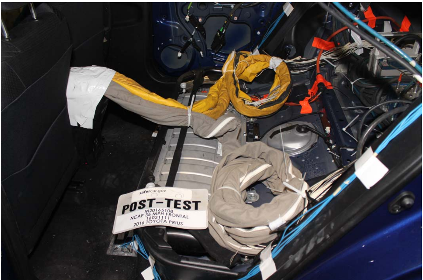
Photo No. 029 - Post-Test Dummy Cable Routing
