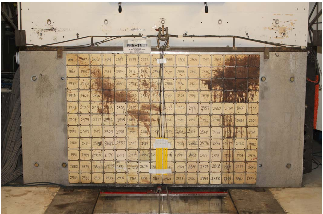
Photo No. 002 - Pre-Test Load Cell Wall
