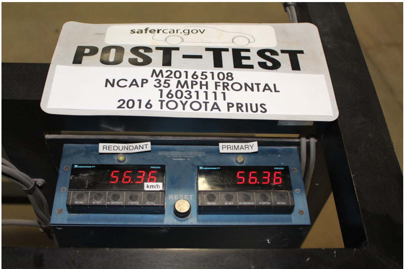
Photo No. 072 - Post-Test Speed Trap Read-Out
