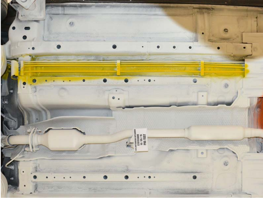
FIGURE 29. Pre-Test Underbody View of Fuel Lines
