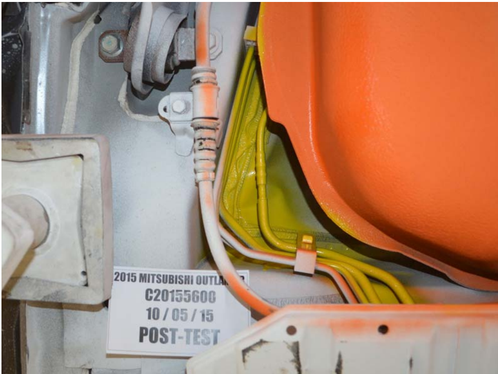
FIGURE 32. Post-Test Underbody View of Fuel Lines
