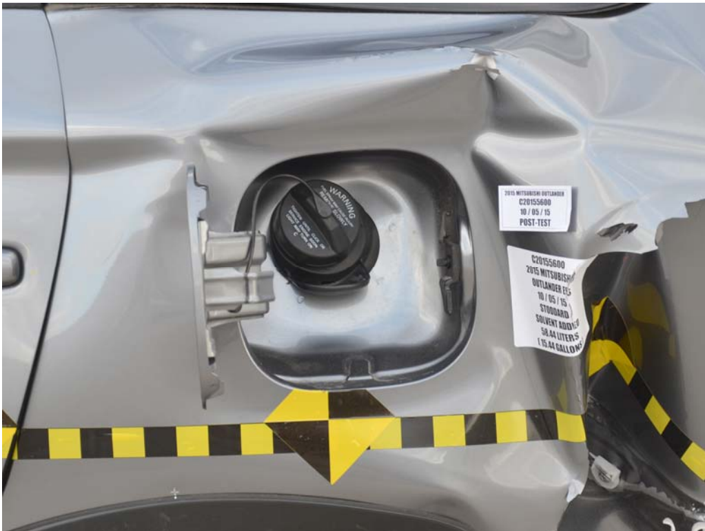
FIGURE 24. Post-Test View of Fuel Filler Cap
